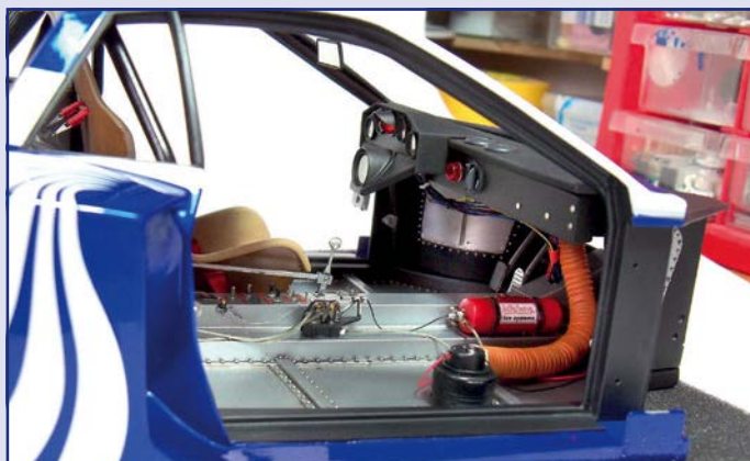
A view into the centre section of the model, revealing the orange ventilation hose, fire extinguisher and switch gear
