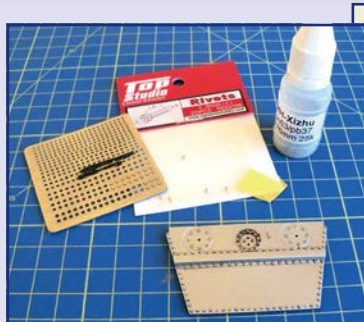
The 'aluminium' chassis, fuel tank and the interior rivets were recreated with 0.5mm and 0.7mm solder balls, convincing and cost-effective solution. In certain areas, Top Studio and MasterClub rivets were used
