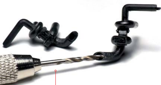
The exhaust outlets were drilled out – very carefully – using a drill bit of an appropriate size
