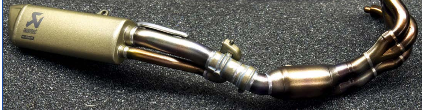
Careful masking was applied to very tip of the exhaust exit and then airbrushed in steel to give a clean visual separation of metallic components
