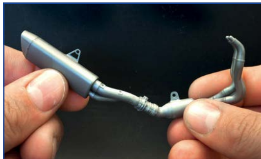
The whole exhaust was built up and ensured all located as intended. Be careful of the lower middle collar piece on fitment as it's a very tight fit
