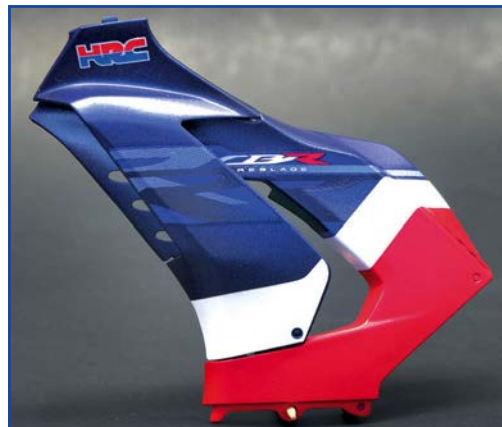
The completed panel pre-clear. All panels are now ready to be sealed in
