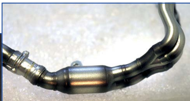
Each weld line was carefully and thinly airbrushed over with transparent smoke to give depth and once the masking is removed - a defined line
