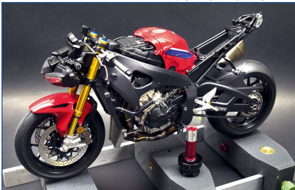
The completed frame with all mechanical parts fitted prior to being closed up by the fairings
