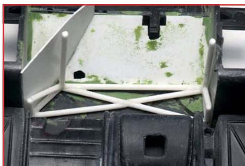
Structural elements in the footwell were recreated with pieces of extruded polystyrene rod
