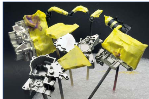
Many of the parts have already been painted and then masked accordingly ready for the final Zero Paint stages
