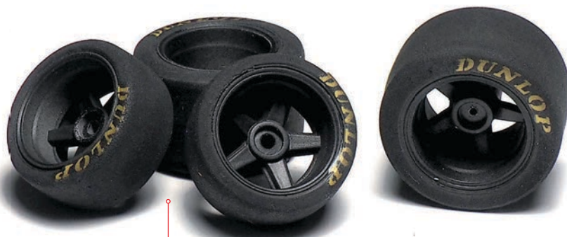
The author sanded the tyre treads by mounting them on an old rim attached fitted in the mini drill, levelling the entire surface including the shoulders, to remove mould marks
