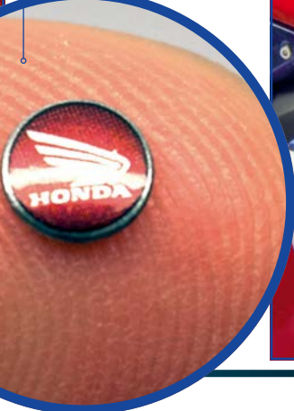
Both Honda badges took a little work: a gloss black base followed by Zero's Chrome silver, the opaque logo decal applied then a gloss clear to seal
