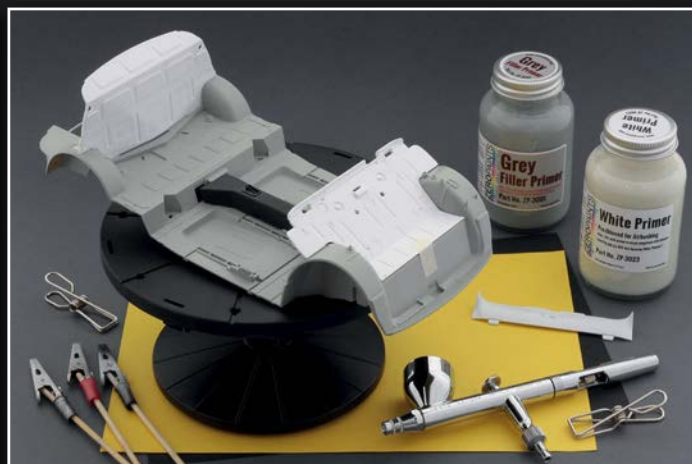
Zero Paints White Primer and Grey Filler Primer were used as undercoats to seal in the raw polystyrene of the kit mouldings
