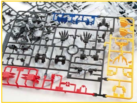
One of the sprues is moulded in several colours, demonstrating the expertise of Bandai in moulding. The parts are very finely detailed
