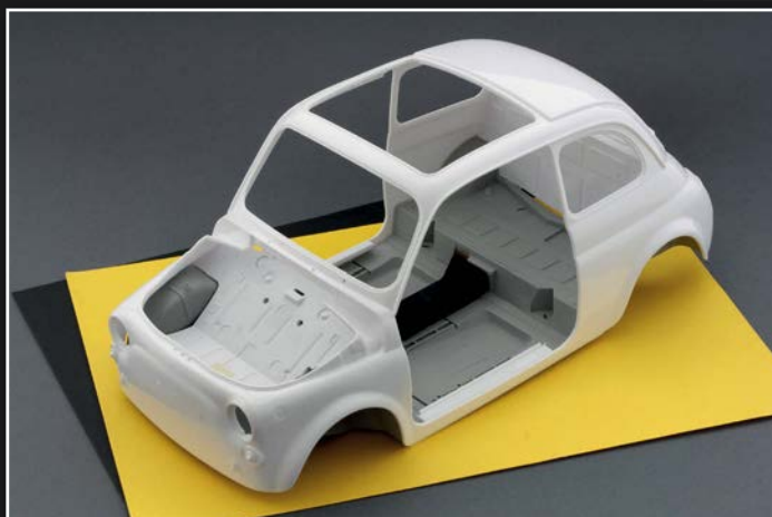
The bodyshell is checked for fit over the lower floor panels
