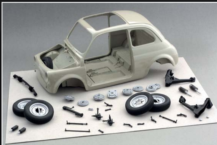
In this view, the brakes, wheels and suspension components are spread out, ready for installation
