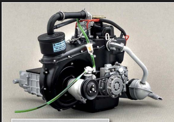
Views of the Fiat's 499cc air-cooled engine, with plumbing and wiring fitted. Italeri have made a perfect replica of this tiny powerplant
