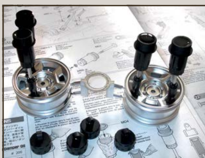
Using the Land Rover wheels to hold the shocks whilst the air rises to the top
