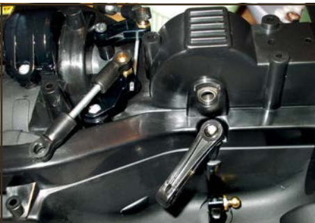
The upper link area is fiddly so it's recommend to build the assemblies first then pop the ball joint on
