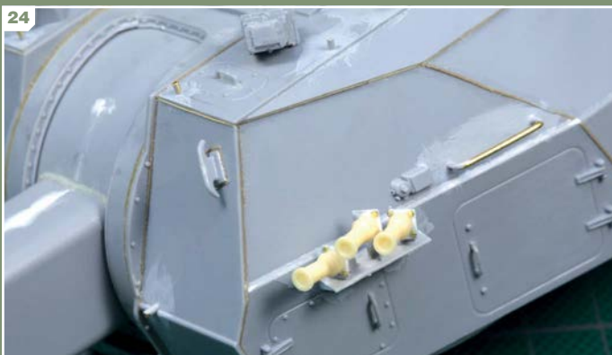
24. We can clearly see the welds along the joints the large panels constituting the turret, made from stretched sprue. It certainly takes time, but what satisfaction and realism they will create after painting!
