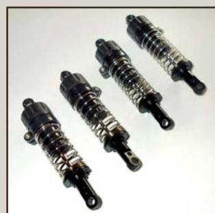
The CC-01 comes with oil-filled shocks with sliding collars for ride height adjustment
