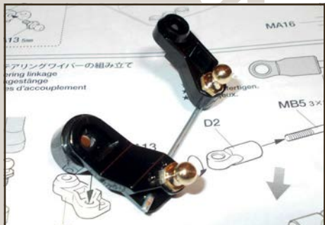
The steering bell-cranks are quite small for the size of model
