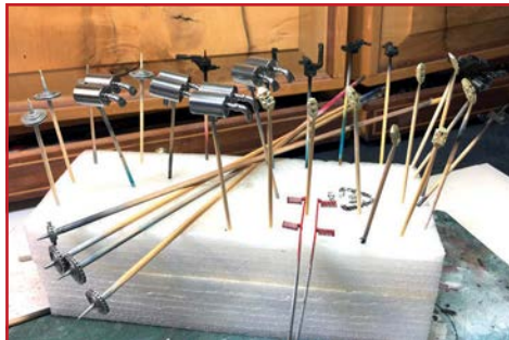
All the brake and suspension pieces were painted together, along with the exhaust ends. Extra pieces were painted up to compare between the HD and ST27 sets
