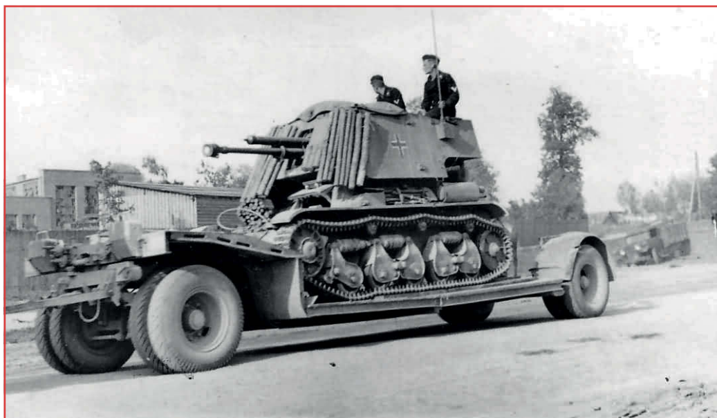
A 4.7cm(t) Panzerjäger auf 35R(f) being moved on a trailer. In this combination, the base tank is French and its new gun is of Czech origin. It would be nice to think Tamiya might release a kit of this Wehrmacht-modified variant in the future. Photo: Bundesarchiv
