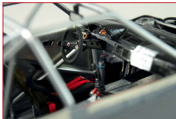
Electronics boxes were treated to some Scale Motorsport CF decals and then matt clear-coated with Tamiya X-86 Flat Clear before the additional wiring was added
