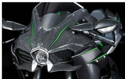
Decals are included to recreate the upper cowl carbon fiber, while clear parts are used for headlight and position lights.
