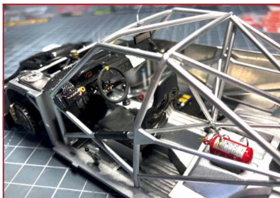
Practically invisible once all assembled, the anti-roll bar levers are works of art in their own right. Multiple PE pieces and handles cut from the original kit parts make up the assembly
