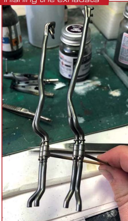
The main sections of the exhaust pipework were glued together before painting. This allows for any joints to be eliminated and give a smoother look
