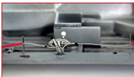
Practically invisible once all assembled, the anti-roll bar levers are works of art in their own right. Multiple PE pieces and handles cut from the original kit parts make up the assembly
