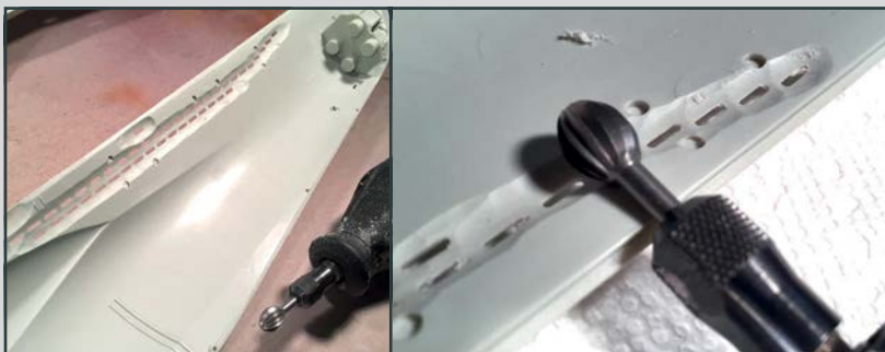
Work began by drilling out, filing and thinning the spillage port holes and their surrounding plastic
