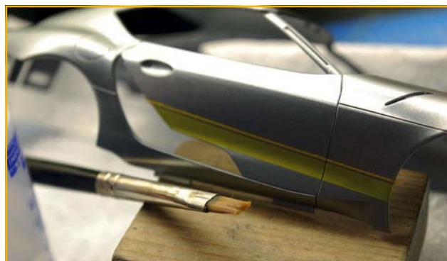
The author found a single layer to be a little transparent, so a second layer was applied directly over each line for more solid finish
