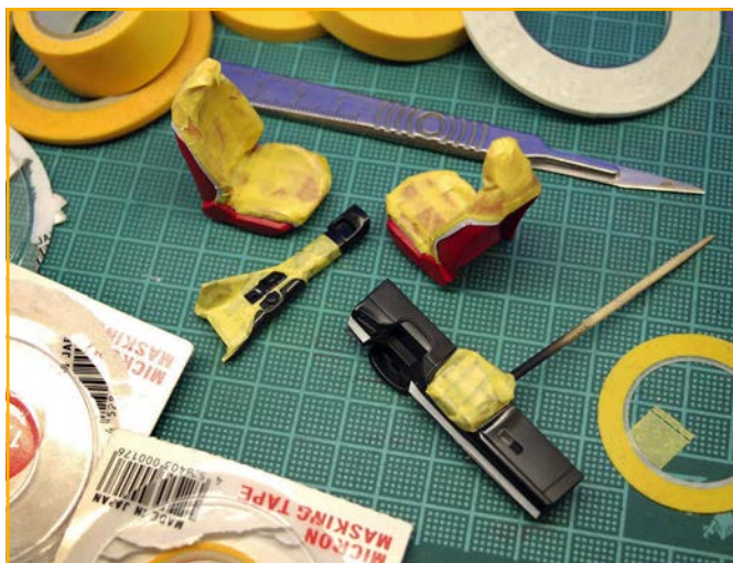
More masking for black parts. The centre console was particularly time consuming as the exposed areas would be matt in finish compared to the covered which remained gloss
