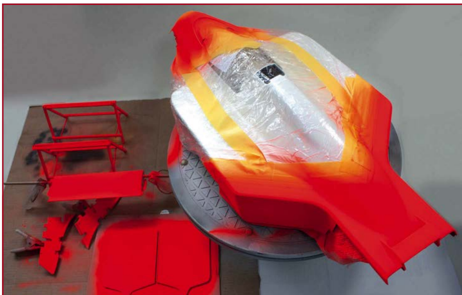
A masking tape template was made for the positioning of the chevron as an insurance policy for repainting. This wasn't needed in the end, but better to keep a physical template in case
