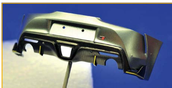
The diffuser was dry-fitted after all of the carbon-fibre work was applied. A real task but well worth the time taken. This will be gloss cleared to contrast against the body
