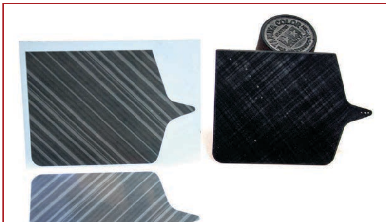
The author made a mask to spray light grey and black through, to create the fine carbon weave effect on the wing uprights, simply cutting a hole in card and used sewing thread and thin masking tape in a random parallel diagonal layout. The real life texture is varied and more random than the uniform decals which I chose not to use. The sprayed texture was tied together with the stiff brush/white pastel technique again. Above right: The close up comparison of the printed decal and the author's personalised result. Both of these are head and shoulders above the kit finish of uniform plain black
