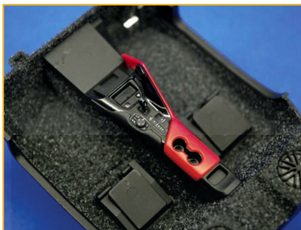
Zero Designs Charcoal colour flocking was the desired route to replicate the carpet material
