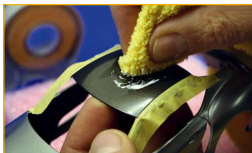
Once cured, the roof was sanded smooth then hand polished to a showroom shine using Scholl Concepts machine compound
