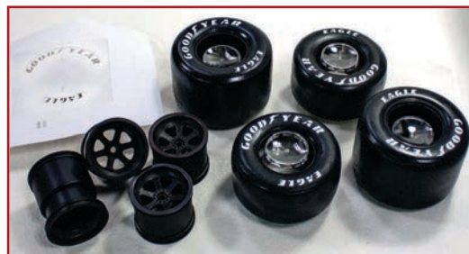
The tyre logos were sprayed using stencils from Autograph. Much more true to life than the kit supplied finish
