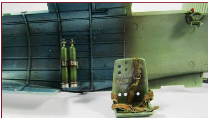
The left-side fuselage half showing the aotake coating and seat with HGW harness
