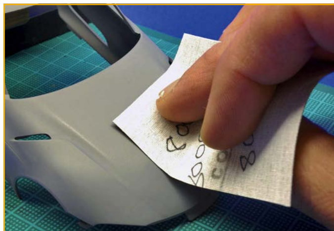
After priming with Zero Paints, the body was left to cure then sanded smooth with various grades of abrasive to ensure the main colour work laid down evenly
