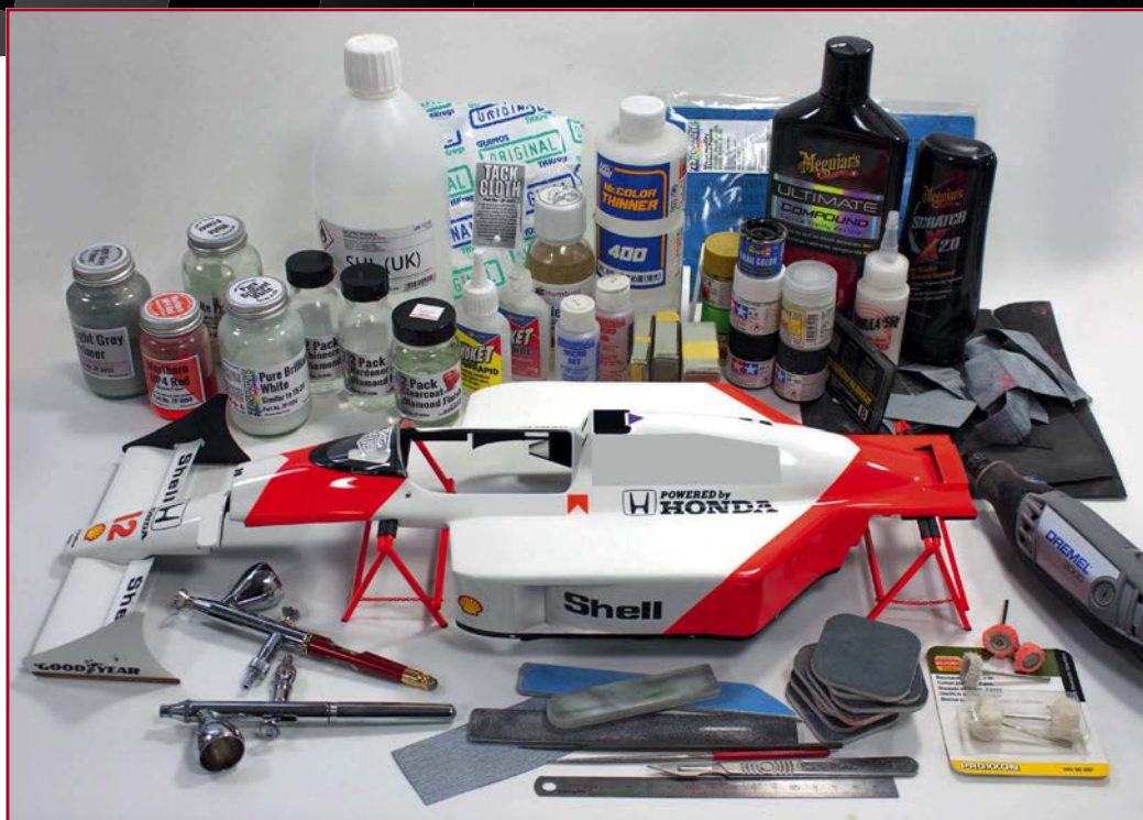
This is the tool kit needed to create the finish on the body work alone. All in one place it looks intimidating, but look closer and it's not that daunting. Everything here is readily available and has been used previously by many authors within the pages of TMMI. The daunting aspect of the kit is its size. It likes to drink paint, and you get a real work out sanding!
