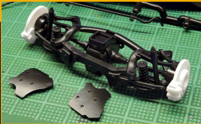
A dry-fit assembly of the rear differential and suspension set up
