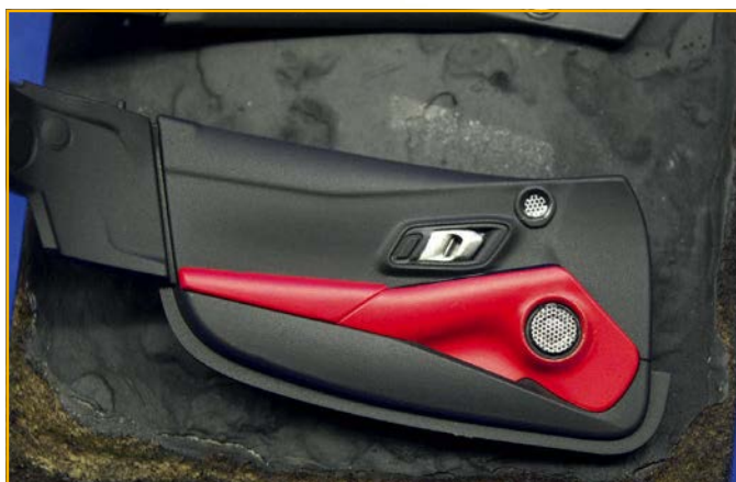
Door card work. This area comprises two decals for the speaker covers; the arm rest is a separate part, thankfully, making paint application much easier. The rest was hand painted
