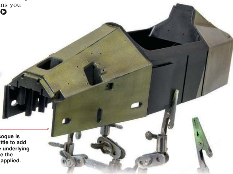
Base coating the monocoque and ducts with metallic grey and smoke. Then on the monocoque alone, clear yellow, with a gloss layer sprayed to prepare for the decals.
