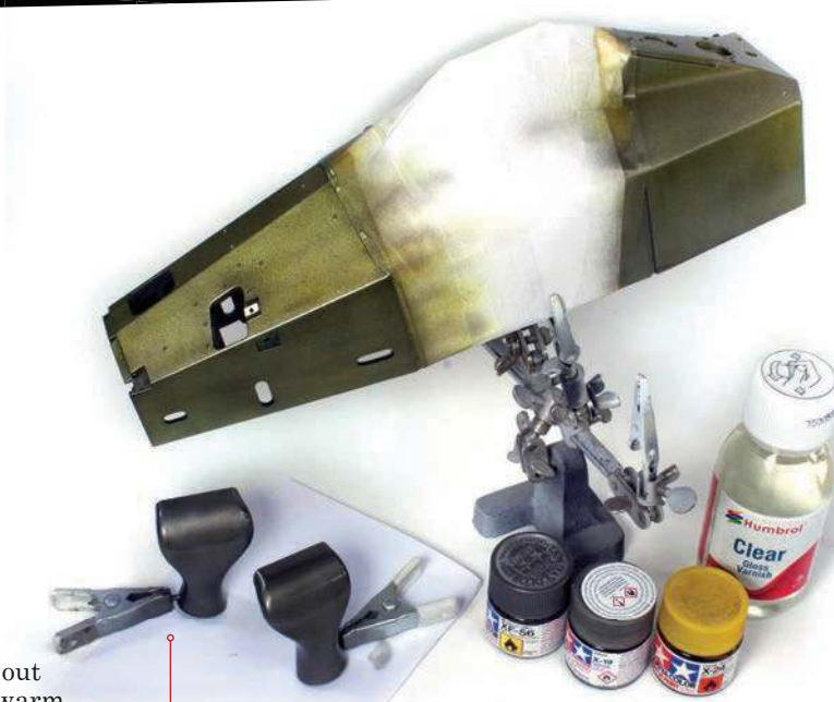
Base coating the monocoque and ducts with metallic grey and smoke. Then on the monocoque alone, clear yellow, with a gloss layer sprayed to prepare for the decals.
