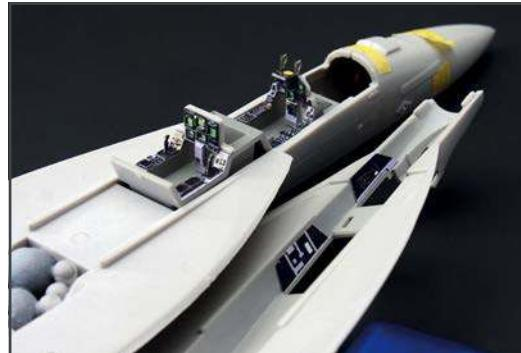
A view into the cockpit before the upper and lower fuselage halves are mated. Note the lead-shot weights to keep the nosewheel down
