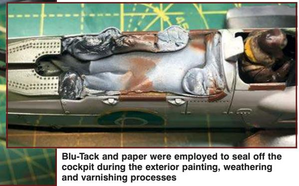
Blu-Tack and paper were employed to seal off the cockpit during the exterior painting, weathering and varnishing processes
