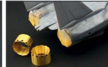
The engine cans await fitting while the airframe is sprayed
