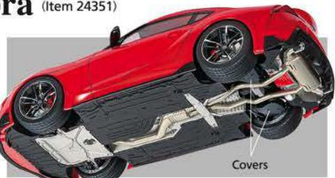
The car's extensive underpanel is depicted, as are front and rear suspension, plus rear arm aero covers.
