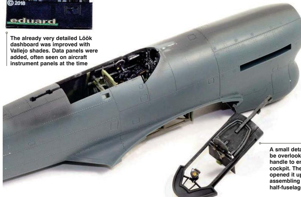
A small detail not to be overlooked: the handle to enter the cockpit. The author opened it up before assembling the half-fuselages
