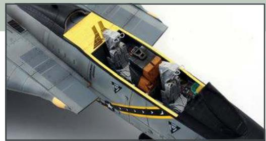
An unpainted photo-etched cockpit frame has been placed over the painted aperture to show where it fits
