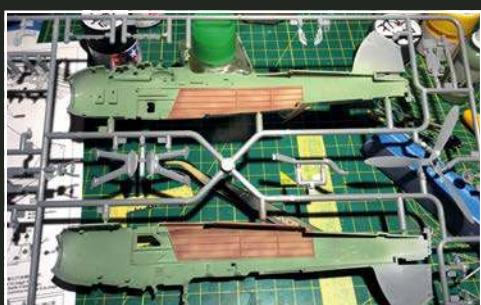
The fuselage interior walls have been painted XF-71 Cockpit Green, with natural wood-coloured areas in the lower section
