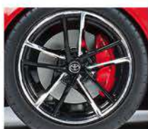
Two-part wheels feature metal plated component.
