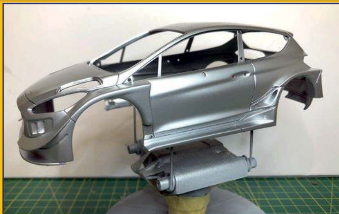
Body painted in Zero Metal Aluminium and cleared with 2k Diamond Clear
