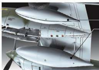
P-38Gs which took part in Operation Vengeance carried one each of 150- and 300-gallon tanks.
