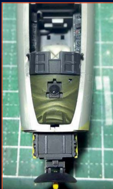
Looking directly down into the cockpit aperture, we can see the fabric-textured instrument coaming, radar gear in the nose and the pilot's side-consoles
