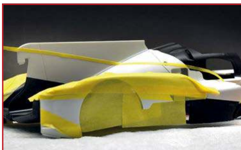
To ensure the lines matched across all panels, the sections were dry fitted and then marked off using Aizu's 1.5mm masking tape. Anything that isn't going to be red is sealed away leaving the latter exposed
