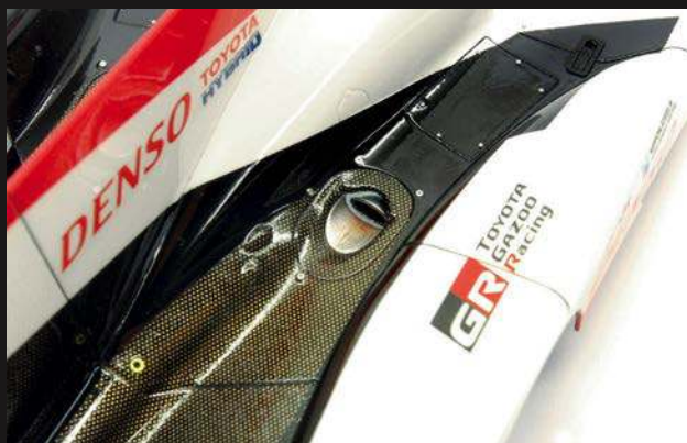
The completed clam with 0.5 and 0.75mm rivets added, carbon work, weathered exhaust heat shield and Blue Stuff decal infills
