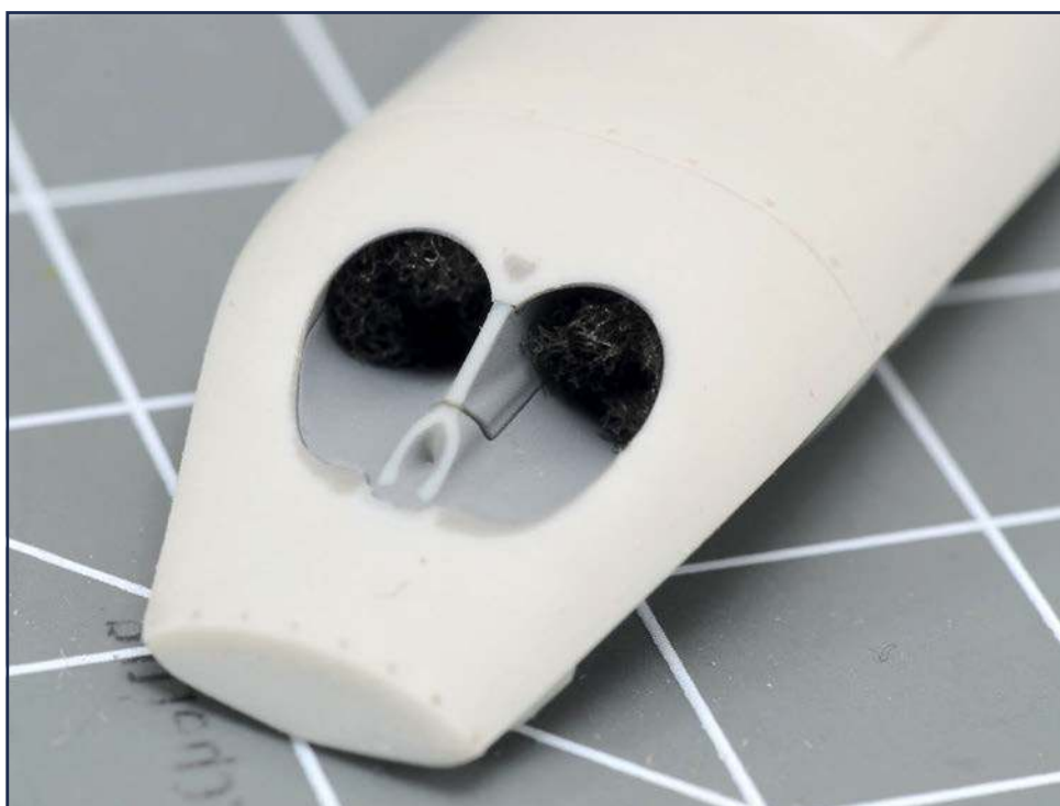
One the intake units had been painted and assembled, small pieces of rubber foam were pushed into the apertures to protect the inner during airframe painting
