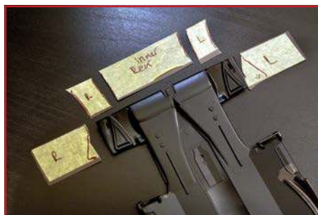
All self templates required to carbon the rear panel sections. This was a really involved process where particular attention had to be paid to weave direction and pattern joining
