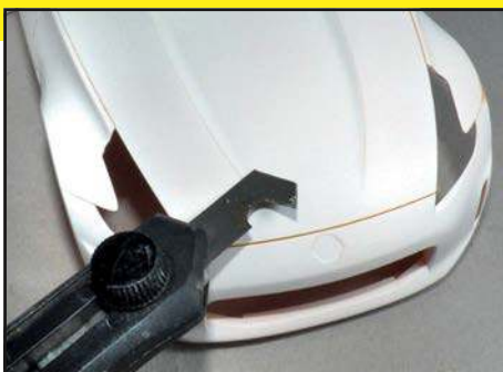
After applying Tamiya white primer, the shut-lines were deepened with the Tamiya engraving tool, to avoid filling them with the layers of paint that will follow
