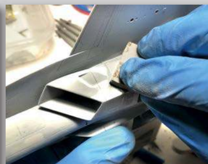
Filling and sanding delivers a seamless result. It's a hard and long process of fitting air inlets and other additions
