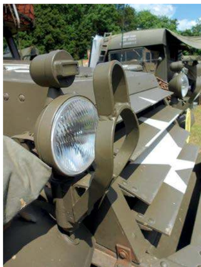
Detail shot of the lefthand side road light and night formation lights, which utilise a late-style guard unit with a double loop form, replacing the simpler single 'D' form of earlier variants
