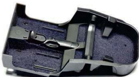
The floor of the cockpit was covered with Spotmodel flocking. To fix it, LP-24 Semi-Gloss Clear was applied by brush on the parts to be treated. The flocking was sprinkled in place and the 'carpet' texture obtained is very convincing
