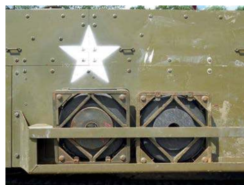
The side-racks were most frequently used to hold mines but were soon filled by crews with their personal gear
