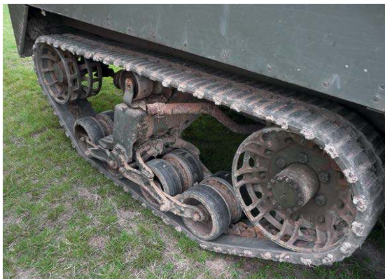
A study of an early bogie system showing the rubberised one-piece track, idler, drive sprockets and wheels. After combat in North Africa a large spring-loaded assembly was added to the rear idler construction
