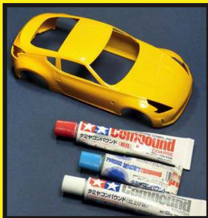
The body was polished with the three Tamiya Compounds in descending order of grain coarseness, before applying layer of Tamiya Modelling Wax with a microfiber cloth
