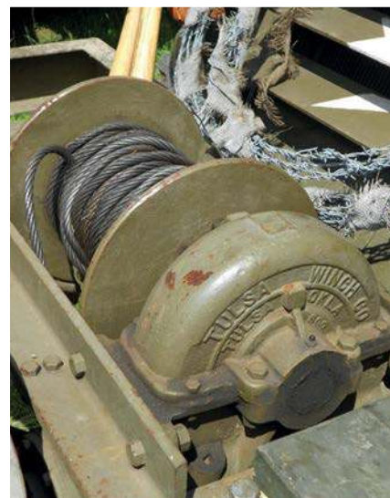
Detail shot of the front winch assembly. This unit had a control lever to the lefthand side for engaging/disengaging the engine clutch during operations. It is said that only one in four M3s had this winch unit
