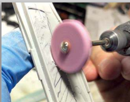
Using a motor-tool with a grinding disc, the fuselage inner walls were thinned, for the resin parts to fit. Always wear a mask and eye protection when doing this
