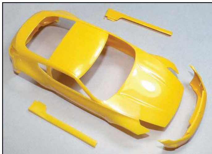
The component parts of the bodywork must be cemented together securely, in order to avoid breakage during installation on the chassis
