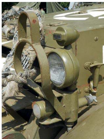
The right side of the same M3 with similar lights and guard construction but with the addition of a traffic horn below the set up
