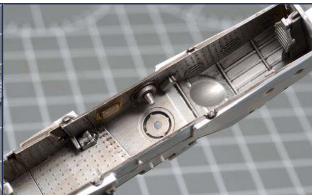
As with the front undercarriage bay, the main bay parts were disassembled and treated to some weathering. Tamiya Panel Line Accent Color 'Dark Brown' was used here to create oil stains and a general film of dirt
