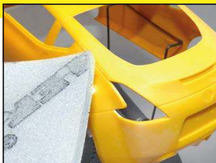
Minor traces of moulding joints were erased with Tamiya abrasive sponge (2000 grit)
