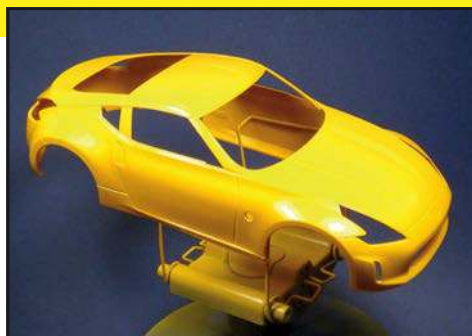
Four layers of TS-47 Chrome Yellow were applied to the body, then left to dry for about a week
