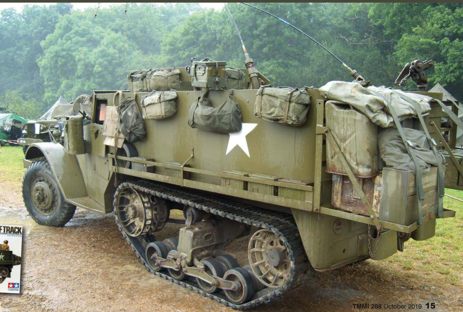
A heavily laden M3 plods its way down a muddy path during the War and Peace show in Kent. Of note are the handy fold-down stowage racks, weighed down with the crew's stowage and jerrycans
