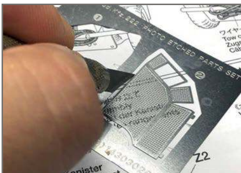
The 2007 edition of this kit came with a fret of photo-etched metal for the turret grenade screens; they are seen here being trimmed from their fret
