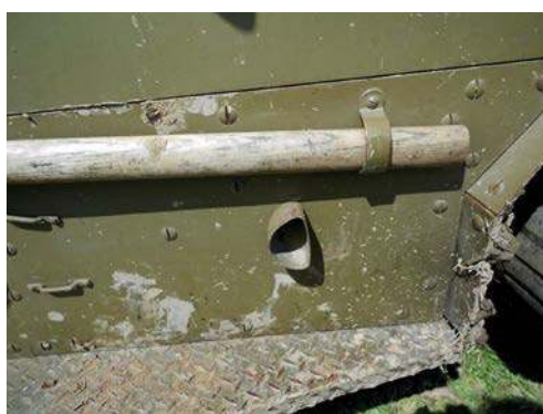
Close-up view of the cabin door, showing the steel-bar tie-downs and large, slot-headed screws used in the M3's construction
