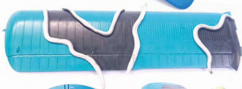
White-Tac sausages are an easy method for masking
