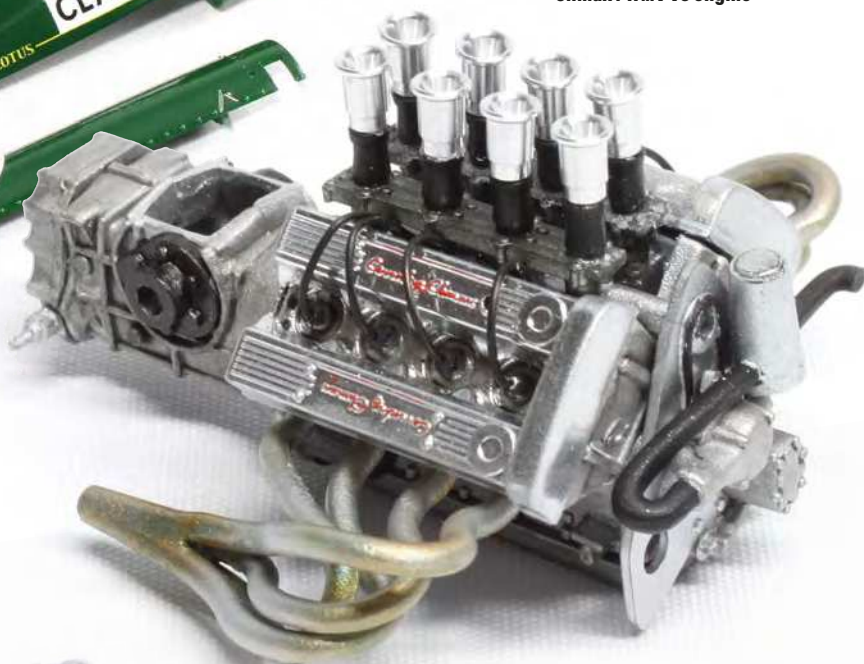
The excellent Coventry Climax FWMV V8 engine
