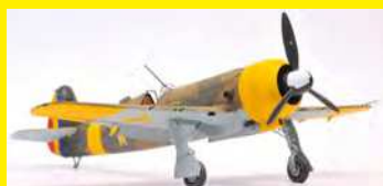
Master modeller Brett Green chose SAC gear for his 1:32 IAR-80A for additional strength and because white metal allows the angle of the gear to be adjusted even after the legs have been glued in place.
