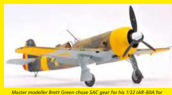
Master modeller Brett Green chose SAC gear for his 1/32 IAR-80A for additional strength and because white metal allows the angle of the gear to be adjusted even after the legs have been glued in place.
