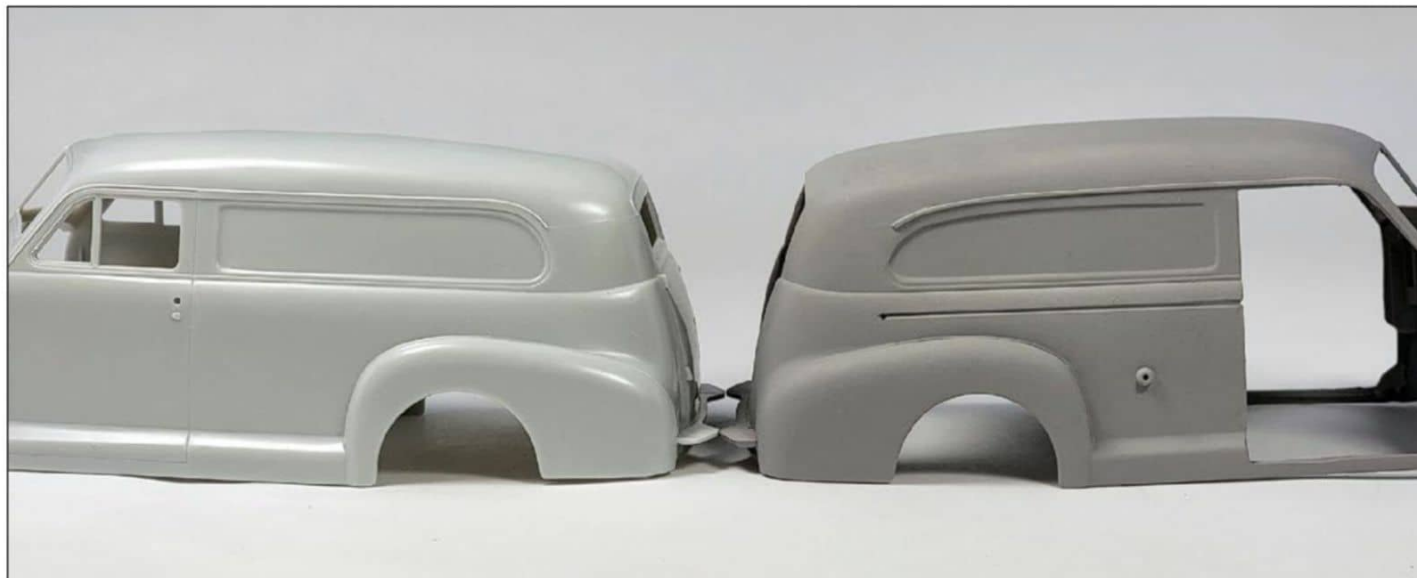
A comparison of the corrected body-side indent shown beside an example of the Galaxy kit's original sedan delivery body.
