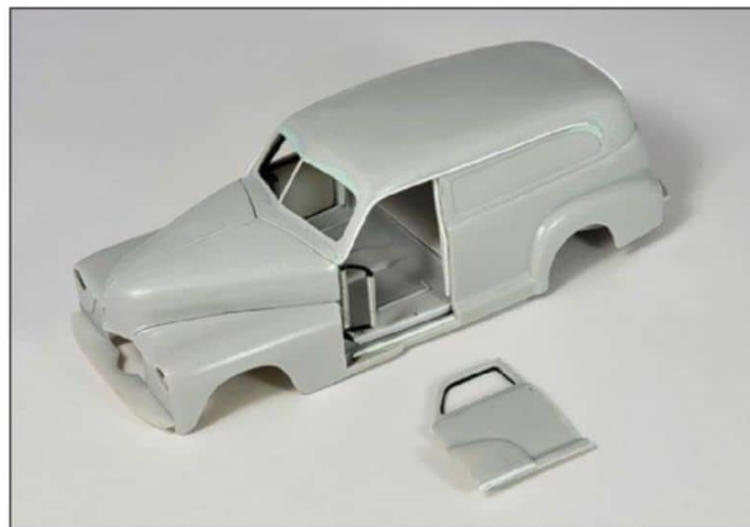
Side door hinge detail started. The front fender inner thickness had to be thinned considerably to allow the "fade-away" door detail to disappear inside when the door opens.
