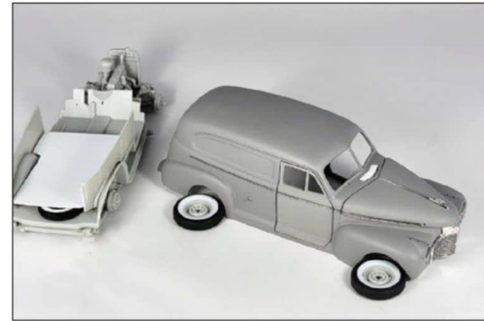
Development of the sedan delivery body with some of the formed stainless wire side trim, as well as the development of the cargo floor with spare tire access. The windshield area has been reportioned, but the door window shapes have yet to be redone at this point.
