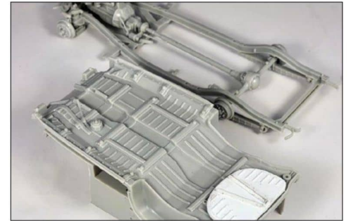
The fabricated styrene correct under-floor spare tire detail added to the kit's passenger car floor.
