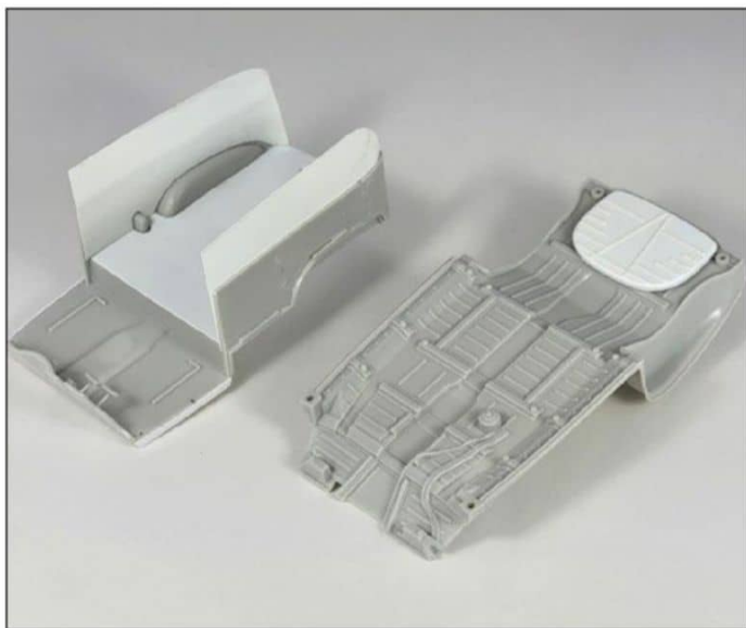
The same under-floor spare tire well had to be fabricated for the post-war model.
