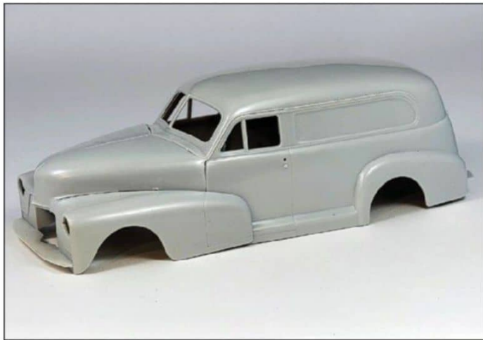
The '48 Chevy body as supplied in the Galaxie kit. The windshield should come down closer to the cowl area, the indent panel is incorrect toward the rear, the door windows are too sharp, and the front fender opening is shown as a simple radius
