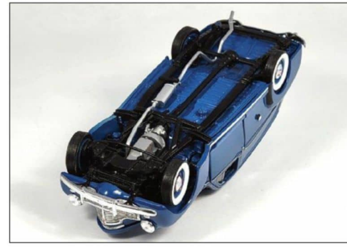
As with the stock 1:1 versions, the prewar and postwar Chevy sedan deliveries share virtually identical drivetrains and underbody detail. Poseable steering as well as corrected spare wheel under-panels have been added to both models.
