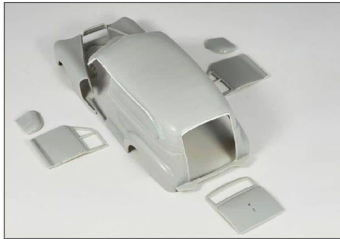
All the doors shown cut out as well as the gutter rails added.
