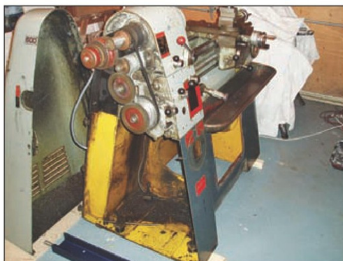
3. Inside the motor/variator housing.
