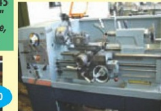
Colchester Student 1800 geared / gap bed lathe
