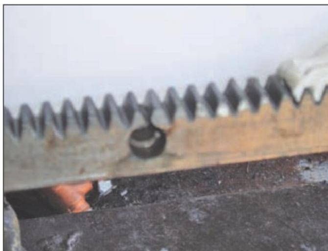
5. The damaged rack.
