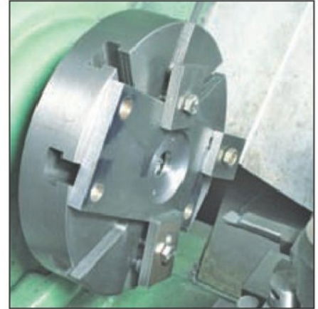
12. Boring the Drive Spindle Carrier (22).
