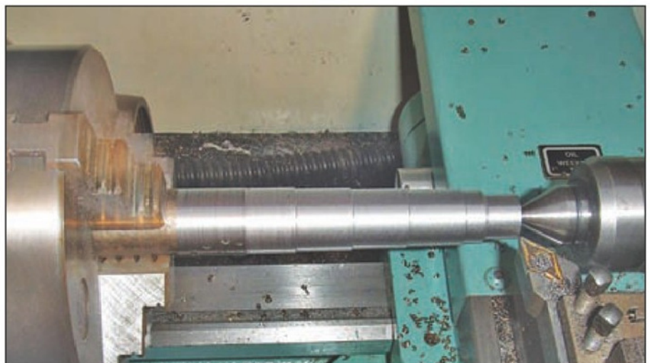
6. Roughing out the bar using steps.
