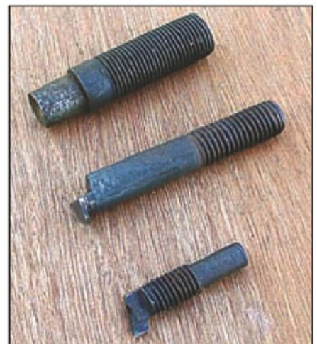
3. Three tools made from Allen screws. Top a punch; middle to cut internal groove; bottom keyway cutter.
