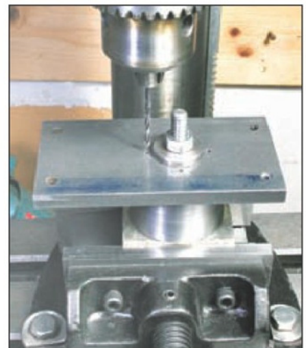
13. Using the Drive Spindle Carrier as a drilling jig for the holes in the Drive Spindle Body (23).
