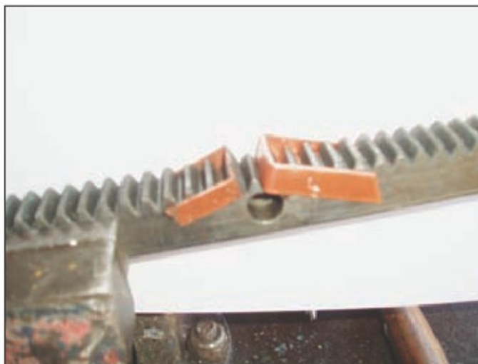
6. Protecting the rack from splatter.
