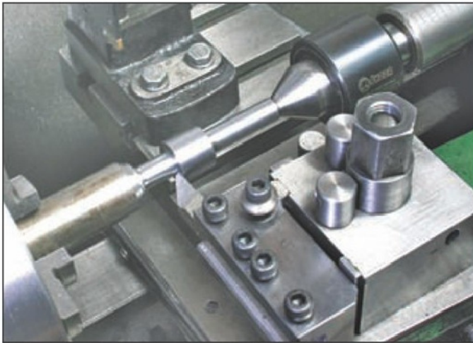
8. Ensuring the two diameters for the ball races are concentric by using left and right hand knife tools.
