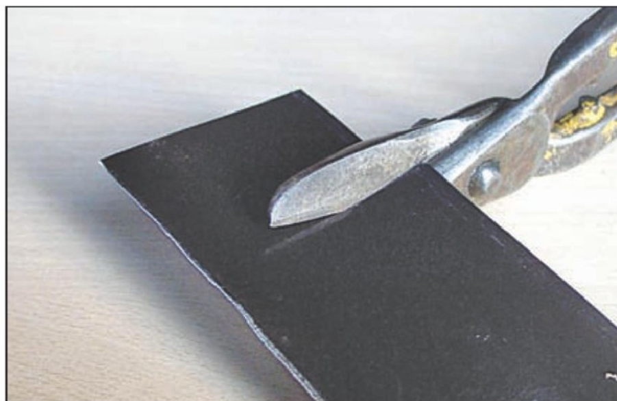
1. Cutting action by shear fracture.
