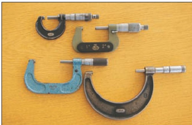
10. Four Micrometers covering a range of 0 to 4 inches. Top to bottom: 0 to 1in. Moore & Wright, 1 to 2in. Etalon, 50 to 75mm GKN Shardlow, 3 to 4in. Moore & Wright.
