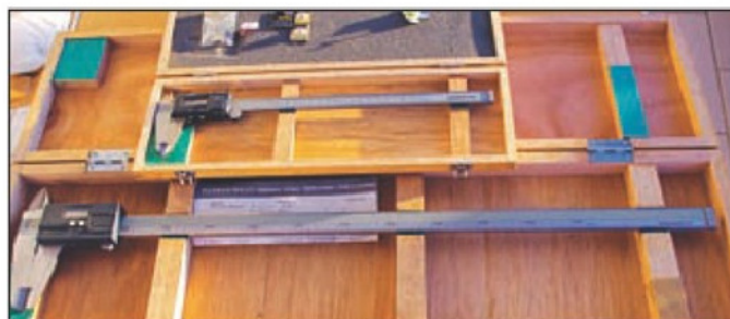
7. Larger digital calipers from Mitutoyo (12inch and 24inch).
