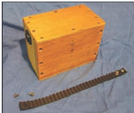
7. Lid foam filler in, lid on, cut down timing belt handle to be fitted.
