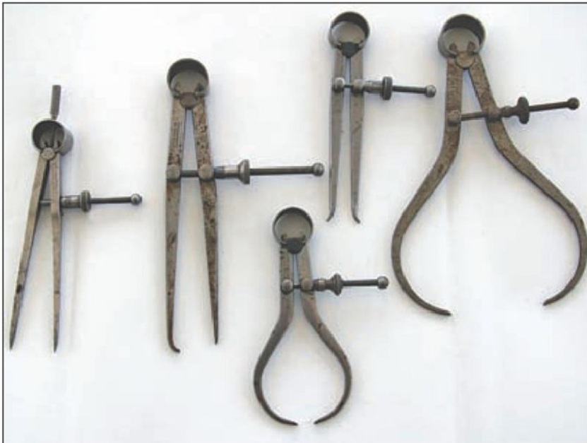
21. Assorted spring joint calipers. L to R: dividers, Jennies, small external, internal and large external.
