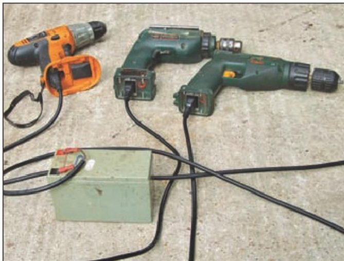
1. Showing first attempt using IEC plug and socket on drill.
