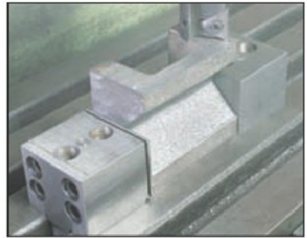
18. This method of machining the fourth face ensured that it was parallel with the other long edge.
