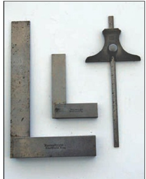
22. Six inch and three inch try squares shown with a 150mm depth gauge.
