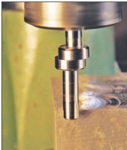
13. The revolving edge finder is kicked to the side.
