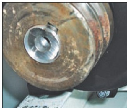
9. The turned shim on the motor shaft.
