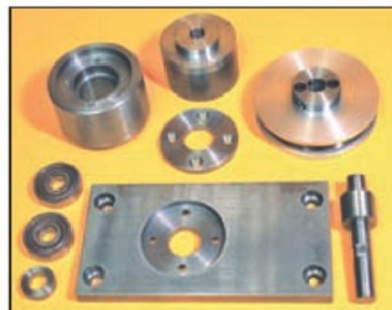
15. The parts that make up the Drive Spindle. The mandrel used in photo 11 is seen rear centre.
