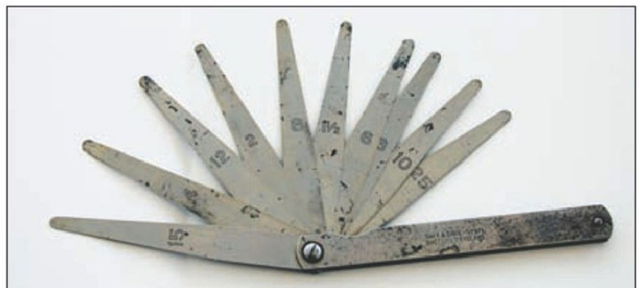
17. Set of feeler gauges showing evidence of over forty years usage.
