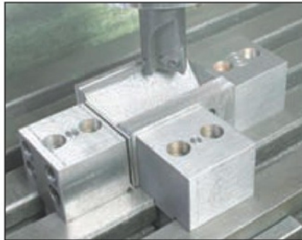
19. The Vee block was firmly against the two square posts ensuring that the surface being machined would be at 90deg. to these faces.
