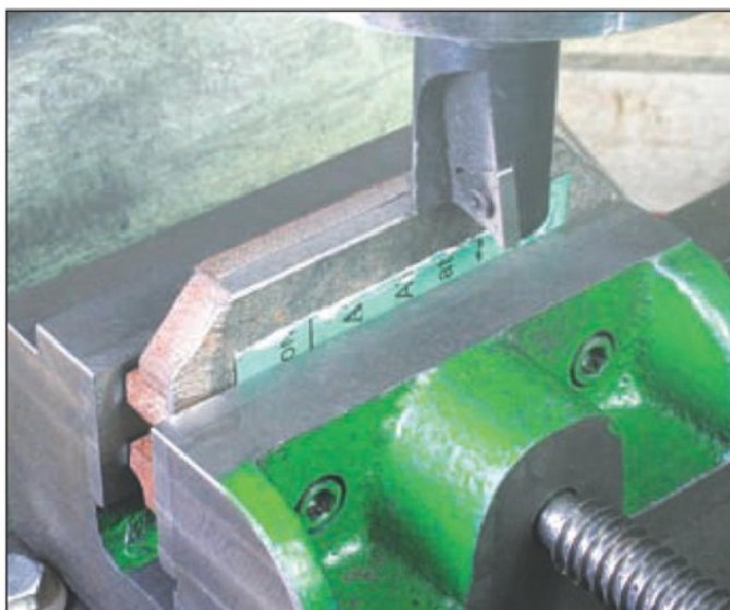
25. Milling the side of the base.
