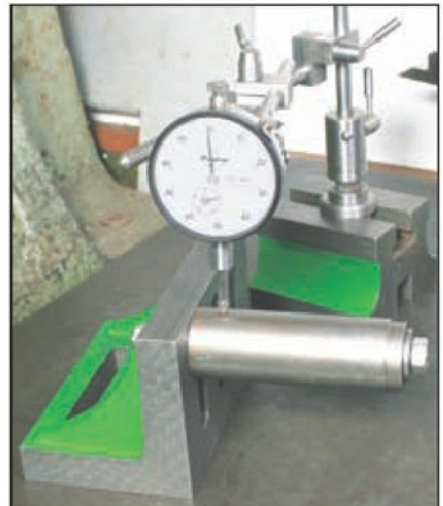
22. Checking that the cylindrical square was accurate horizontally.
