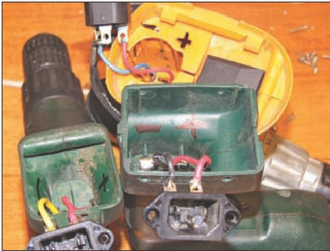
3. Mark the contacts to maintain polarity (this is the original IEC installation).
