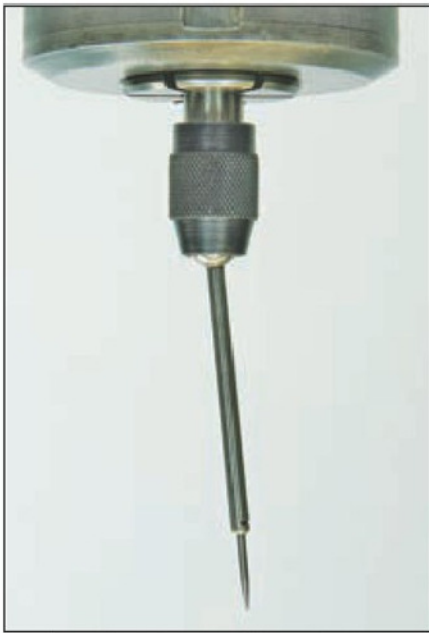
10. The pointed probe of the wiggler to locate scribed lines. Not running true yet.
