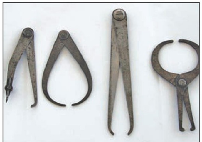
20. Assorted friction hinge calipers. L to R: Jennies (usually for marking out), Two typical external types, and finally a Set for visible indication of a hidden dimension.
