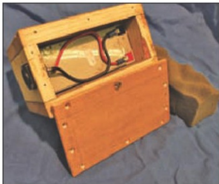
6. Gel battery installed and connected - note foam packing to fill space.
