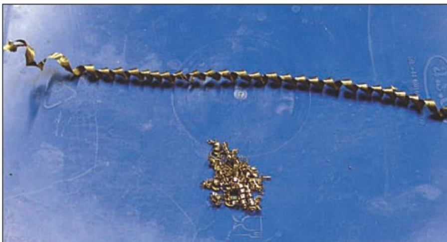
2. Swarf from free cutting steel below gives a quick test to confirm your material really is free cutting.
