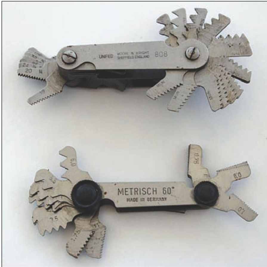
18. Two sets of thread gauges. Imperial covers 4 to 60 tpi Whitworth and 4 to 42 tpi unified. The metric set gives pitches ranging from 6mm down to 0.25mm.
