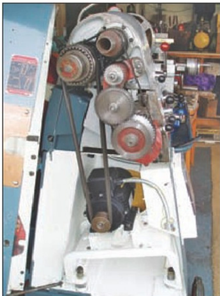
8. The motor on its new frame.
