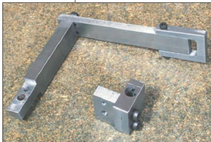
18. The File Carrier Assembly (4).
