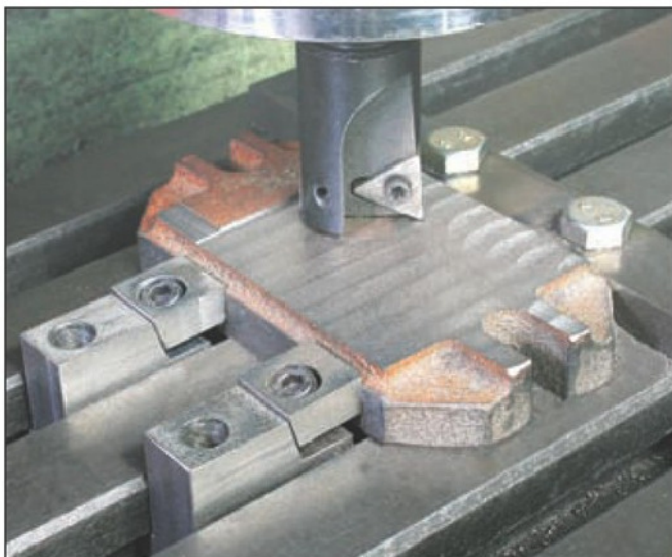
27. This method of milling the top surface of the base ensured that it was accurately parallel with the underside.
