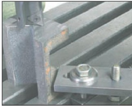
17. Machining the third face, there is a second clamp behind the casting.
