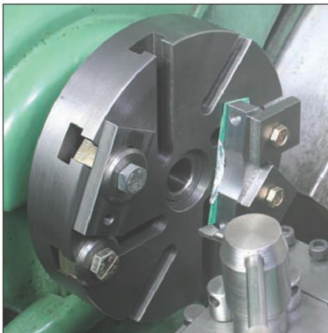
30. The clamp has a curved recess rather than the normal Vee.
