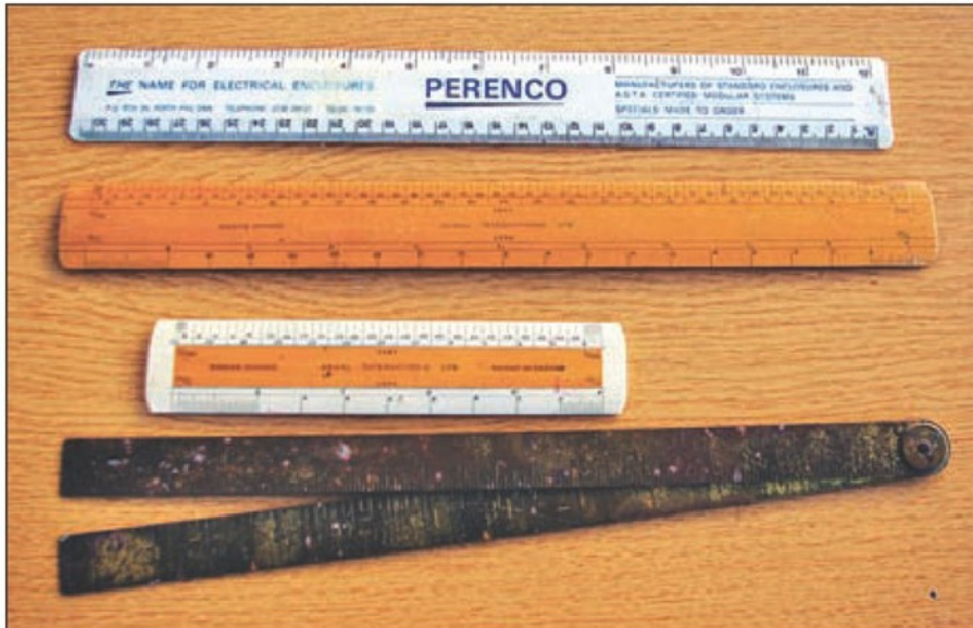
1. Top to bottom, a cheap plastic ruler, 12 inch wooden draughting scale, six inch composite scale and a folding 24 inch brass rule more suited to woodworking.
