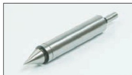
15. The controversial edge and centre finder with a conical point.
