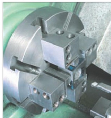
17. Boring one of the Slider Blocks.
