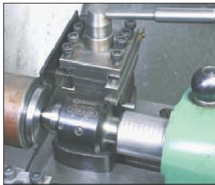
10. Parting off the Outer Clamp Ring (24) from the end of a long (not seen) bar.
