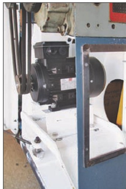
14. The new mounting frame.
