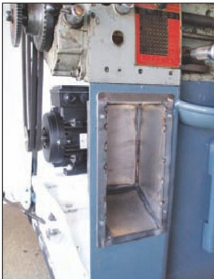
15. The new enclosure.
