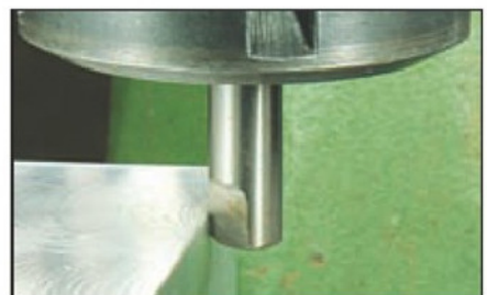
3. A flat ground on the cylinder of a drill. As a matter of fact, I used a broken slot drill here.
