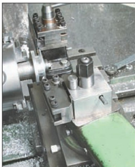
14. Producing the angled faces on one of the pulleys.
