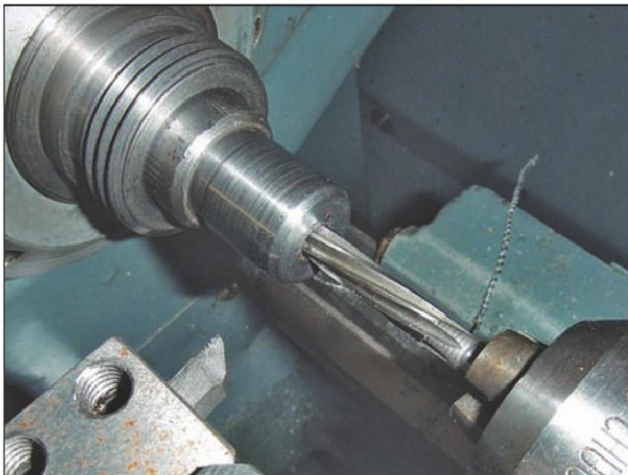
8. Reaming to \frac{1}{4} in. diameter before splitting the collet.
