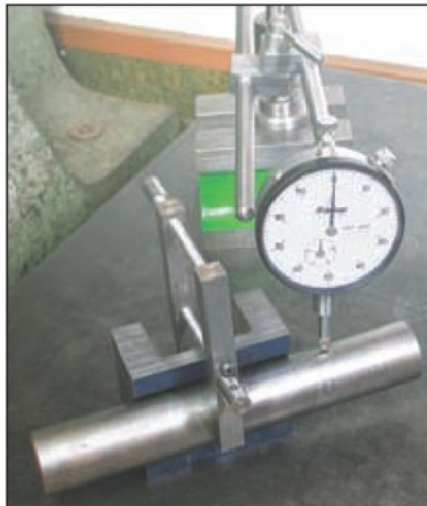
21. This test showed that the Vee was not quite parallel with the sides.
