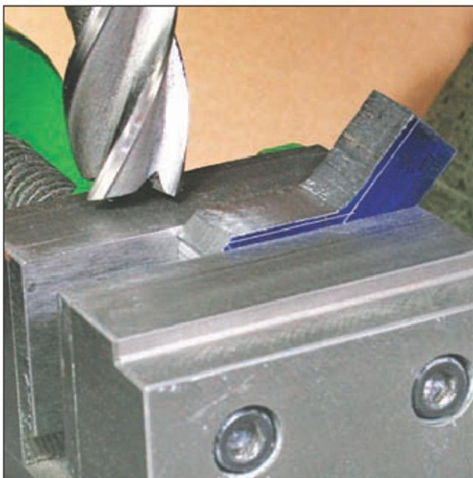
29. Shaping the clamp.
