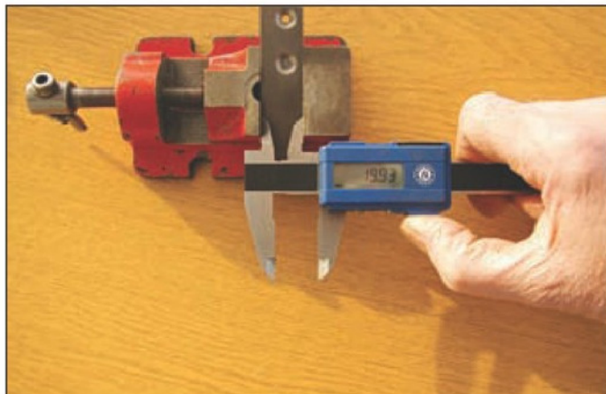
9. Measuring between the vice jaws with the inside points.
