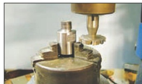
3. Milling spanner flats on the adaptor.
