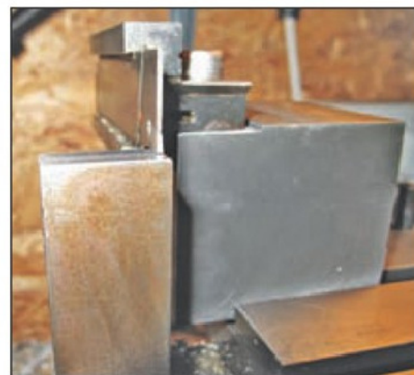
42. Checking the final centre height.
