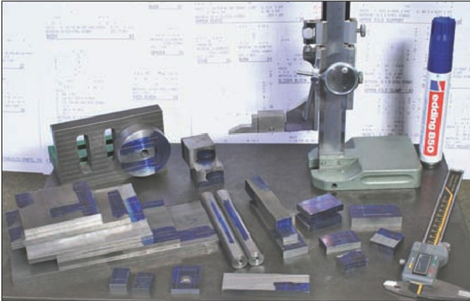
2. Marking out all the parts at the same time.
