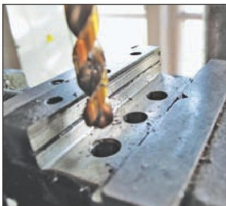
40. Drilling the holes to finished size in the bench drill.
