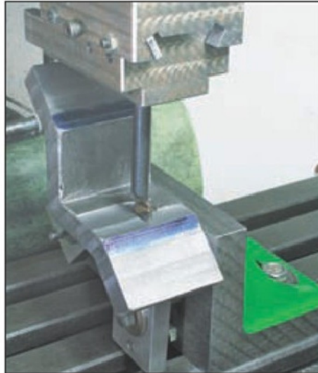
6. The cutter used in the previous photographs had insufficient reach to machine the Vee so my boring head was used instead.
