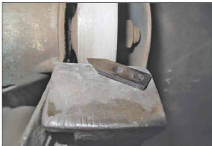
36. Another view of grinding the relief angles.
