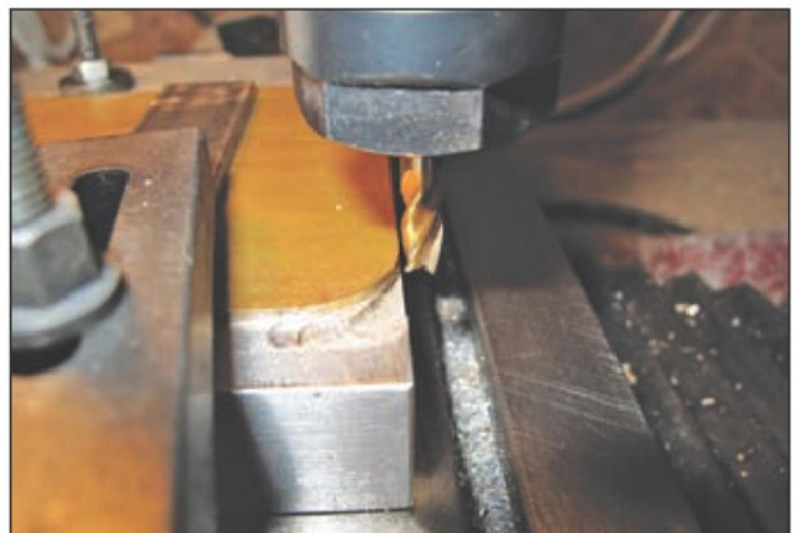
9. Machining 15mm corner rads.
