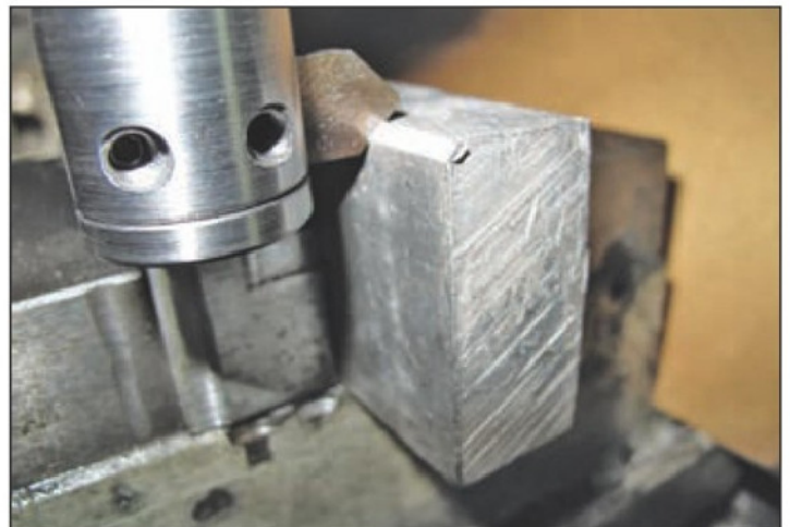
43. Proving the 45degree cutter.
