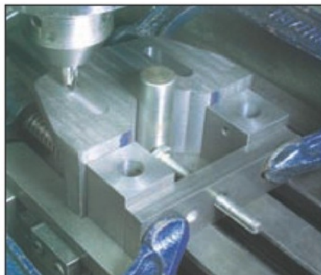
7. Using a slot drill to produce the fixing slots. The round bar gives a reference point for positioning them relative to the Vee.
