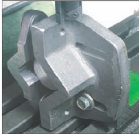
9. The second end being machined having been set up in a similar manner to that in photo 8.
