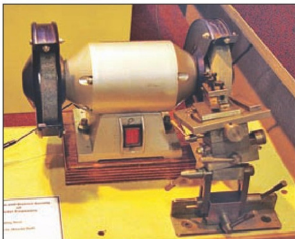
25. Graham Hutchinson made this grinding rest to a design by former MEW editor Harold Hall.
