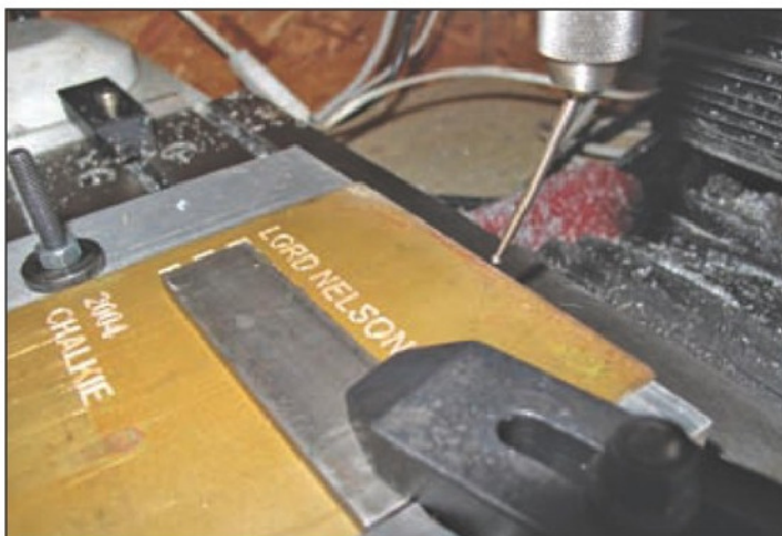
8. Establishing absolute zero.
