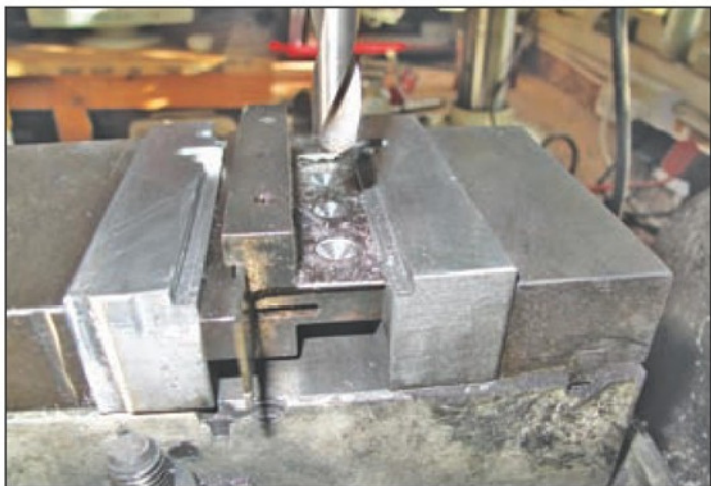
38. Pitching out hole centres on the mill.
