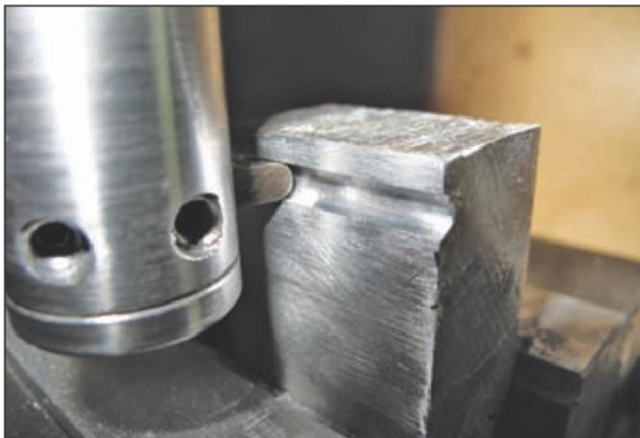
42. Proving 0.187in. diameter cutter.
