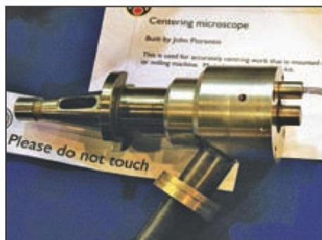
19. John Florentin's centering microscope. The spring and weight are to establish the focal position.
