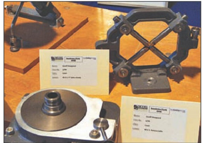
16. - plus 5in. lathe steady and rotary table.
