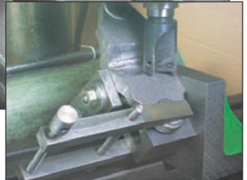
12. The Vee in the clamp being made.
