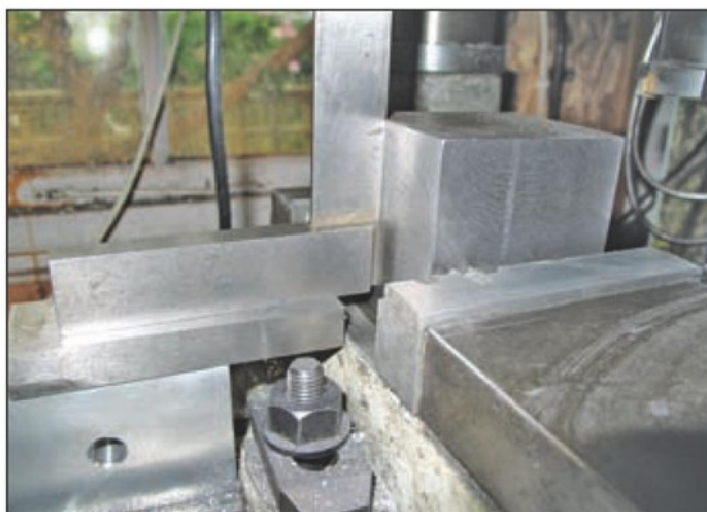
26. Setting the billet to machine the ends square.
