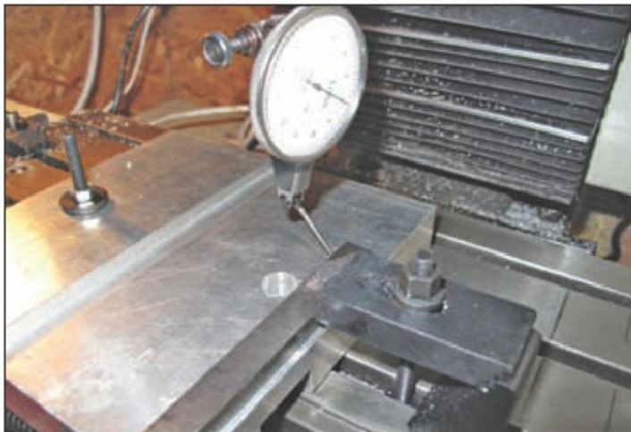
6. Lining up a straight edge prior to cutting the corner rads.
