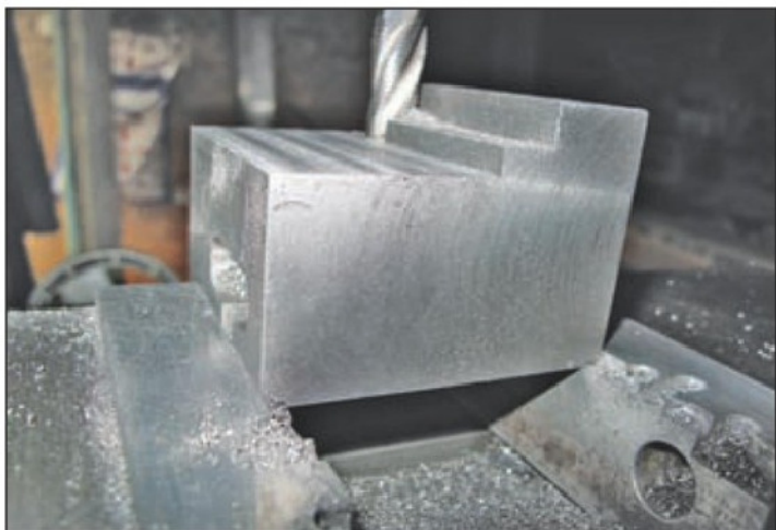
43. Rough machining the tool base.
