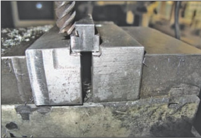
32. Machine equal amounts from each face to suit the cross slide tenon.
