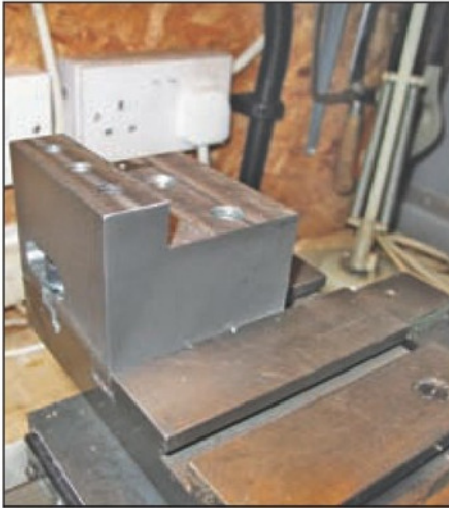
52. Parting tool block ready for tool.
