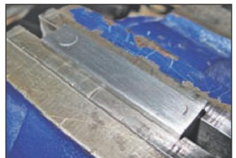
37. File peened ends flush to tee nut.
