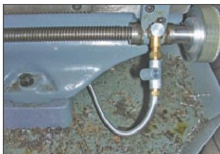
16. Tailstock end leadscrew bearing banjo.
