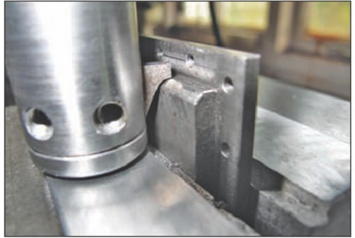
40. Machining the radius.
