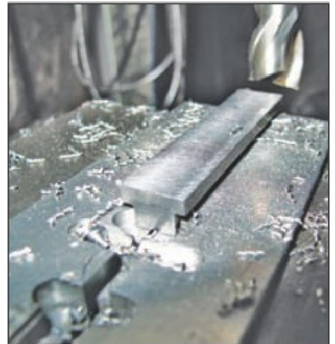
34. Machine Tee to size.
