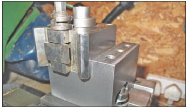
48. Quick change tool post in position.
