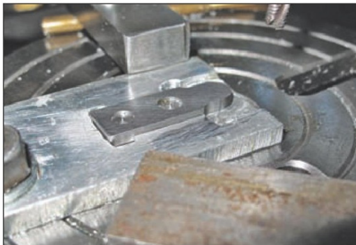
34. Finished 0.187in. fly cutter.
