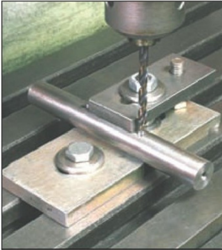
6. An alternative cross drilling method to that shown in photograph 5.
