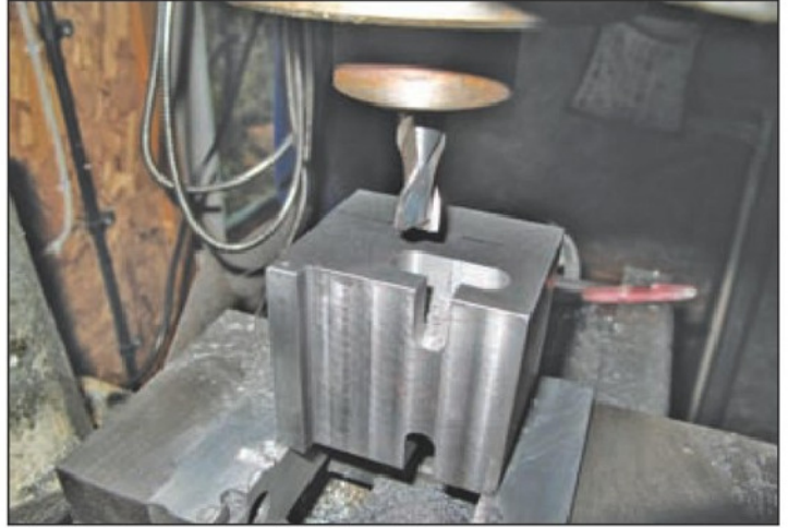
31. Slots to accommodate clamping nuts.
