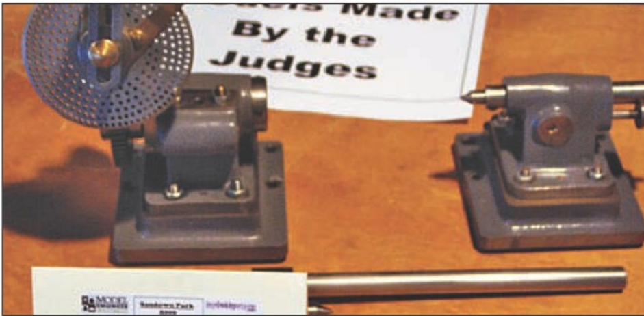
12. George Thomas designed versatile dividing head - Geoff Sheppard.
