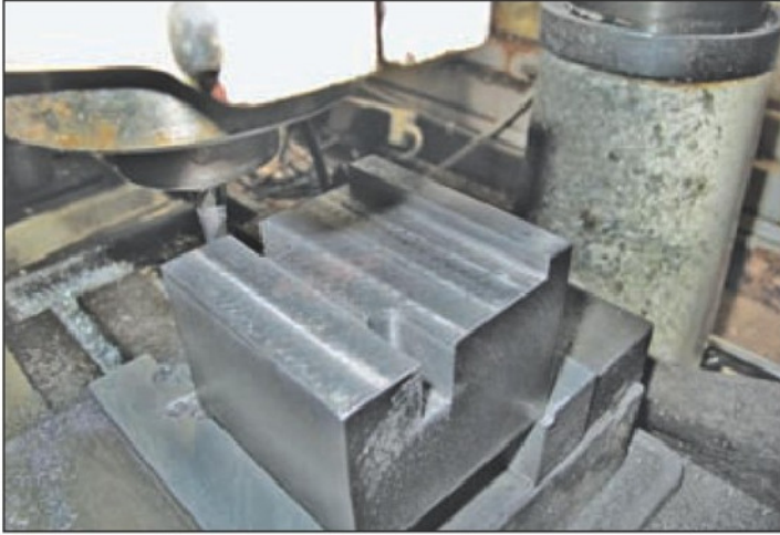
30. Slots need to line up with the rear tenon.
