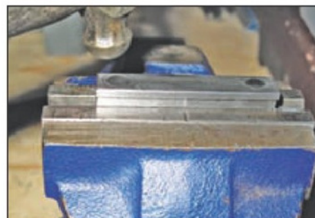
36. Peening over the studs with light ball peen hammer
