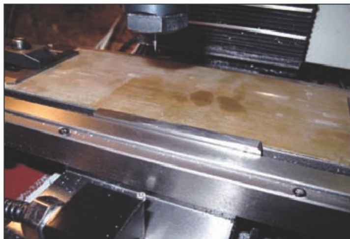
2. Aligning the brass plate with the machine.
