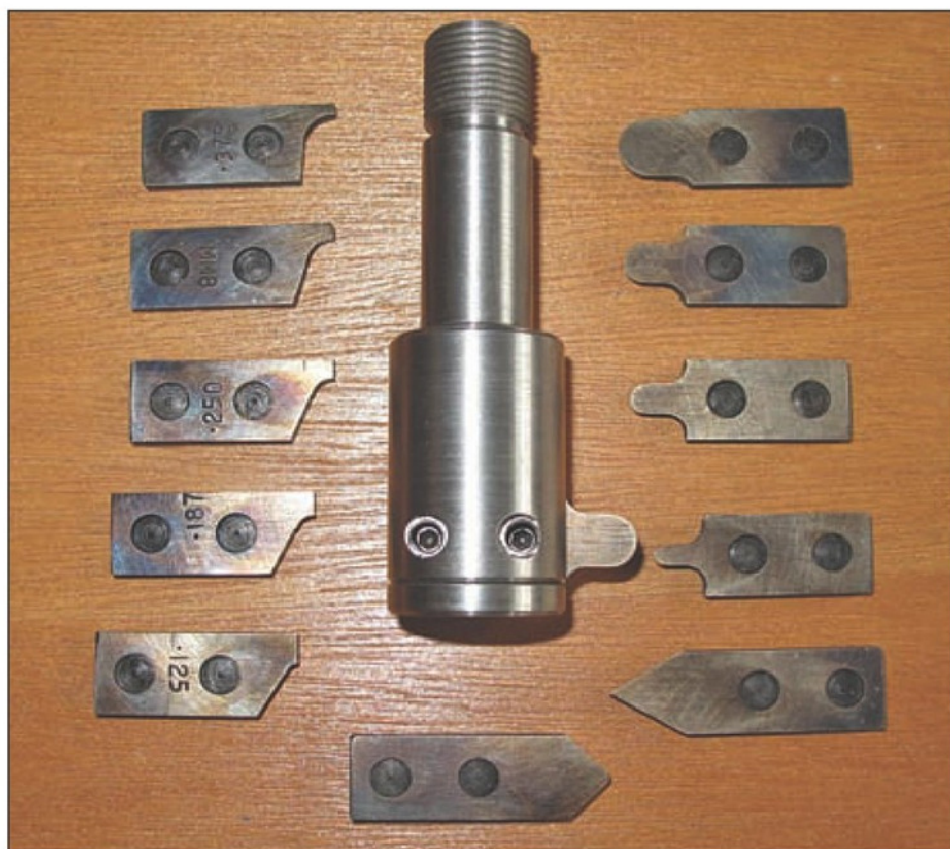
30. The finish machined 0.187in. radius cutter.
