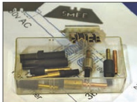
21. Work and tooling for the spark eroder.
