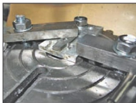
32. Cutting the right hand flank.
