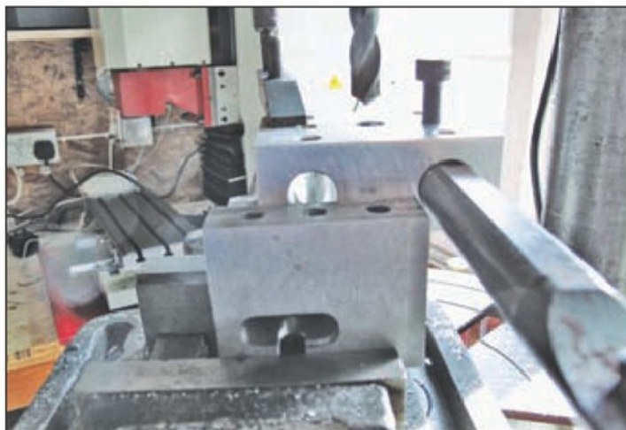
44. Transferring clamping hole centre position.
