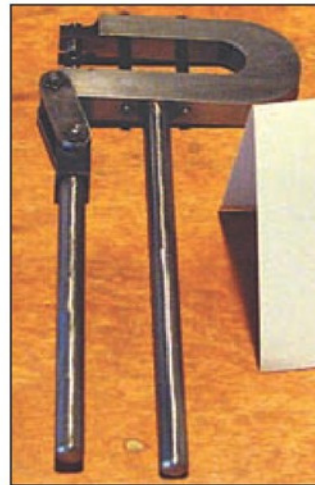
15. Geoff also brought this hand rivet press -
