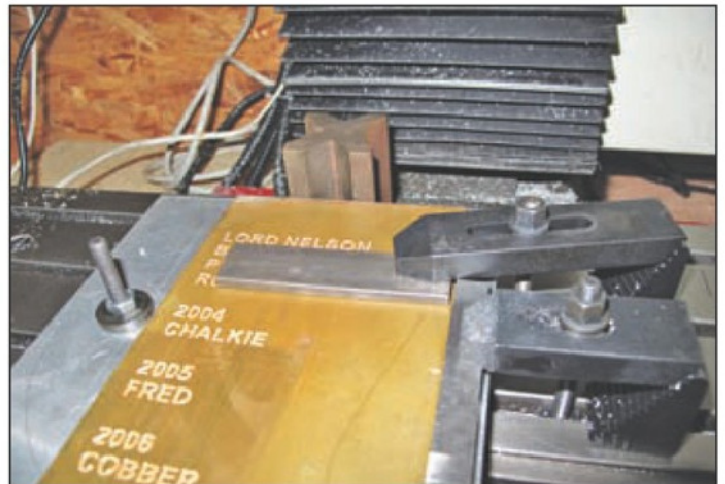
7. Loading the plate for machining the rads.
