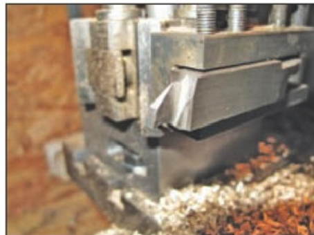
50. Trepanning the centre out.
