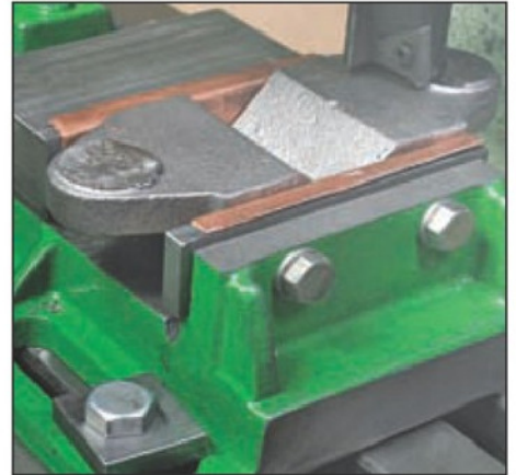
10. Facing the fixing lugs on the clamp
