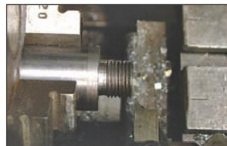
2. Checking the adaptor external thread.
