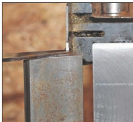
41. Determining the stock removal to achieve centre height, using feeler gauges.
