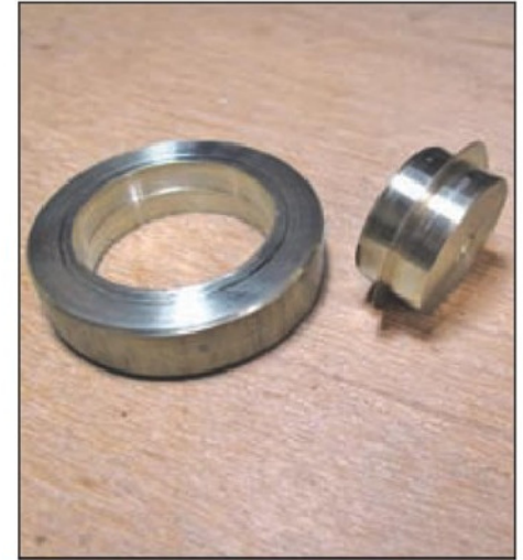
54. Trepanned ring and centre with its web.
