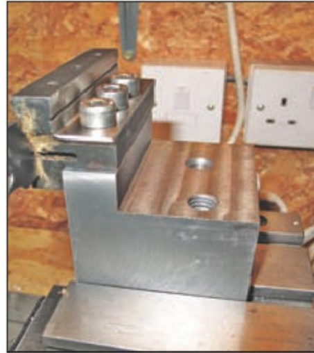
53. Parting blade in position.
