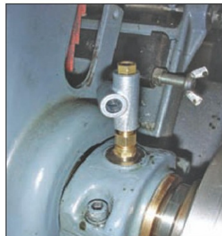
10. Headstock connector fitted to lathe.
