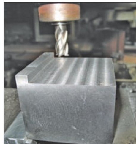
29. Finish machine, leaving a couple of thou for final fitting on the bench.
