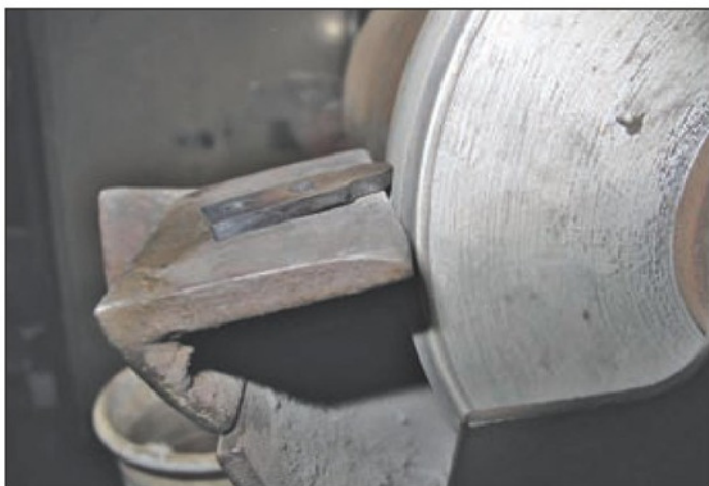
35. Grinding the relief angles.
