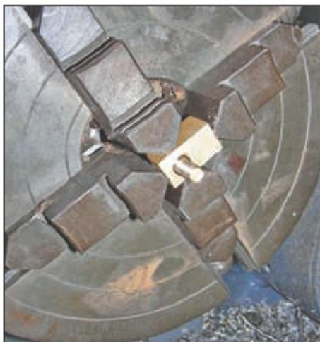
8. Turning and threading the connector.
