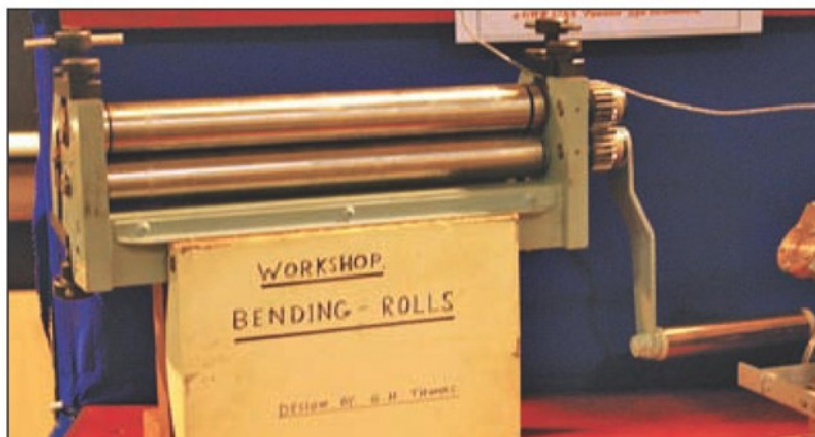
27. Bending rolls to the George Thomas design on view at the Staines society stand.
