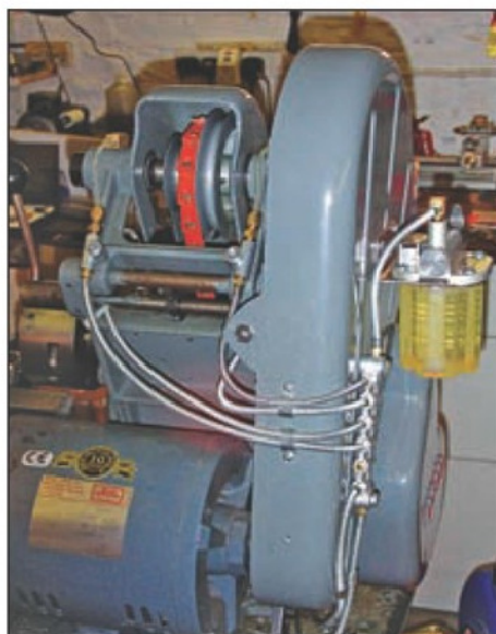
1. Most of the lubrication system can be seen in this photo.
