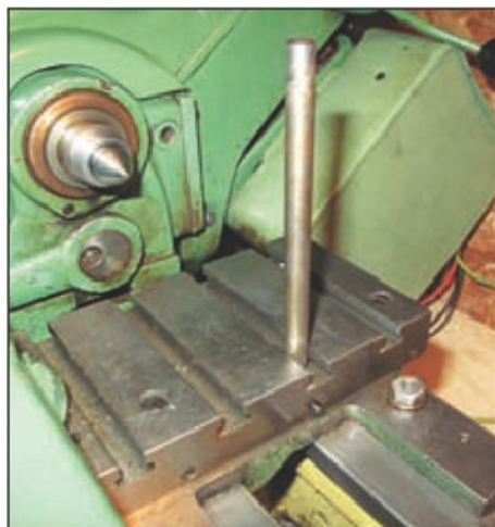
27. Sizing Tee slot with a drill blank.
