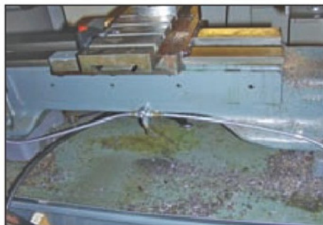
6. The three way connector on the back of the lathe bed.
