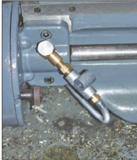
12. Banjo connector to leadscrew bearing.
