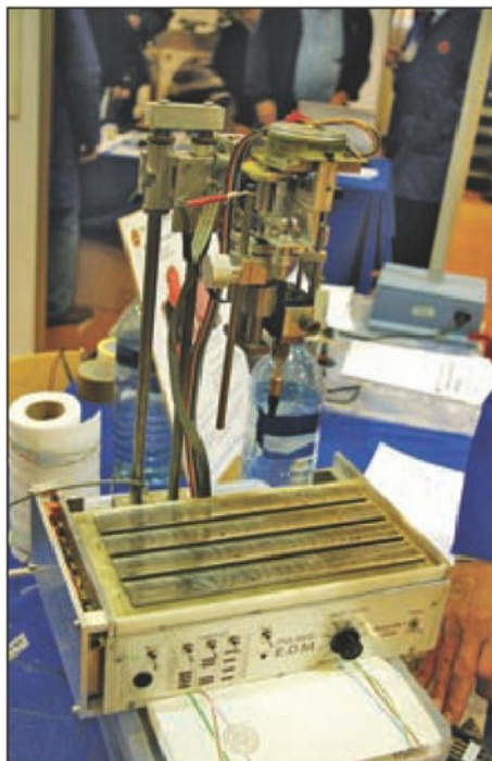
20. Spark erosion machine with electronic control of downfeed and waveform.
