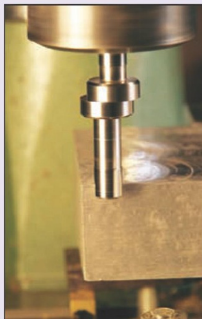
SETTING UP WORK DATUMS
