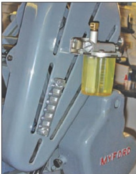
5. The reservoir is mounted on the belt guard.
