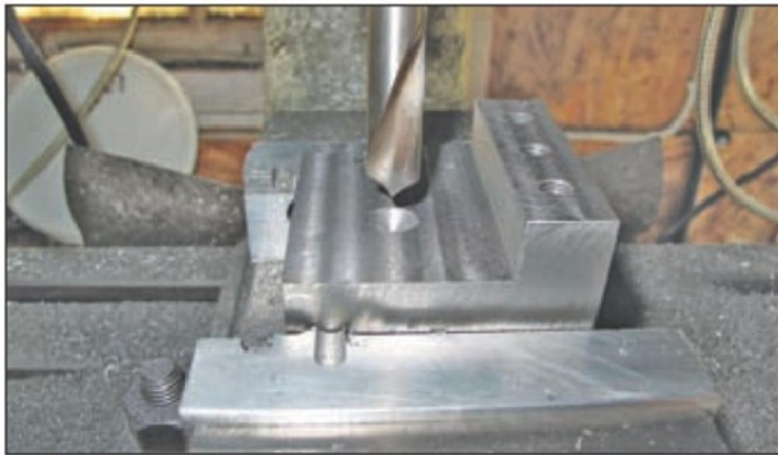
47. Centring tool post position.
