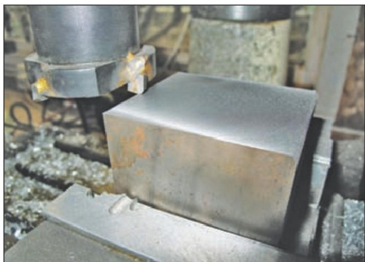
25. Machining the billet square.
