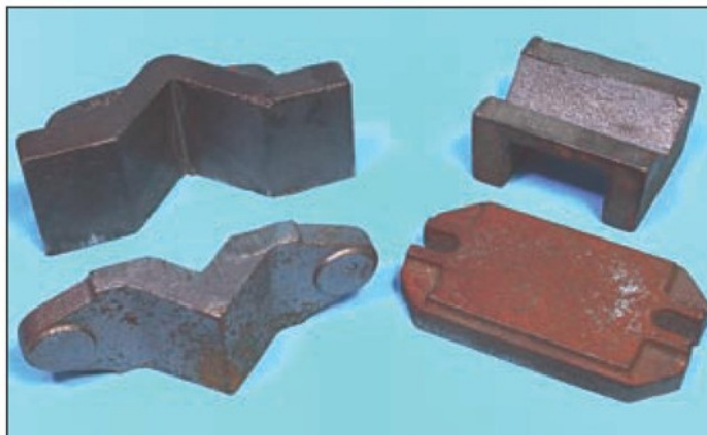
2. The castings as supplied, both for the Keats angle plate and the Vee angle plate.
