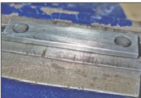
35. Studs protruding from tee nut.
