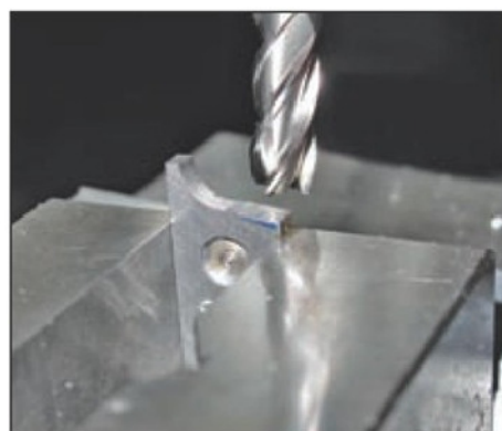
30. The finish machined 0.187in. radius cutter.
