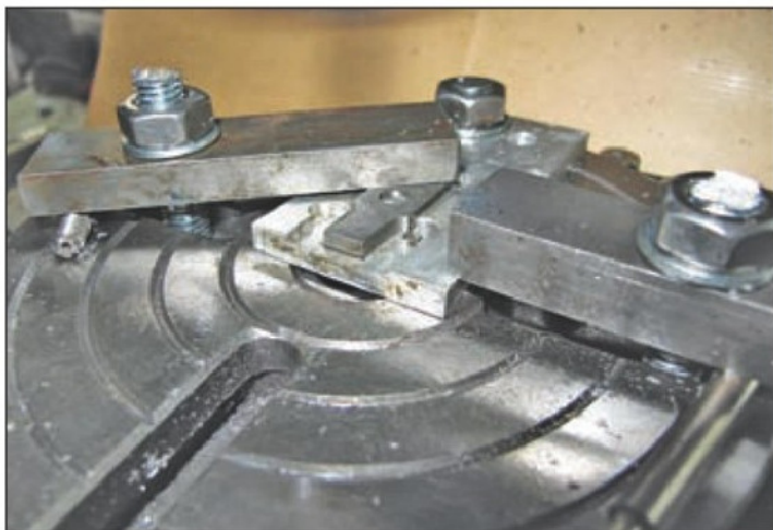
33. Cutter before final machining. Clamp removed for clarity.
