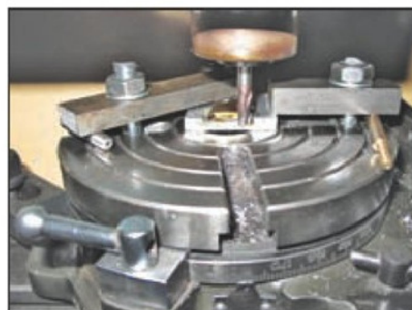
31. Cutter blank sitting in fixture location and resting against recessed back stop.
