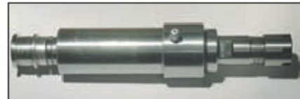
1. The finished spindle.
