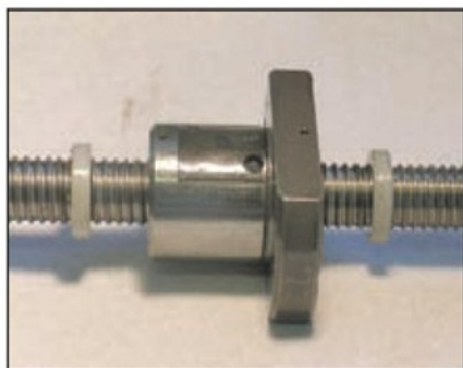
2. The nylon wipers moved clear.
