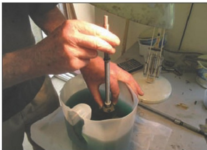
4. Cleaning the ball screw.
