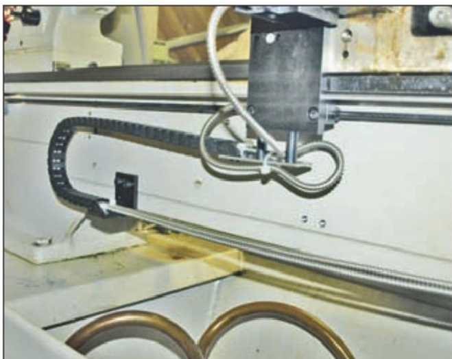
4. The cable chain.
