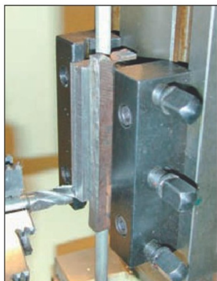
5. Machining the angles on the tool grinding holder.
