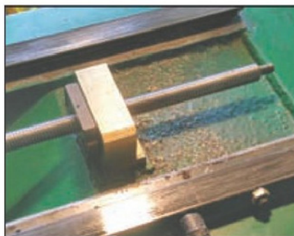
3. Brass swarf under the table.
