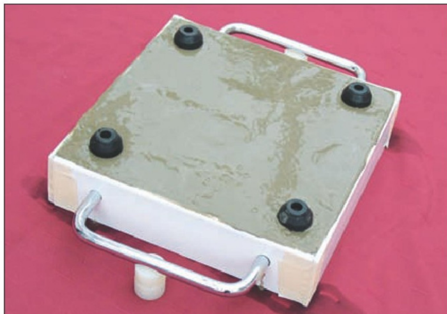
4. The underside of the finished surface plate.
