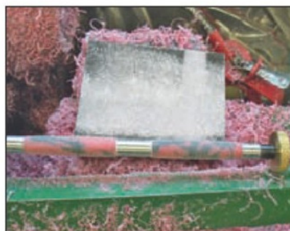
11. Sanding block for 1st stage of finishing.
