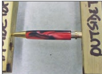
15. Pressing in the centre joint.
