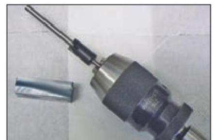
18. Trimming an insert.
