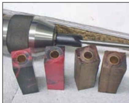
9. Blanks ready for mandrel.
