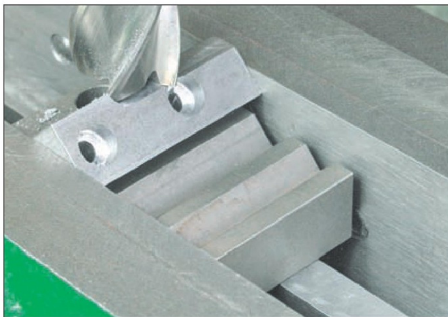
Photo 17. An easy method of holding the "Small diameter" jaw for chamfering.
