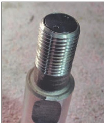
Photo 2. Threaded end cap beneath which was the loose retaining nut.
