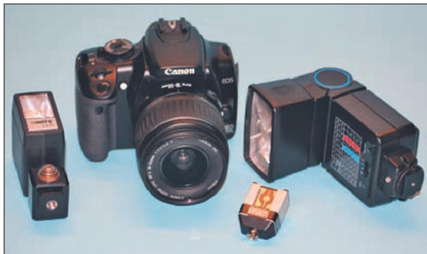
Photo 5. The main items that make up the items used, left to right. The secondary flash unit with slave fitted. The Digital SLR camera. An automatic flash gun for the main flash and in front the adapter for connecting the main flash to the camera via a cable (Ref. 1).
