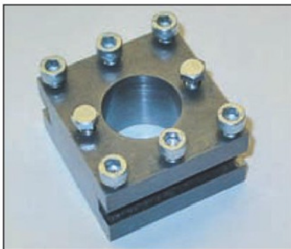
Photo 6. A finished toolholder.
