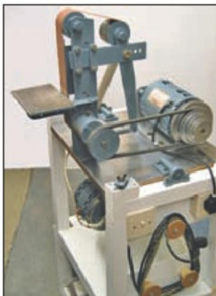
Photo 3. The small bench in linisher mode.
