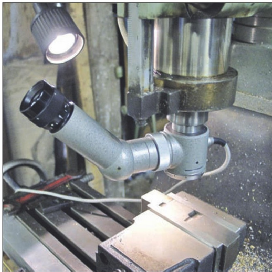
photo 10. Microscope successfully fitted to the VMC mill.
