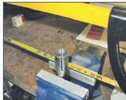
Photo 4. Hacksawing the slots in the pillar.
