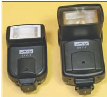
Photo 8. Two non dedicated flash guns that can be used with any camera, either hot shoe mounted, connected via a cable or using a Digital Slave.
