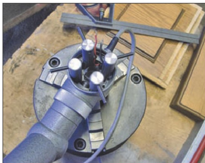
Photo 7. Setting the prism using four keys. The eyepiece has been rotated to allow the graticule to be viewed, whilst the assembly is inverted.
