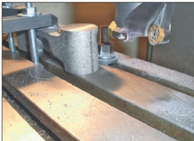
Photo 8. Finishing cut being taken
