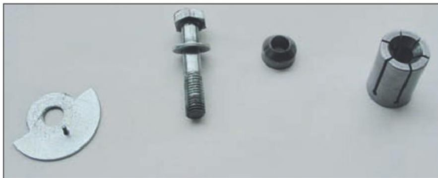
Photo 3. Component parts of the pillar assembly.
