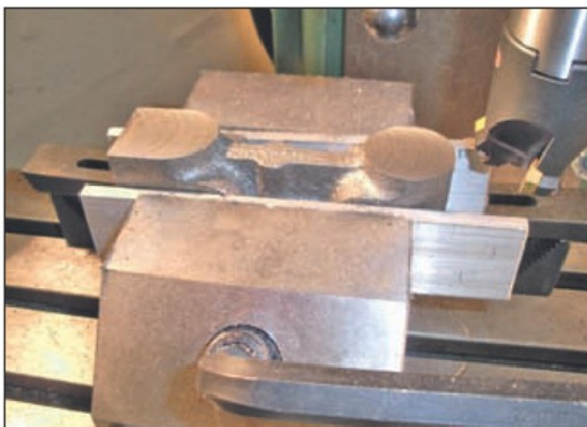
Photo 3. The casting being milled to thickness.
