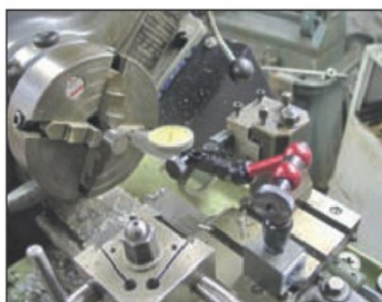
Photo 13. Centering up in the four jaw on the Myford with the smallest unit.
