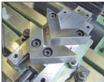
Photo 7. "Non approved" bending operation.
