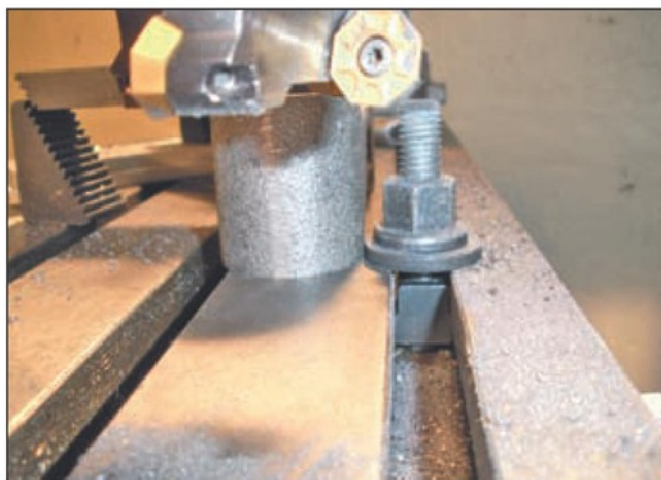
Photo 9. Note the stop to stop the casting moving.
