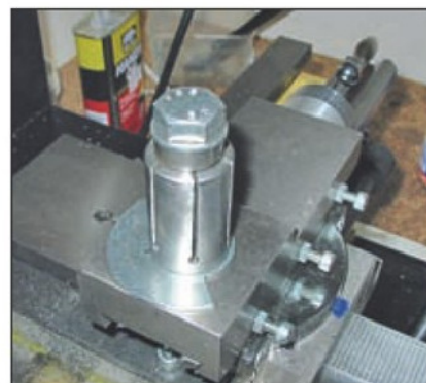
Photo 2. The pillar fitted to the top slide.
