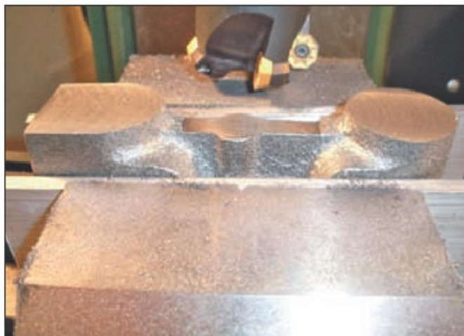
Photo 5. The lower milling complete.
