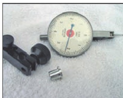
Photo 11. Detail of fine adjustment feature, with clock and adapter bush.
