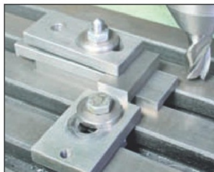
Photo 15. Surfacing the end of a thin piece clamp.
