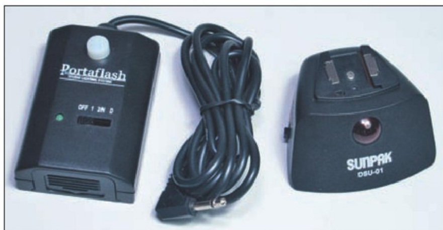
Photo 6. Two Digital Slaves which ignore the camera's pre flash, firing the flash in sync with its main flash
