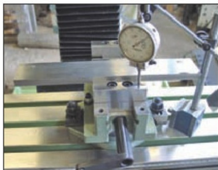
Photo 6. No lift was discernible when clamping work.
