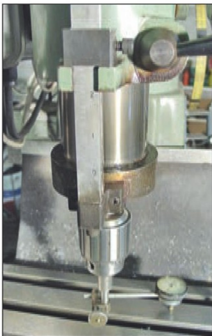
Photo 9. Checking mill head for squareness.
