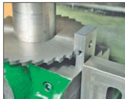
Photo 16. Making the slot in one of the "thin piece larger diameter clamps".
