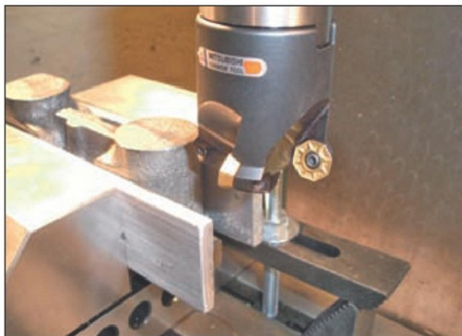
Photo 2. Another of the milling setup showing the tipped cutter used.
