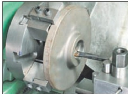
Photo 21. Holding a large disk for machining. I have modified the drawings to make these jaws longer so as to increase the depth of the grip to those seen in the photograph.
