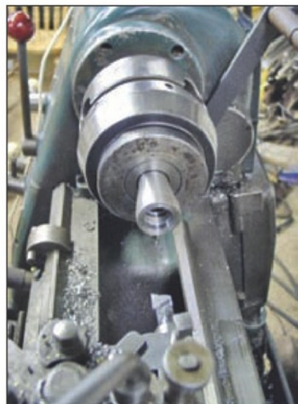
Photo 4. Machining the new arbor.
