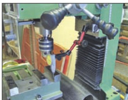
Photo 12. The vice may be clocked square by attaching the mag base to a machined face on the mill head.
