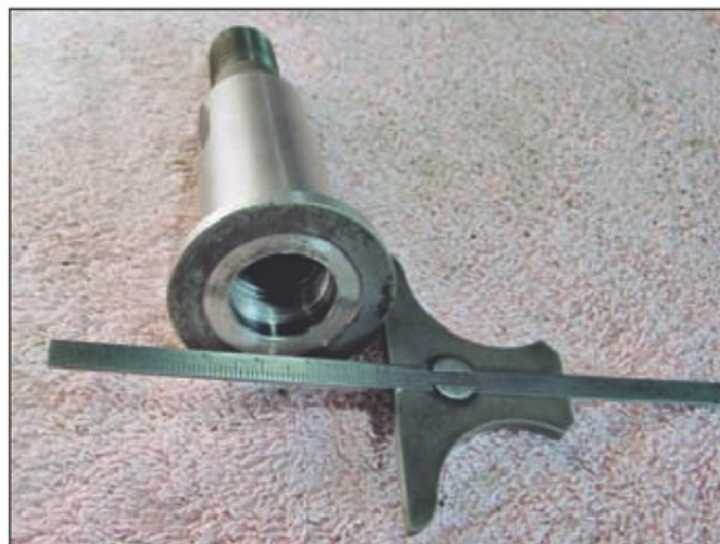
Photo 5. Depth gauge shows how far in the mirror is located.
