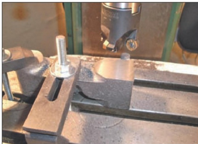
Photo 7. Finishing the drill head casting parallel.
