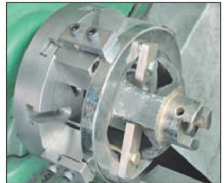
Photo 22. Showing that a mix of holding methods can be used on a single workpiece.
