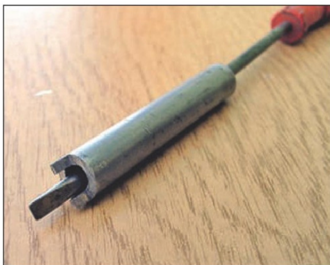
Photo 8. Hollow screwdriver to adjust the orientation of the crosshairs.
