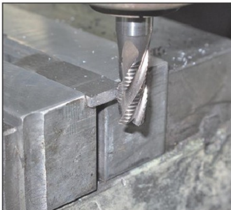
Photo 13. Squaring off one end of the cutter blank.
