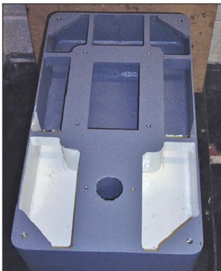
Photo 13. Coolant tank painted up.
