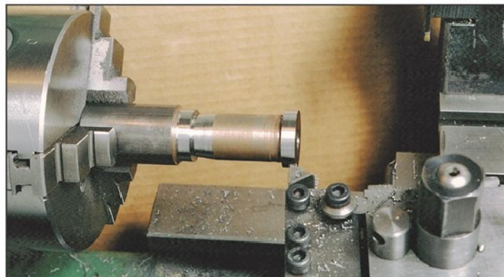
Photo 3. Setting the top slide in preparation for turning the taper.
