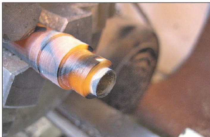
Photo 13. Turning the battery case to size.
