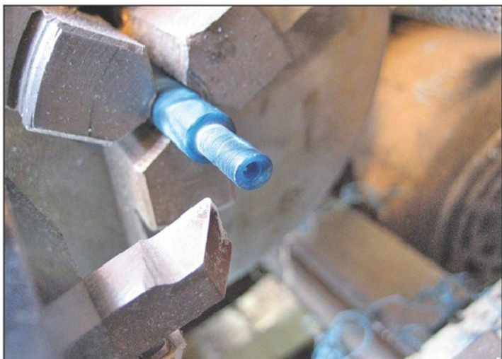
Photo 16. Turning the LED mounting to size.
