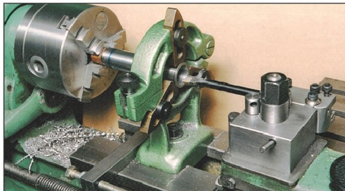
Photo 4. Machining the adapter bore.
