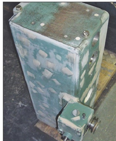
Photo 15. Gearbox joint for rubbing down.
