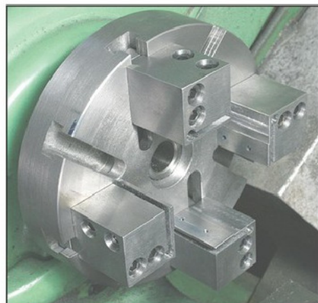
Photo 2. The modified design is similar to a conventional four jaw chuck.
