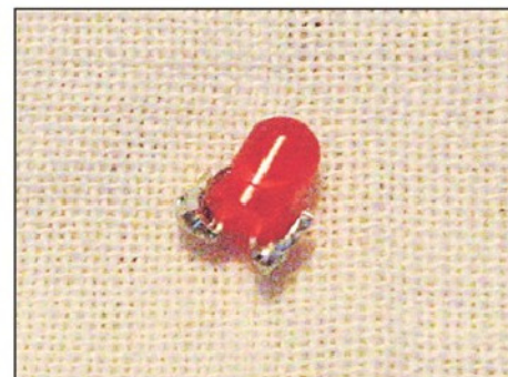
Photo 21. Cutting the LED wires very short.
