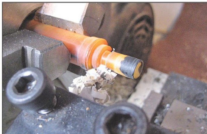
Photo 14. The battery case ready for parting off.
