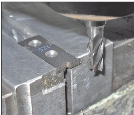
Photo 26. Milling to the centre of the hole.
