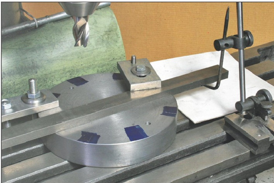
Photo 6. Positioning the body accurately on the machine table.
