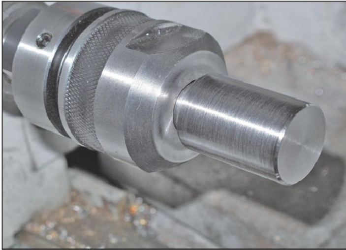
Photo 6. Turn holder body true, by holding in the Autolock.
