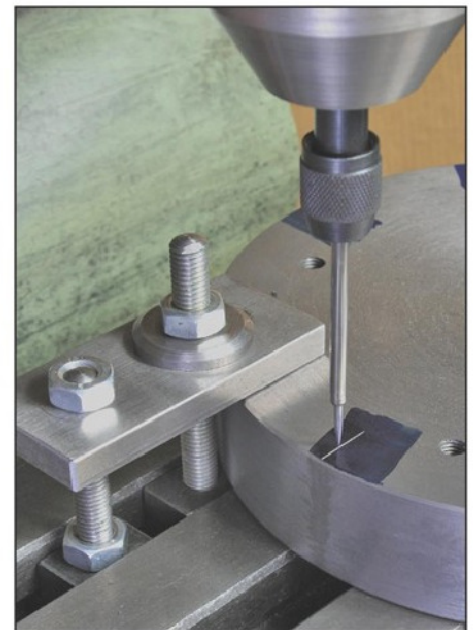
Photo 8. Lining up the machine spindle with one of the marks on the body.
