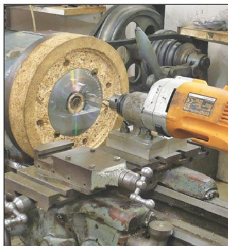
Photo 4. Drilling a division plate in progress.
