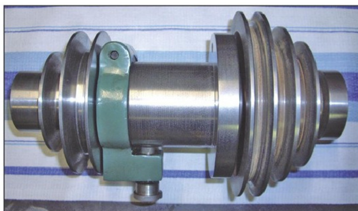
Photo 20. Counter shaft cleaned up.
