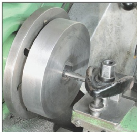
Photo 3. The body in its initial stages of being machined.
