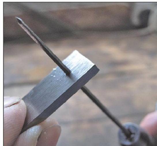
Photo 22. Hand broaching the primary clearance angle.
