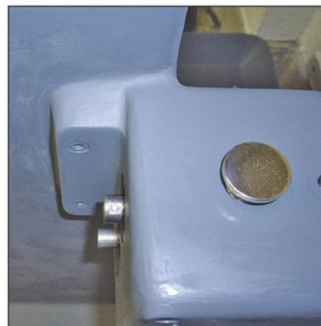
Photo 12. Gearbox filling detail.
