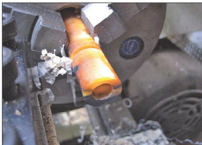
Photo 3. Parting off the centre insulation.
