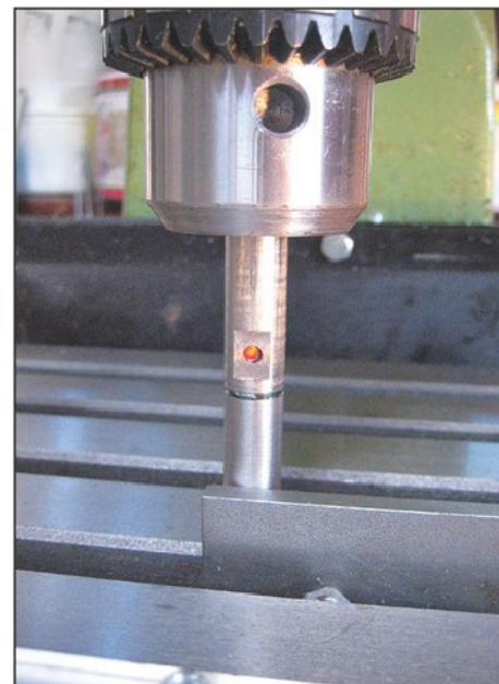
Photo 1. Finished edge finder in mill.
