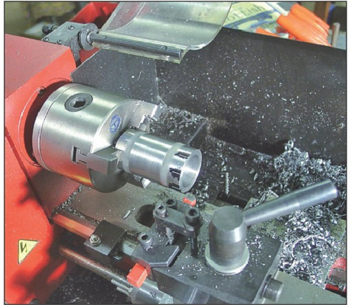
Photo 7. Angular positions scribed with Vee tool on side.
