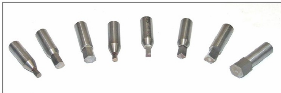
Photo 3. Broaches made from HSS.
