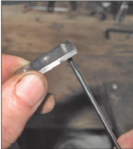
Photo 23. Sizing the 0.125in. hole with silver steel.
