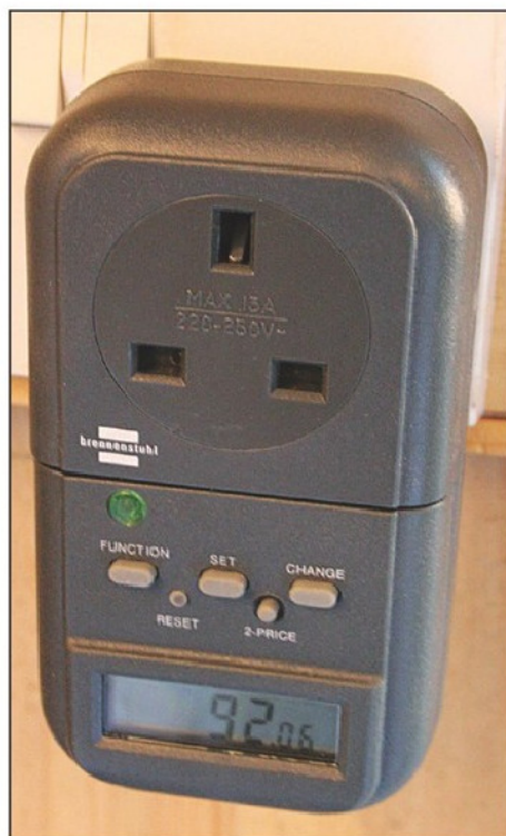
Photo 2. The meter for checking electricity usage.
