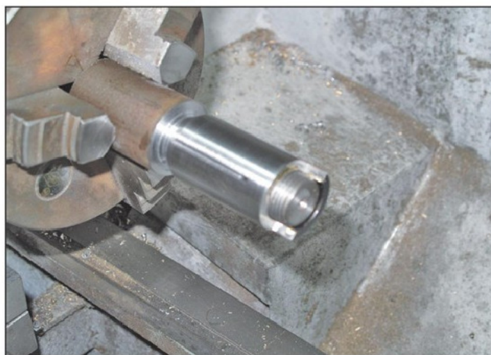
Photo 5. checking thread with the collet.
