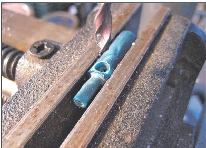
Photo 18. Expanding the hole to allow room to solder the LED and resistor.
