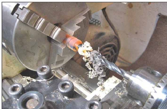
Photo 12. Drilling the hole for the batteries.
