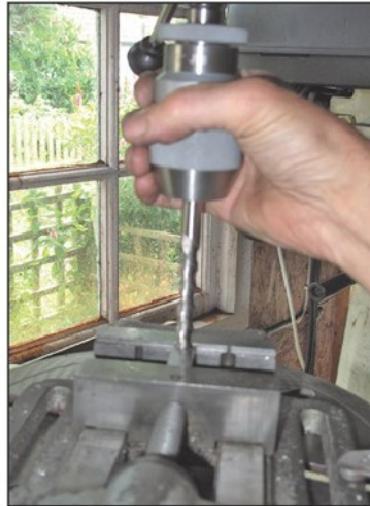
Photo 24. Using a fast fluted taper reamer mounted in the bench drill.
