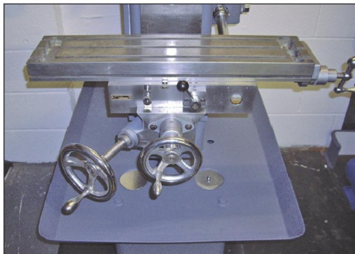
Photo 25. Table fitted, machine nearly finished.
