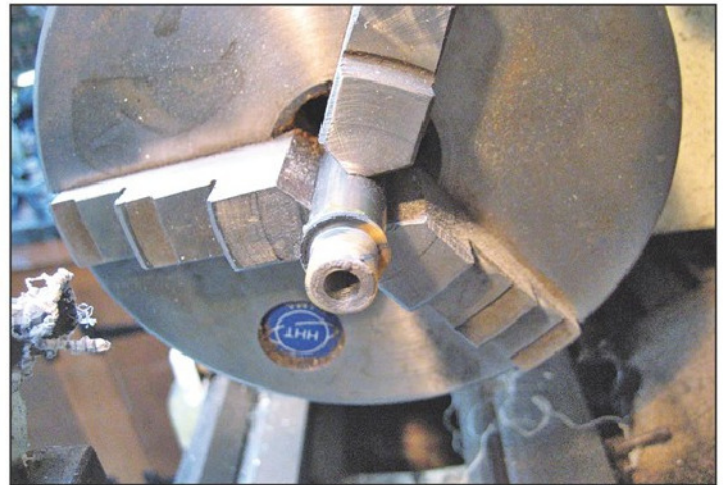
Photo 8. Turning the insulation to shape.
