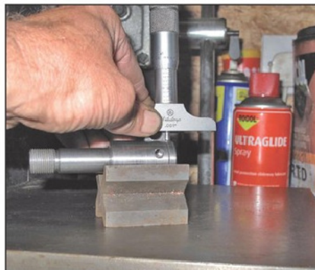
Photo 27. Working out the side clearance angle.
