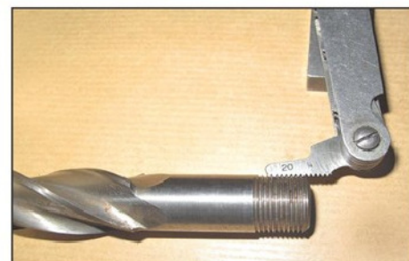
Photo 1. Establishing thread pitch at 20 TPI Whitworth form.
