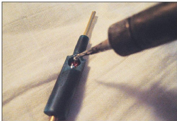
Photo 22. Showing the LED and resistor soldered to the central conductor.
