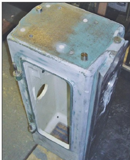
Photo 14. Column filled ready to rub down.
