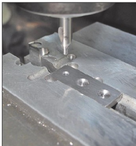
Photo 17. Centre drilling concave radius positions.
