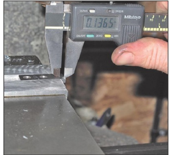
Photo 25. Measuring the wall thickness to establish total material removal.
