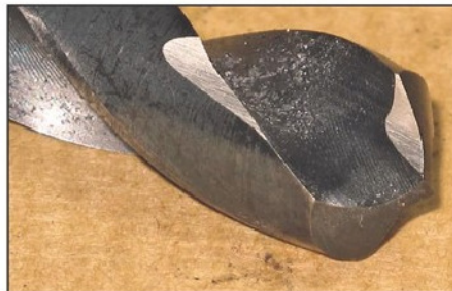
Photo 9. Drill after the web thickness reduction.
