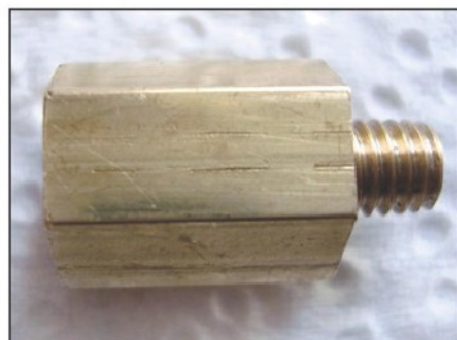
Photo 25. Side view of check valve body.
