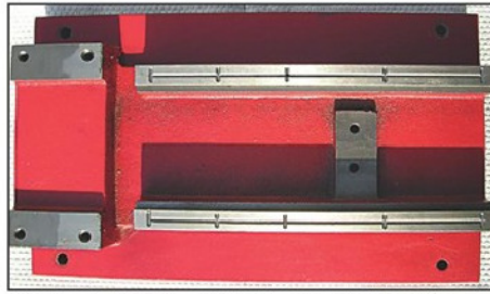
Photo 4. Finished Y axis oil distribution channels in base.
