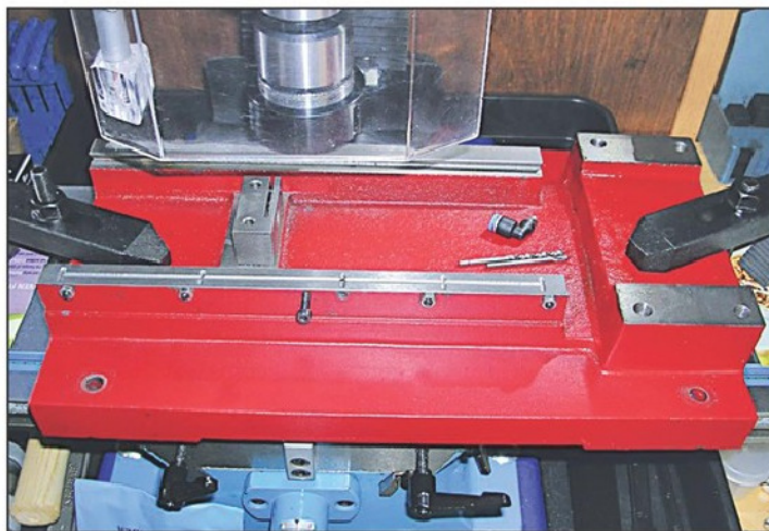
Photo 2. Cutting the Y axis oil distribution channels.
