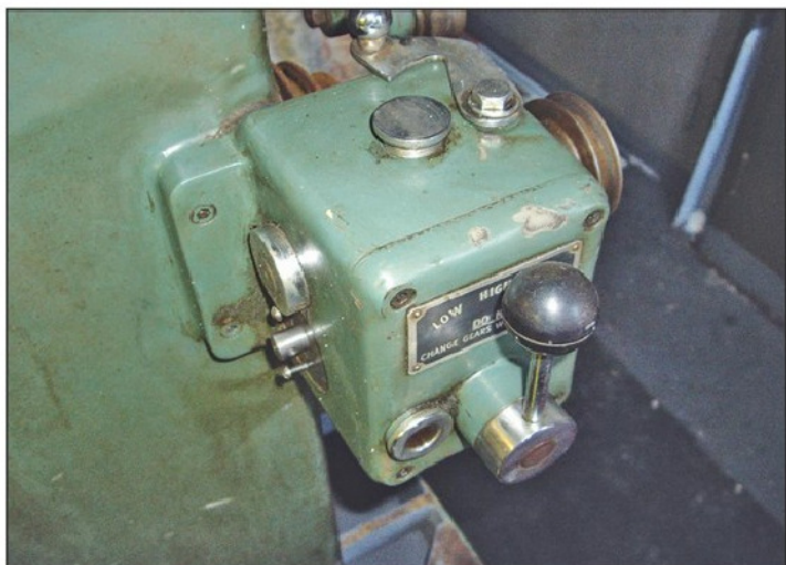
Photo 5. Power feed gearbox.
