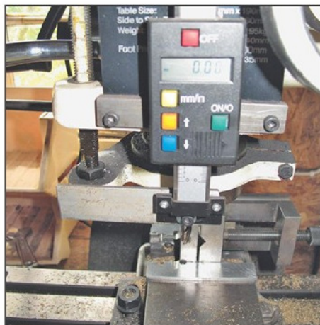
Photo 19. Z axis digital read out.
