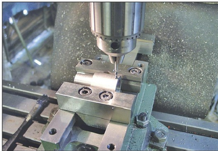
Photo 4. Tapping M3 for bearing retention screws.
