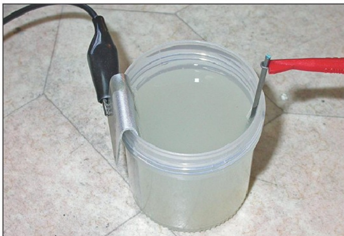
Photo 3. The simple anodising bath.
