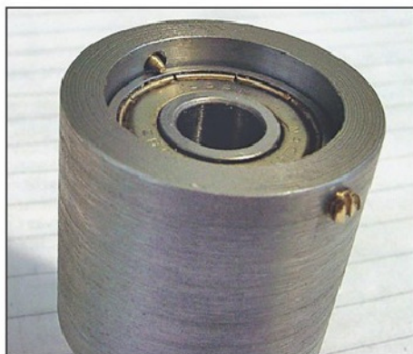
Photo 5. Tapers on screws lock bearings in place.
