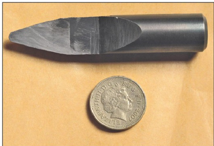
Photo 1. Silver steel "D" bit, milled to centre line, hardened and stoned to achieve smooth cutting edge.
