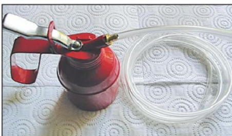
Photo 34. The finished oil pump (can) with quarter inch tubing fitted.
