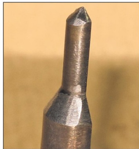
Photo 23. Backed off cutting faces.
