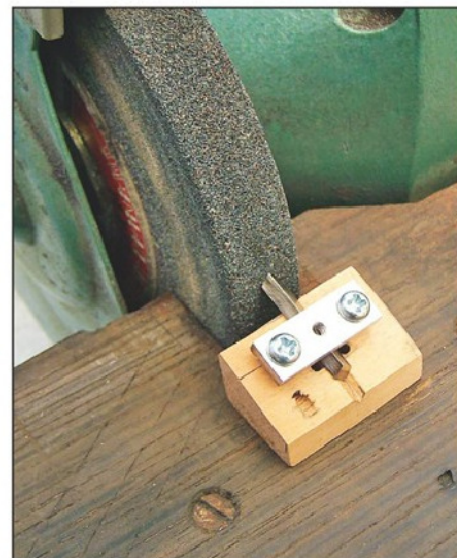
Photo 9. The sharpening jig on the grinder.
