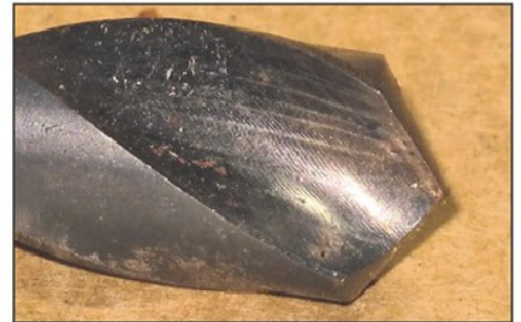
Photo 8. Drill before the web thickness reduction.
