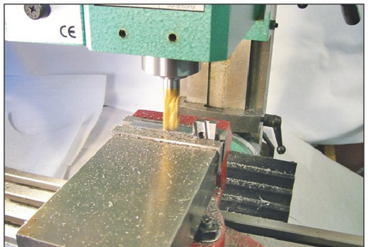
Photo 7. Finishing the tool shank.
