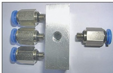
Photo 14. Bottom view of Y, Z and oil can manifolds.
