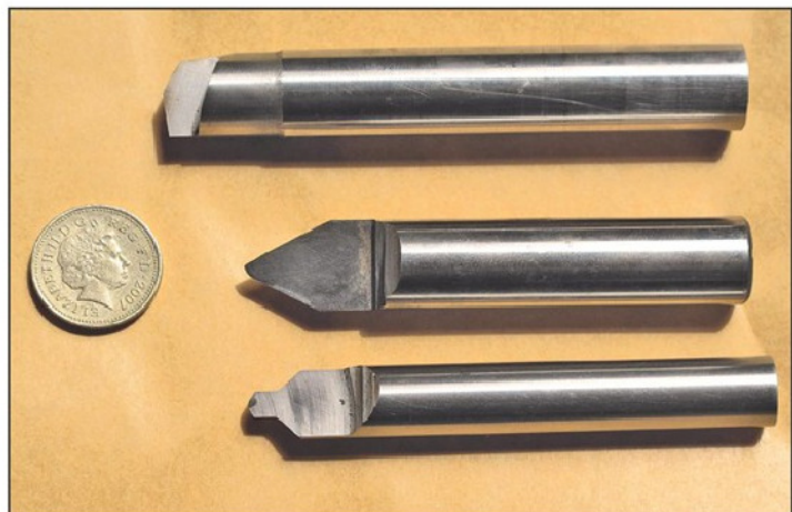
Photo 3. D bits ground from round HSS.
