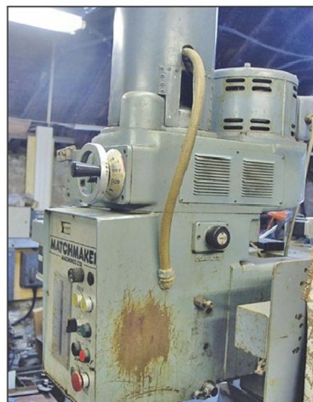
Photo 1. Matchmaker transmission is heavyweight and better suited to slow/medium speed applications.
