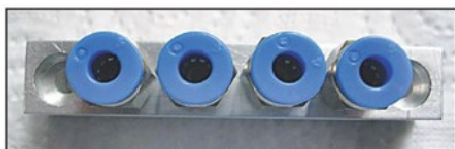
Photo 18. Top view of X axis manifold with push fit studs in place.
