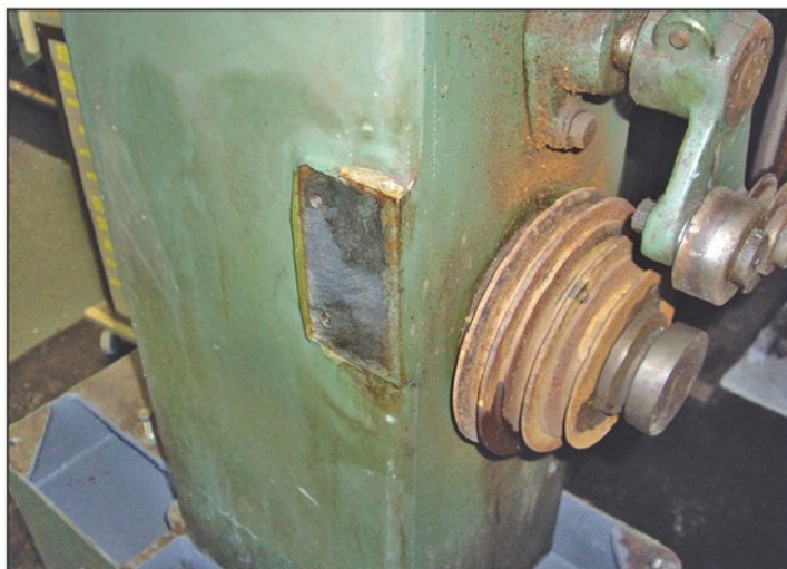
Photo 6. Power feed gearbox removed.
