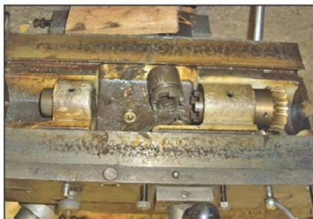
Photo 4. Inside the saddle at initial strip down.
