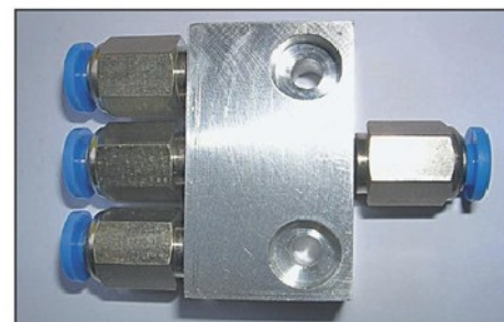
Photo 15. Front view of Y, Z and oil can manifolds.
