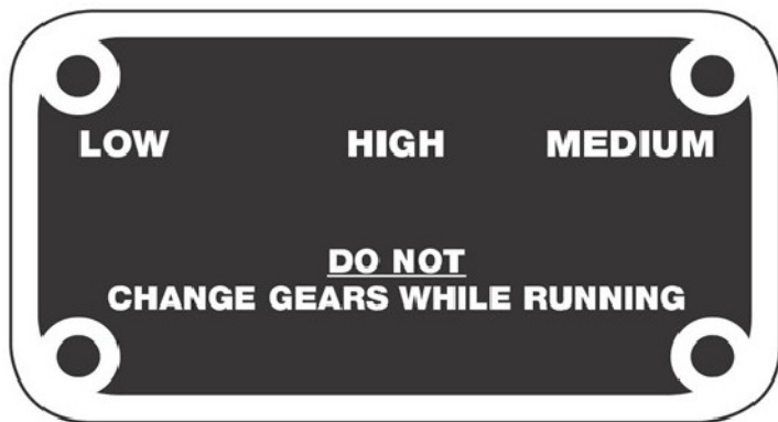
Power feed gearbox warning label made up using Word processor software for printing on transfer paper
