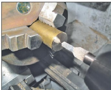
Photo 24. Proving D bit by plunge cutting
