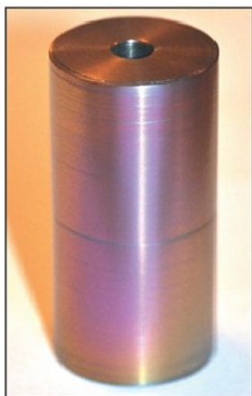
Photo 7. The first attempt at anodising the pendulum.
