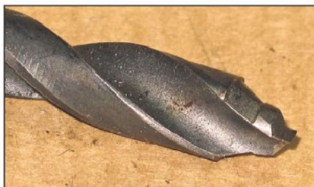
Photo 13 . Web thickness reduction.
