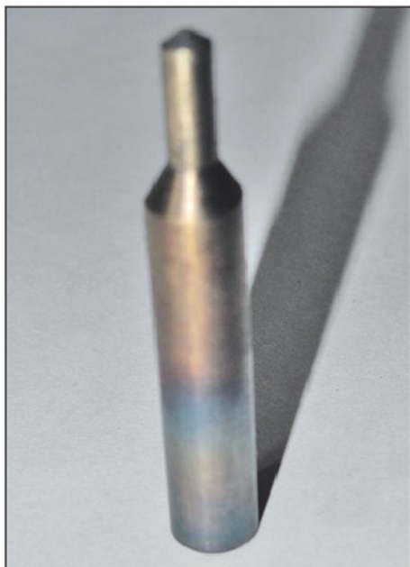
Photo 21. Tempering colours run from heat source at the base. Cutting faces achieving light straw colour.
