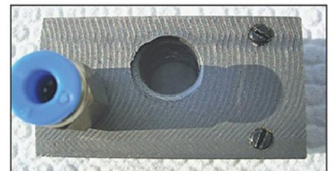
Photo 8. First attempt at oil distribution channel in leadscrew nut, front view.
