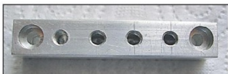
Photo 17. Top view of X axis manifold.
