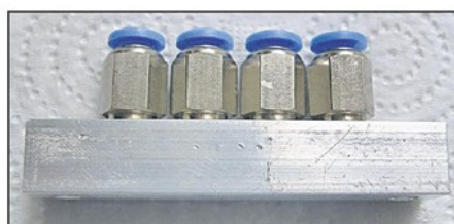
Photo 19. Front view of X axis manifold with push fit studs in place.
