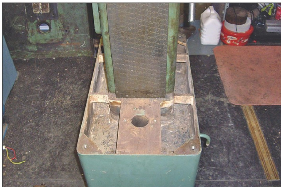
Photo 10. Coolant tank cleaned out.
