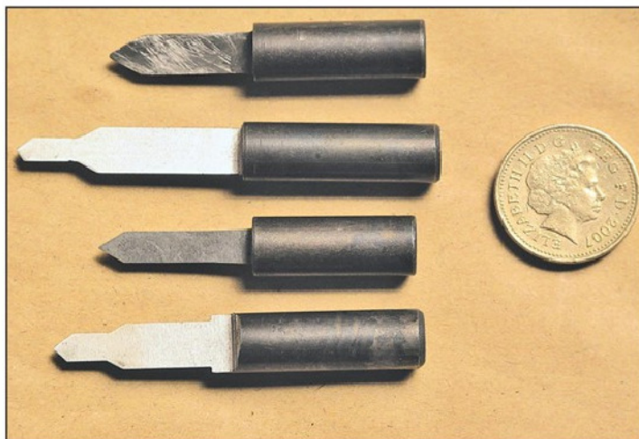
Photo 2. A range of silver steel "D" bits.
