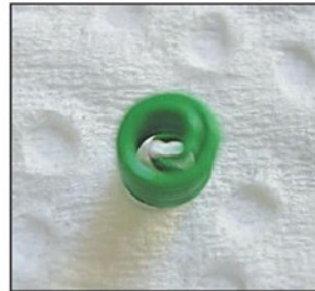
Photo 28. Close up of check valve spring.
