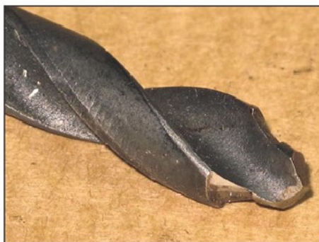
Photo 11 , a double diameter form drill, with 45 degree blend face.
