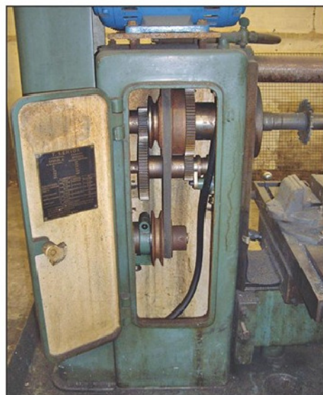
Photo 8. The column showing the side door.
