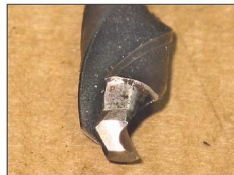
Photo 12 . Cutting face backed off.
