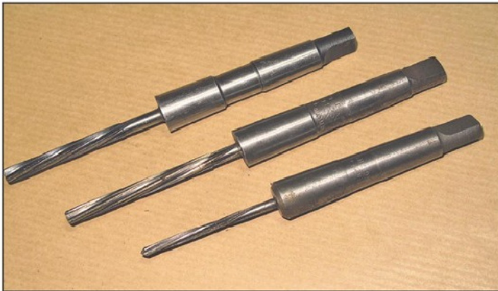
Photo 7. Small diameter machine reamers.
