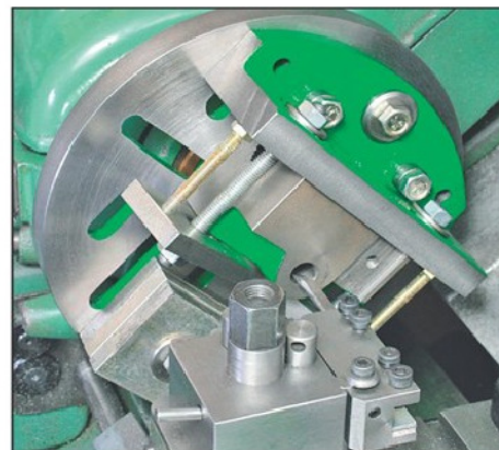
Photo 15. A typical use for the faceplate with angle plate.
