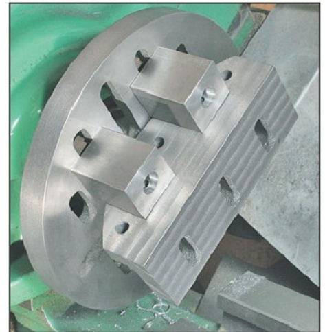
Photo 9. Whilst not actually machined in this way the photograph illustrates the method suggested by Hemingway for machining the angle plate if the workshop does not possess a milling machine.
