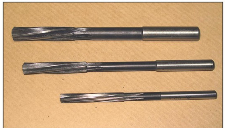
Photo 10. Chucking reamers with relieved shanks.
