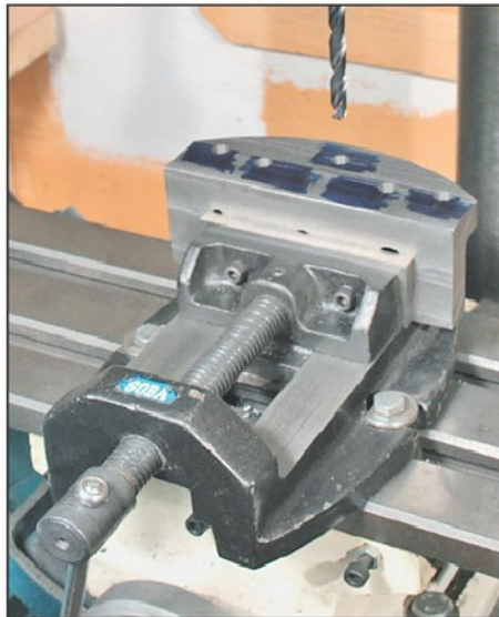
Photo 8. Drilling the fixing holes in the base of the angle plate.
