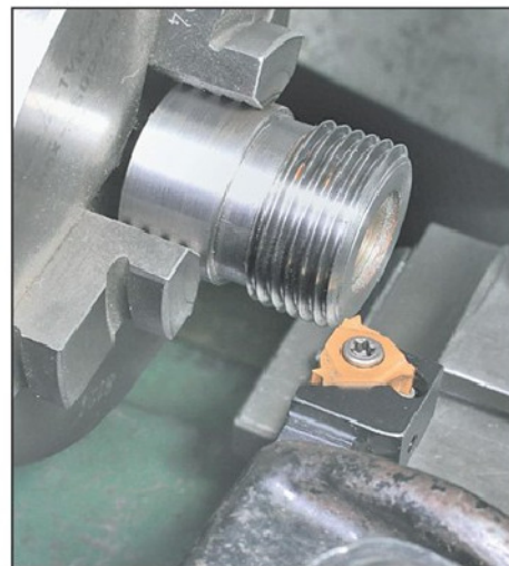
Photo 2. Ideally the gauge should be made with a tool that produces the full thread form.
