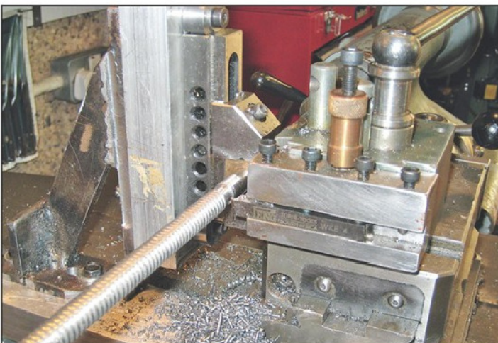
Photo 14. Screwcutting the leadscrew.
