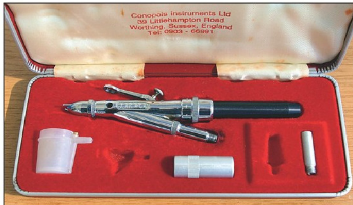
Photo 6. Conopois airbrush (no longer made) was considered a high quality item.
