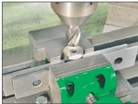
Photo 12. Machining the steps of the Tee nuts.
