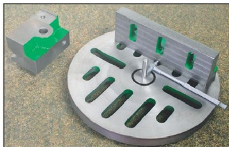
Photo 14. Using a bore diameter gauge to set the distance of the angle plate from the centre of the faceplate.
