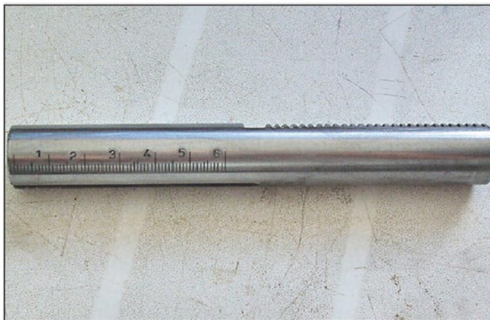
Photo 22. The finished tailstock.
