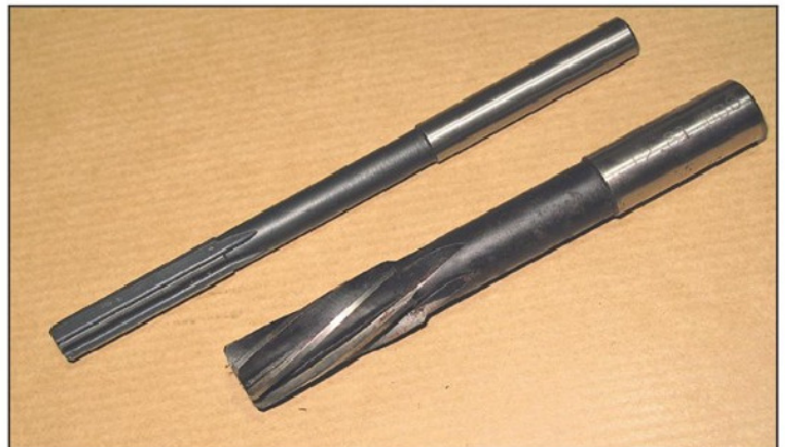
Photo 4. Straight and helical fluted chucking reamers.
