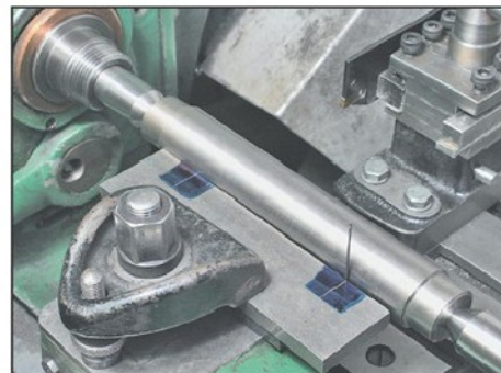
Photo 3. Setting the top slide to an angle of 0.6deg. gives a 100:1 axial to radial ratio.
