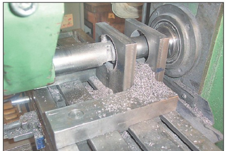
Photo 6. Boring the headstock.
