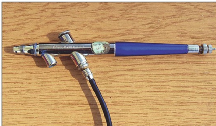
Photo 5. Badger 200 airbrush is a low to mid range device.
