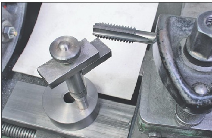
Photo 7. Checking the setting of the tap, the leading edge must cut very marginally deeper.
