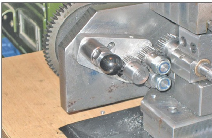
Photo 19. The tumbler gear system.
