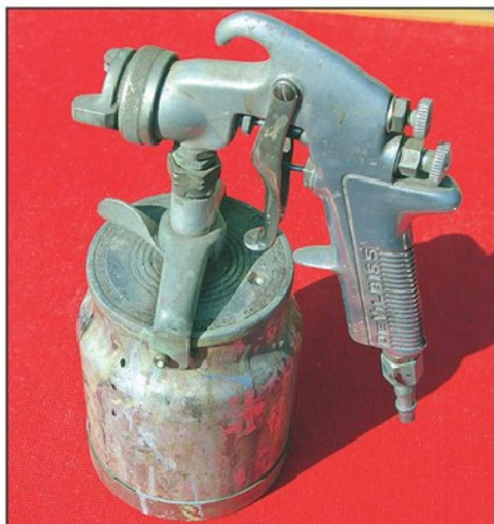
Photo 7. DeVilbiss spray gun large enough for vehicle respray work.
