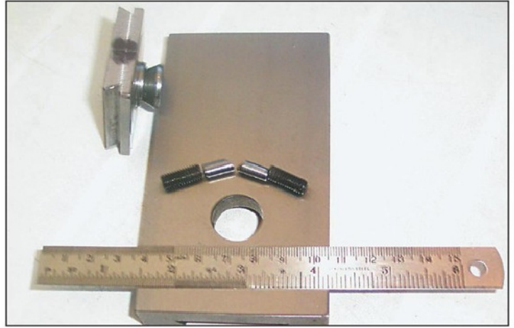
Photo 12. The swiveling topslide is similar to the Myford Super 7 mount.
