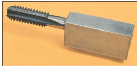
Photo 6. A simple holder for holding a tap being used for machining internal threads.
