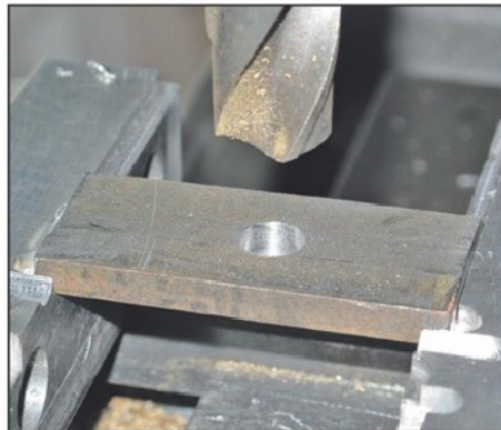
Photo 15. Ready to drill with a \frac{27}{32} drill.
