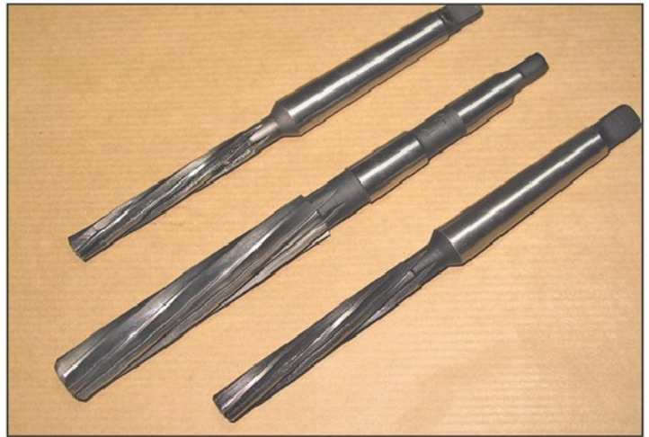
Photo 2. Different sizes of machine reamers, mounted on 2 Morse shanks.
