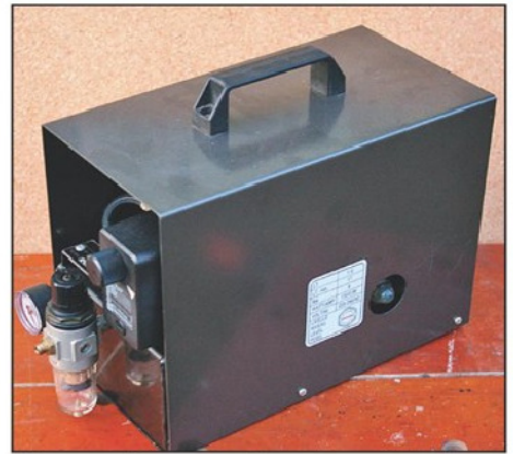
Photo 12. Better quality compressor has small receiver and pressure cut off switch.
