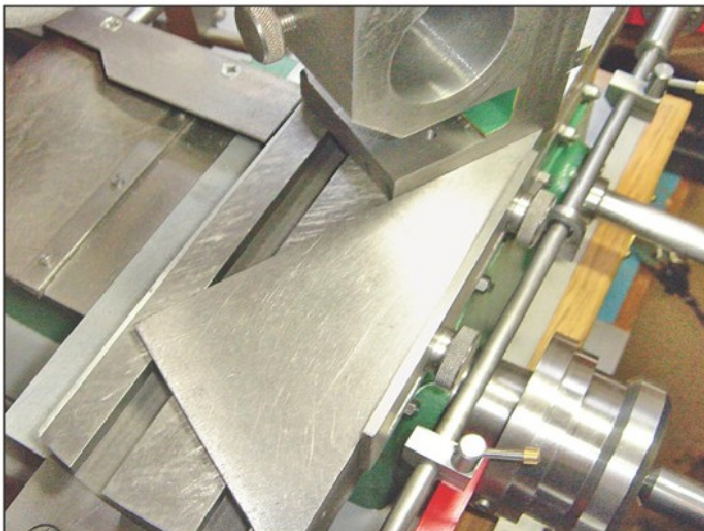
Photo 15. The bracket is set to 30deg.
