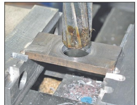
Photo 18. Reamer with cutting paste applied.
