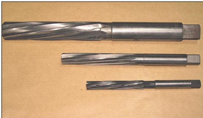
Photo 3. 1in. to 3/8in. diameter hand reamers.
