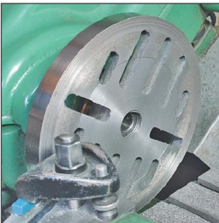
Photo 3. Facing the plate's main face.
