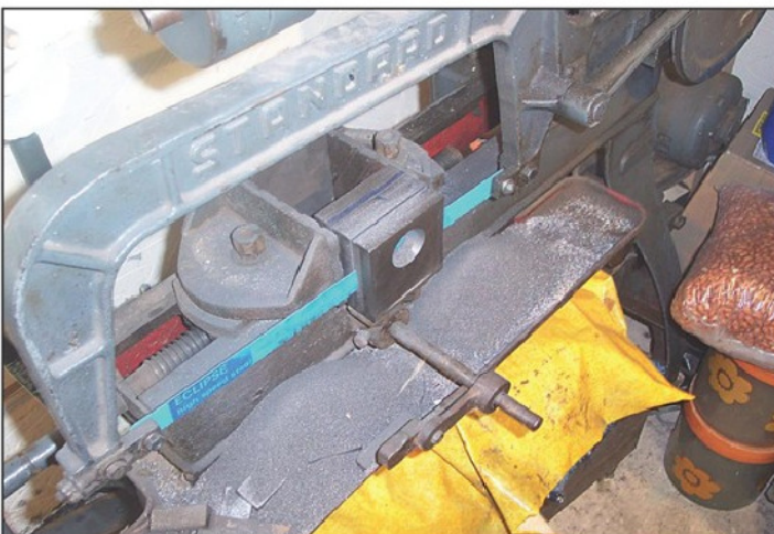
Photo 5. Making the headstock blanks.
