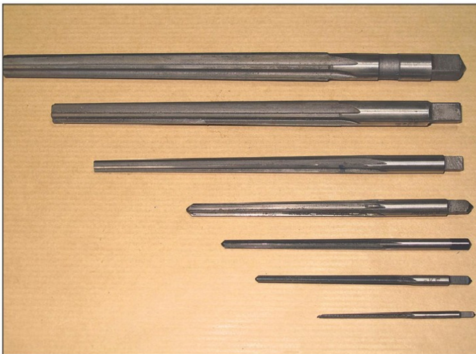
Photo 21. Selection of different size taper pin hand reamers.
