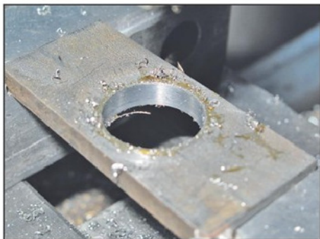
Photo 19. The finish reamed bore.
