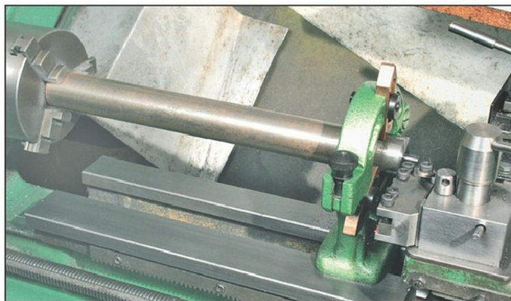
Photo 16. Using the fixed steady as shown enables small parts to be made without there being a small length of bar left in the chuck after parting off that may not find a use.
