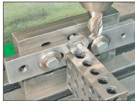
Photo 13. Machining the ends of the Tee nuts.
