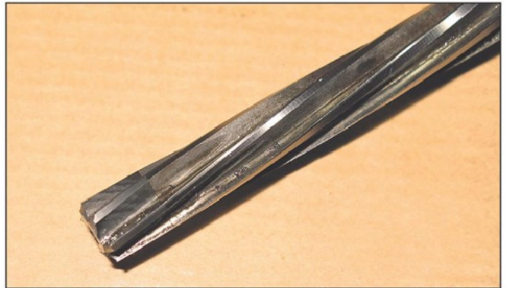
Photo 8. HSS machine reamer with carbide tip.
