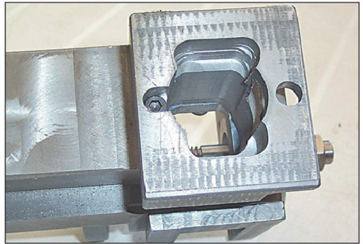
Photo 4. The finished hole through the bed.
