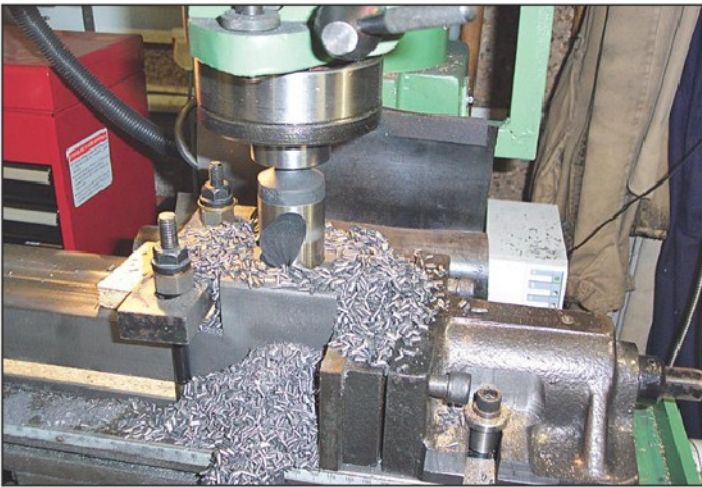
Photo 3. Drilling a hole through the bed.
