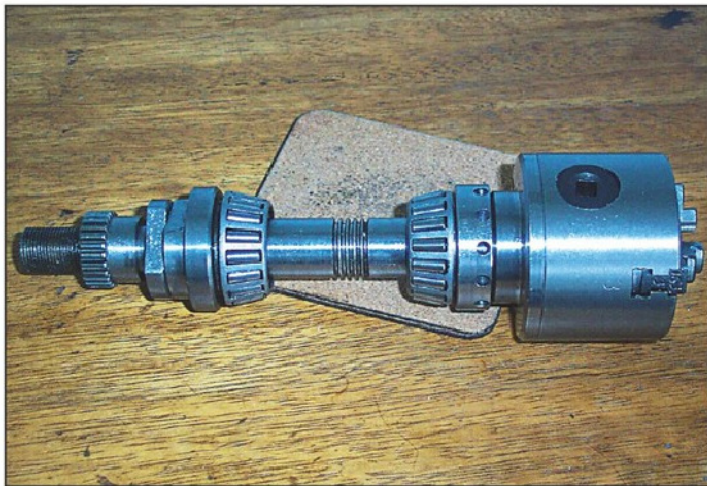
Photo 9. The mandrel and tapered roller bearings.
