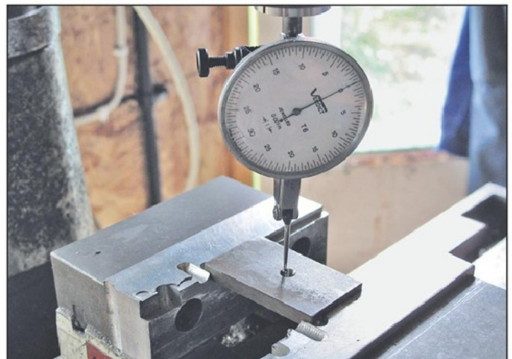
Photo 12. Picking up pre drilled centre on the bench drill.
