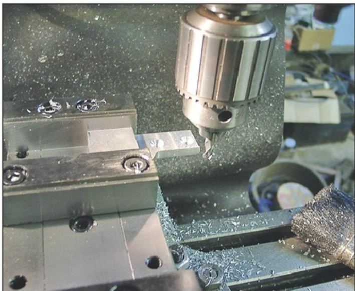
Photo 14. End of bracket is trimmed to be flush with main head body.
