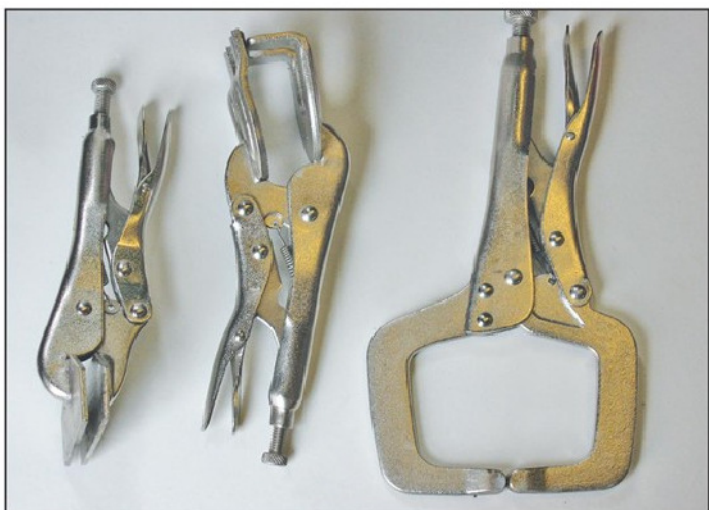
Photo 8. Assorted welding clamps, ideal for quick and easy clamping of awkward items.
