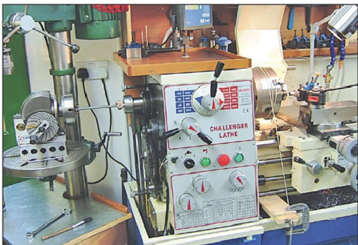
Photo 7. Dividing head supported on drill table for graduating scales.
