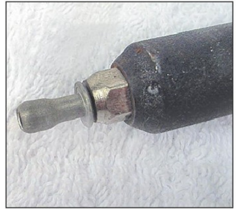
Photo 8. Pop rivet compressed.
