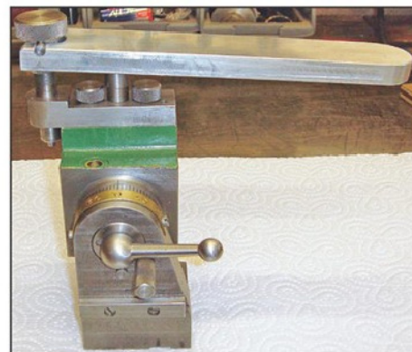
Photo 5. The universal head and bracket.
