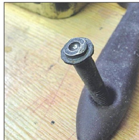
Photo 4. Support dolly for round head rivets made from a bolt.
