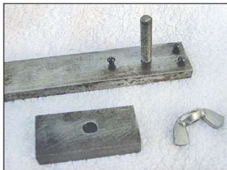
Photo 2. Jig for trimming rivets to length.
