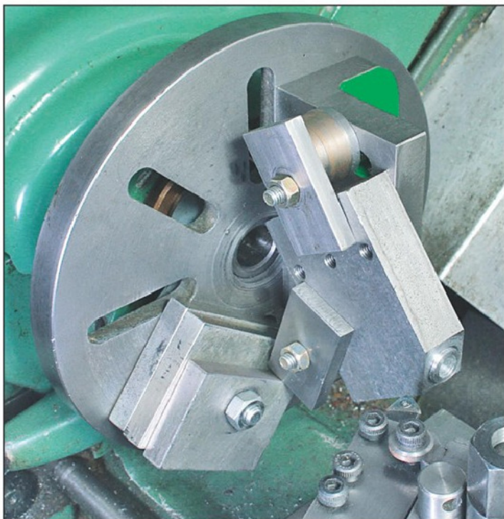
Photo 11. An example of an angle plate being used.
