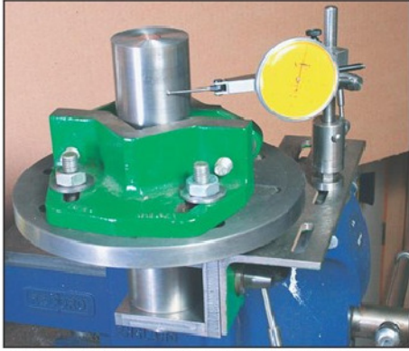
Photo 13. Setting the bar in the Keats angle plate to run true.
