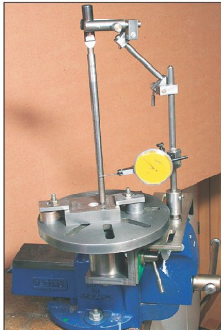
Photo 18. Using the balancing fixture to set up a workpiece with a centre finder and DTI.
