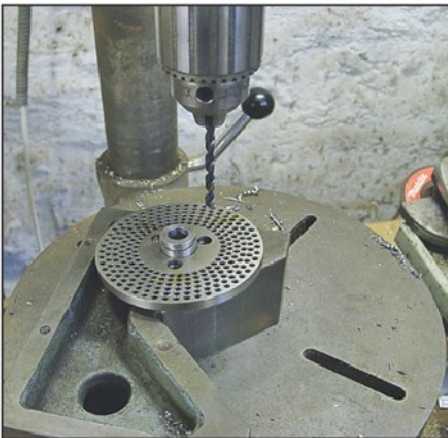
Photo 10. Spotting through for plate attachment.
