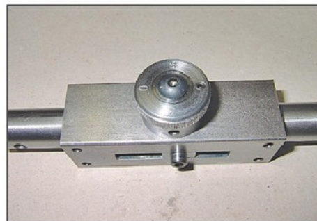
Photo 5. New depth stop dial and slide block secured with a screw head turned down to fit the lever bar.
