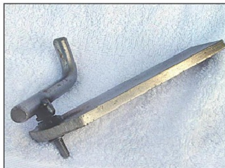
Photo 11. Home made insertion tool using Allen screw.
