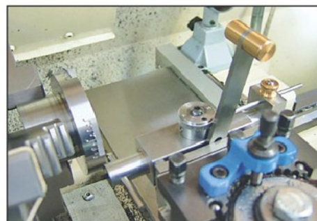
Photo 6. Indexing a scale on the diameter.
