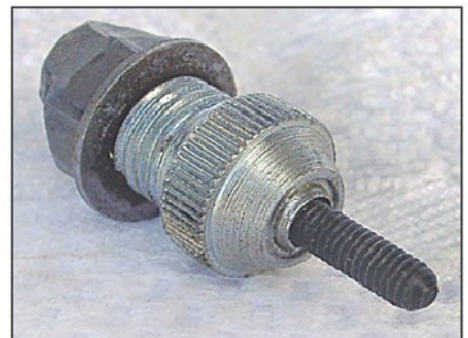
Photo 12. Insertion tool made by welding nut to professional item. Static nose is simply held in mole grips.
