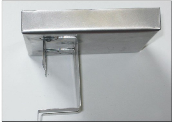
Photo 13. Tray and brackets after welding.
