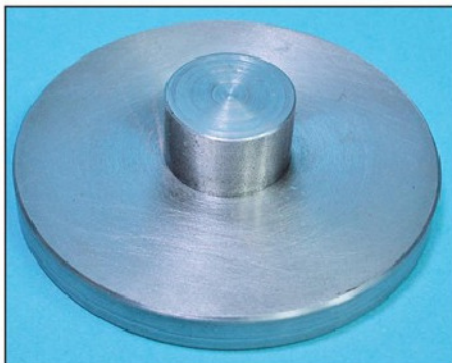
Photo 14. A small (75mm diameter) shop made faceplate for mounting in the three jaw chuck.
