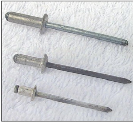
Photo 6. Three typical Pop rivets.
