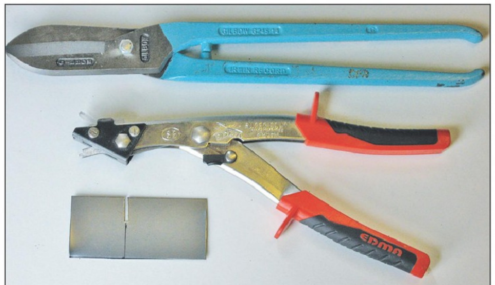
Photo 3. Gilbow shears and a hand operated nibbler, cheaper alternatives to the bench mounted shear.
