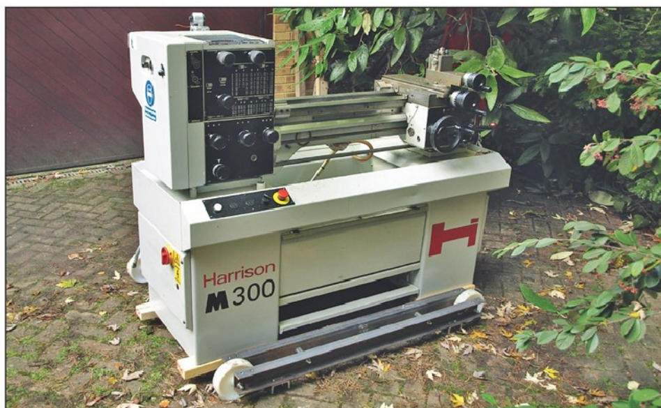
Photo 3. The homemade wheeled cradle.
