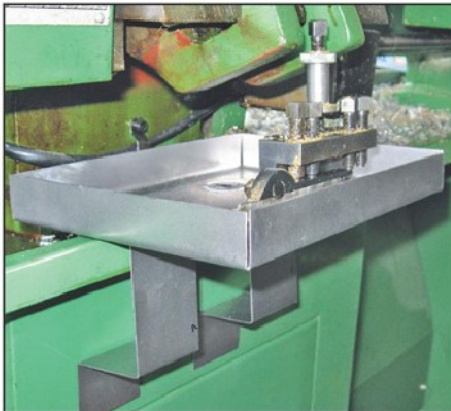
Photo 1. Finished tray in use on the lathe.
