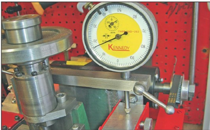
Photo 3. The new dial indicator holder.
