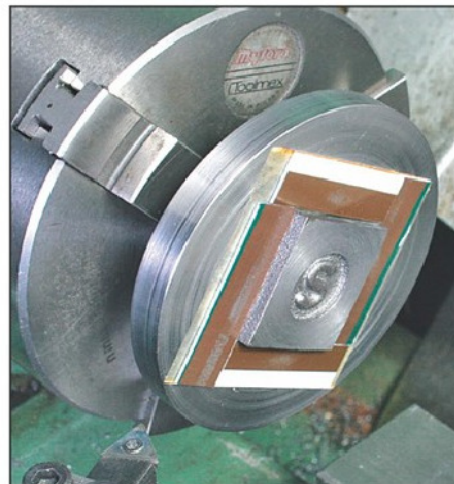
Photo 15. Machining a steam chest cover. The cover is held using double adhesive tape.
