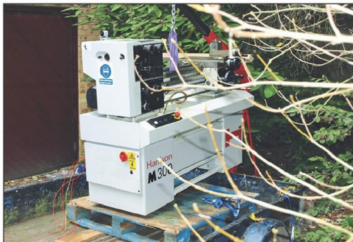
Photo 1. Lifting the lathe from the trailer.
