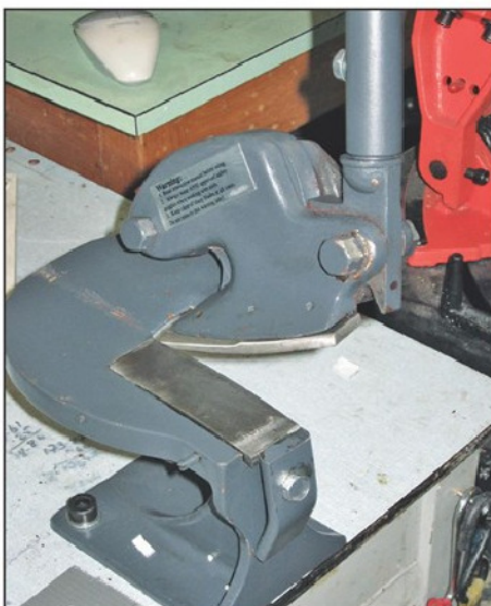
Photo 2. Throatless shear - cuts sheet material very easily and efficiently.
