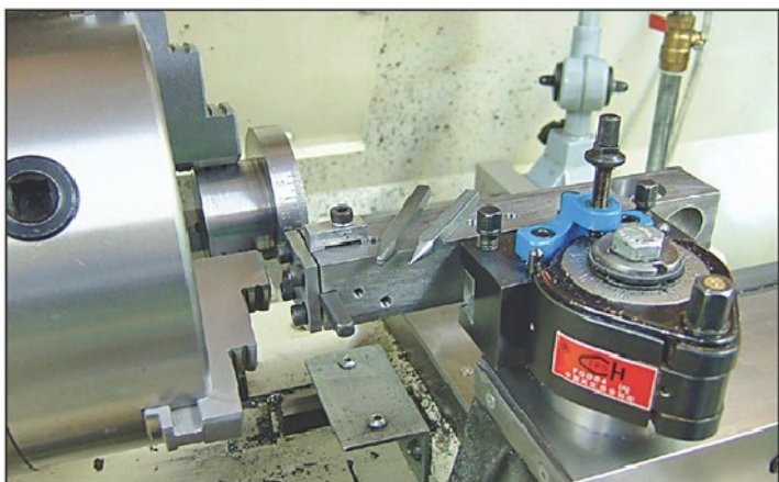
Photo 9. Number stamping the indexed scale.
