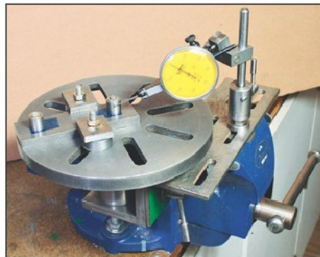
Photo 19. Toolmaker's buttons have been fixed to the workpiece and the first one is being set to run true when it will be removed for machining to take place.
