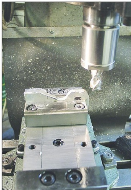
Photo 13. Initial squaring up of material for the bracket.
