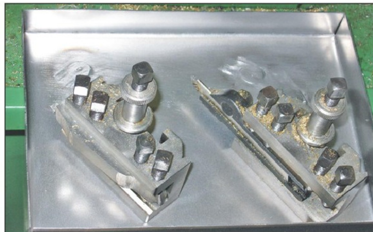
Photo 14. Finished tray in use and showing welds ground flush.
