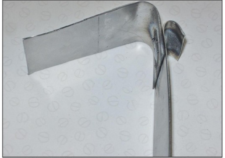
Photo 11. The weld featured in photo 9 after being subjected to a concerted attempt to break it.
