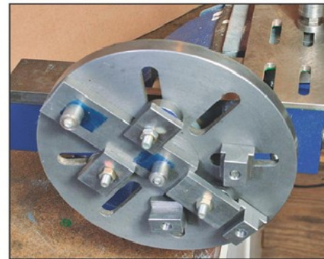
Photo 20. The balancing fixture has been moved into the balancing position and weights added, compare this with photograph 19.
