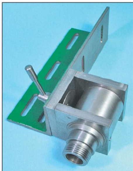
Photo 17. A faceplate balancing fixture.
