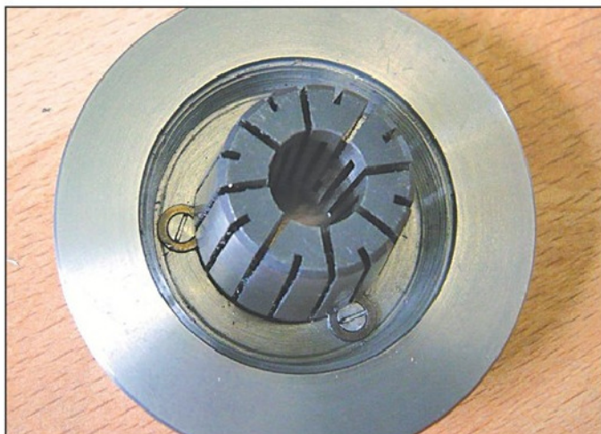
Photo 40. ER32 collets can be fitted directly to the lathe mandrel.
