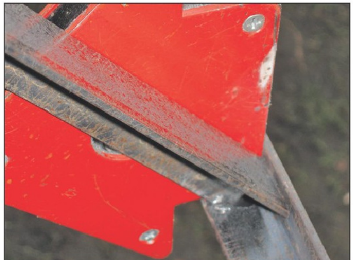
Photo 9. Mounting handles to main body
