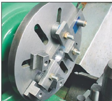
Photo 3. The first button has been removed and the workpiece bored.
