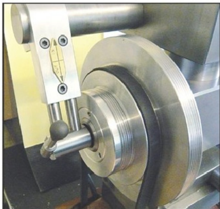
Photo 41. The cam operator controls the boring head.
