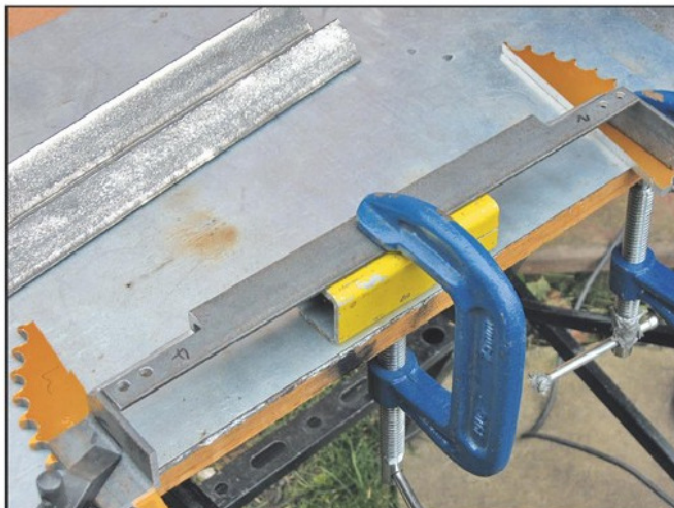
Photo 8. Aligning feet for welding again!
