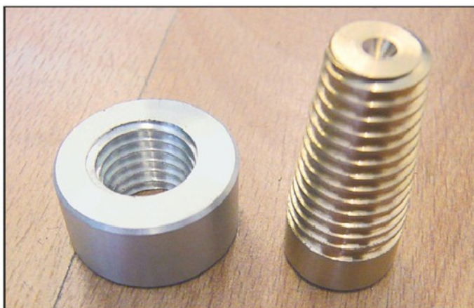
Photo 42. An example of taper threading.
