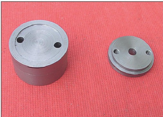
Photo 19. Completed upstand (left) and clamp disc (right).
