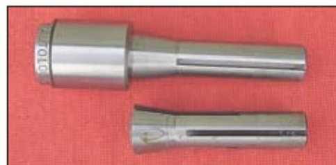
Photo 7. R8 Clarkson Milling chuck above, and collet below.
