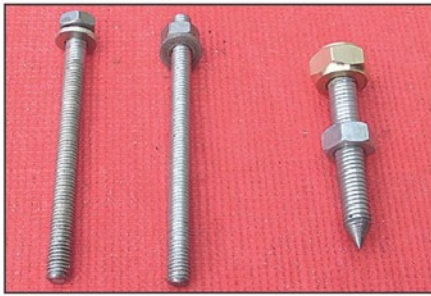
Photo 13. Adjuster screw on right shown with the two screwed rods.
