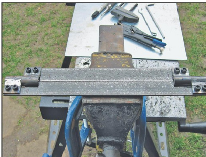
Photo 6. Pivots mounted to main body.
