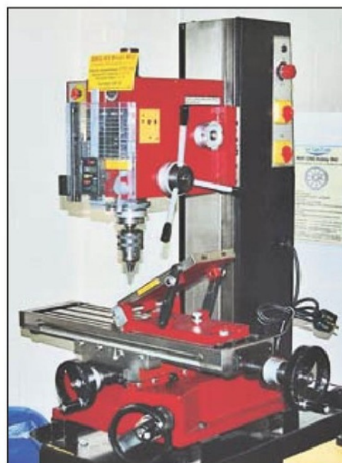
Photo 6. X3 from Arc Euro Trade has a fixed head, a dovetailed column and variable speed.
