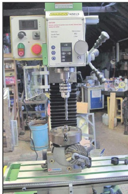
Photo 15. A tall set up, still room to work and the head could rise further.
