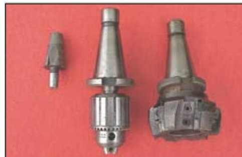
Photo 8. An INT 30 adapter (left) shown with two INT 40 arbors carrying drill chuck and face mill.
