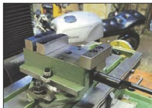
Photo 15. Warco DH1 vice has gripping length similar to footprint.
