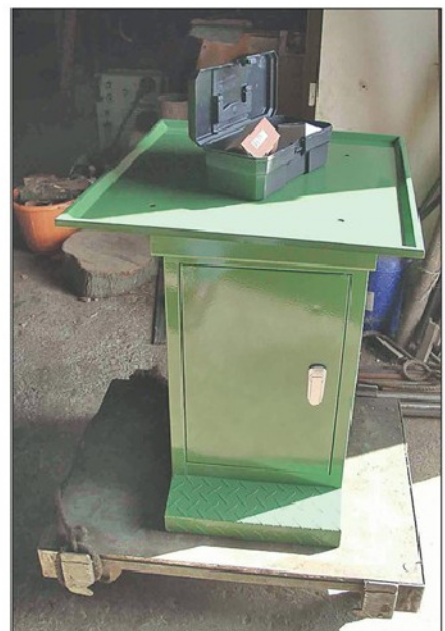
Photo 4. Stand and tray perched on trolley for easy movement. Also visible is the supplied toolbox.
