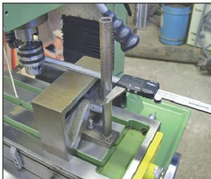
Photo 12. Set up to assess leadscrew accuracy.
