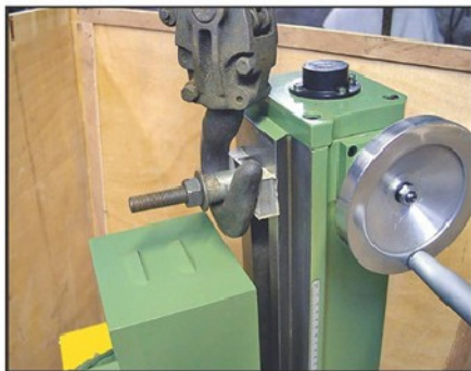
Photo 5. Lifting bracket clamped to machine column.
