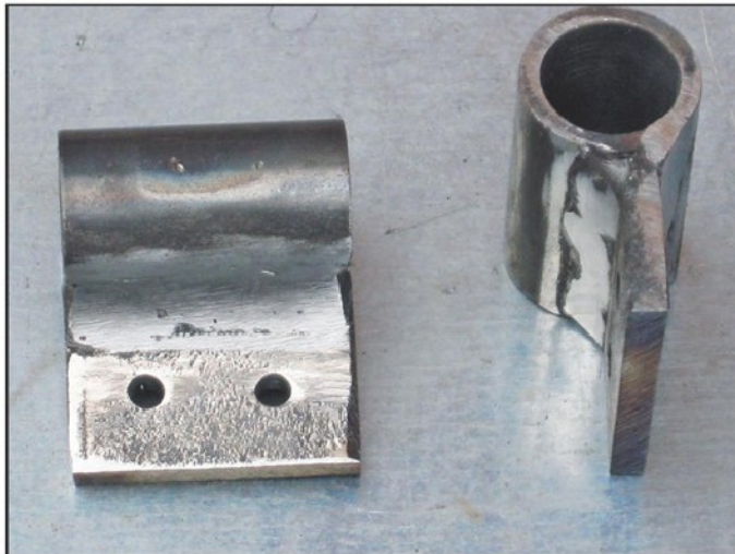
Photo 4. Pivots after welding.
