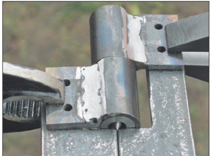
Photo 5. Aligning pivots on folder main body.
