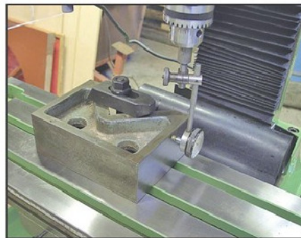
Photo 13. Perpendicularity of X and Y was investigated by clocking along sides of Vee block.
