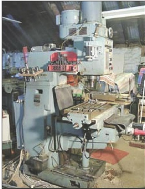
Photo 1. Matchmaker, though CNC, shows typical industrial vertical mill construction.
