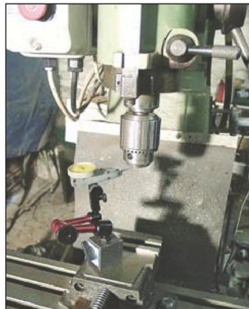
Photo 12. Clock positioned to check spindle end float.
