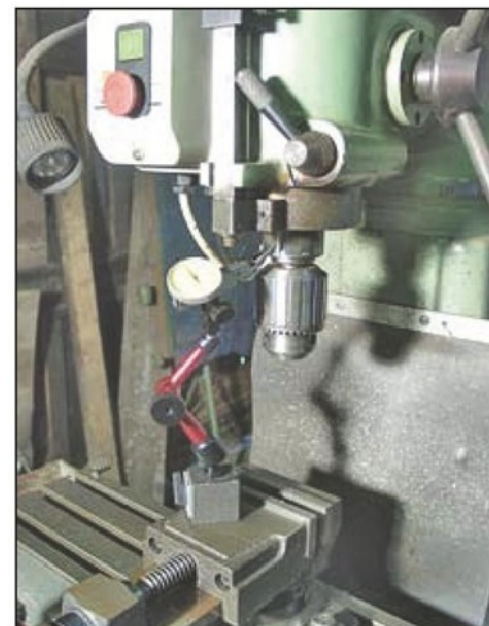
Photo 11. Checking for lateral play in bearings and quill.
