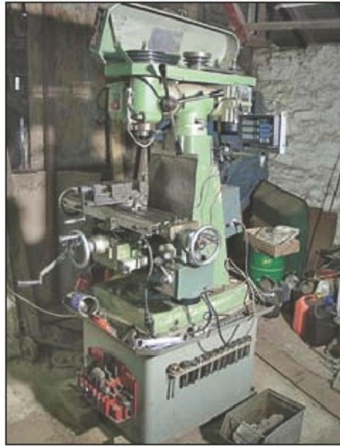
Photo 2. VMC mill, Myford variety with low speed conversion and digital readout on two axes.
