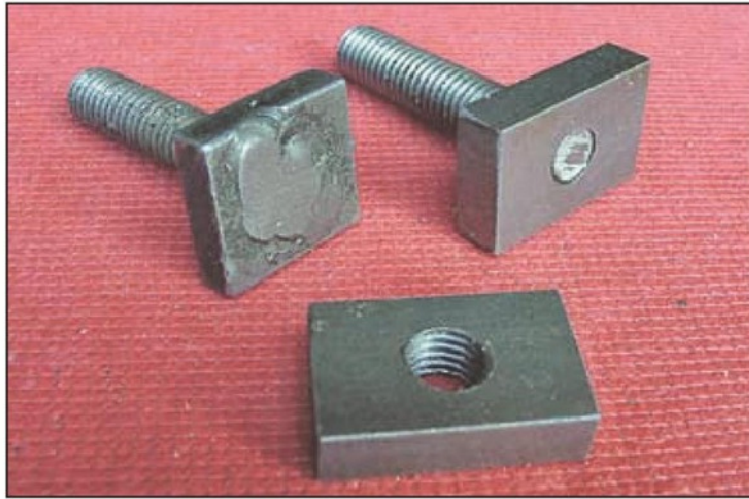
Photo 16. Rudimentary Tee bolts and nuts.
