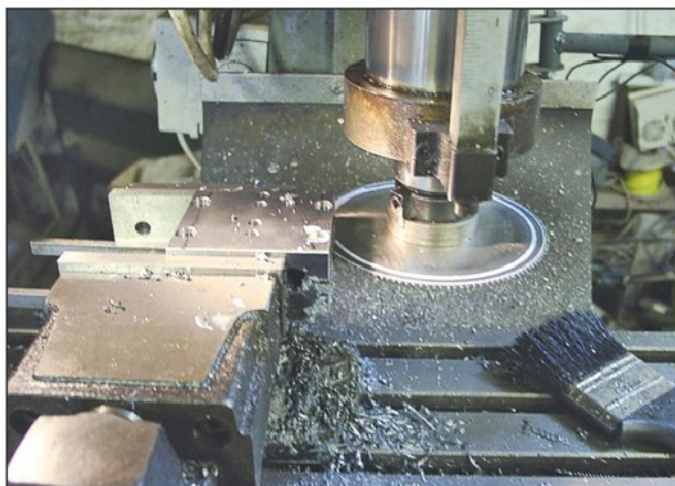
Photo 5. Slitting saw used to cut slots.
