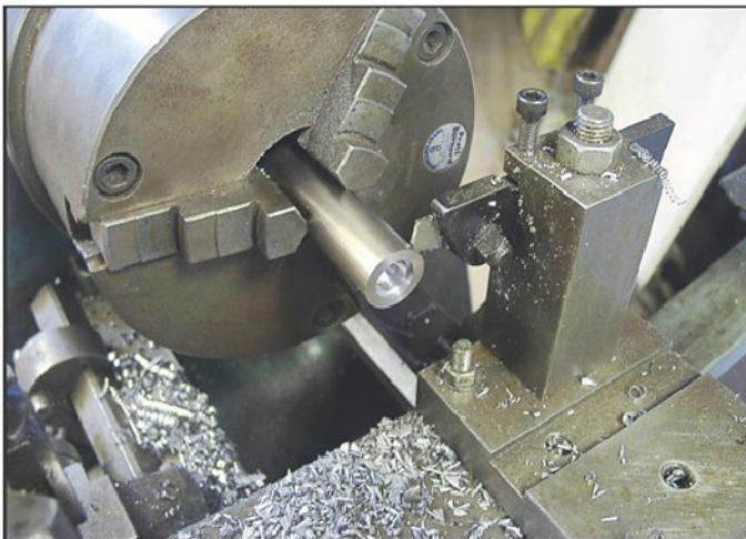
Photo 11. Commencing the part off operation on the spacer.
