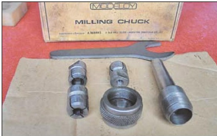
Photo 18. This Modeloy chuck has 2MT arbor and served both on mills and lathe.
