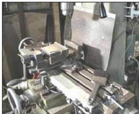
Photo 13. Typical 4in. swivelling milling vice, this one from Vertex.
