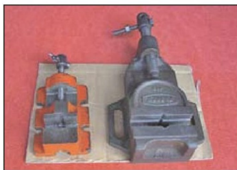
Photo 14. Myford vice (left) is a quality product useful for fine work, note weld repair beneath screw on vice to right.
