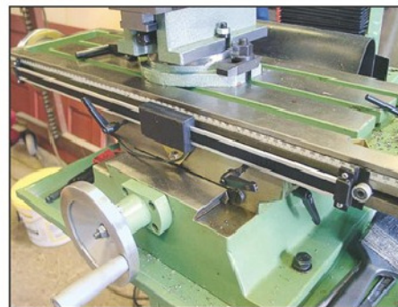
Photo 3. Scale fitted to WM18 mill.
