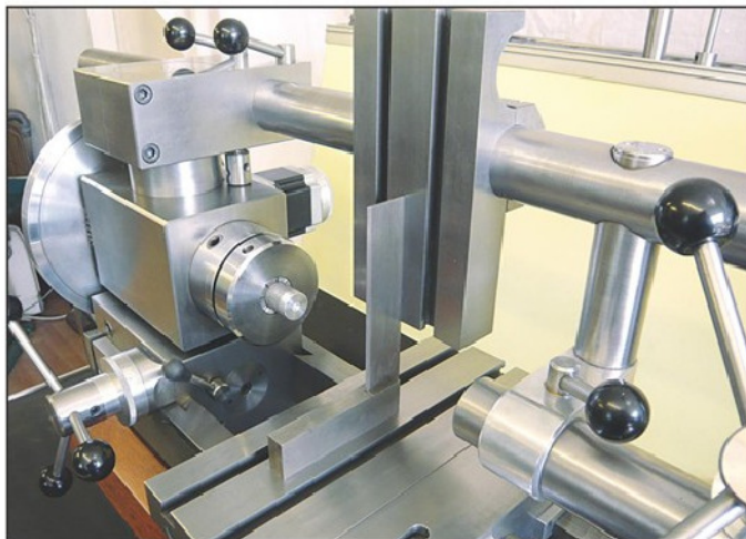
Photo 38. The mounting table can be mounted on a cross bar...
