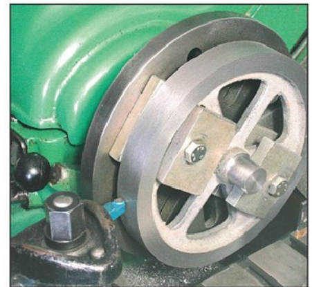
Photo 9. Not all large components are difficult to fix as this photograph of a flywheel being machined shows.
