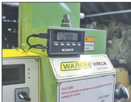
Photo 5. Remote readout is held in place by magnets.
