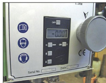
Photo 9. Detail of front of head showing built in DRO and to the right, the fine feed wheel for quill movement.
