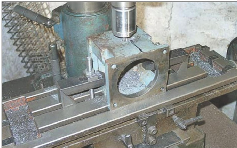
Photo 4. Machining a casting on the Naerok 350.
