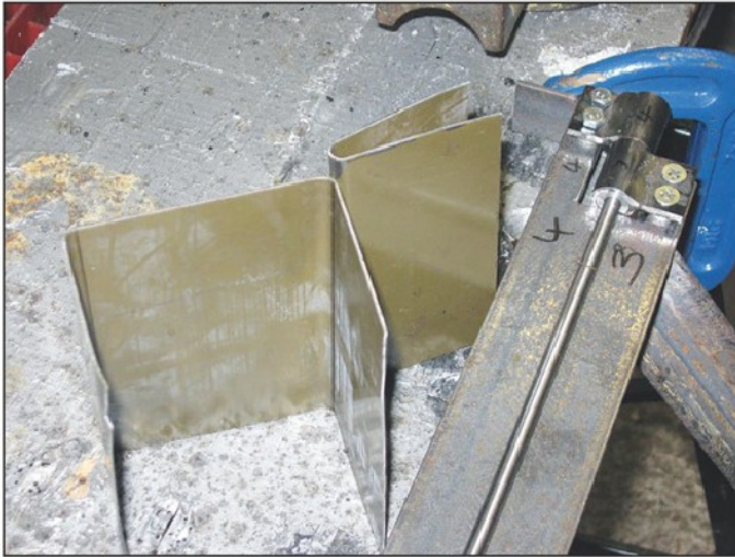
Photo 10. Test pieces produced using the folder
