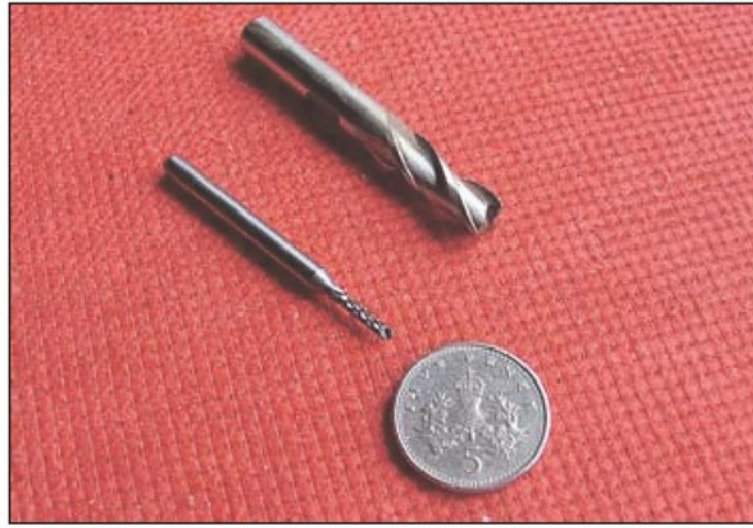
Photo 10. 1/16in. FC3 cutter above, and 1/16in. solid carbide below.
