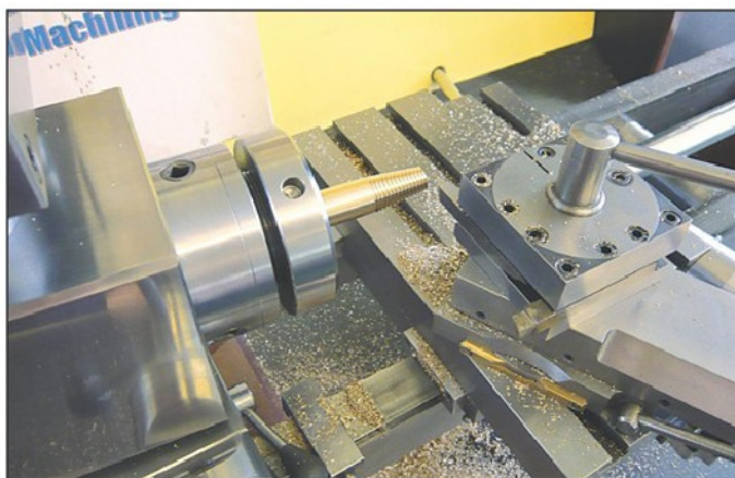
Photo 43. Taper threading in the lathe.
