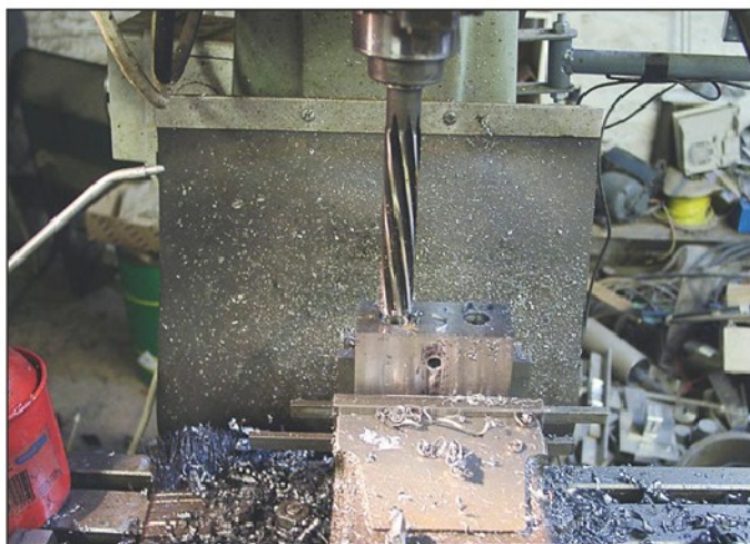
Photo 4. Reaming the bore for the spindle.
