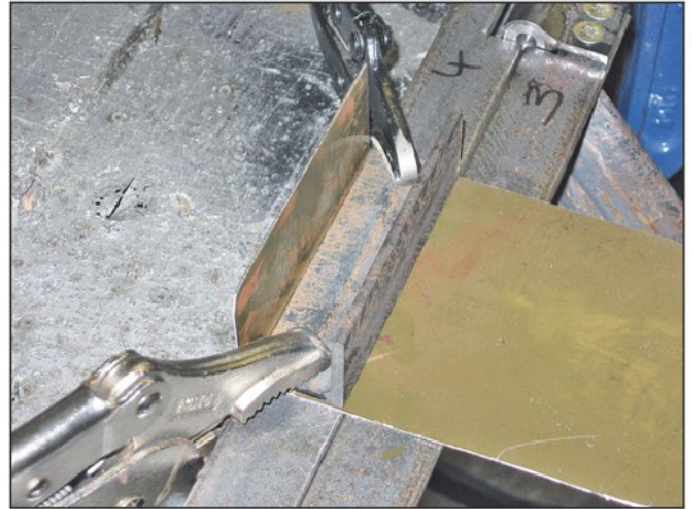
Photo 11. The folder in action producing a sharp bend
