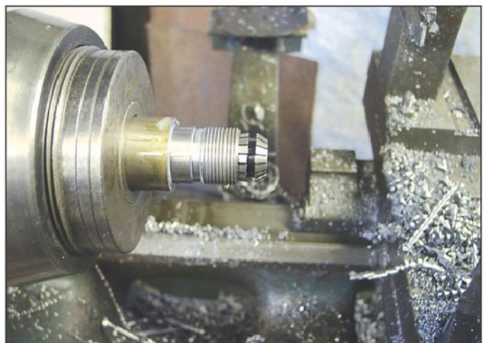
Photo 6. Collet is tried for size, about 4mm projection to the extraction groove.
