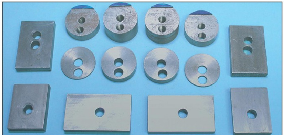
Photo 10. The faceplate clamp components. The small raised portion of the packing piece has been marked with marking blue to highlight its position.
