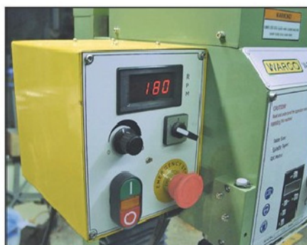
Photo 8. With the spindle running, the rev counter has large, clear numerals.
