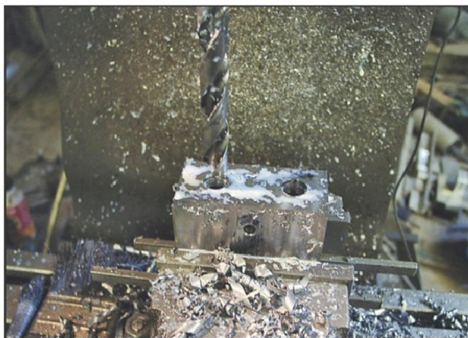
Photo 3. Drilling the body.
