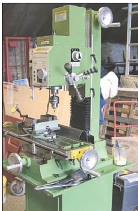
Photo 5. Warco WM 18 features dovetailed column, inclinable head and variable speed.
