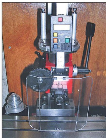
Photo 13. The guard mounted on the mill.
