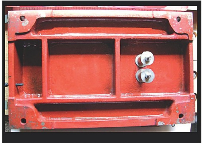
Photo 16. The base has had a thin coat of resin.
