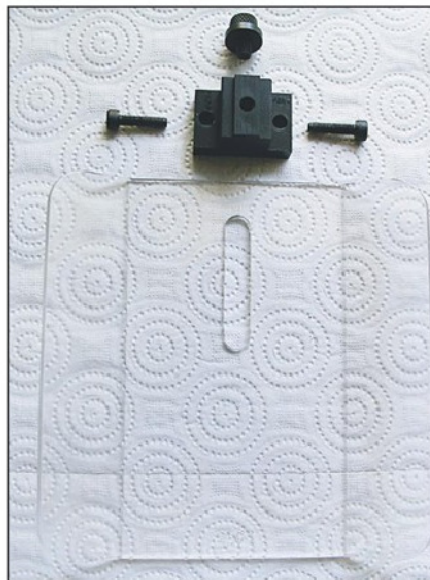
Photo 10. The spindle guard assembly.
