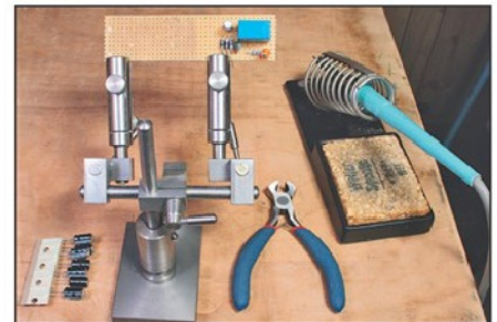
Photo 16. Being used as a heavy duty helping hand for assembly.
