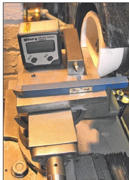
Photo 56. Three way vice set up to grind lathe tools.
