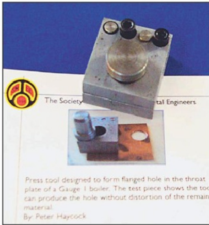
Photo 11. Press tool for small boiler throat plate - Peter Haycock.
