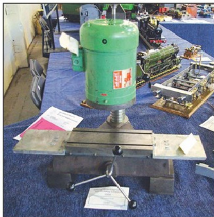
Photo 20. MES surface grinder by Mr A Bootland.
