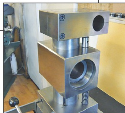
Photo 21. The headstock bored out for the bearings.
