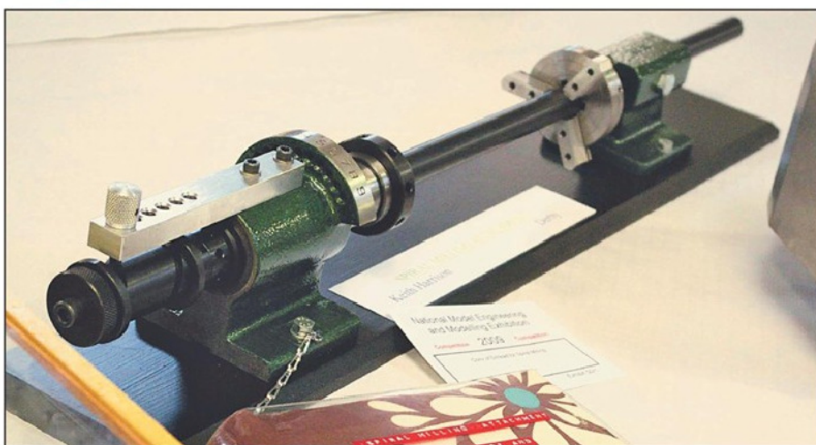
Photo 3. Mr K Harrison's modified dividing head for spiral milling.
