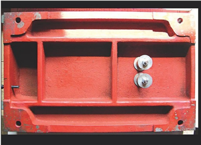
Photo 15. Copper tube between the washers protects the bolt holes.
