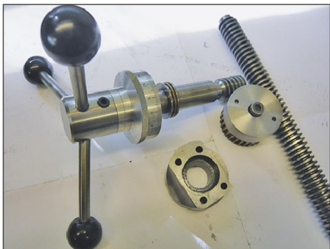
Photo 25. The headstock raising and lowering handle
