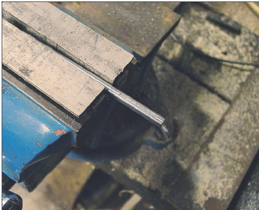
Photo 6. Work is easier to hold if left long.
