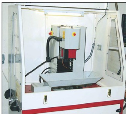
Photo 24. KX1 CNC mill from Arc Euro Trade.
