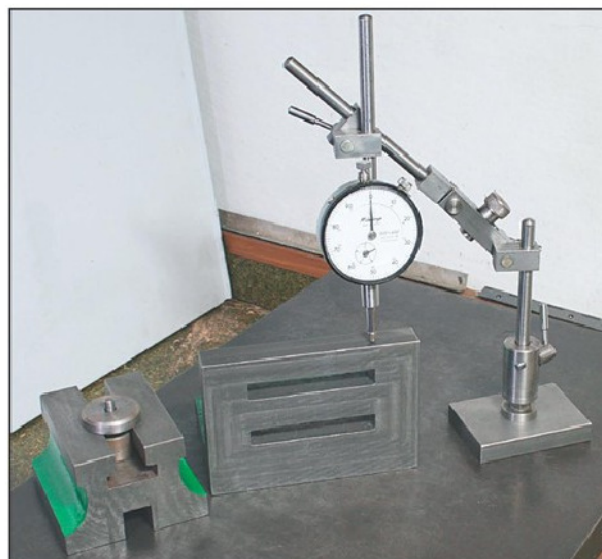
Photo 12. Showing a typical use for the Adjustable Arm. The photograph also shows an alternative base. (Ref. 2)
