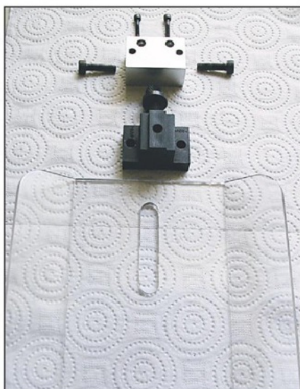
Photo 12. The parts for the new spindle guard assembly showing the spacer block.
