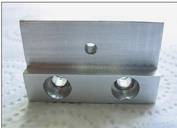
Photo 6. The block carries the bottom end of the DRO.
