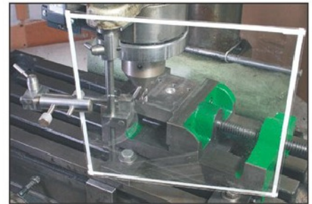
Photo 15. The guard in this picture is not intended to prevent contact with the moving cutter, though it may help. Its intended purpose is to protect the operator from flying fragments of hot swarf.
