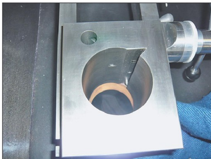
Photo 26. The key can be removed to rotate the headstock.
