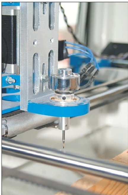
Photo 5. The motor assembly on the machine, compare its size to the Dremel in photo 2!
