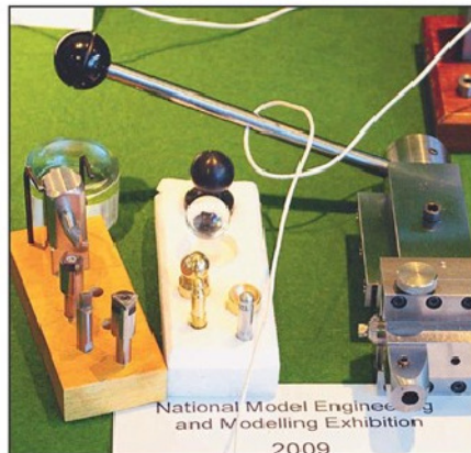
Photo 17. Modified ball turning tool by Mr S Hauptman.
