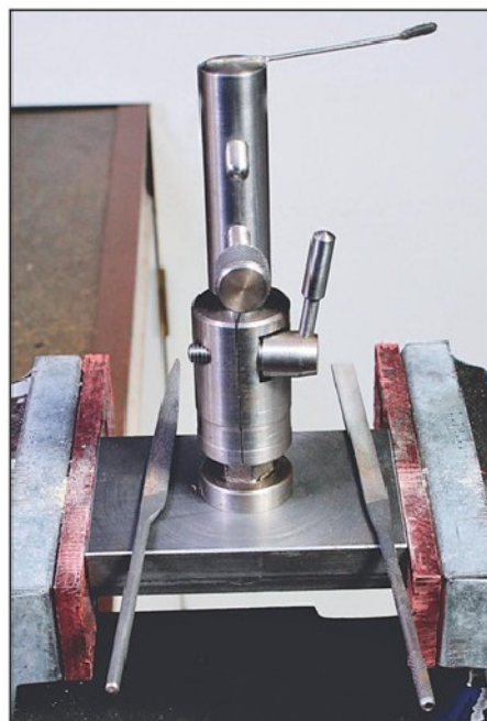
Photo 12. Showing a typical use for the Adjustable Arm. The photograph also shows an alternative base. (Ref. 2)
