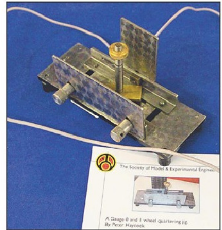
Photo 13. Wheel quartering jig for gauges 0 and 1 - Peter Haycock.
