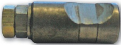
Photo 67. Excess metal is removed prior to boring.
