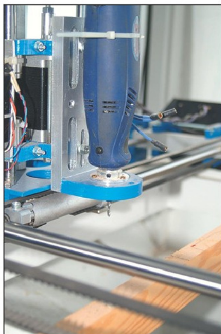
Photo 2. Dremel style tool in the miller, note the cable tie to steady it.
