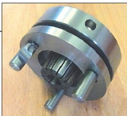
Photo 20. Collet chuck showing camlock fittings.
