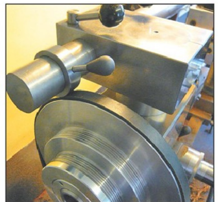
Photo 27. The cam is used to lock the mandrel.
