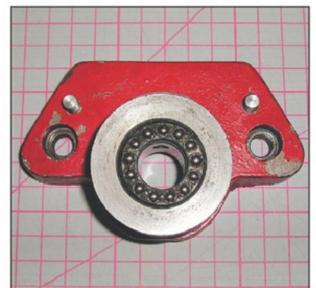
Photo 10. Bearing plate drilled and tapped.
