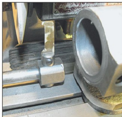
Photo 54. The hook shaped finger for sharpening saws.
