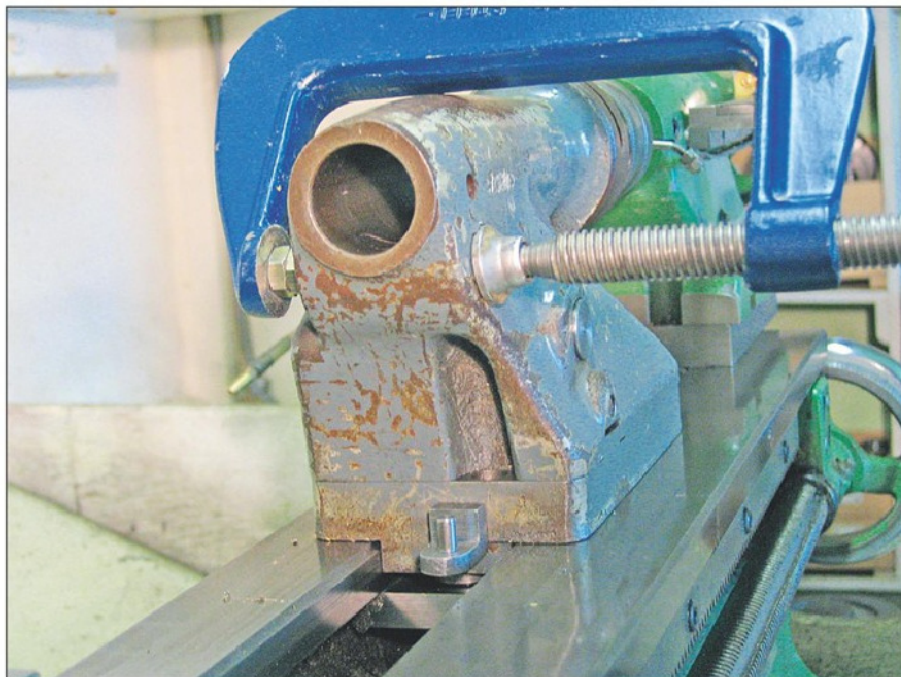
Photo 68. The method of securing the split clamp prior to boring.
