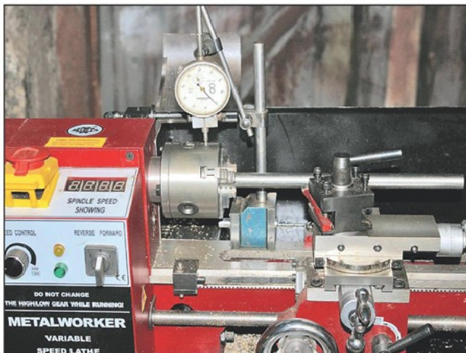
Photo 8. Movement caused by pushing up/down on the bar would be picked up by the DTI. This lathe has been retro fitted with taper roller races for extra rigidity.
