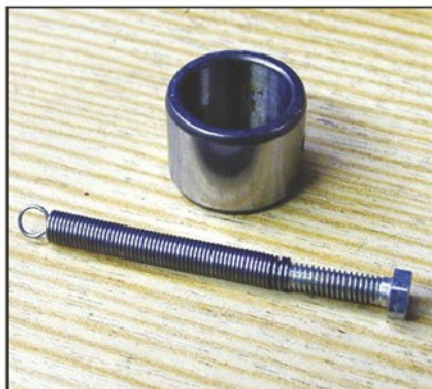
Photo 12. Detail of one track, tension spring, and 5BA screw.
