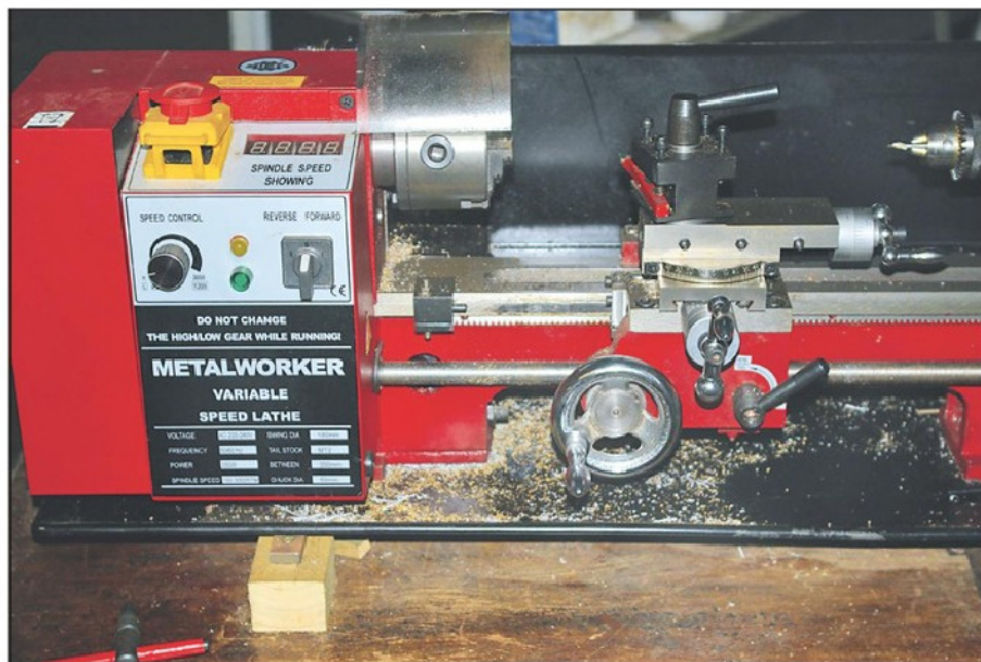
Photo 1. Mini-Lathe typifies the straight bed design.
