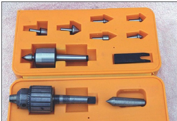
Photo 13. The drill chuck and centre (bottom row) are regarded as essential; the live centre kit (upper section) can be useful for particular types of job.
