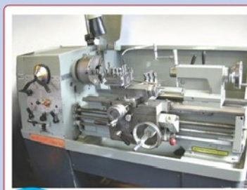
Colchester Student 1800: 6" x 24" + gap bed, 3 & 4 jaw chucks + 240 volts!
