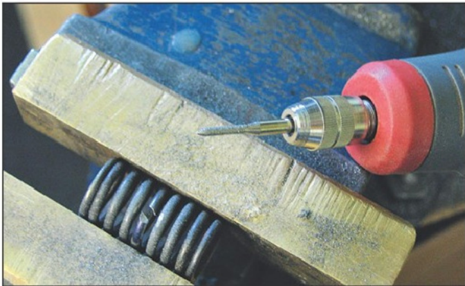
Photo 57. Separating the halves of the spring with a diamond burr.
