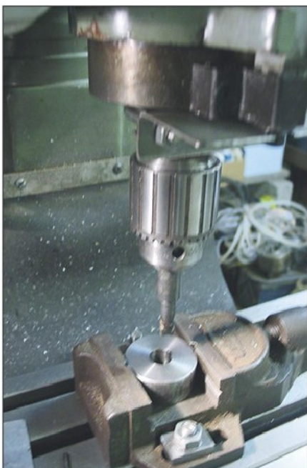
Photo 21. Keyway tool and spindle lock fitted.
