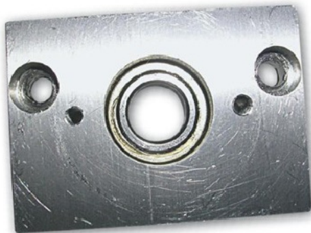
Photo 3. Finished bearing plate.
