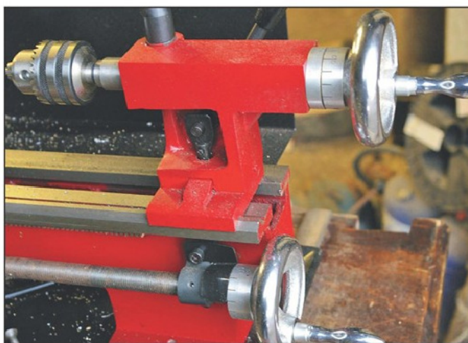
Photo 16. This Mini-Lathe has been fitted with a leadscrew handwheel, also an indexable collar on the tailstock wheel.
