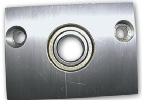
Photo 2. Partially completed bearing plate.
