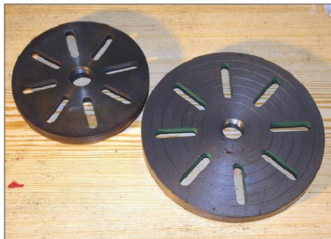
Photo 11. Myford now offer a larger 9in. (228mm) diameter faceplate (right) in addition to the earlier pattern.
