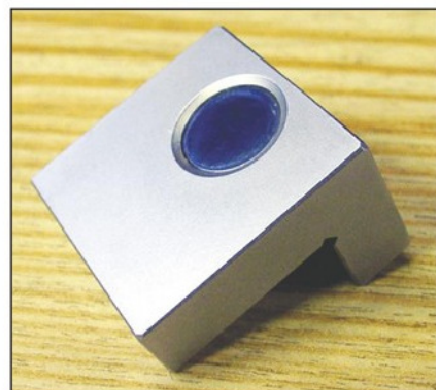
Photo 14. Detail of the edge accessory. The mirror features a fine line which is in line with the lower vertical face.
