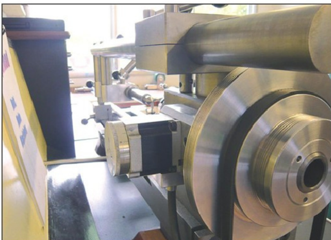
Photo 4. The stepper motor at the side of the headstock. Note the 3 step Poly Vee belt drive pulley.
