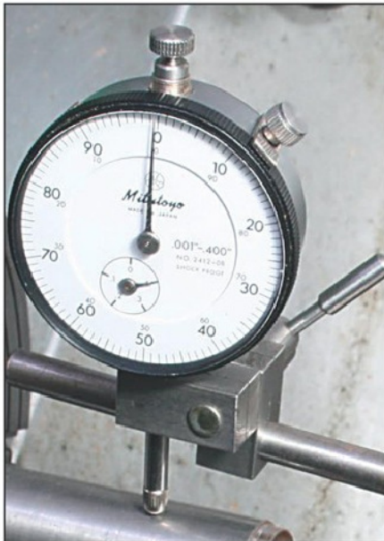
Photo 4. One half of a Swivel Joint is being used to hold a dial indicator by holding the indicator's barrel. A half joint with a larger bore will be required.
