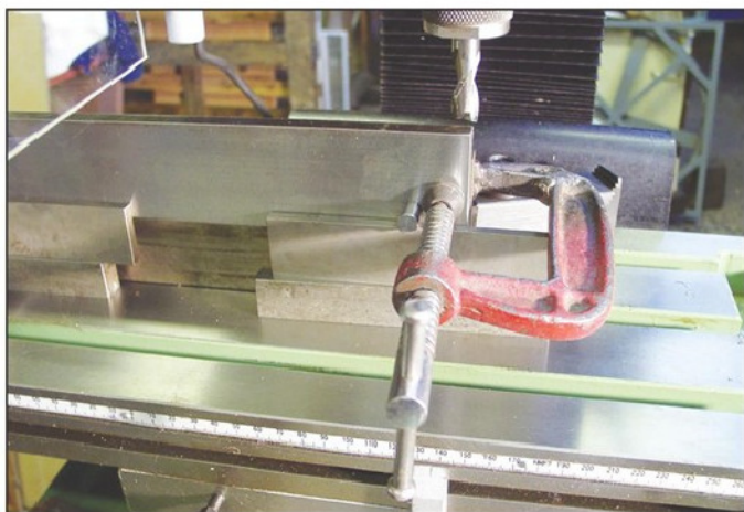
Photo 7. Edge is trued to the pins by locating pins on parallels.
