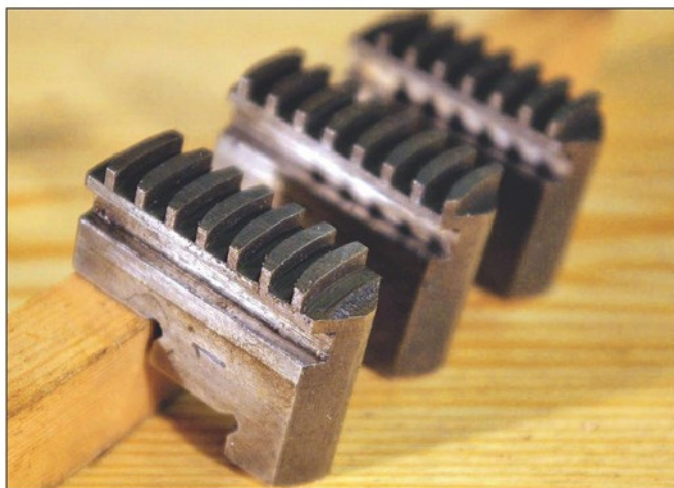
Photo 12. Jaw in the foreground has lost its innermost tooth.
