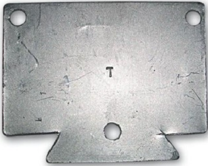
Photo 5. Template used to transfer hole positions to thrust plate.
