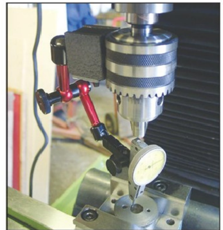
Photo 17. The chuck has been tightened to lock the outer ring, then the mag base attached. The clock can then be used to set the hole in the work concentric with the spindle.
