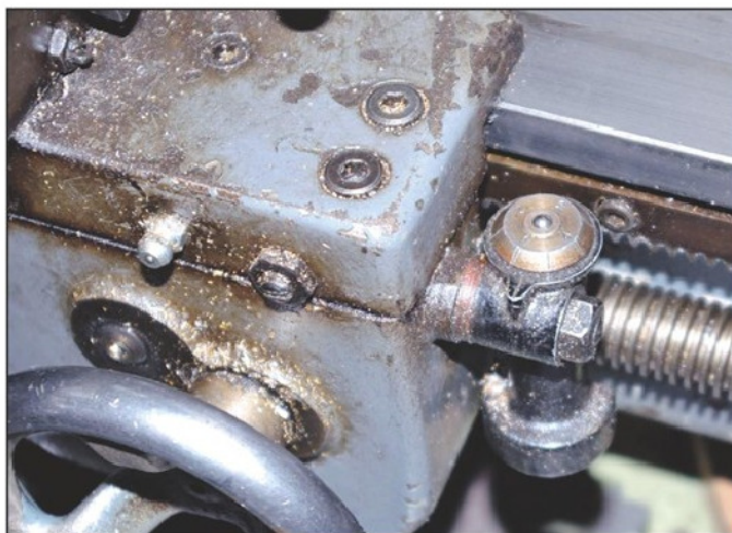
Photo 18. Threading dial indicator can be added to Myford.
