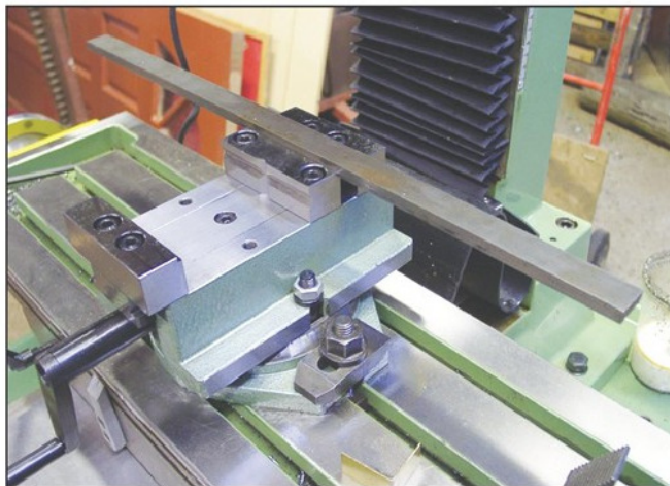
Photo 2. For approximate setting, a long straight bar may be sighted against the Tee slots.
