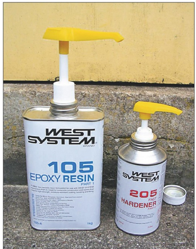
Photo 17. Epoxy resin and hardener used to make the epoxy granite.
