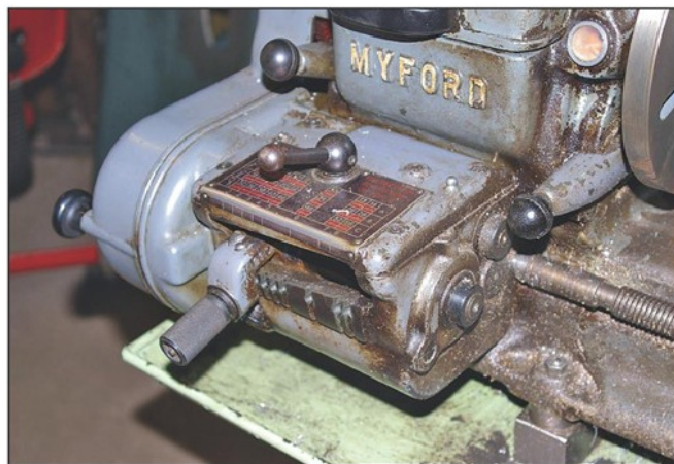
Photo 5. Quick change gearbox on Myford.
