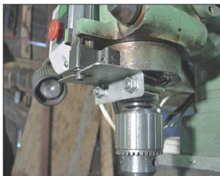
Photo 22. Detail view of spindle lock in position.
