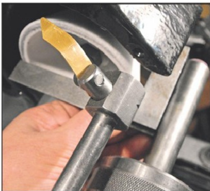
Photo 46. Checking for square.
