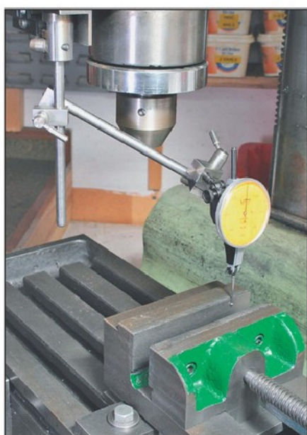
Photo 2. Mounting a DTI on the milling machine can be problematical. This method, which shows a vice being positioned, makes the process very straight forward.
