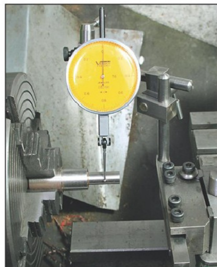
Photo 7. A simple Angle Mount is one way of mounting a DTI on the lathe.
