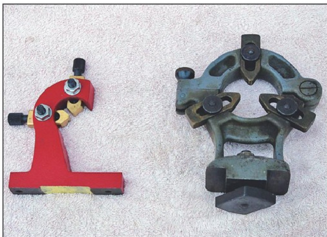
Photo 17. Travelling steady for Mini-Lathe (left) and fixed steady for Myford (right).
