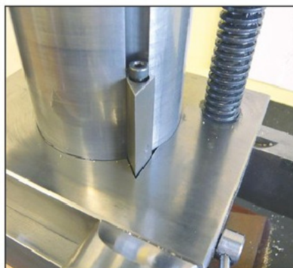
Photo 18. Triangular gib being lifted out. The top screw is unscrewed to serve as handle.
