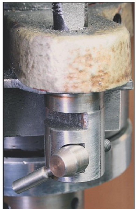
Photo 6. A close up of the Fixed Mount on the milling machine head. This is held by replacing the nut that secures the down feed stop.
