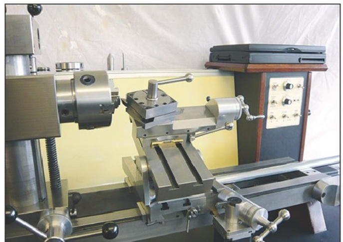
Photo 5. The headstock fully raised for large diameter turning.
