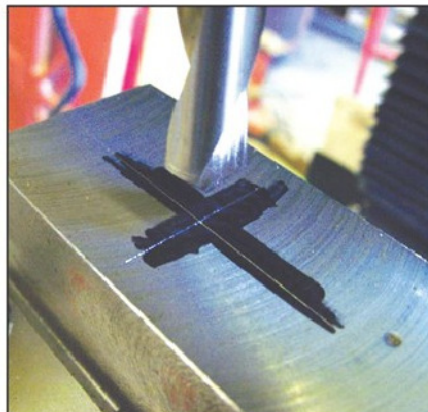
Photo 16. Using a spotting or centre drill, the spindle is rotated so that the chisel edge is aligned with one scribed line. The position can be checked with magnifying glass or by dabbing down on to the work. The spindle is then turned 90 degrees and the process repeated.
