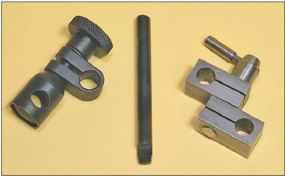
Photo 3. Commercial (left) and shop made (right) swivel joints. The bit in the centre is for producing the tapered hole in each half joint, see drawing.
