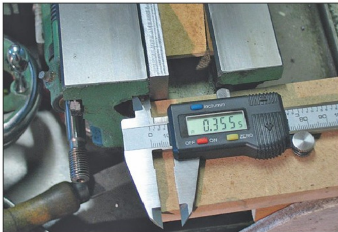
Photo 53. Measuring the depth of the front undercut of the bed.
