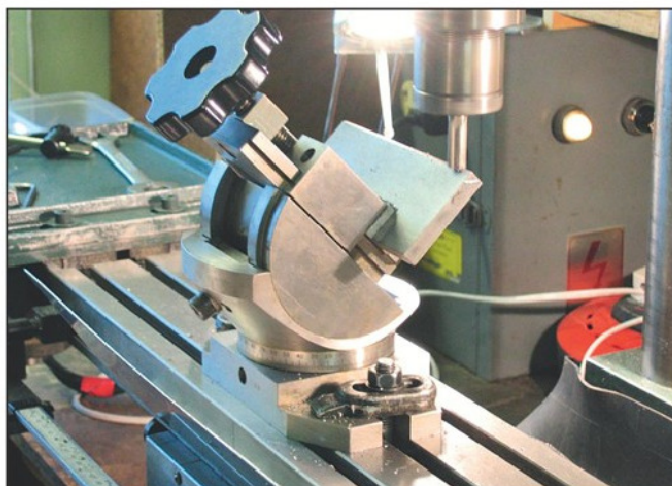
Photo 47. Chamfering the underplate.
