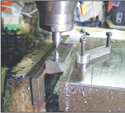
Photo 15. Here the rod blank was held by two Allen screws in the fixture clamped in the vice. Setting the datum position was achieved by means of two pointed accessories, lined up using a magnifying glass.
