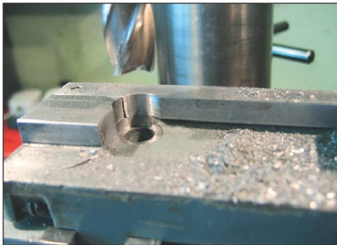
Photo 50. Counterboring the base underside for the securing bolt.
