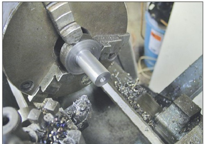
Photo 5. Rough turning extension shaft.
