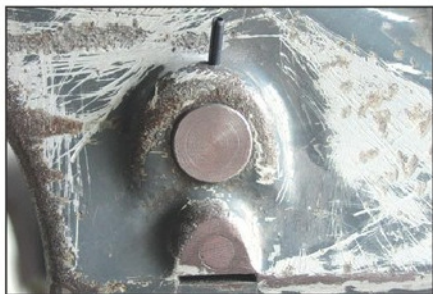
Photo 51. The spring roll pin about to be hammered into its hole.
