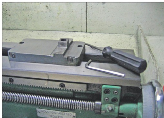
Photo 48. Checking the fit of the tailstock base to the bed shears.
