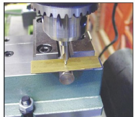
Photo 19. When the strip is level, the drill is on centre.
