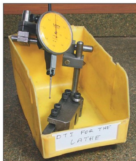
Photo 8. If you have a spare quick change holder then the set up in photo 7 can easily be retained for immediate use.
