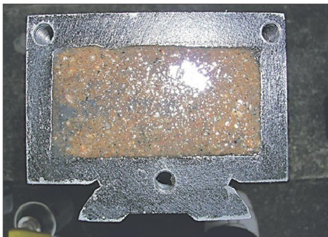
Photo 4. Holes drilled and tapped in top of X1 column. Note epoxy granite fill.
