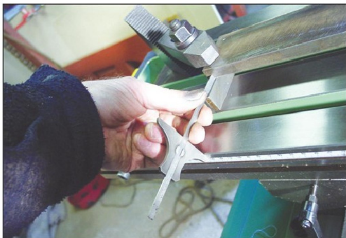
Photo 5. With care, good accuracy can be achieved using a depth gauge. The error measured here was 0.002in.
