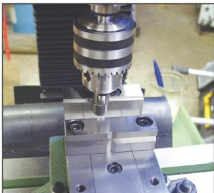
Photo 11. Lower section of edge finder has moved about 1mm to the left giving positional indication.
