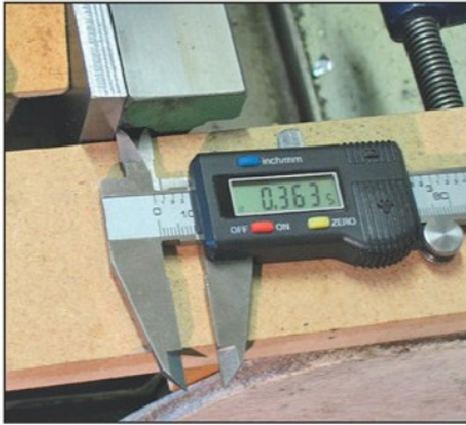
Photo 54. Measuring the depth of the rear undercut.
