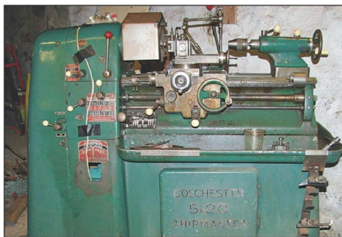
Photo 3. Colchester Chipmaster dates from the fifties and weighs in at some 500Kg.
