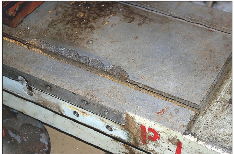
Photo 6. It's not a cross slide, it's actually part of an X-Y table, but these Tee slots show what damage can be inflicted by careless clamping and over tightening.
