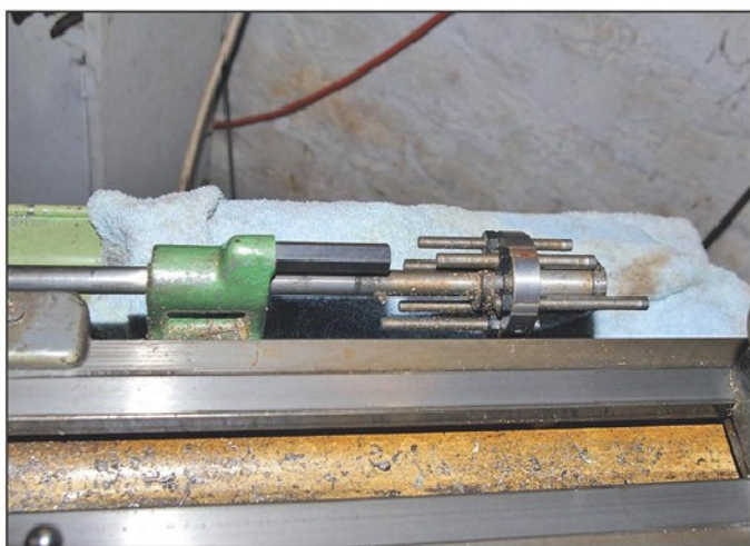
Photo 15. Myford multi position stop fits to rear of bed and is a more complex attachment.
