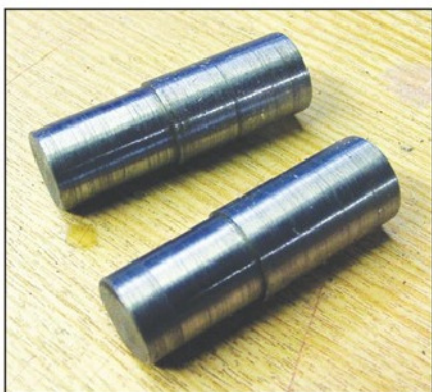
Photo 3. A pair of setting pins for the VMC mill.
