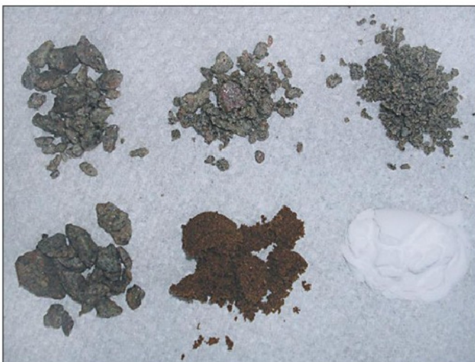
Photo 16. Aggregates used in epoxy granite.
