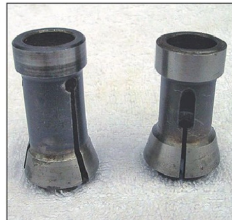
Photo 6. Correct MA99E collet (left) and modified 233 (right).
