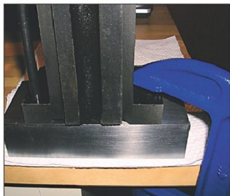
Photo 16. Transfer punching column mounting holes.
