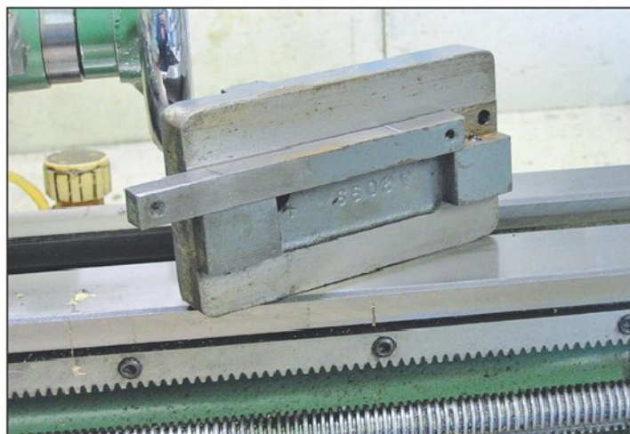
Photo 45. Underside of tailstock showing released adjustment bar.
