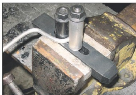
Photo 4. Makeshift bending rig for forming handle.
