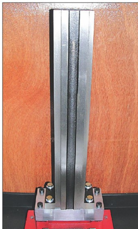
Photo 20. Fixed column on adaptor block mounted on X1 mill base.
