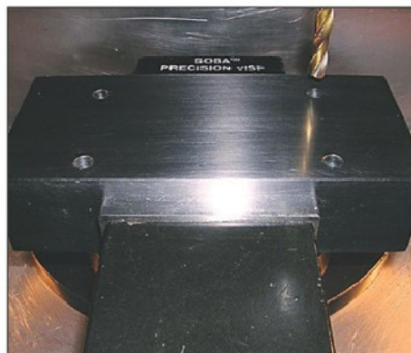
Photo 17. Column mounting holes being drilled in adaptor block.
