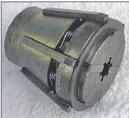
Photo 14. Detail of Multi Size collet shows the sliding blades. (In this pattern the blades project forwards flush with the face of the collet.
