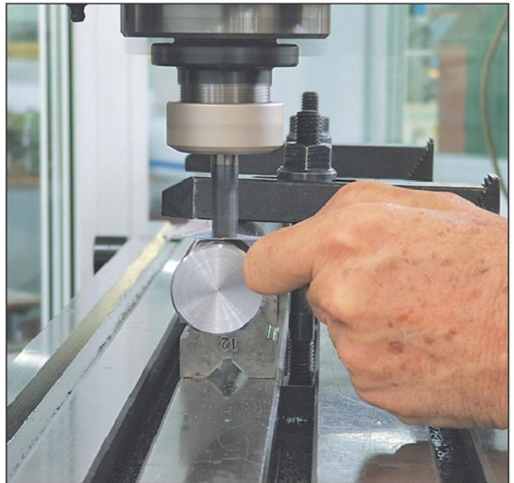
Photo 7. Setting cutter to the top of work diameter using thin paper.
