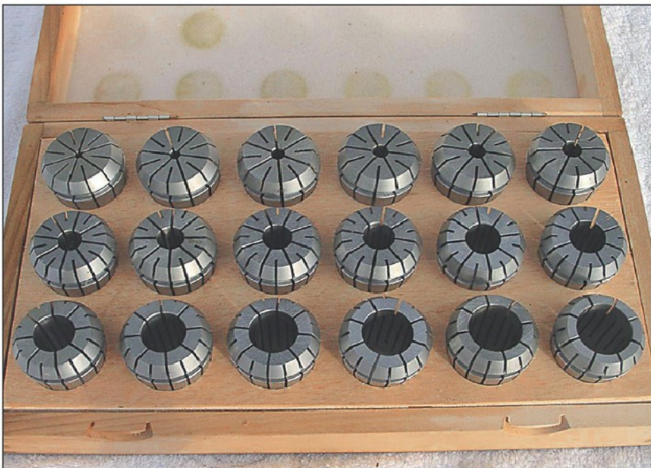
Photo 16. Eighteen ER32 collets cover diameters from 2mm to 20mm.
