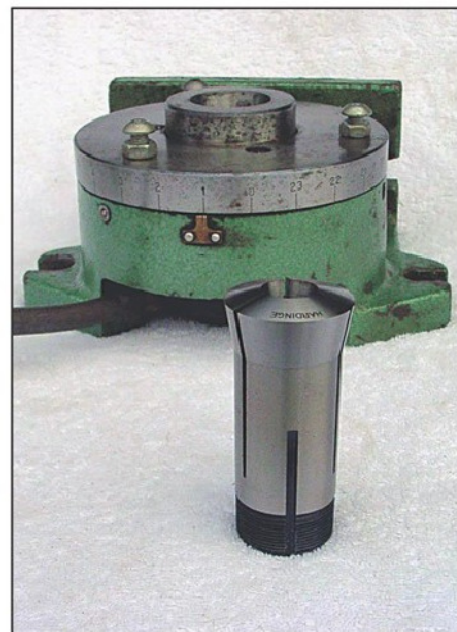
Photo 9. Foreground, a typical 5C collet, to the rear, a rapid action rotary table which accepts these collets.
