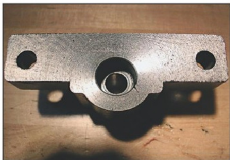
Photo 6. Inner recess of bearing block.
