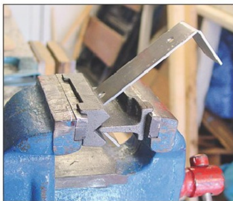
Photo 8. Bending the square part of the brackets.
