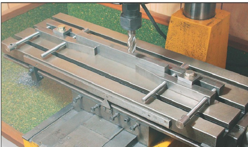
Photo 14. Requiring to reduce a one inch bar along its length to twenty-five millimetre, toolmaker's clamps made the top surface fully available for machining.
