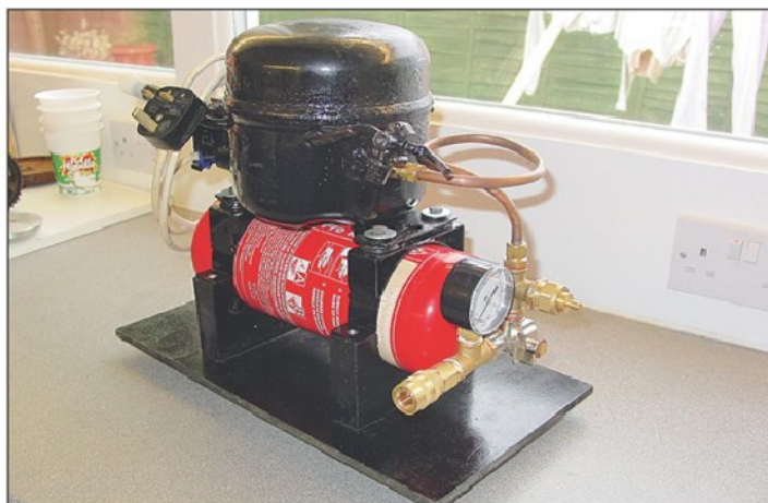
Photo 12. The complete compressor, assembled and ready to run.
