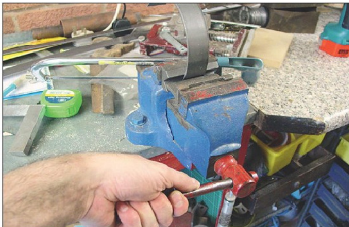
Photo 5. Bending the end of the mounting bracket.
