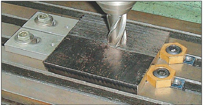
Photo 17. Two clamps being used to hold a piece of black iron whilst it is being reduced to the thickness required. The clamps are always used with fixed opposing jaws.
