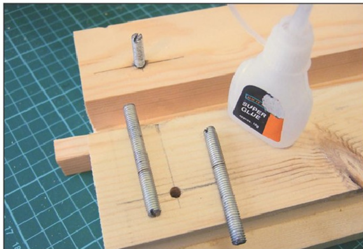
Photo 40. The 5mm studding is screwed into the frame to retain the X mountings. The studding has a saw cut to enable them to be screwed into place. Cyano glue is optional.
