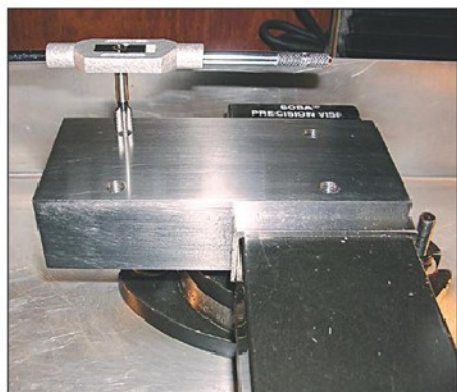
Photo 18. Column mounting holes being tapped.
