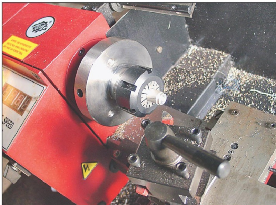
Photo 18. Typical ER32 chuck fitted to Mini Lathe.
