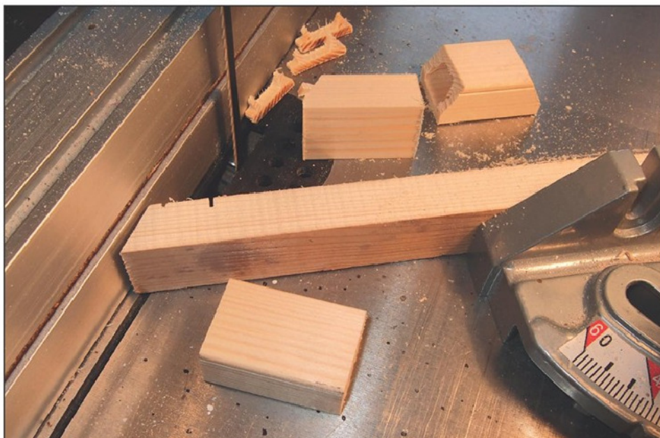
Photo 44. Cutting the wooden trunking to make the cable tracks.
