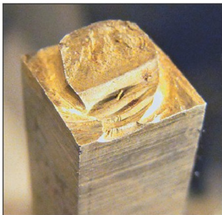
Photo 26. Cutting up HSS tool bits.
