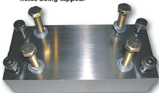
Photo 19. Column adaptor block showing screw fixings.
