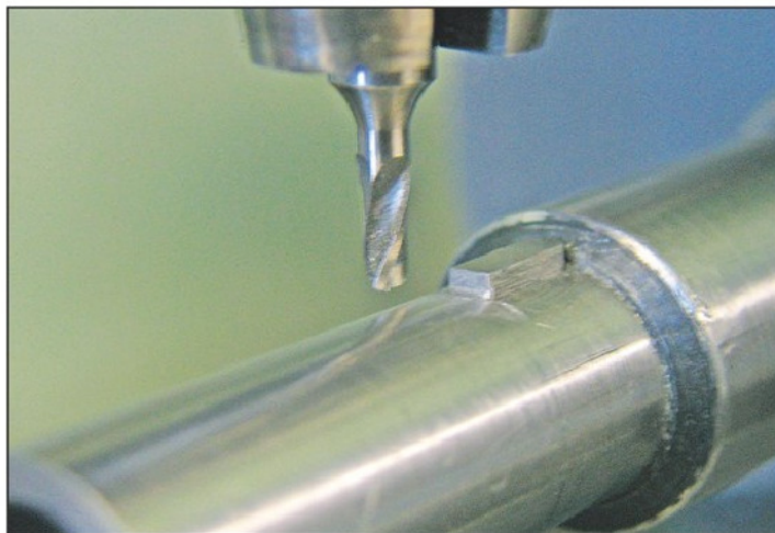
Photo 34. Machining the end of the key.
