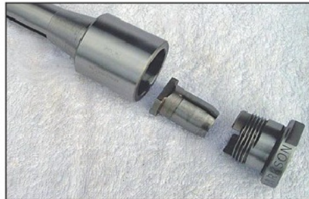
Photo 11. Left to right, body, collet and closing ring for Clarkson system.
