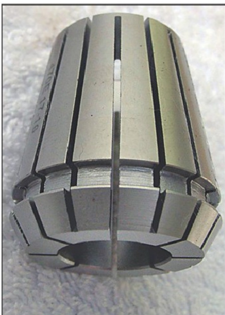
Photo 17. Detail view of ER32 collet shows the slots which run from alternate ends, permitting parallel collapse over 1mm range.
