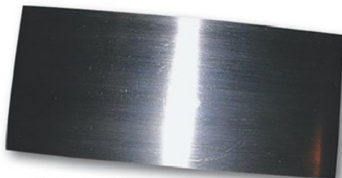
Photo 15. Column adaptor block milled to size.
