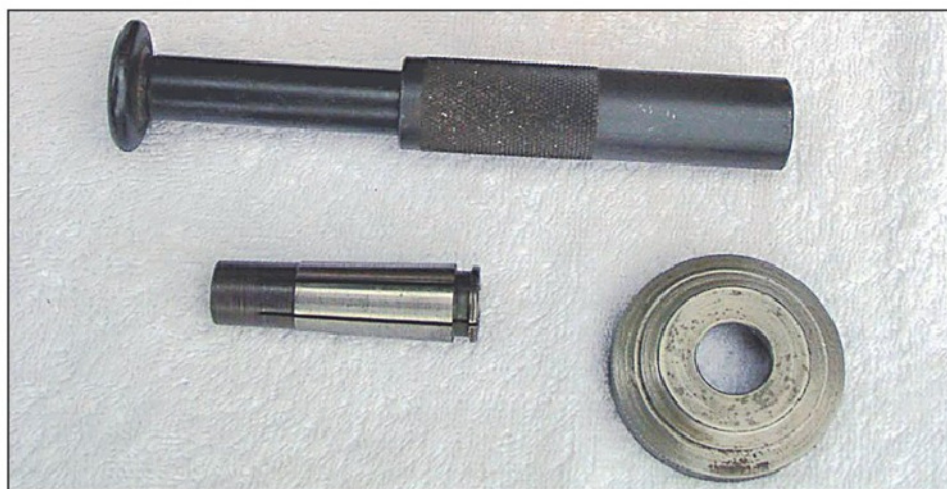
Photo 1. Collet, closing ring, and installation tool for Myford patent collet.
