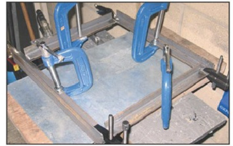
Photo 8. Second frame side members clamped to first for tack welding.
