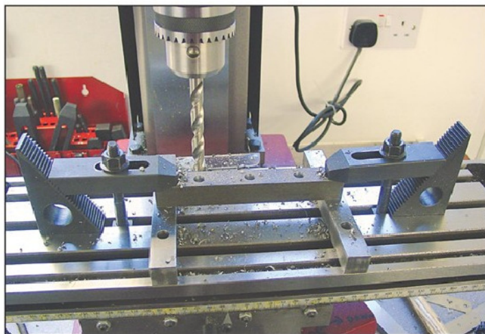
Photo 2. Drilling the three holes.
