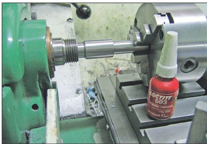
Photo 32. Arbor inserted and secured with Loctite 603.
