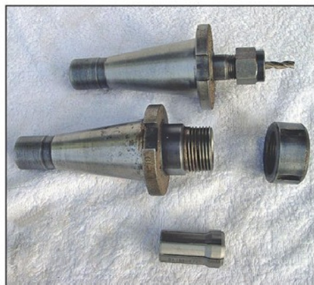
Photo 19. Two double angle collet chucks and a typical collet.
