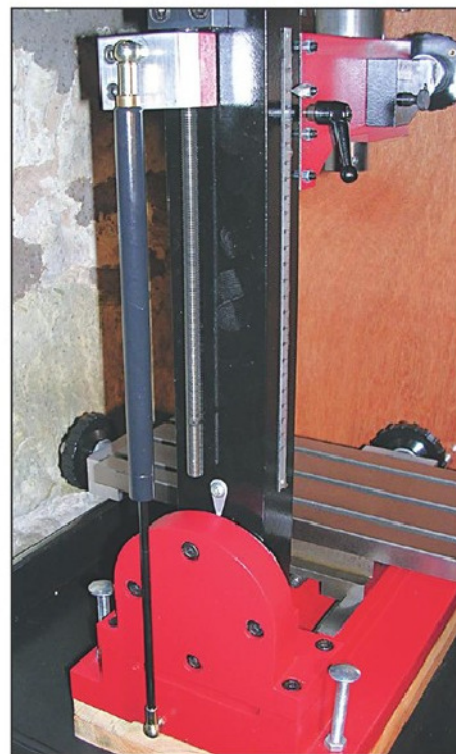
Photo 24. Gas strut fitted behind column of X1 mill.
