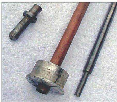
Photo 8. The elements of an adapter to handle 3mm material in a half inch collet. Bottom - slotted adapter, middle - guide tube, top - pusher bar.
