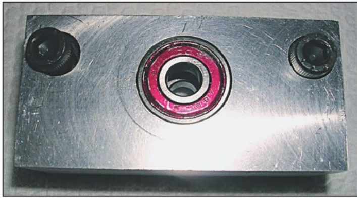
Photo 9. Front view of completed new ball bearing block.
