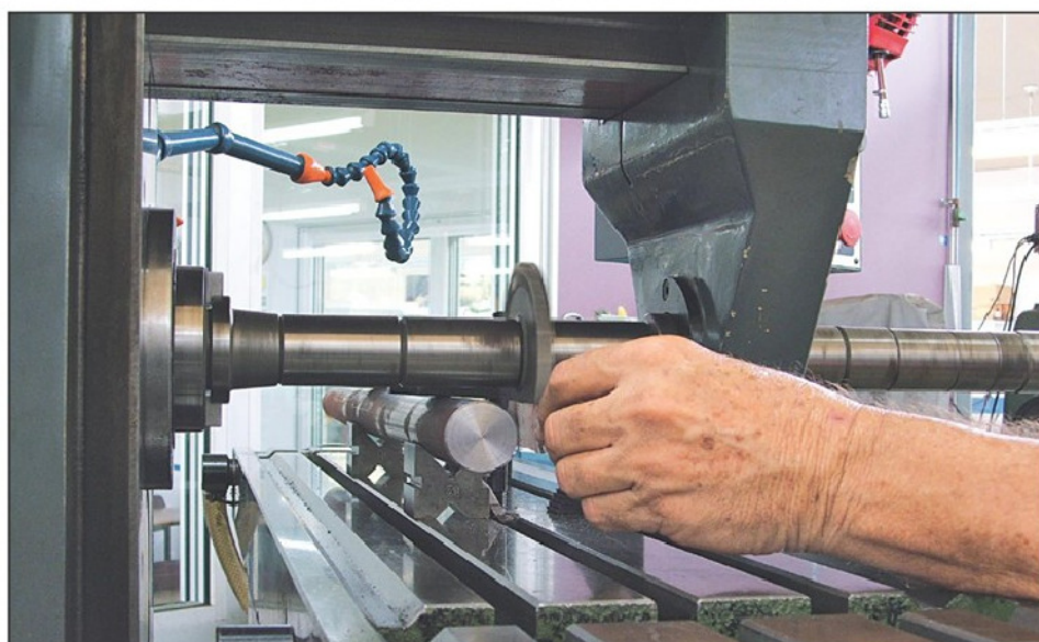
Photo 3. "Picking up" the diameter of bright round bar with paper and revolving side and face cutter.
