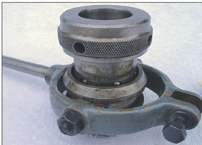
Photo 4. Dead length collet chuck for Myford, shown nose down, with the actuating balls visible.
