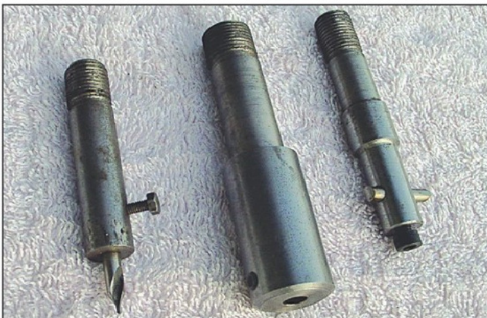
Photo 12. Three adapters made to fit Clarkson collets; left centre drill, middle FC3 holder, right fly cutter.
