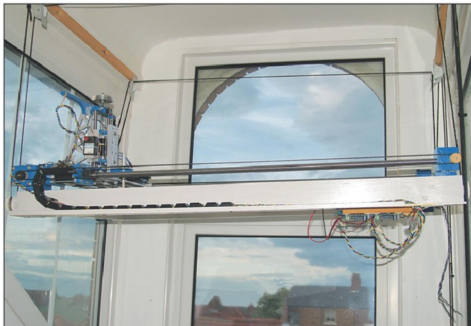
Photo 38. The router in the raised position. The electronic board is on the right.
