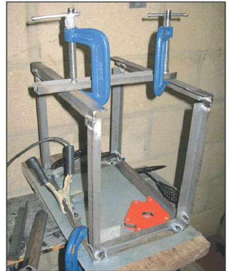
Photo 9. Clamping frame sides for welding in 200mm side members.
