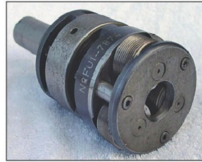
Photo 11. Fette FU1 thread rolling head caters for diameters from 6 to 10mm.
