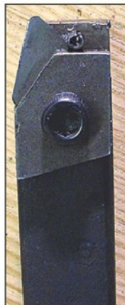
Photo 5. Plan view of tool shows corner radius and edge angle.
