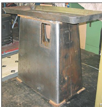
Photo 6. The stand has been completely rubbed down and is ready for priming.
