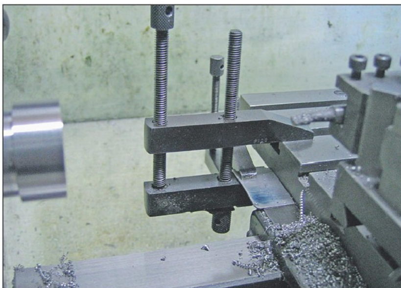
Photo 13. As photo 12 with swarf deflector added.
