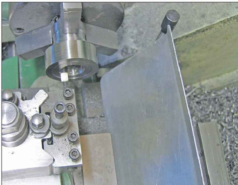
Photo 14. Cross slide stop with swarf sweeper clamped to first clamp.
