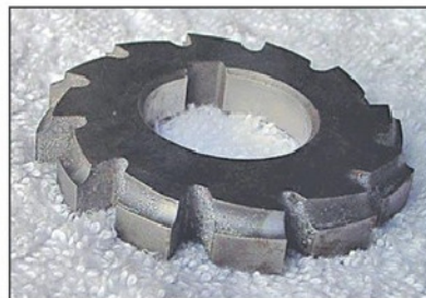
Photo 14. Milling cutter for external radius.
