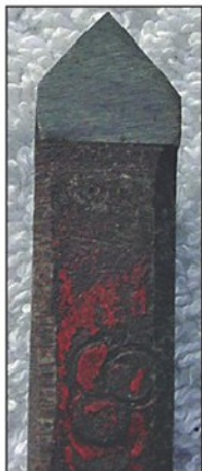
Photo 4. In production both edges might be engaged to simultaneously chamfer successive workpieces.
