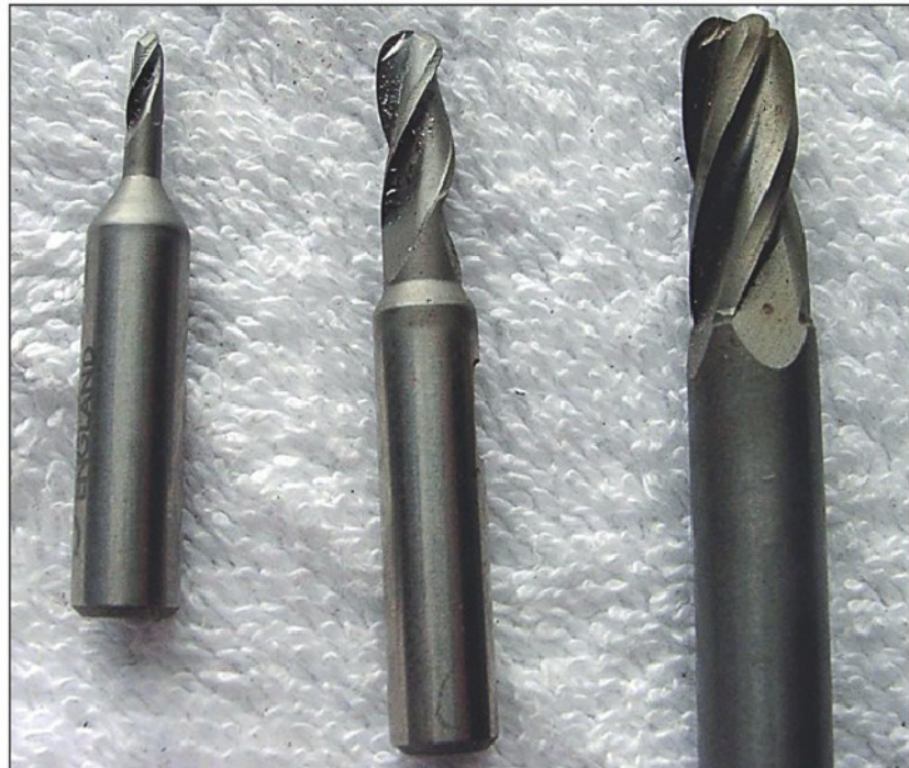
Photo 13. Ball nose/internal radius cutters.
