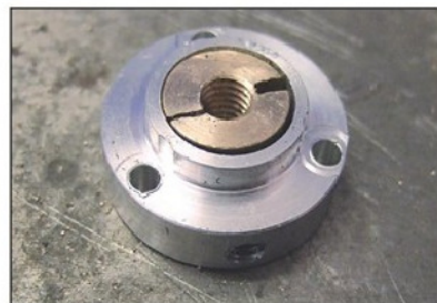
Photo 11. The drive nut mount is drilled for three retaining screws.
