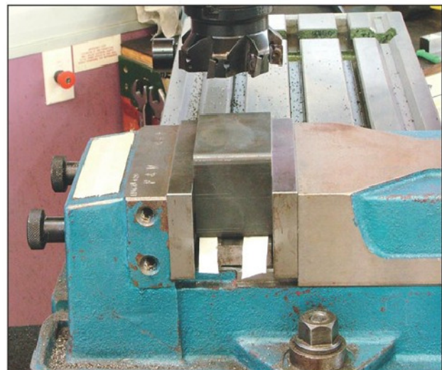
Photo 6. Two cigarette papers under both ends of work.
