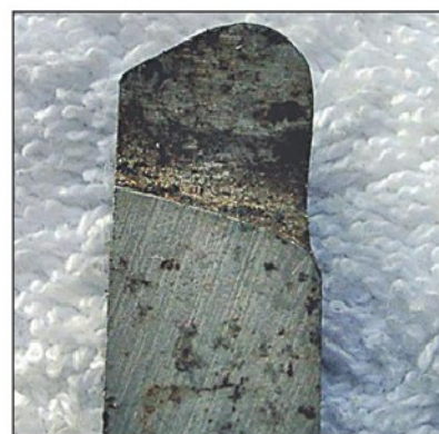
Photo 1. Form tool for fillet radius.
