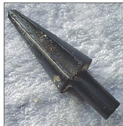
Photo 9. Although intended for opening up holes in car bodywork, this cutter will produce tapered holes though not in thick material.
