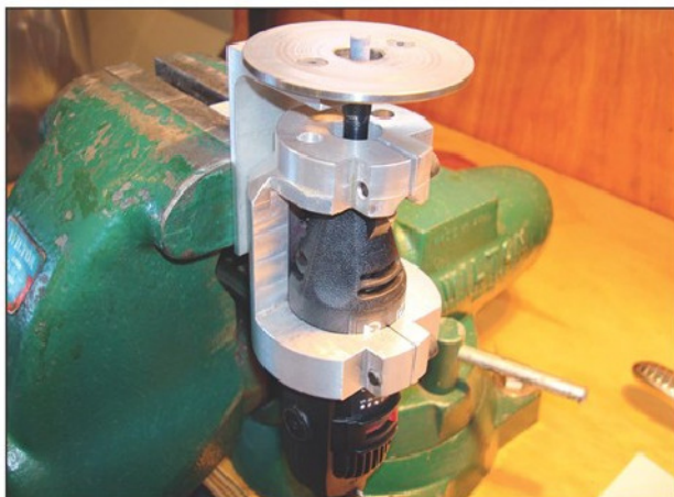
Photo 6. The grinder mounted in the vice.
