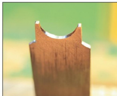
Photo 10. A cutter after sharpening.
