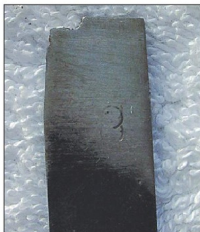
Photo 8. Home made form tool in gauge plate.
