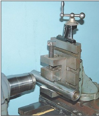
Photo 11. Milling the new keyway.
