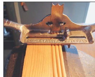
Photo 11. Reeds cut with the new homemade cutter.
