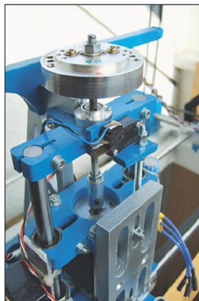
Photo 15. The anti "squeal" device is shown fitted here together with the Z homing micro switch and the long motor mounting screw used as a trigger.
