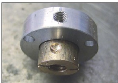
Photo 12. The mount has been drilled and tapped m4 and the drive nut has been shallow drilled for alignment as well as split for anti-backlash purposes. It has been slid out of position in the photo for clarity.
