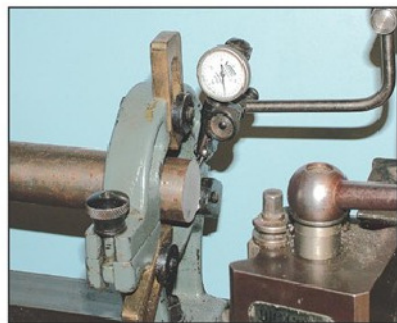
Photo 2. Clocking the end of the bar.
