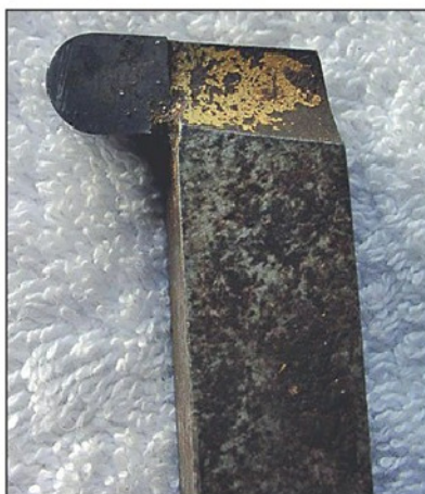
Photo 7. Tipped tool to work on end face.
