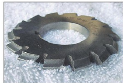
Photo 15. Typical involute gear cutter.
