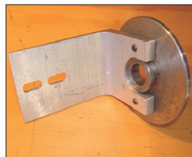
Photo 5. The aluminium bracket with the round table.
