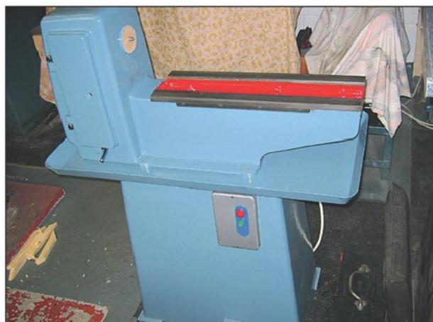
Photo 8. The stand and main casting have been reunited.
