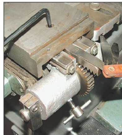
Photo 7. Adjustment of MK2 rack and pinion.
