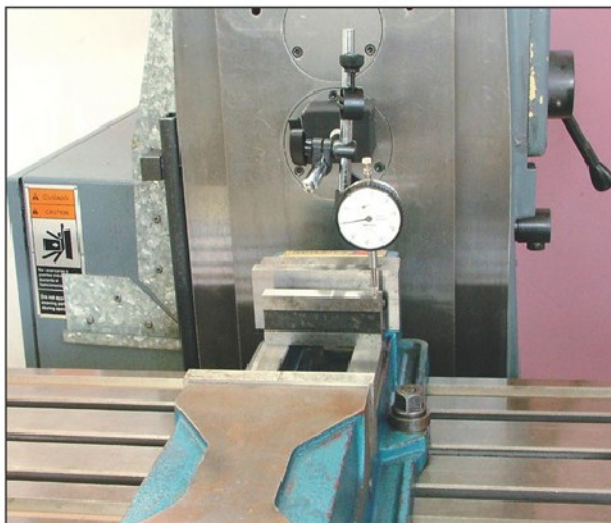
Photo 2. Check vice base over width.
