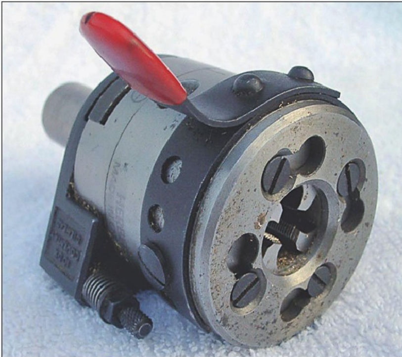
Photo 10. A typical Coventry die head, this one a \frac{3}{4} in. size.
