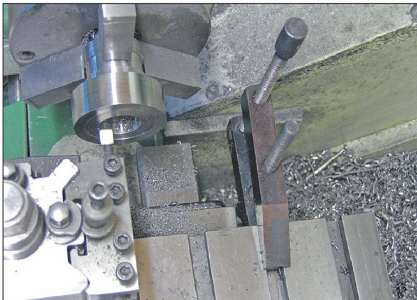
Photo 12. Top view of rear cross slide stop used for boring.
