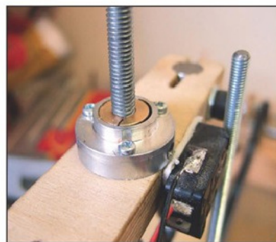
Photo 13. The completed drive nut assembly.
