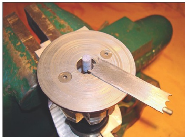
Photo 9. Grinding a cutter by hand.
