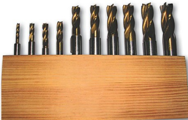
Photo 13. TiN coated HSS 4-flute end mills.
