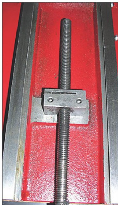
Photo 10. Y axis leadscrew and nut.
