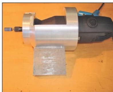
Photo 4. The pillar grinder mounted for use as a toolpost grinder.
