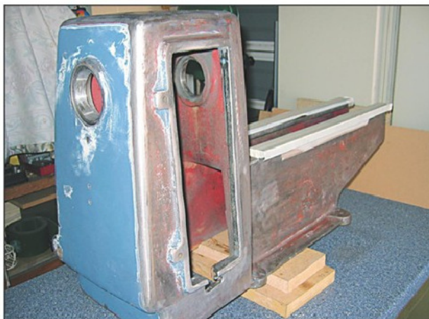
Photo 4. The main casting is taken down to bare metal...
