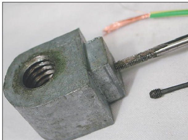
Photo 4. Fitting the grub screw.
