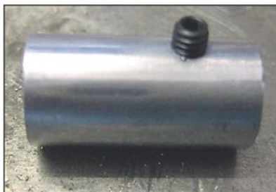
Photo 10. The stepper shaft adaptor; don't forget to put a flat on the stepper shaft to take the grub screw.
