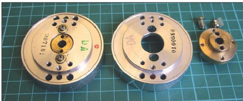
Photo 14. The anti "squeal" device. Note the slightly enlarged holes just off centre and the silicone tubing on the assembly screws. Use thread lock on the assembly screws.
