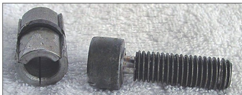
Photo 3. Allen screw with two grooves and the home made collet.
