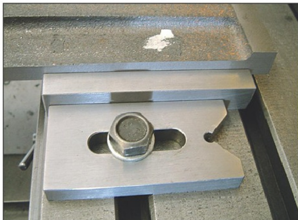
Photo 16. A stop piece set square across the table with a packing block to align the next edge at right angles for finishing.
