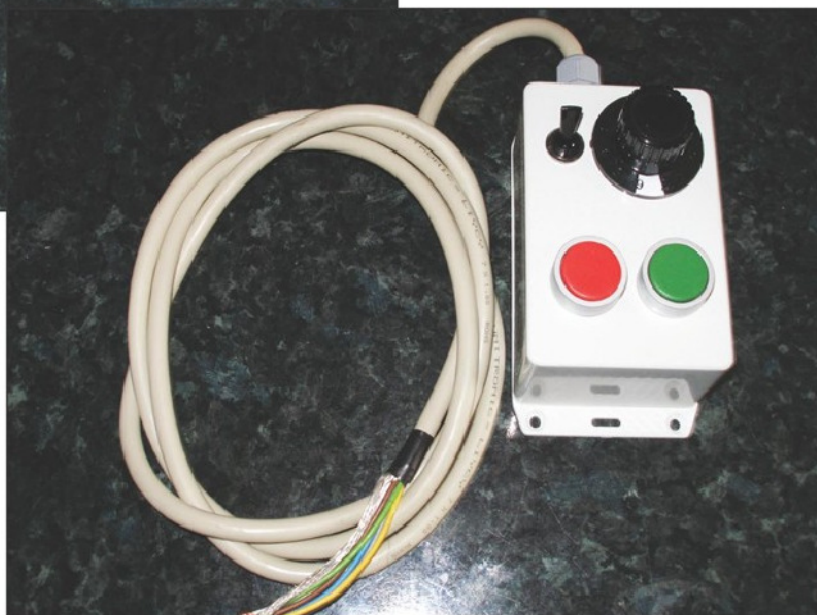
Photo 2. The control pendant.
