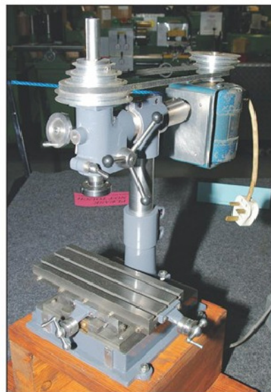
Photo 4. 6 inch scale Dore Westbury Mill.
