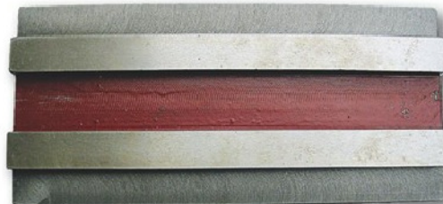
Photo 4. The underside of the mill table. Note the just about adequate finish on the sliding surfaces.
