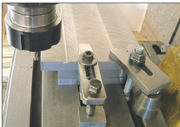
Photo 19. Extra clamp fitted prior to forming the start of the rip fence slot.
