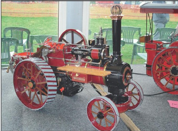
Photo 10. 1 1/2 inch scale Allchin Royal Chester traction engine.
