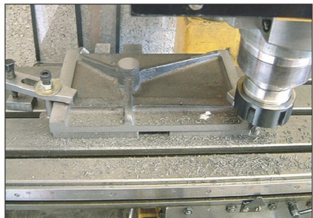
Photo 15. The rib set parallel to the mill table to finish the front edge.
