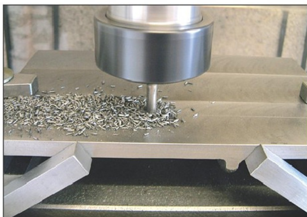
Photo 18. Stop blocks, a close fit in the front T slot to align the work for forming the cross-cutting fence slot.
