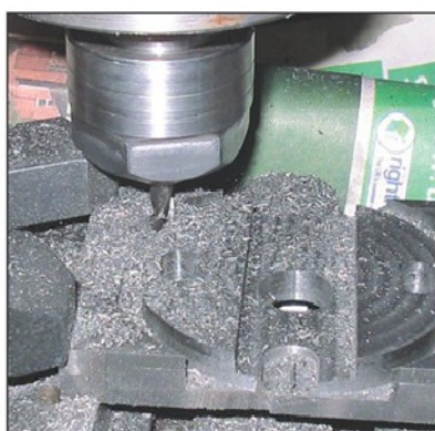
Photo 37. CNC machining the Vee block back plate on Dore Westbury CNC mill.
