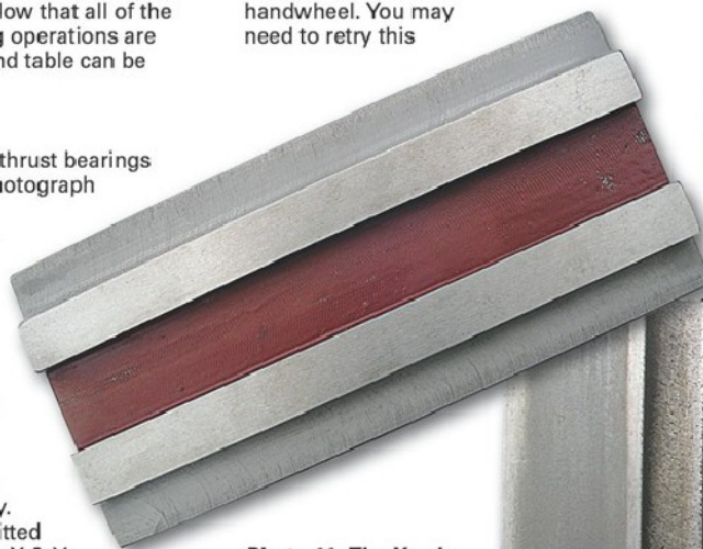
Photo 11. The X axis sliding surfaces of the X0 compound table after lapping.
