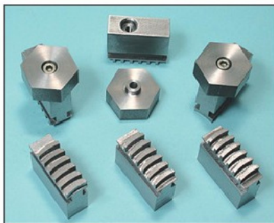
Photo 12. Two sets of shop made jaws, one having been adapted for fitting hexagonal jaws.
