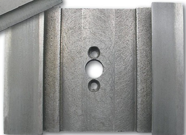
Photo 11. The X axis sliding surfaces of the X0 compound table after lapping.
