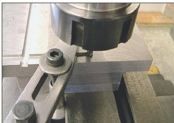
Photo 21. The main clamp replaced after cutting up to the temporary clamp.
