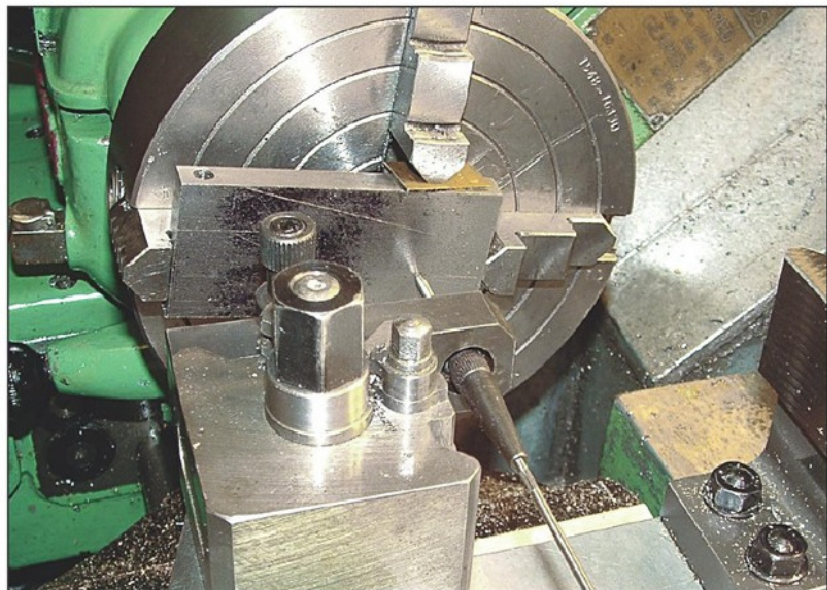
Photograph 6: Dixon tool holder form of the Centring Tool in use.
