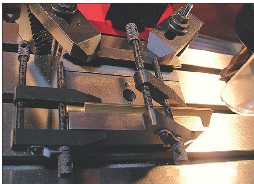
Photo 6. The brass gib strip is clamped to the saddle of the X0 compound table ready to square off the end.
