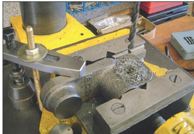
Photo 9. Drilling the cotter hole with a clamp to prevent lifting.
