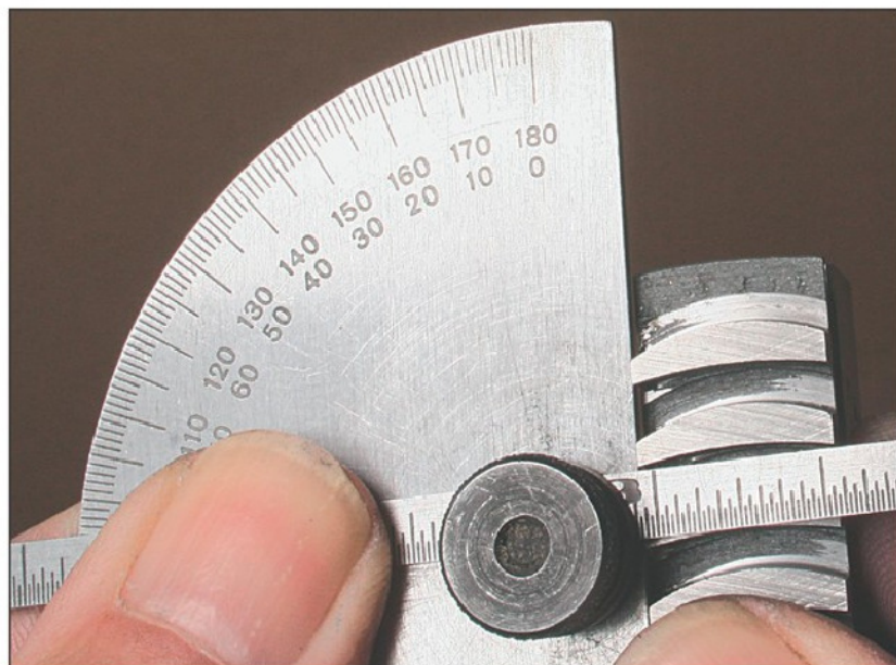
Photo 9. Measuring the angle across the tips of the jaw teeth.
