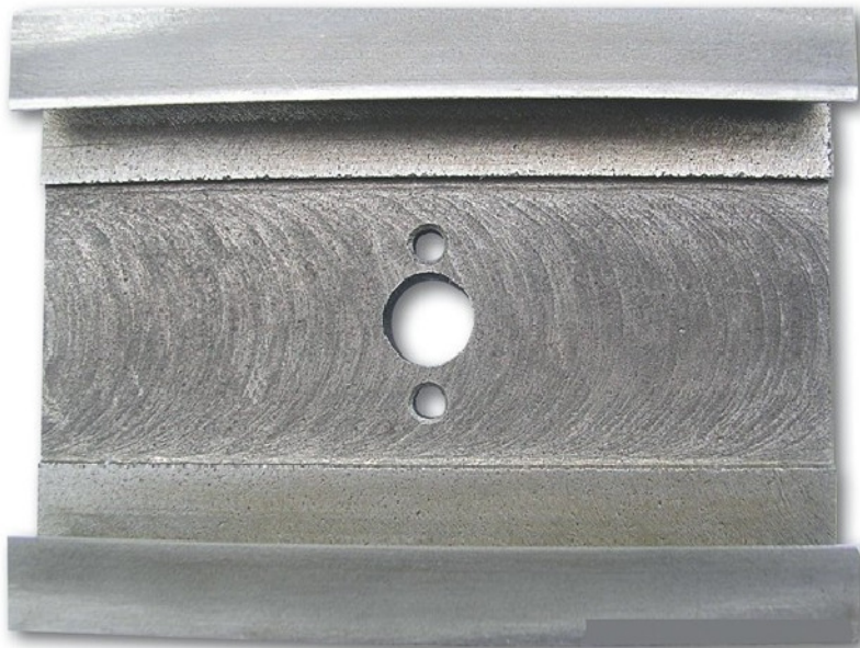
Photo 10. The Y axis sliding surfaces of the X0 saddle after lapping. Note the distinctive grey surface indicating metal has been lapped away.
