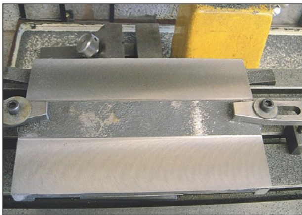
Photo 12. The table having had the outer faces fly-cut.
