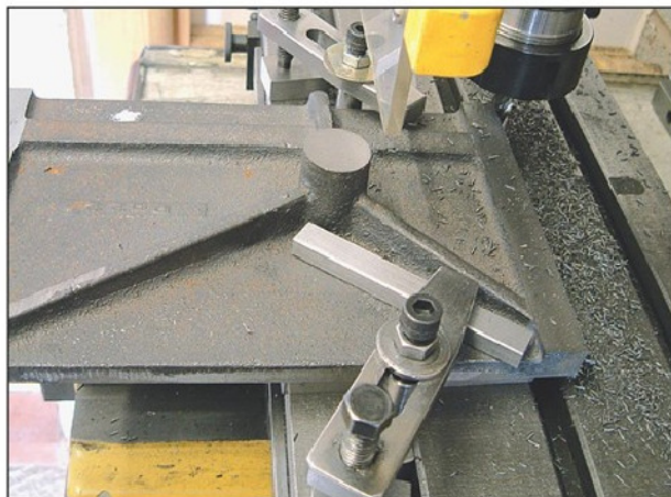
Photo 17. Cutting taking place at the rear due to space restrictions of the Y feed.
