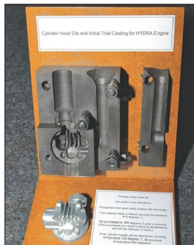
Photo 5. Metal dies for Hydra castings.
