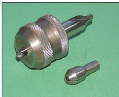
Photo 11. Cutting the nose cone taper with a no 5 centre drill.
