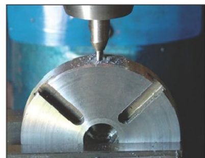
Photo 6. Drilling the tommy bar holes.
