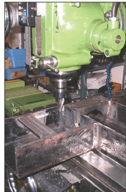
Photo 9. Machining the underside.
