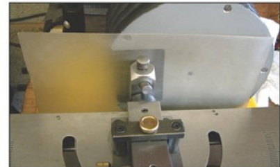
Photo 27. Plastic film used to keep the dust at bay.
