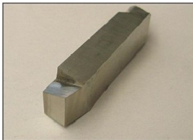
Photo 7. Finished tool awaiting the honing of the tip radius.
