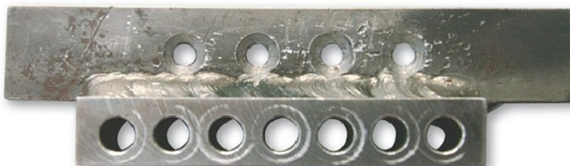
Photo 1. The drilling jig.
