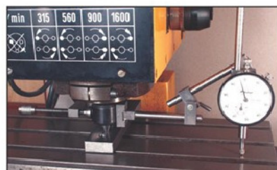
Photo 5. A set up that enables small adjustments to the angle of the tilting head to be made using the table traverse.
