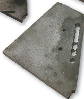
Photo 9. The finish drilled slot.
