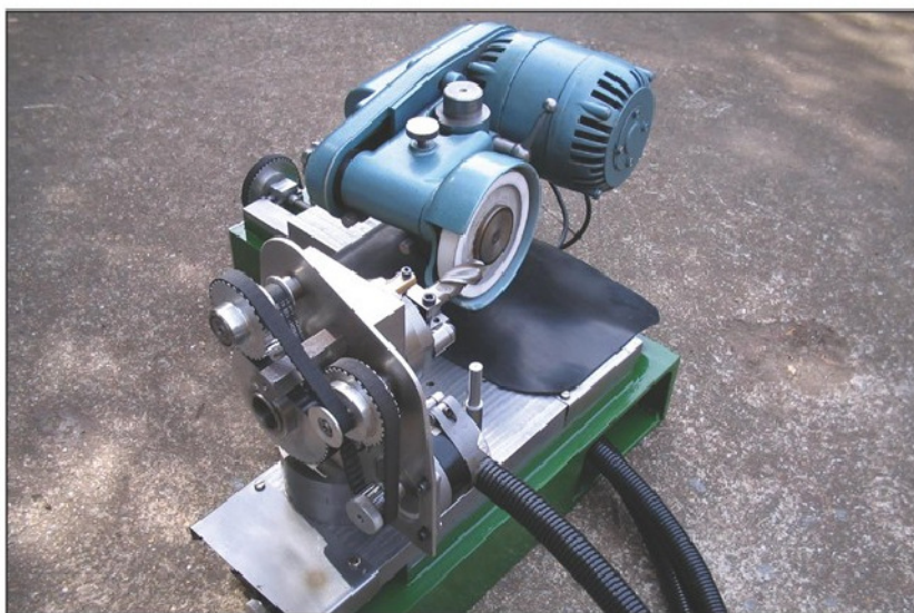
Photo 2. View from rear showing timing belt pulleys.
