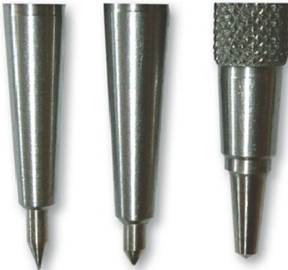
Photo 30. Selection of punches with inserted HSS points.
