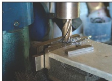
Photo 9. Making the tee nuts.
