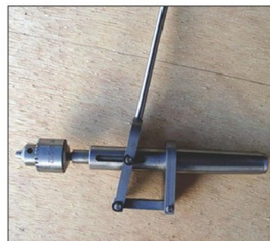
Photo 1. Sensitive drilling attachment as supplied by Myford.
