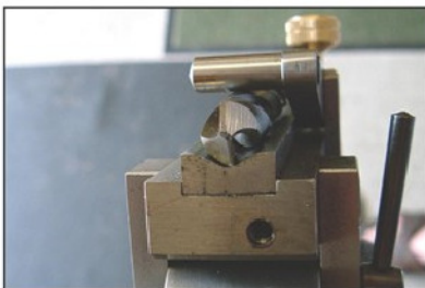
Photo 17. The first lip set for grinding.
