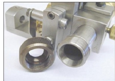
Photo 29. Small (Cowells) collets used for tool holding.
