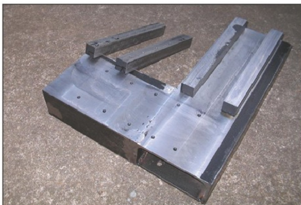
Photo 11. Fitting the blanks for the dovetails.
