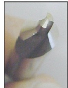
Photo 16. A re-sharpened centre drill.
