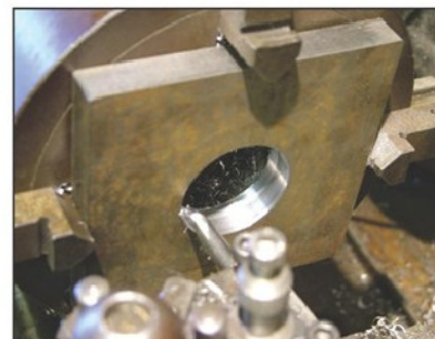
Photo 2. Boring the baseplate.
