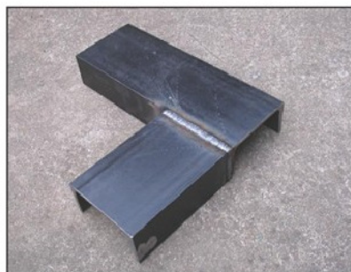
Photo 6. Two base channels welded together.
