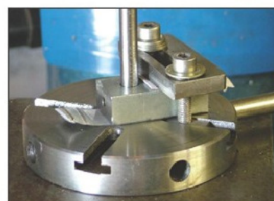
Photo 11. Setting up a link for milling.
