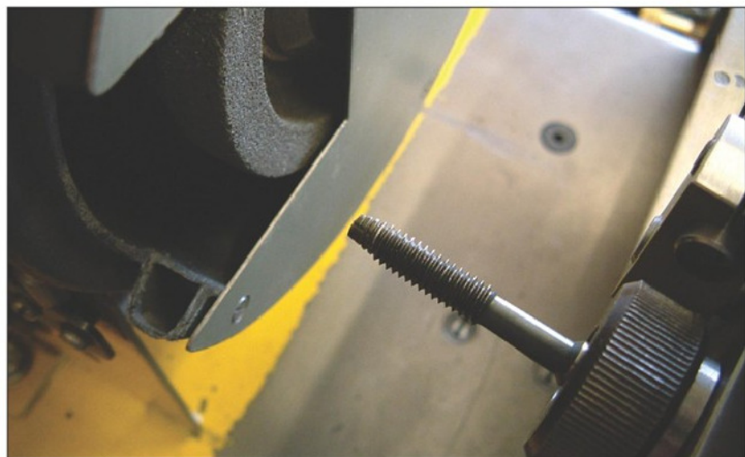
Photo 31. A tap held in a collet for sharpening.
