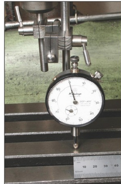
Photo 4. Checking if the table's surface is parallel with the dovetails on which it moves. Again the error should be no more than 0.025mm over 300mm.
