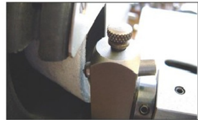
Photo 26. The holder automatically presents the diamond in the optimum position.
