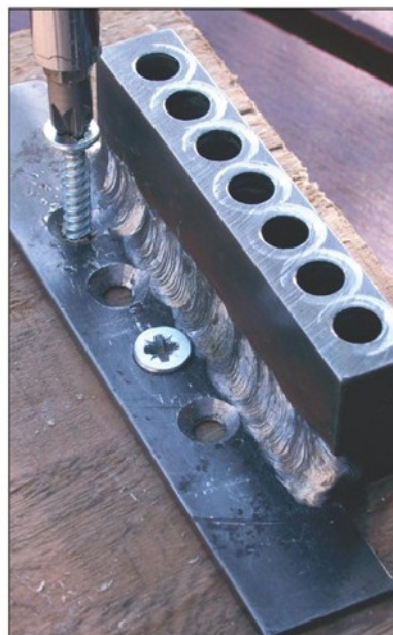
Photo 2. Screwing the jig down.
