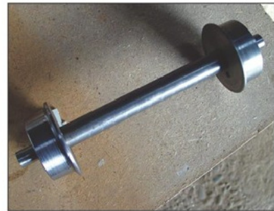
Photo 21. Wheel set showing tyre profile.
