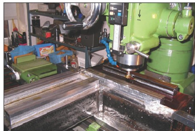
Photo 12. Machining the dovetails.
