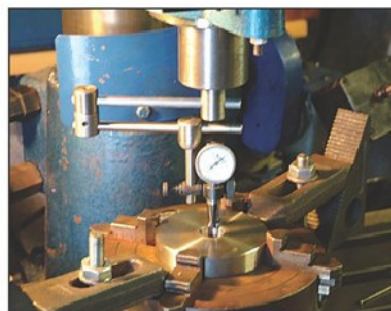
Photo 3. Clocking the top of the rotary table true.
