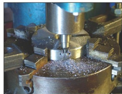
Photo 4. Milling the slots.
