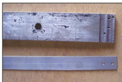
Photo 14. Drilling/milling operations were completed before sawing off the small parts.
