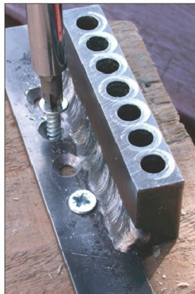
Photo 5. Screwing down using the offset holes.
