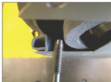
Photo 34. The first pass should only touch the rear of the threads.
