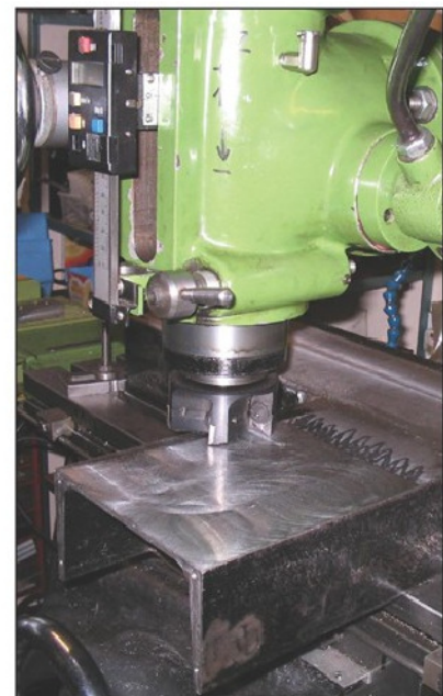
Photo 10. Machining the top surface.
