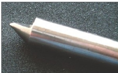
Photo 40. A half centre produced from \frac{1}{2} dia. HSS (should wear well).
