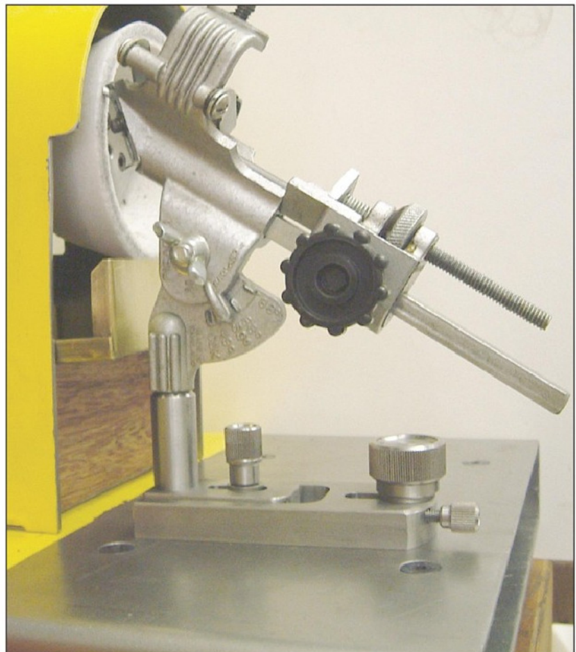
Photo 19. A commercial drill jig is easily fitted to the Worden.
