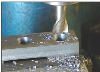
Photo 8. Counterboring the mount.
