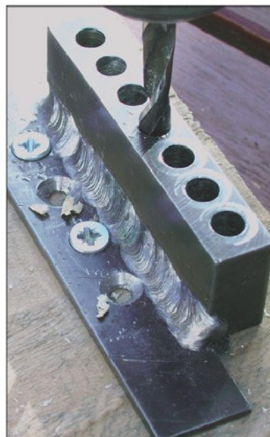
Photo 3. Drilling the first holes.
