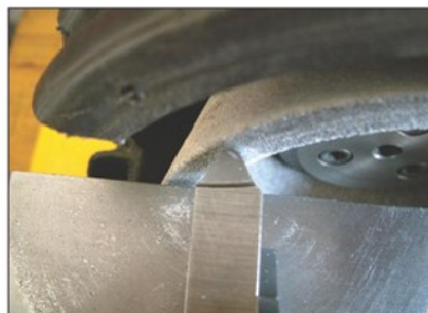
Photo 24. Ensuring that the tool remains on the vertical centreline as it is swung.
