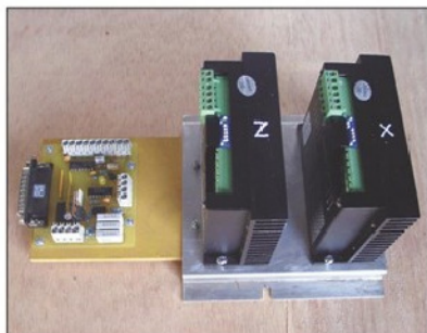
Photo 11. Sub assembly of interface and Arc stepper drivers.
