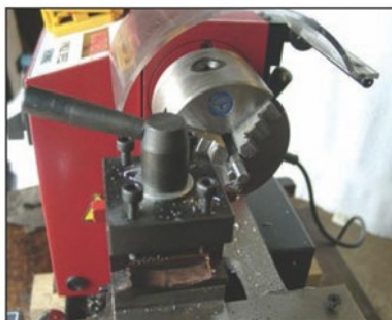
Photo 4. Turning down the stand offs ready for threading.
