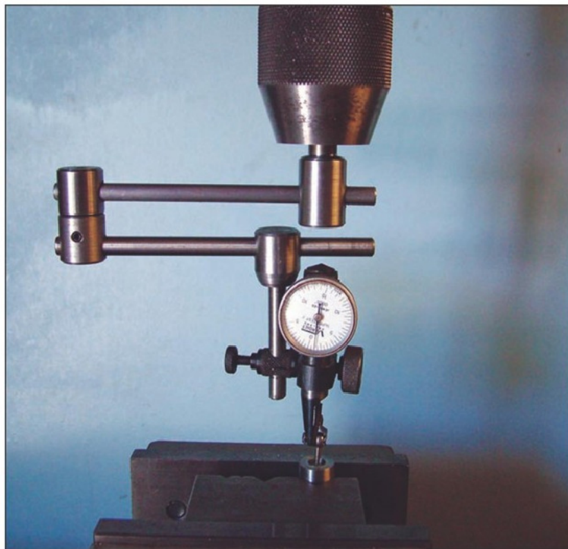
Photo 2. Clocking a small hole.
