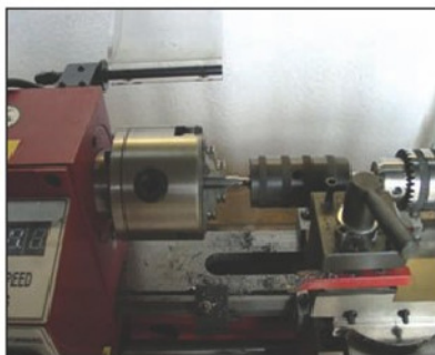
Photo 5. Threading using a tailstock guided die holder.
