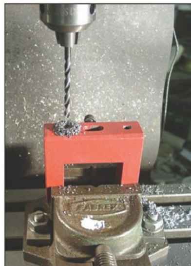
Photo 7. Drilling hole for second stand off.
