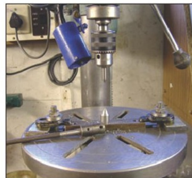
Photo 2. An alternative setup for drilling the cross holes.
