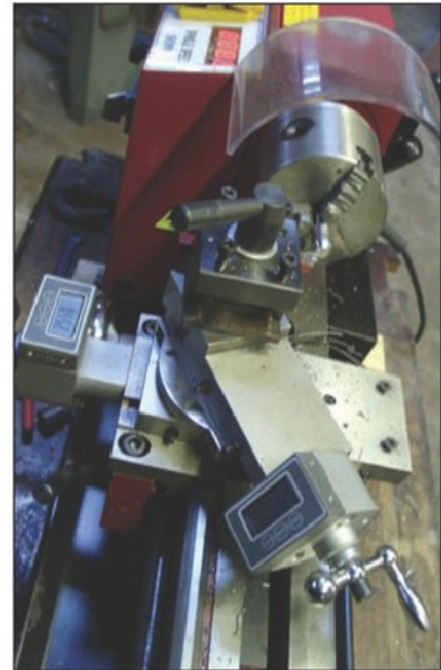
Photo 17. Set up for turning the 60 degree point.
