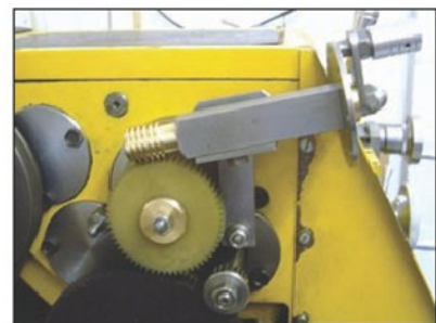
Photo 13. Clearance is minimal when using the 60 tooth wheel.
