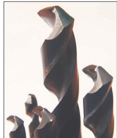
Photo 19. Split point geometry drills are becoming more available but are too complex for sharpening in the average home workshop.
