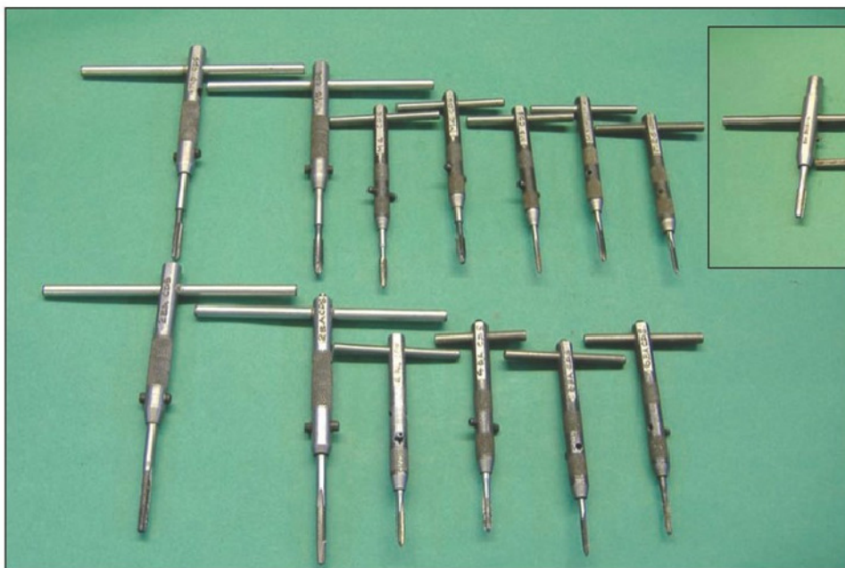
Photo 3. The finished tap wrenches all engraved ready for use.
