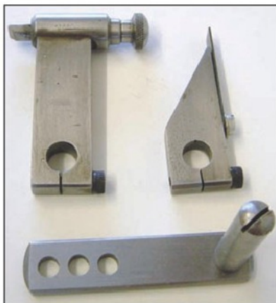
Photo 6. Indexing components using a spring plunger.
