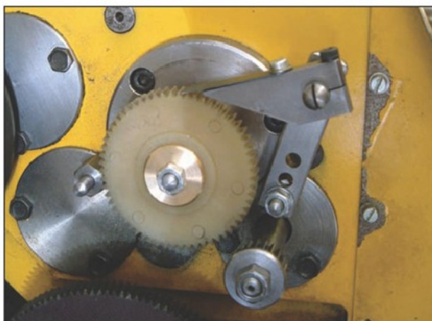
Photo 8. The simple direct indexing setup.
