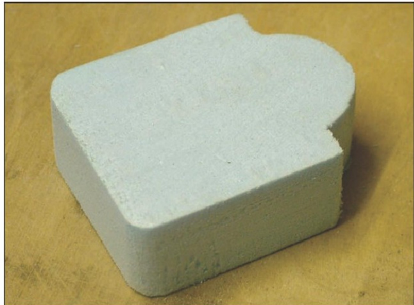
Photo 1. A simple sacrificial styrofoam pattern.
