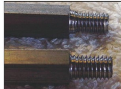
Photo 6. Upper component threaded using die normally, lower has second operation with die reversed taking thread closer to shoulder.
