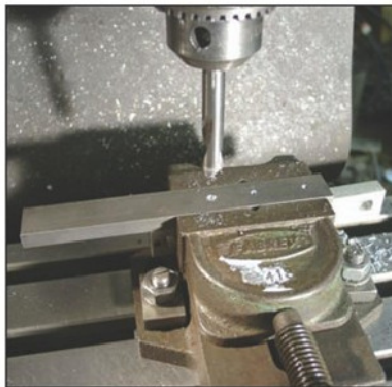
Photo 3. Spotting the hole positions on the bridge.
