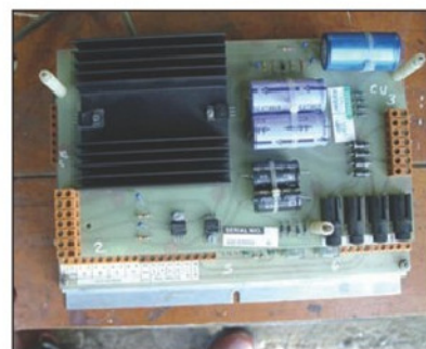
Photo 5. The regulator board.
