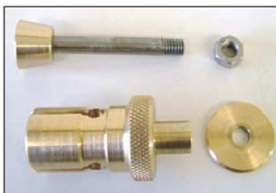
Photo 7. The headstock mandrel adaptor.
