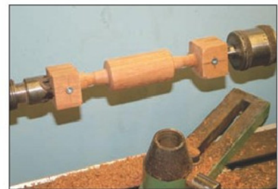
Photo 4. Turning the wooden pattern with dowels fitted.
