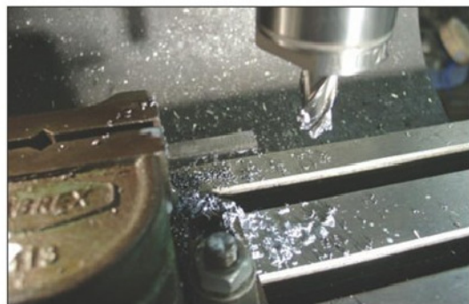
Photo 2. Milling the backing piece.
