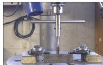
Photo 6. Using one of the wrenches in the drilling machine.
