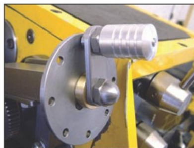
Photo 12. The eight hole index plate.
