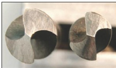
Photo 8. This photograph shows how the different clearances in photo 7 affect the chisel angle.
