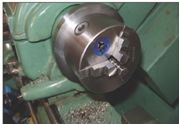
Photo 11. The assembled chuck on the lathe.
