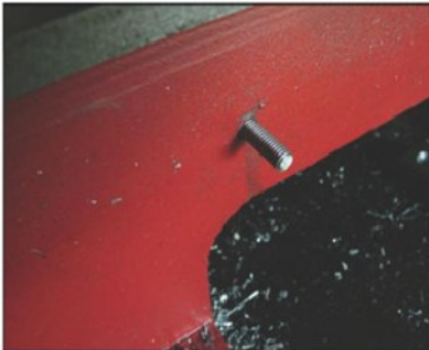
Photo 3. M5 screwed rod avoids wear to tapped hole in bed.
