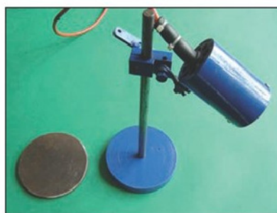
Photo 19. This light has a magnetic base.
