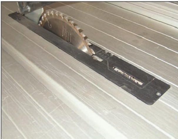
Photo 31. This saw bench has a scoring attachment.
