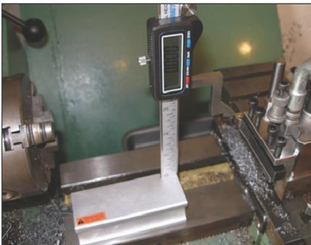
Photo 6. Setting the tool tip to the exact centre height.
