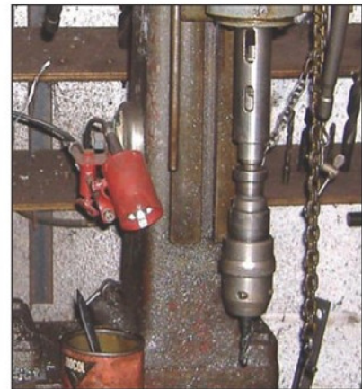
Photo 17. This light uses a magnetic mounting.
