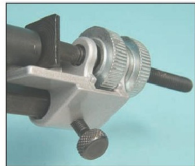
Photo 10. The jigs end stop and adjustment.
