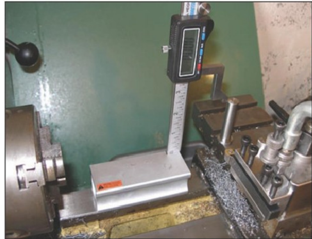
Photo 5. Setting the height gauge to the centre height.
