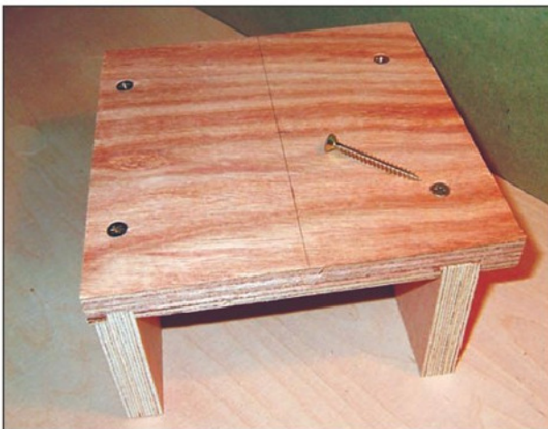
Photo 33. Simple screwed and glued construction is strong enough.
