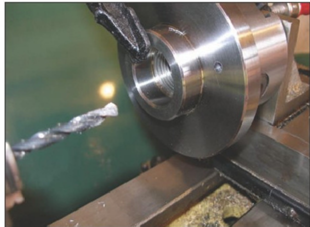
Photo 9. The first hole drilled.
