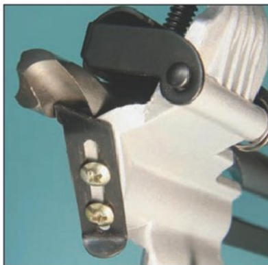
Photo 9. The finger intended for setting the drills rotational position.
