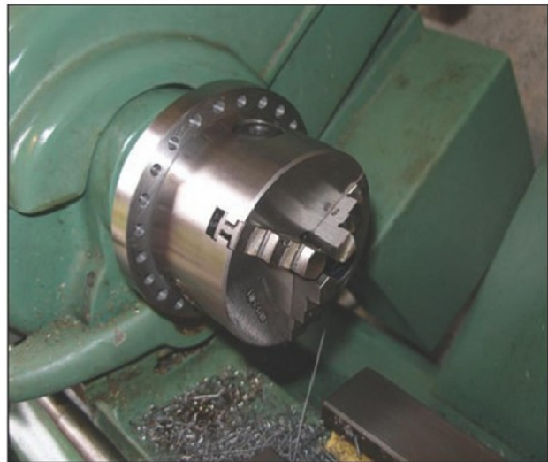
Photo 4. The finished drilled backplate on the lathe.
