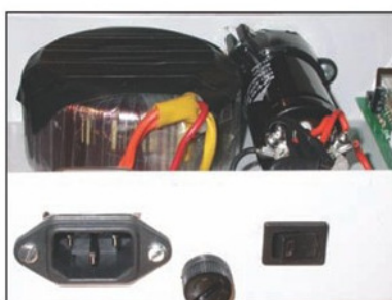
Photo 3. The power supply connections.
