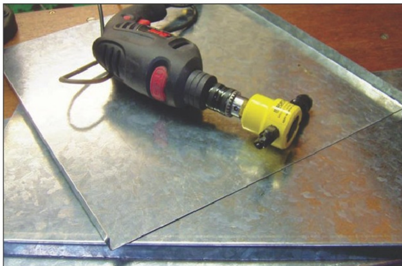
Photo 26. A sheet metal nibbler will be very useful.
