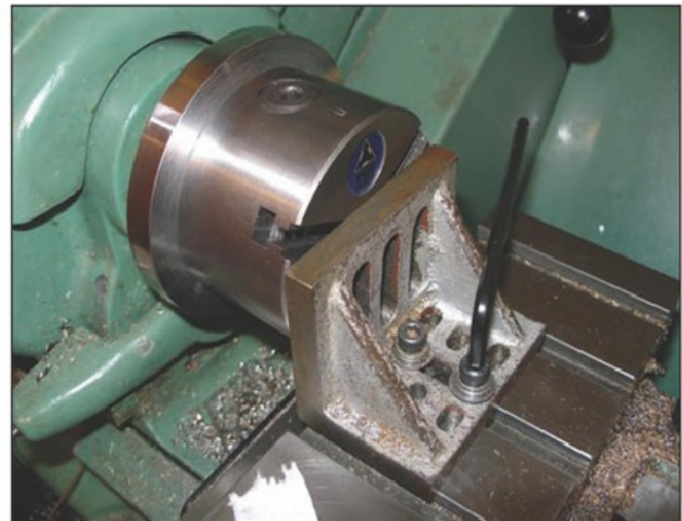
Photo 3. Setting the angle plate parallel to the chuck face.
