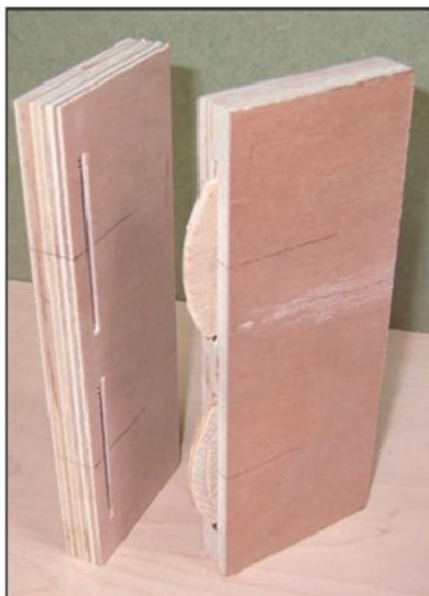
Photo 36. A biscuit joint ready for fitting together.
