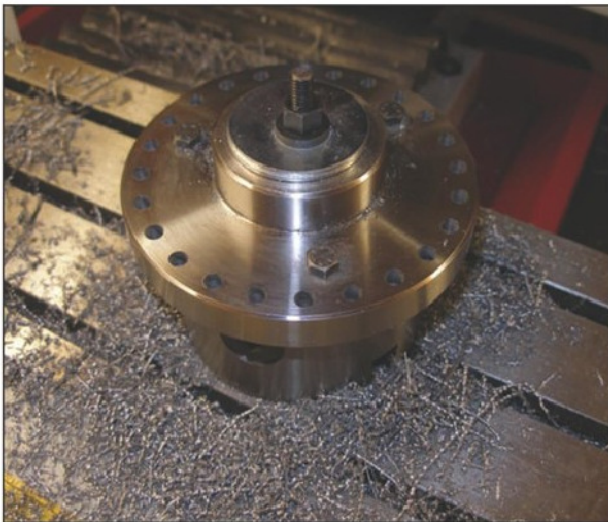
Photo 3. The swarf is shiny, not discoloured through too much heat.
