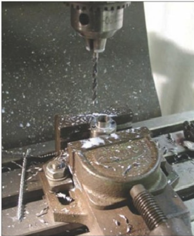
Photo 19. Drilling and tapping the pillar.
