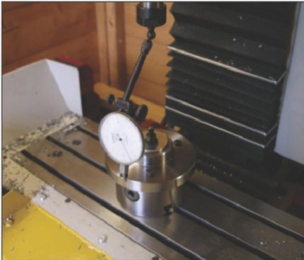
Photo 1. Clocking the outside of the backplate true.
