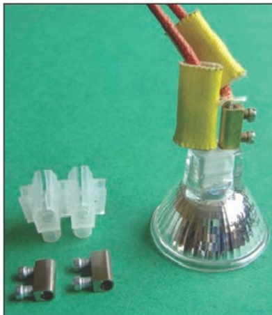
Photo 5. Terminals are cut out from a terminal block.
