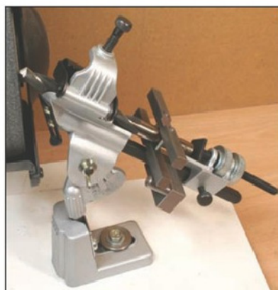
Photo 5. The jig in photo 2 set up ready for use with the offhand grinder.
