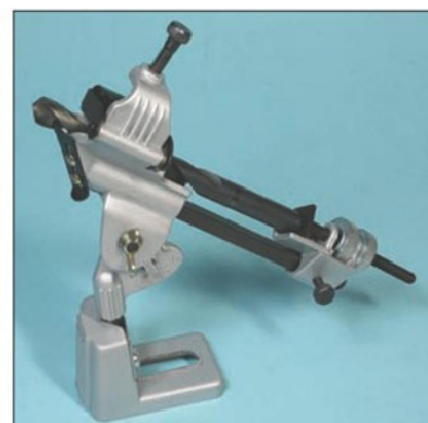
Photo 2. This jig, for use with an offhand grinder, is capable of more accurate results than the DIY version in photo 1.
