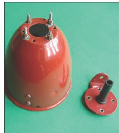
Photo 9. The end of the light showing method of mounting the end plate.
