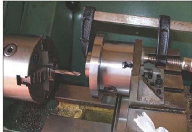
Photo 7. The backplate is clamped to the chuck.
