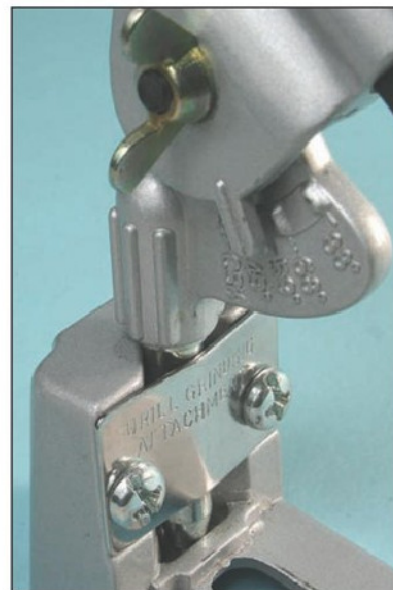
Photo 6. This view shows the spindle on which the jig rotates to carry out the sharpening process.
