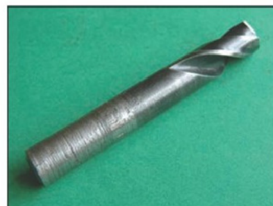
Photo 1. The drill used showing the modified end to stop snatching.
