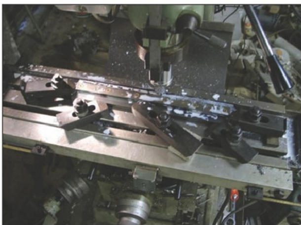
Photo 13. Clamps added and stop pins removed to clear cutter.
