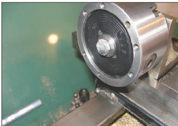
Photo 4. The chuck mounted on the angle plate.
