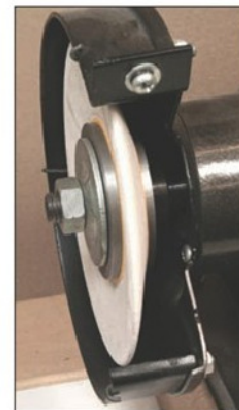
Photo 14. A saucer grinding wheel is useful, amongst other tasks, for point thinning.
