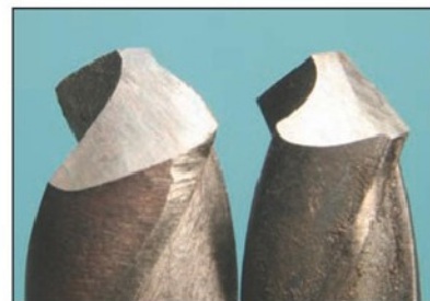
Photo 7. Two drills sharpened with the wrong clearance with too much on the left, too little on the right.
