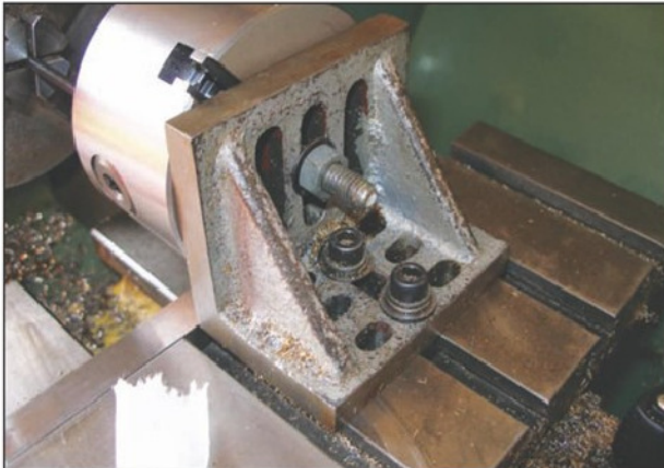
Photo 6. The chuck is bolted to the angle plate by a bolt through the centre.
