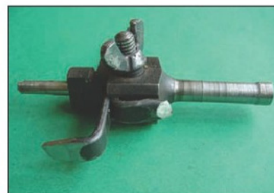
Photo 3. A typical tank cutter for cutting the larger holes.
