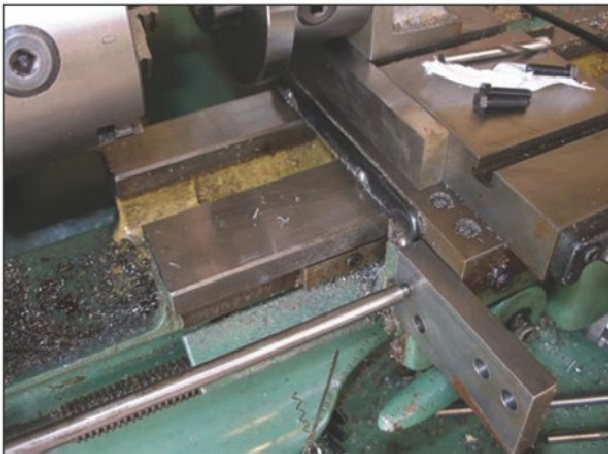
Photo 8. Setting the stop so the drill can't go too deep.
