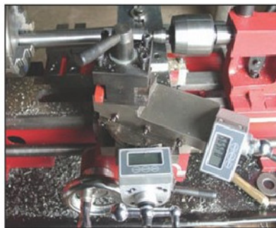
Photo 24. Top slide set over about 25 degrees.
