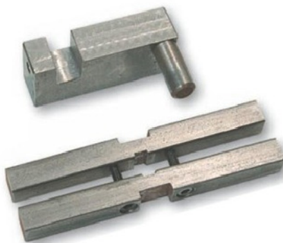
Photo 12. This device enables the drill to be rotated accurately 180deg. between sharpening sides one and two.
