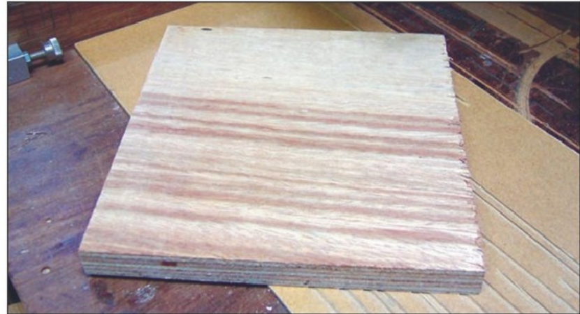
Photo 30. A backing board is one method to stop spitting the ply.
