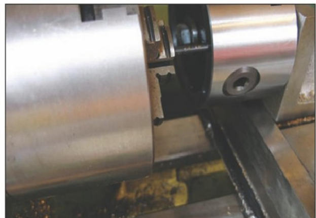
Photo 5. Lining the hole up with a drill shank.
