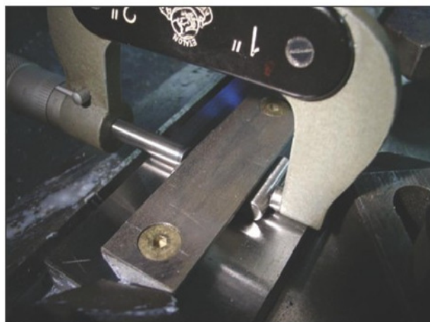
Photo 14. Width is checked at several places over rollers.
