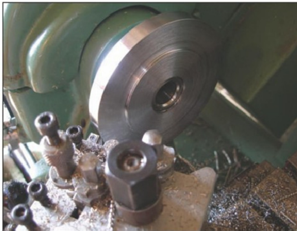
Photo 2. Chamfering the backplate after turning the chuck register.
