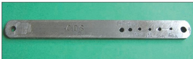
Photo 10. The plate used for shortening screws.
