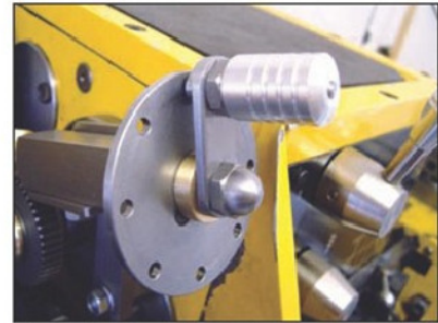
Photo 24. One hole pitch equals one deg.
