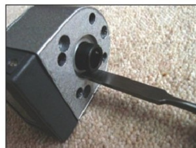
Photo 7. A scraper is employed to ease the counterbore.
