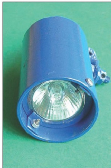
Photo 4. Robust home built 12 volt light.
