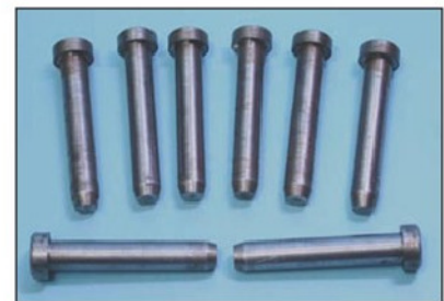
Photo 7. A saddle stop can be of considerable help when producing batches of identical parts, in this case setting the thickness of the pin heads.
