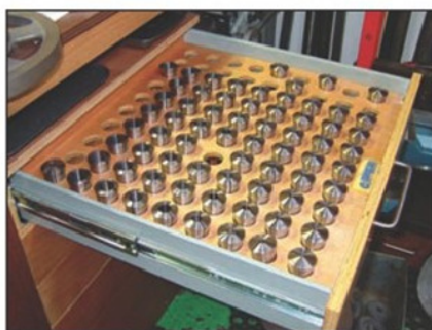
Photo 6. Collets can be stored in a tray rather than thrown in a drawer.
