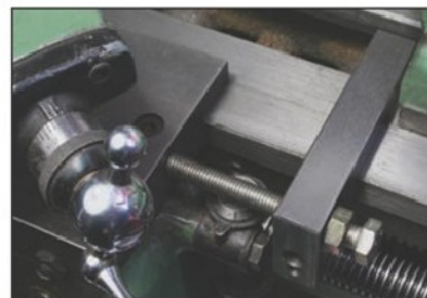
Photo 6. For a right hand face, the stop has to be moved to the other side of the saddle.
