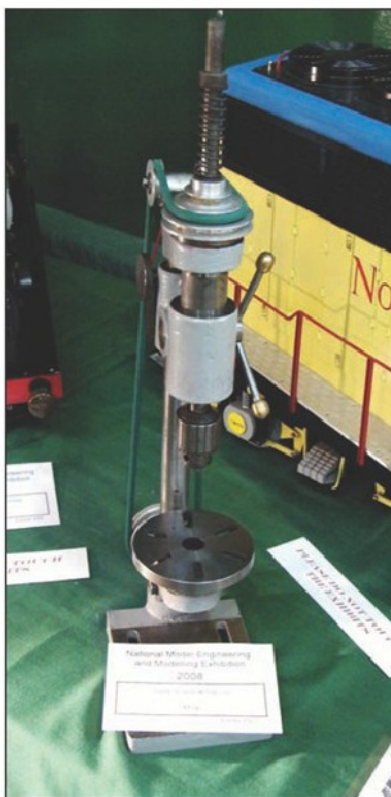
Photo 18. A freelance designed Sensitive Pillar Drill by Mr A King.
