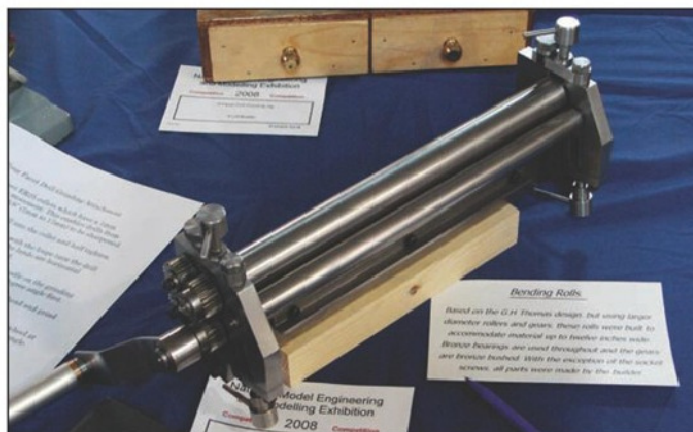
Photo 4. The Bending Rolls entered by Mr P Martindale are based on the classic George H Thomas design, but have been scaled up using larger diameter rolls and gears, to cater for material 12 inches wide. Bronze bearings are employed.
