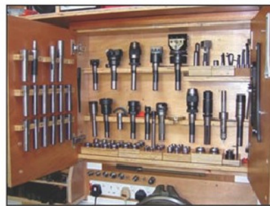
Photo 5. The 'R8' cabinet. The ER collets are in wooden blocks on the bottom shelf.
