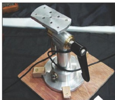
Photo 12. This woodcarving clamp, by Mr C Manns, allows the work to be rotated in two planes for access.
