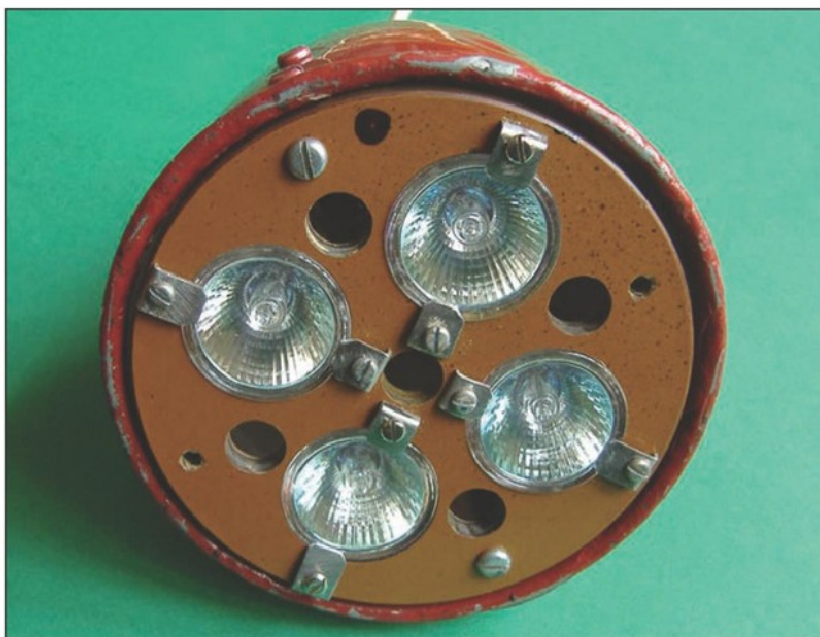
Photo 3. Machine light converted to take halogen units.
