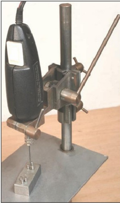
Photo 10. The hole size was 1mm and a sensitive drilling machine was required.
