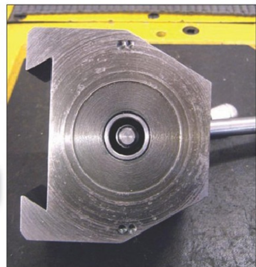
Photo 10. Two pairs of dimples for square and facing settings.
