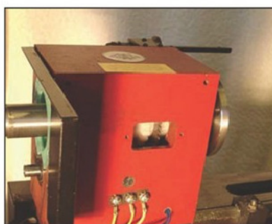
Photo 19. The sensor disc and spindle spacers can be seen through the aperture.
