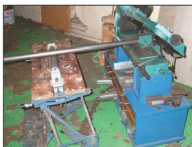
Photo 20. A workmate is used as a roller material support.
