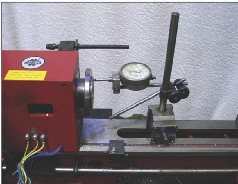
Photo 29. End float is checked with a clock gauge.
