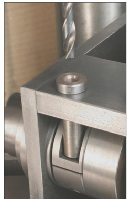
Photo 2. With a hole having to line up with a hole in the frame, a longer bush achieves the required result.
