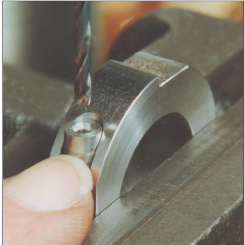
Photo 1. A simple drill bush makes this task an easy one.
