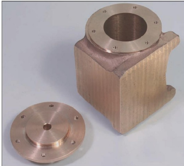
Photo 16. The parts having been drilled.
