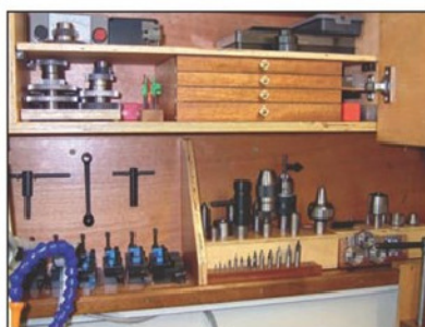
Photo 12. Drawer knobs are made from brass bar.
