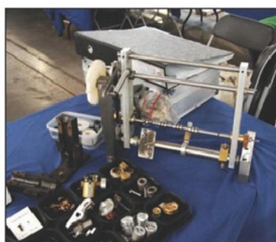
Photo 9. The cam grinding jig employed by Mr M Sayers.
