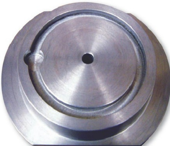
Photo 16. Slot cleaned up.
