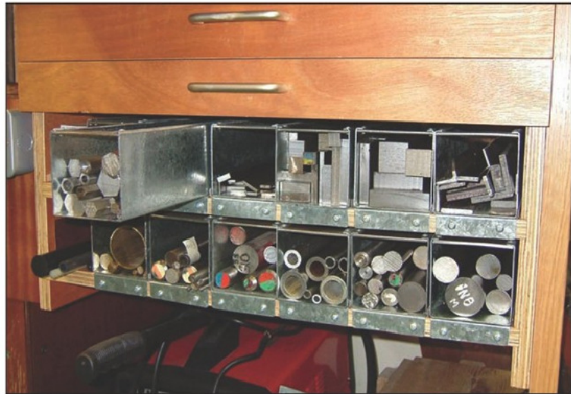
Photo 13. Galvanised trunking is used to store material. Square plastic guttering is a useful alternative.
