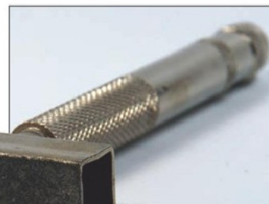
Photo 11. Multi point diamond hand wheel dresser.
