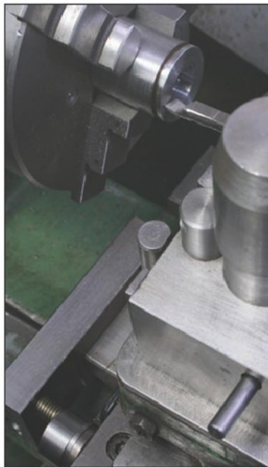
Photo 2. When boring a blind hole, the boring tool is traversed using the top slide to just touch the front of the workpiece with the gauges still in place. The hole will then be the correct depth once the gauges are removed.
