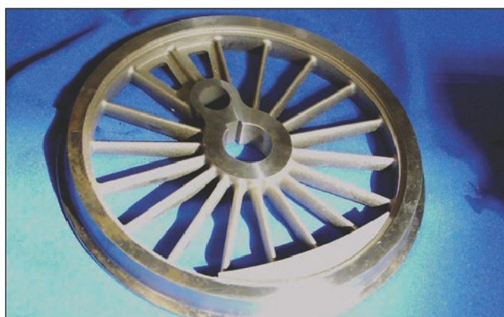
Photo 8. Locomotive wheel from Mr J Grabsch produced largely by electro chemical machining.
