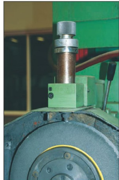
Photo 13. Multi point diamond dresser permanently mounted on a surface grinder.
