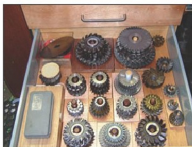
Photo 9. Larger milling cutters are stored on dowels.
