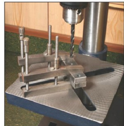
Photo 5. The clamps in photo 4 in use.
