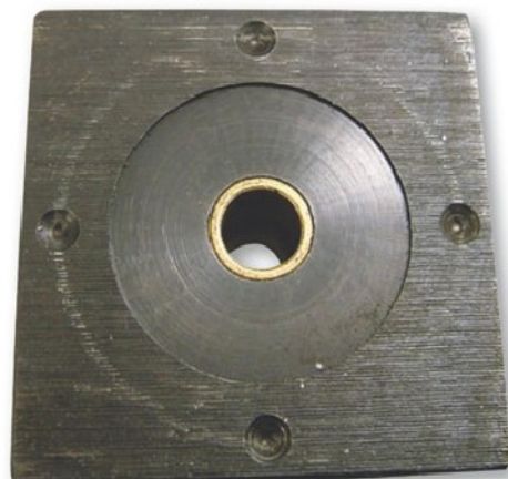
Photo 3. Underside view of toolpost showing dimples.
