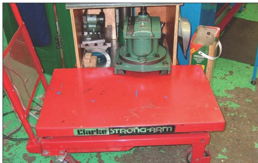
Photo 16. A hydraulic table is very useful in the workshop.
