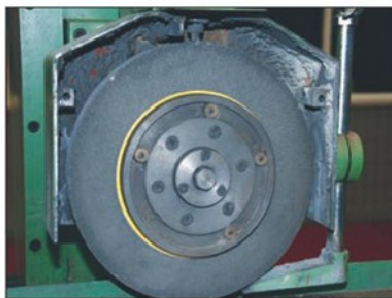
Photo 7. Balancing weights on a mounted grinding wheel.
