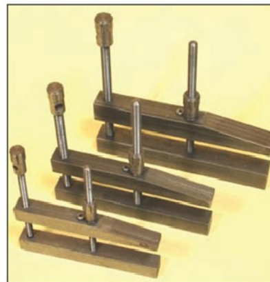
Photo 4. A form of toolmakers clamp that has distinct advantages in some cases.
