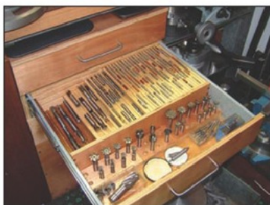
Photo 8. Cutters are stored upright in blocks to protect cutting edges.
