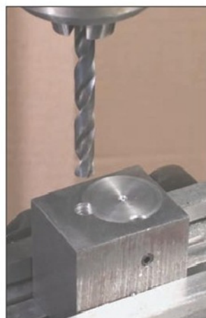
Photo 17. Using a jig to drill and tap a partial hole in a round component.
