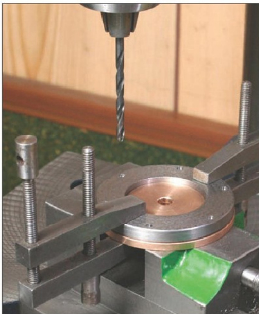
Photo 15. The end cover being drilled.
