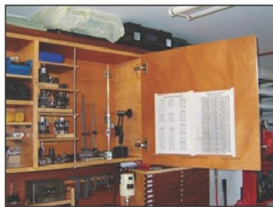
Photo 4. A typical wall mounted cupboard. Note the use of studding to support the small shelves.
