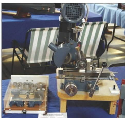
Photo 7. A Tool and Cutter Grinder to the well known Stent design, shown with accessories by Mr T Bracken gained a First.
