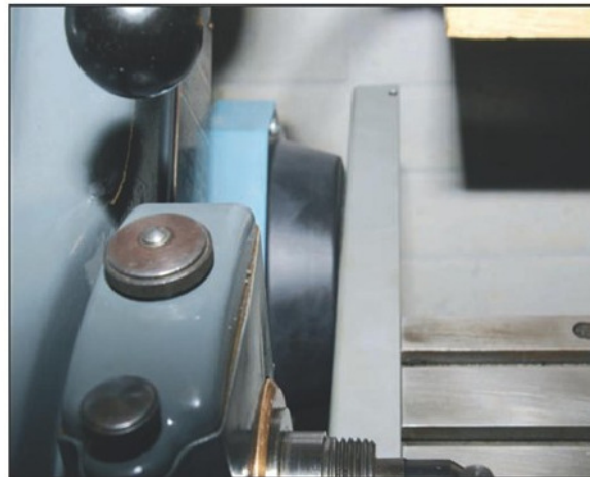
Photo 19. X axis SINO reading head clearance against motor.
