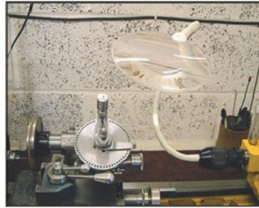
Photo 12. A magnifier was used to read the drum index.
