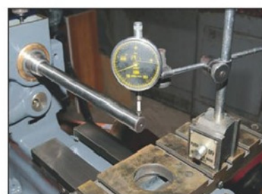
Photo 5. DTI Reading at end of test bar.
