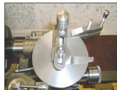
Photo 10. The temporary indexing hole is in the scrap metal that is clamped to the plate.
