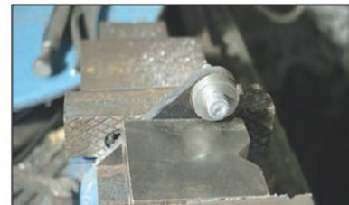
Photo 18. Clamping method to reduce vibration.
