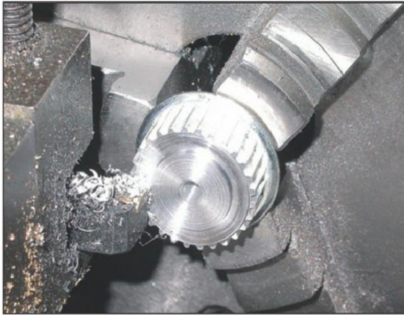
Photo 3. Removing the flange from the large pulley.
