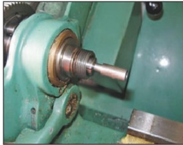
Photo 6. The back stop fitted in the collet.
