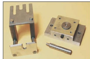
Photo 7. Accessories for an arbor press for use when punching holes.
