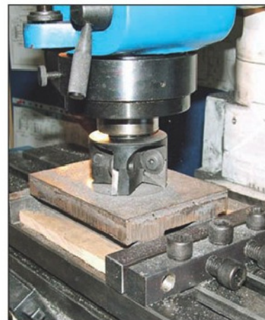
Photo 2. Face milling Cast Iron.
