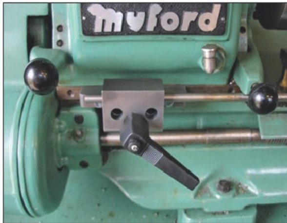
Photo 1. The finished stop fitted to the Myford.
