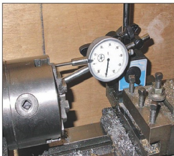
Photo 11. Checking for leadscrew backlash.
