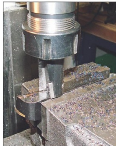
Photo 3. Milling a hardened lathe tool holder.
