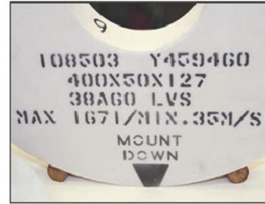
Photo 4. A large grinding wheel, 400mm diameter X 50mm wide X 127mm bore.
