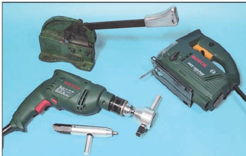
Photo 13. Four methods of cutting sheet materials, jig saw, power cut and nibbler attachments for use with a power tool, and a small guillotine.
