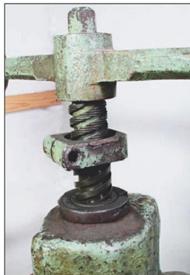
Photo 3. A fine pitch thread is usually provided on the outer diameter to provide the fine adjustment for a down feed stop.
