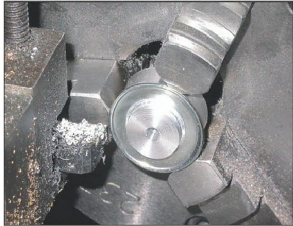
Photo 4. Shortening the pulley boss.
