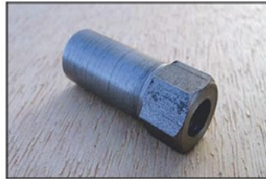
Photo 8. The toolpost nut.
