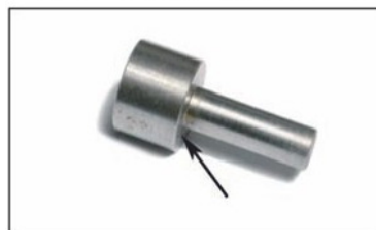
Photo 6. Solid plugs need an undercut.
