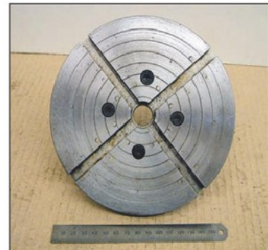
Photo 16. The homemade faceplate used to bore the banjo plates and sector fingers.
