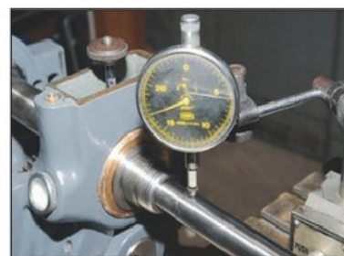
Photo 4. DTI Reading at Headstock.
