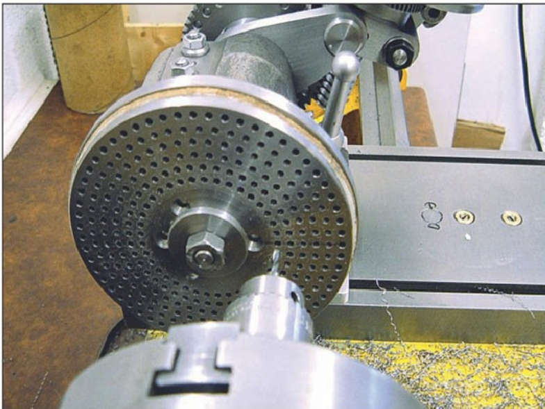
Photo 15. Check the holes by going to the first hole.
