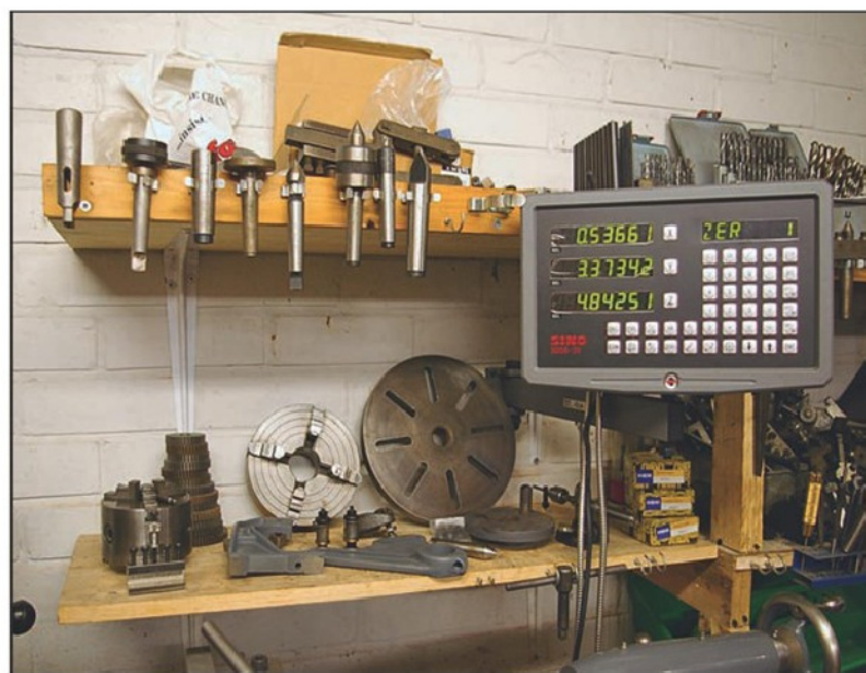
Photo 20. The SDS6-3V Console mounted on the wall.
