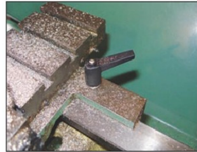
Photo 7. The carriage lock.
