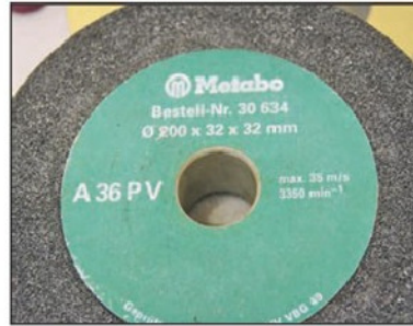
Photo 3. A typical grinding wheel. Note the maximum speed rating.
