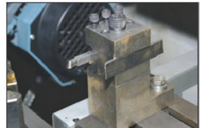
Photo 23. G H Thomas rear toolpost mounted and ready for use.
