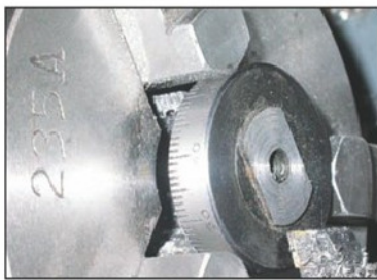
Photo 5. Remove the boss from the lathe dial.
