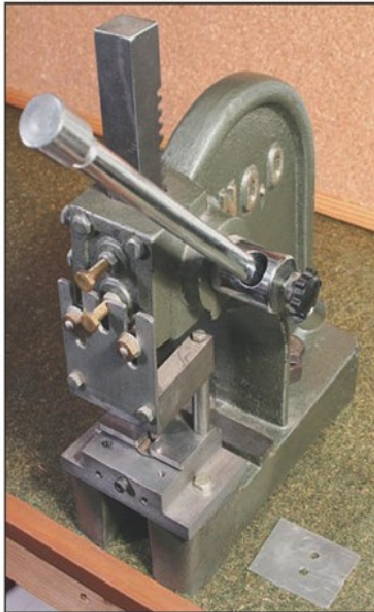
Photo 8. An arbor press set up for punching holes. See workpiece on the right.
