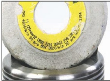
Photo 5. A wheel that does not appear if it has been well looked after.
