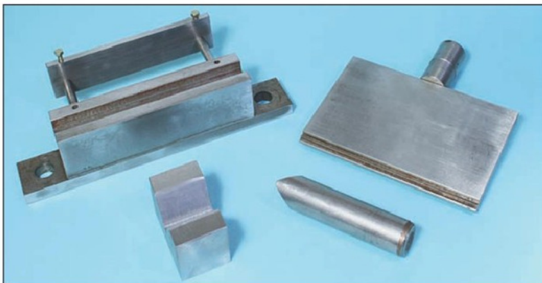
Photo 10. Accessories to enable bending of sheet and strip materials using a fly press.
