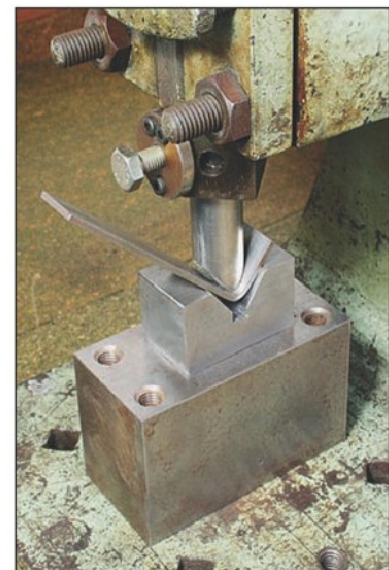
Photo 11. Bending strip material on the fly press.
