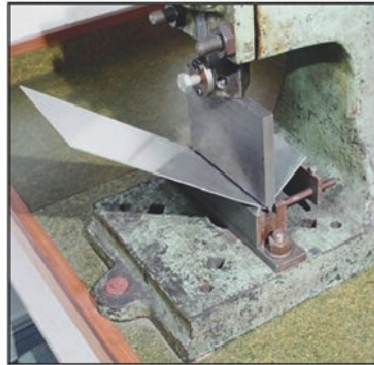
Photo 9. Using a fly press for bending sheet steel.
