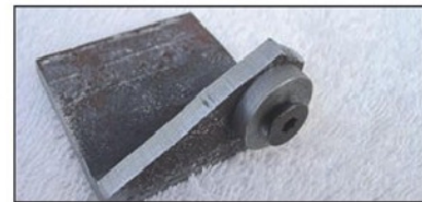
Photo 17. A turned button is used as a filing guide.
