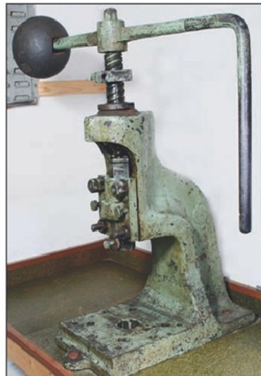
Photo 2. A much used small fly press of 3 tons nominal size.
