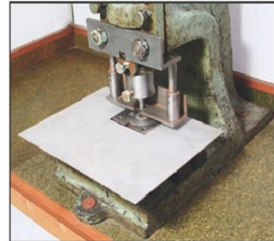
Photo 5. An overhead stripper assembly makes it possible to punch holes in large sheets. The set up also includes an auxiliary table for supporting larger workpiece's.
