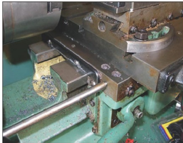
Photo 2. The stop rod position.
