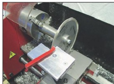
Photo 20. The cut away top supports the work behind the disc face.
