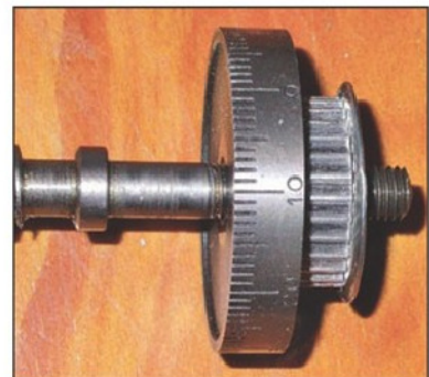
Photo 6. The front of the dial will act as a new pulley flange.
