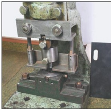
Photo 1. By repeat punching at about \frac{1}{4} of the hole's diameter, slots can easily be produced (right of picture) using a fly press.
