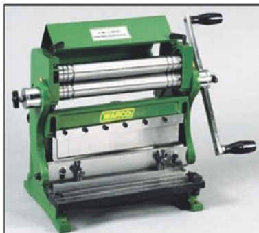
Photo 12. The Warco 3 in 1 sheet metal machine is available in 4 widths from 305mm up to 1000mm.
