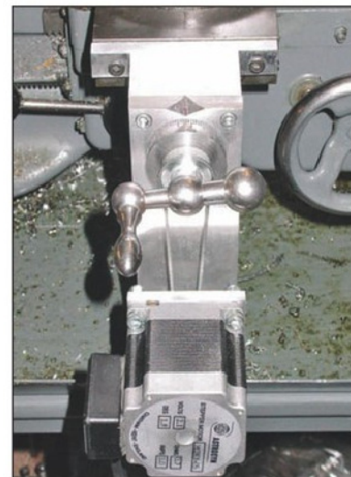
Photo 9. Tighten the belt by moving the motor in the slots.
