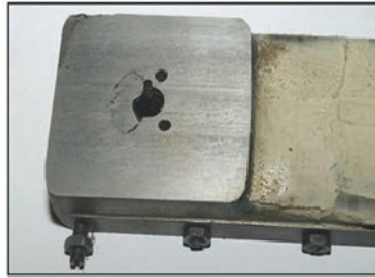
Photo 9. Top slide after building up with weld.
