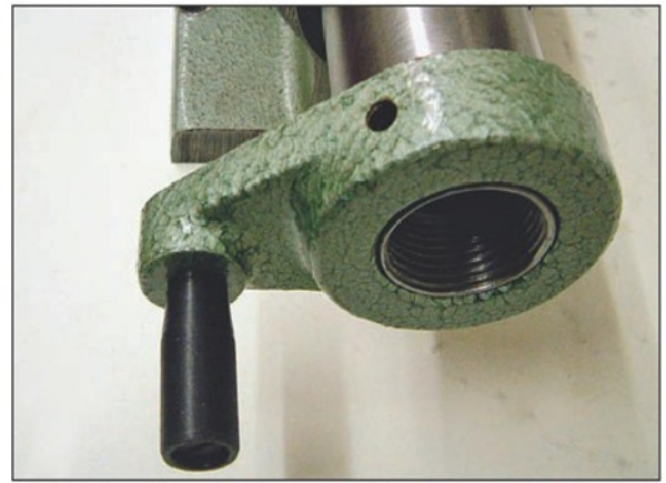
Photo 20 This handle is used for tightening the collet and turning the spindle.
