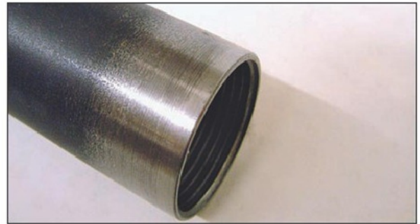
Photo 22. The slightly reduced end of the sleeve.
