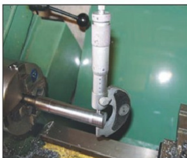
Photo 13. Measuring the other end of the test bar.
