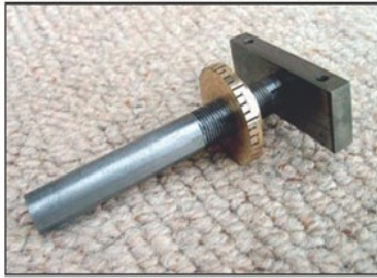
Photo 15. Pillar assembled with adjuster wheel and cradle base.
