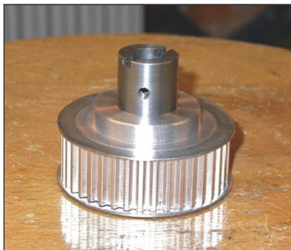
Photo 5. The leadscrew pulley with the new thrust collar.
