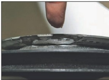
Photo 11. The countershaft weld after repairing.
