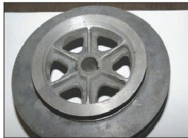
Photo 12. The pulley after skimming.
