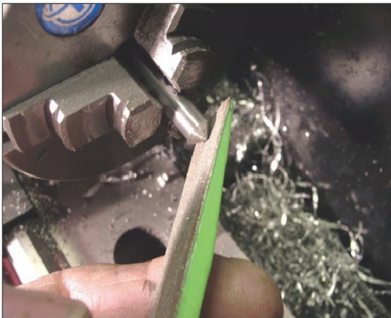
Photo 6. After hardening, the point was given a lick with a diamond hone.
