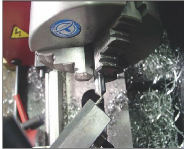
Photo 5. The point was turned using a part off tool, not particularly recommended but it happened to be convenient.
