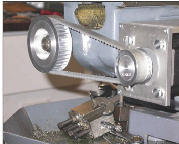
Photo 11. A rear view of the motor showing the mounting plate.
