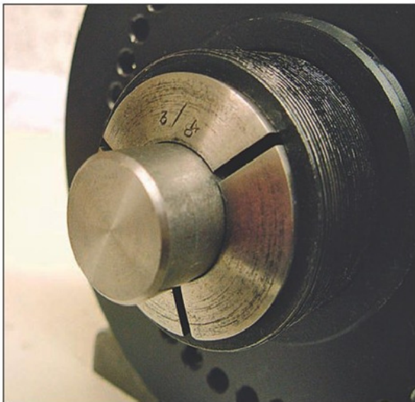
Photo 15. A bit of bar used to test the new drawbar.
