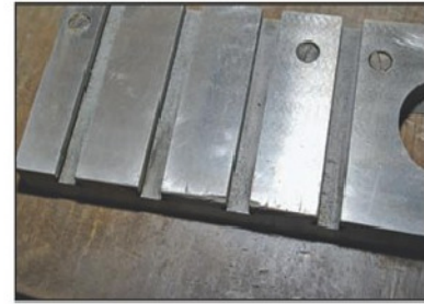
Photo 10. Surface grinding improved the cross slide.
