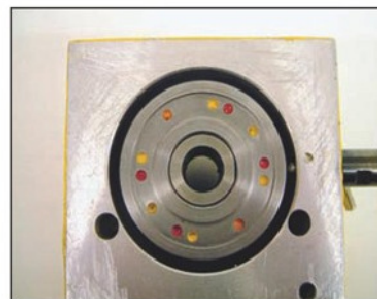
Photo 2. The coloured dots allow quick indexing.
