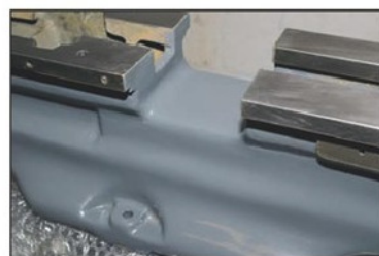
Photo 7. The lathe bed after spraying.
