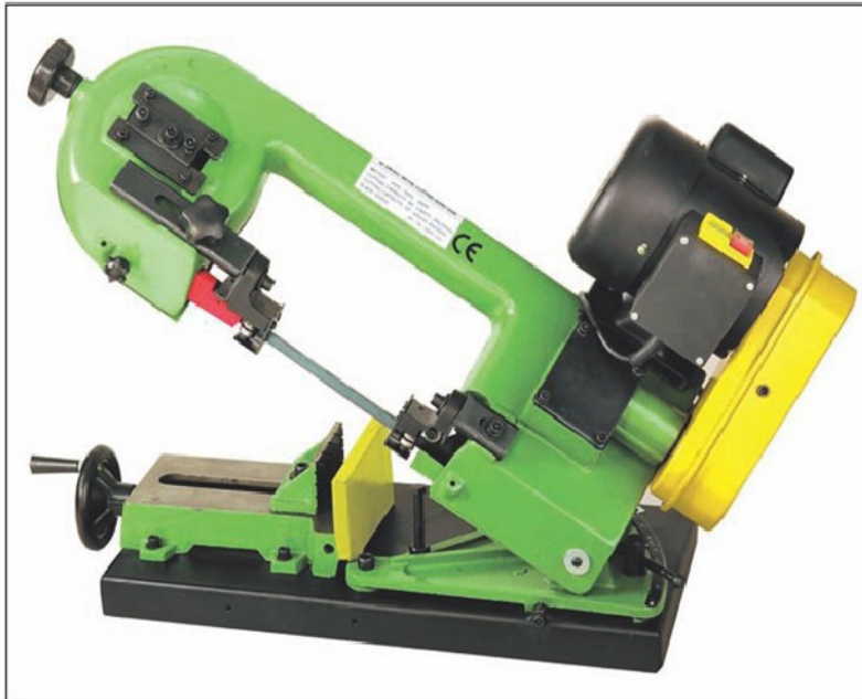
Photo 11. A small bench mounted horizontal bandsaw will avoid the need for floor space but could use up valuable bench space.
