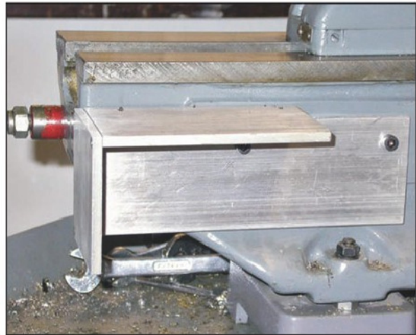
Photo 8. The motor mounting bracket is fitted using the existing holes in the lathe.
