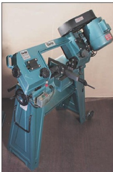
Photo 10. A horizontal bandsaw will minimise a lot of hard graft cutting bar materials.
