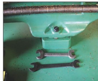
Photo 7. The Myford adjustable mount at the tailstock end.
