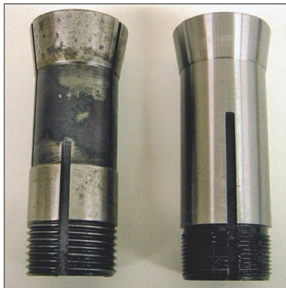
Photo 3. My old collet left, compared with a 5C collet, right.
