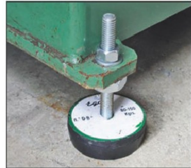
Photo 5. The stand needed raising quite a bit at the headstock end.
