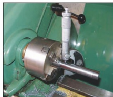
Photo 12. Measuring the test bar.
