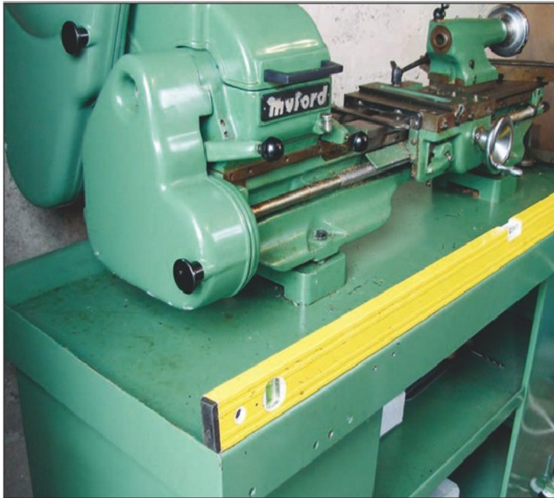
Photo 4. Levelling the stand up lengthways.
