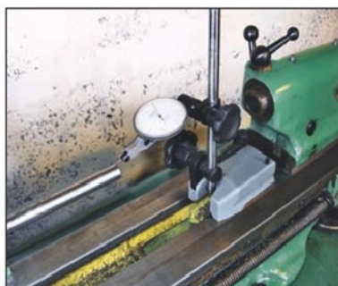
Photo 10. Testing with an indicator while tightening the bed down.
