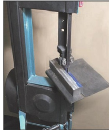
Photo 13. Some horizontal machines can be used in a vertical mode but this facility should only be considered for occasional use.
