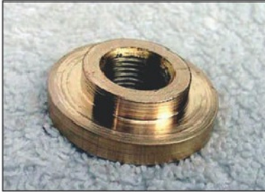
Photo 10. The adjuster wheel, turned and tapped.
