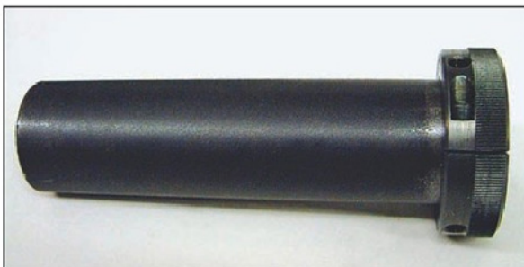
Photo 23. The locking collar on the sleeve.
