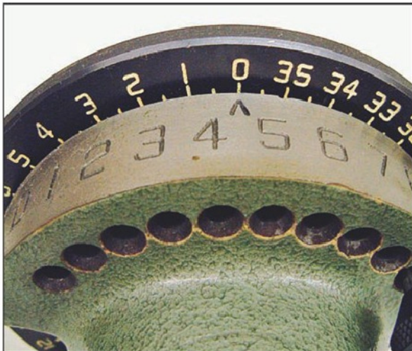
Photo 25. The original fiducial indexing mark.
