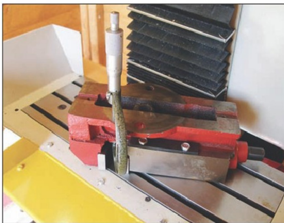
Photo 7. Checking the vice thickness.
