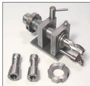
Photo 6. An end mill sharpening fixture for use with the grinding rest in photo 4.
