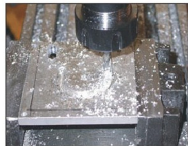
Photo 9. Machining the motor mounting holes on a CNC mill.
