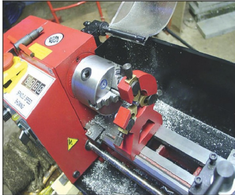
Photo 19. Fixed steady positioned close to the chuck for setting.
