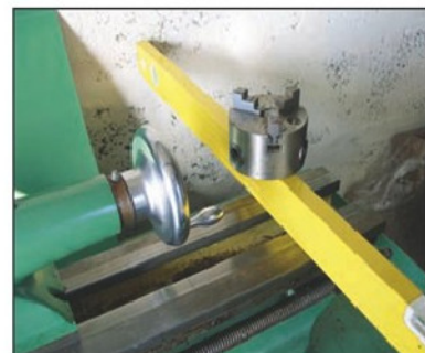
Photo 8. Levelling the lathe bed crossways.
