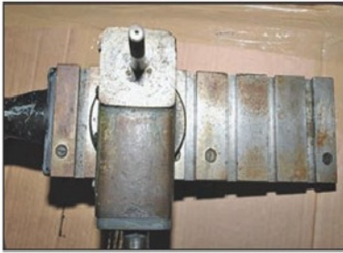
Photo 8. The cross and top slide before renovation.
