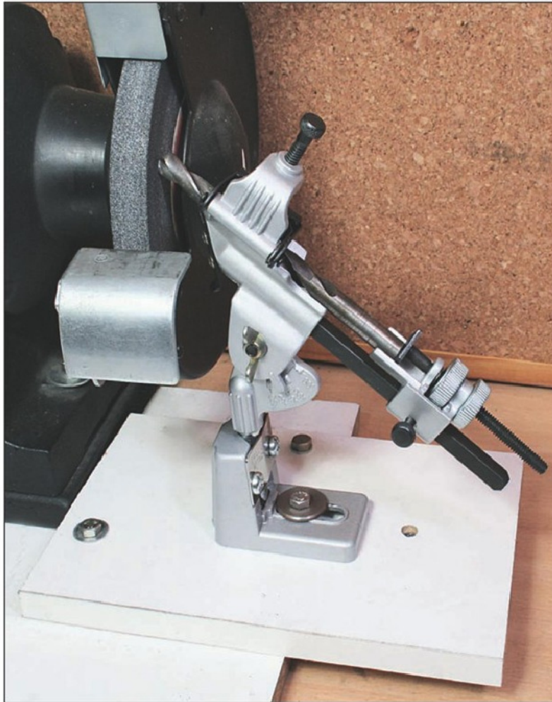
Photo 3. Except for woodworking tools, drill grinding fixtures are the only sharpening accessory commercially available for use with an off hand grinder.
