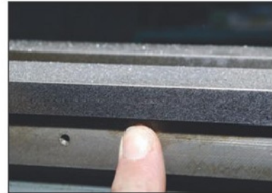
Photo 14 The second pass cleaned the bed up completely.
