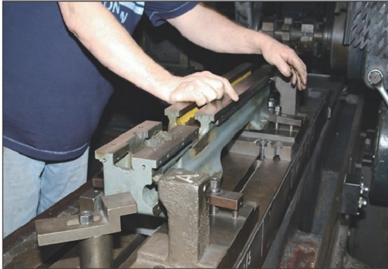
Photo 10 Setting the bed true on the horizontal mill.
