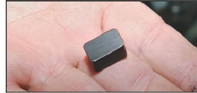
Photo 11 One of the ceramic tips used to mill hardened beds.
