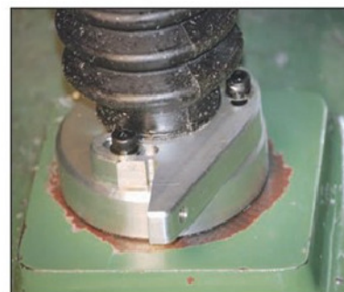
Photo 17 The finished bracket installed on the Z-axis ball nut flange.
