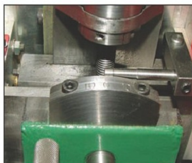
Photo 7 Scale for the tilting grinding head.
