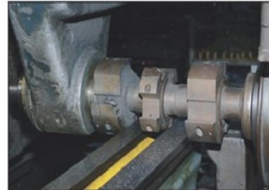
Photo 12 Milling the front shears.
