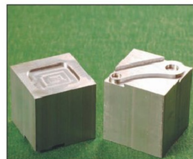
Photo 8 First cuts – simple pocket and curved profile – both in 2 1/2in. square blocks.
