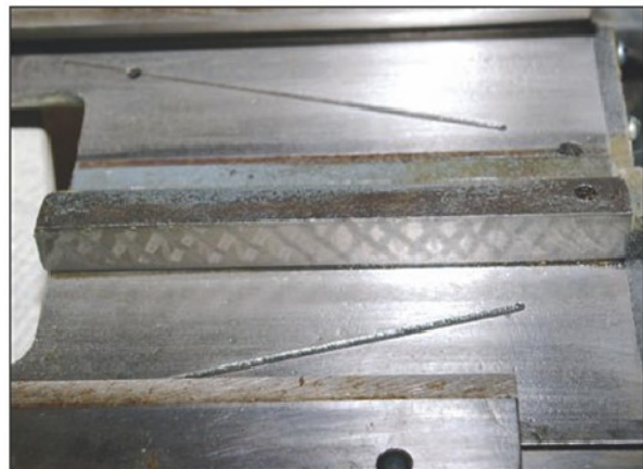
Photo 24 The "fast" edge on the saddle after scraping.
