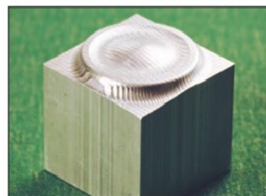
Photo 13 A 3D test block.
