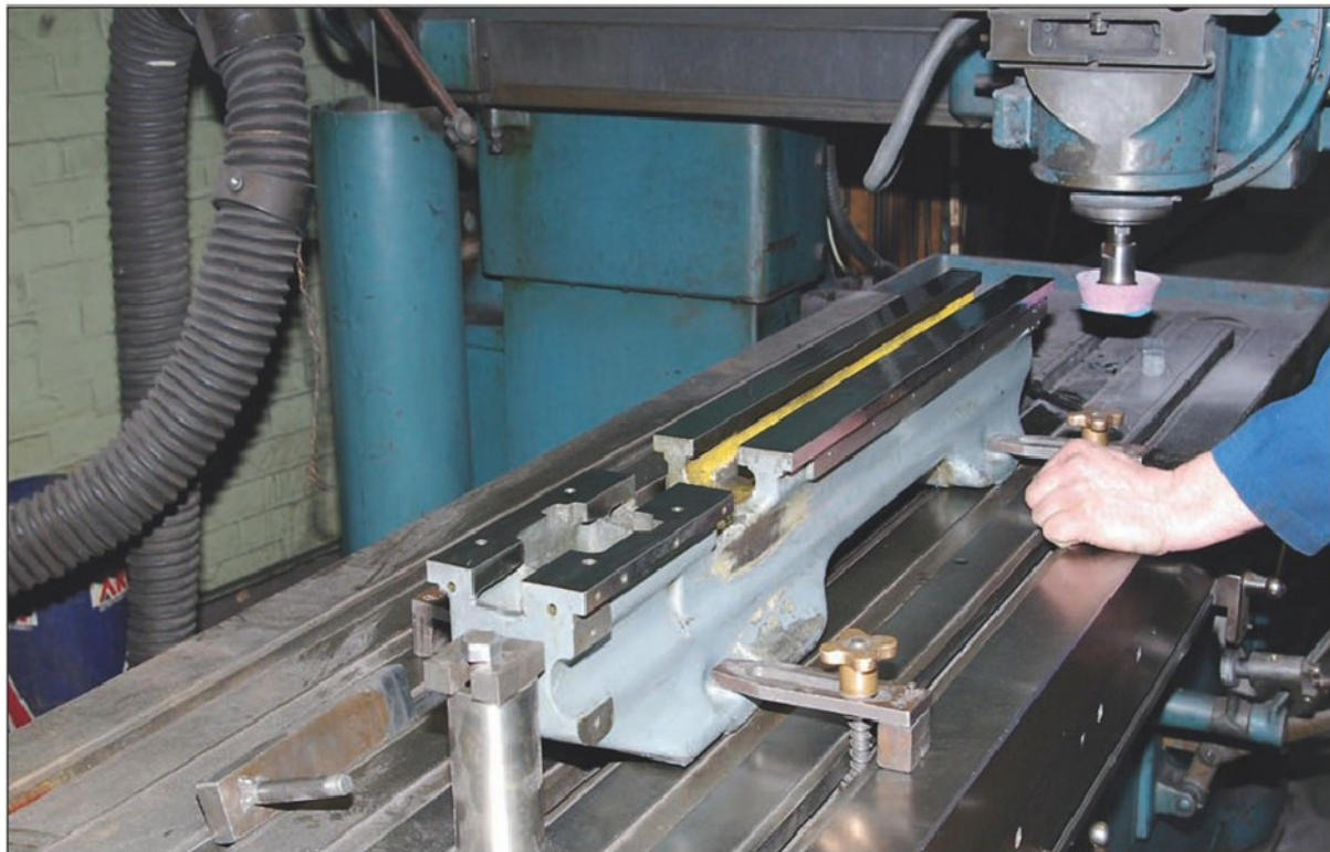
Photo 18 Grinding the underside of the shears.
