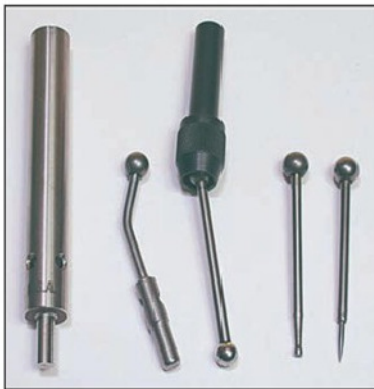
Photo 28 Two edge finders, illuminated and a Wiggler.
