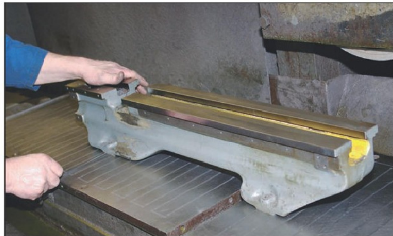
Photo 15 Setting up the bed to surface grind the top faces.
