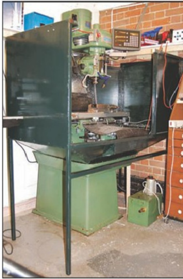
Photo 9 The freestanding enclosure to contain flying swarf and coolant.
