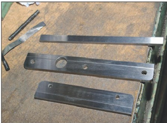
Photo 23 The strips with the steps ground in.
