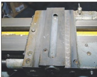
Photo 7 There was a lot of wear on top of the saddle.
