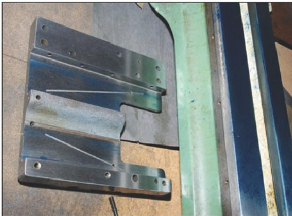
Photo 21 Testing the saddle with marking blue.
