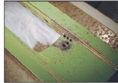
Photo 6 The chain drilling in the knee casting to provide clearance for the Y-axis ball nut.
