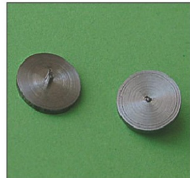
Photo 21 The parted off components showing the pips.
