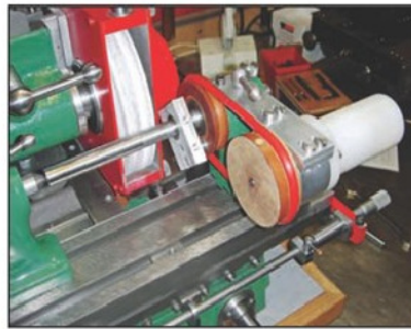
Photo 10 Drive unit on RH tailstock.
