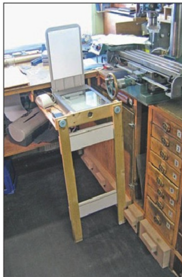
Photo 14 Flatbed scanner in the working position. Note clearance for handles cut in 'H' frame.
