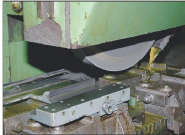
Photo 20 Grinding the underside of the saddle.
