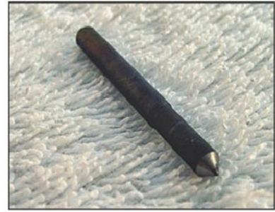
Photo 8 Transfer punch made from silver steel.
