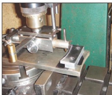
Photo 6 Engraving the table scale.
