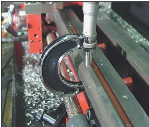
Photo 3 Measuring the front shear.
