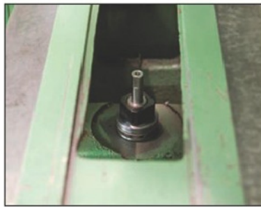
Photo 3 The top of the Z-axis ball screw awaiting pulley.
