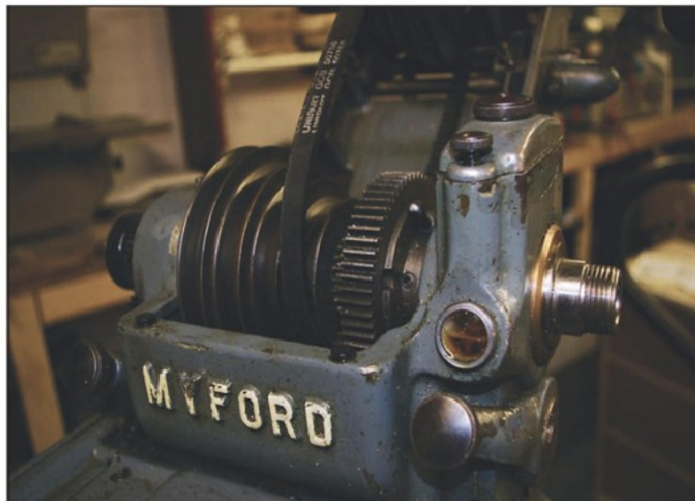
Photo 2 The headstock before refurbishing.
