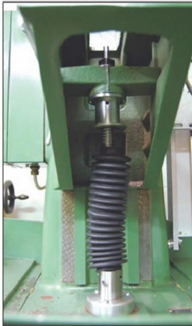
Photo 2 The Z-axis ballscrew. 2 Morris Minor rack gaiters await clipping into place.
