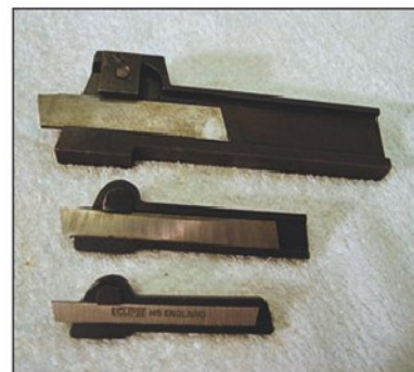
Photo 11 Three commercial part off tools, top \frac{5}{8} - \frac{1}{2} in. middle \frac{1}{2} in. bottom \frac{1}{4} in.
