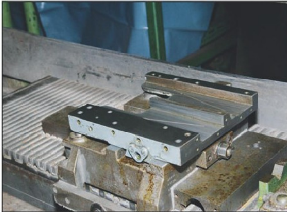
Photo 19 The saddle is set up in a special jig for grinding true.
