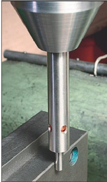
Photo 27 The light in this edge finder lights when it contacts the item being located.
