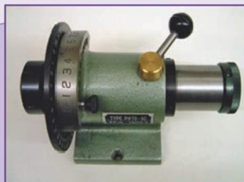
A spin on collets Jim Whetren modifies a spin indexer
