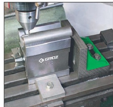
Photo 26 A magnetic V block should only be used for lightweight duties and then only when security of the workpiece and V block is certain. If in doubt, use another method.
