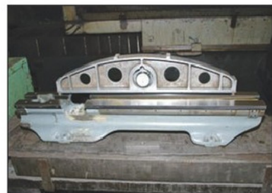
Photo 17 Testing the bed after grinding.
