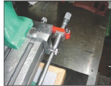
Photo 5 Removable table adjuster and micro setting for table stops.
