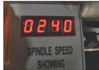
Photo 5 A digital readout on the C1 lathe.
