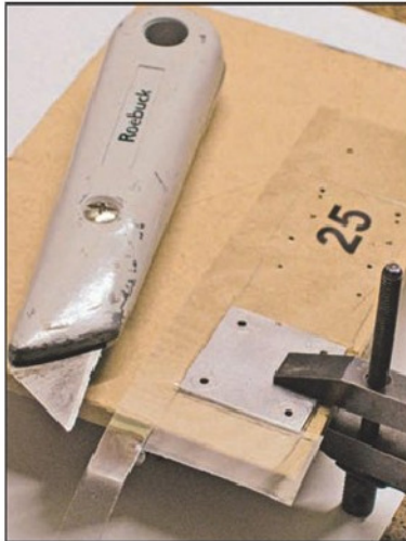
Photo 23 Cutting numbers from film using clamped jig.
