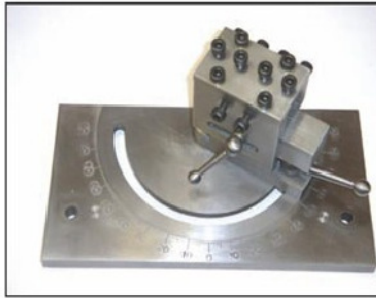
Photo 3 Square tool grinding fixture.
