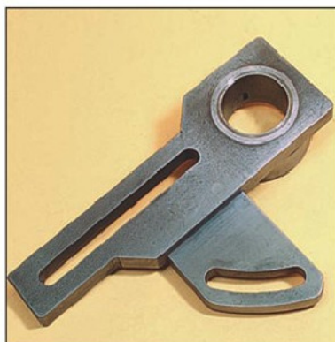
Photo 33 A rotary table is ideal for making the curved slot in this change wheel quadrant.
