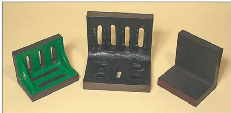
Photo 22 The three common forms of angle plate
