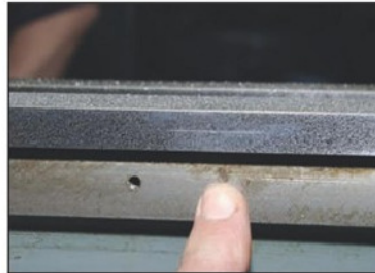
Photo 13 The first pass left some marks in the bed.
