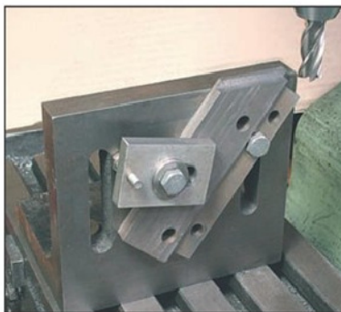
Photo 21 Positioning a workpiece is often easier using an angle plate rather than a vice.
