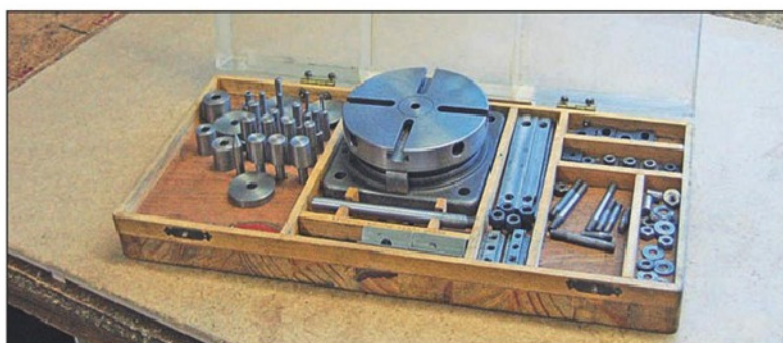
Photo 31 Dedicated storage for a small hand operated rotary table.
