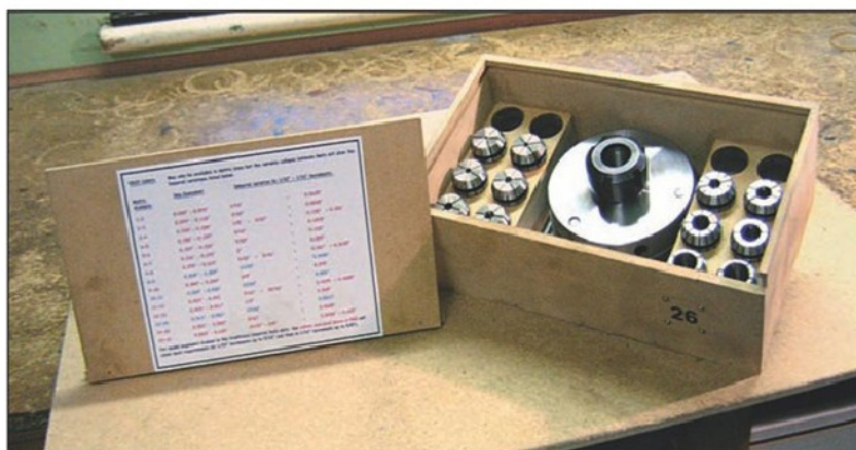
Photo 30 Dedicated storage for an ER25 Collet chuck and collets.
