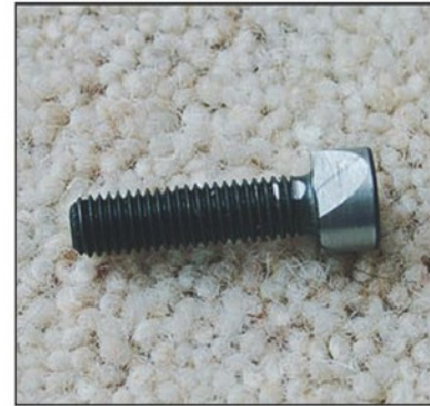
Photo 18 Clamp bolt after modification.
