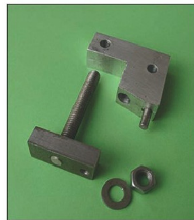
Photo 5 Component parts of the front clamp, note the lower surface filed away.
