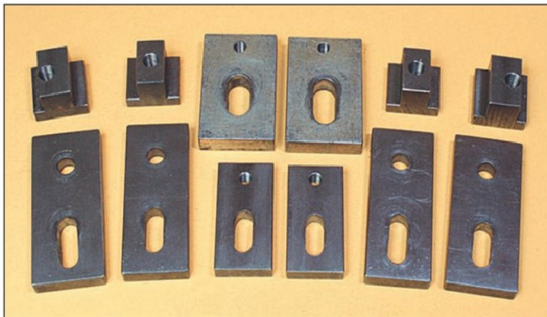
Photo 14 Shop made light duty clamping components will be preferable to the commercially available kits in most cases.
