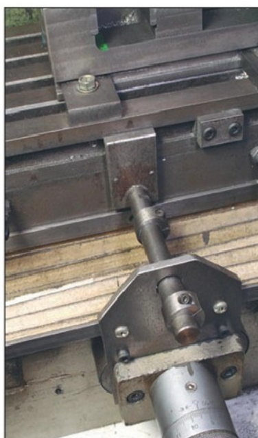
Photo 5 As Y axis stops are rarely available on machines as purchased, shop made stops, as those in the photograph are the only option.
