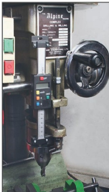
Photo 4 A digital display has been added to a mill/drill's down feed.
