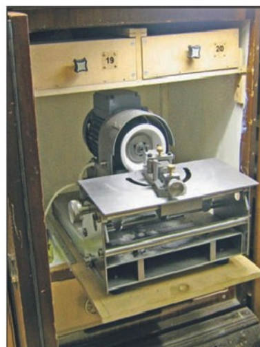
Photo 13 Cabinet for "Worden" tool grinder.
