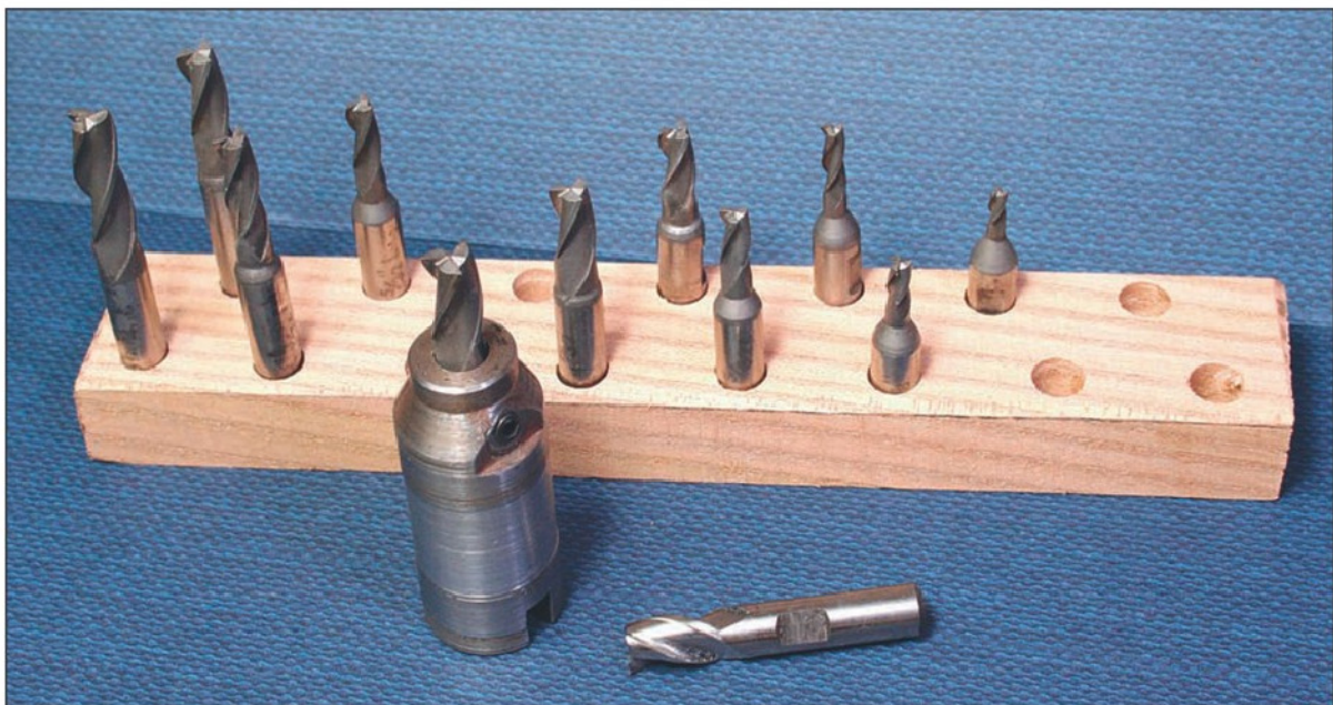
Photo 8 Mini mills are can be plunged and are primarily used for milling closed end slots and open-ended grooves.
