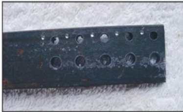
Photo 24 One piece of flat bar has been drilled to create five small clamps.
