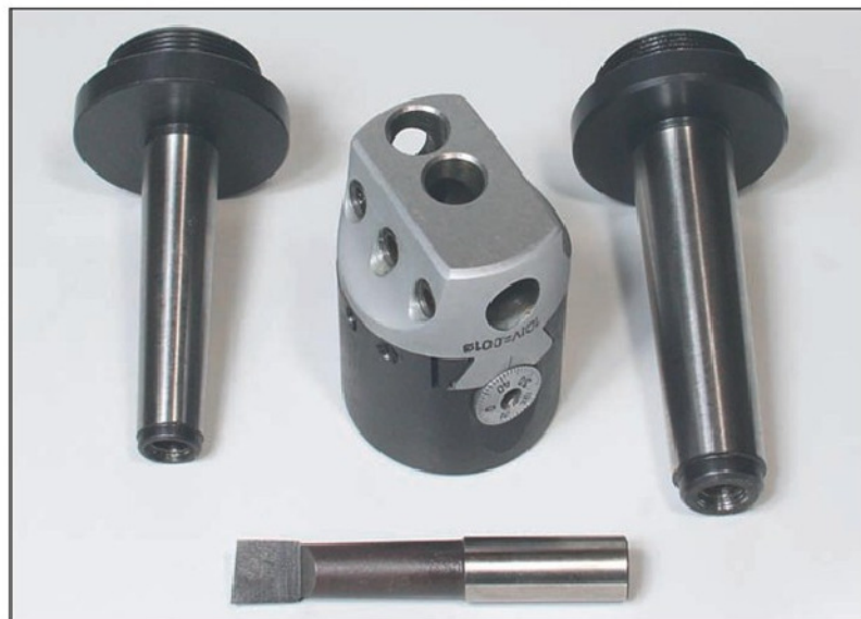
Photo 12 A boring head with numbers 2 and 3 Morse taper shanks.
