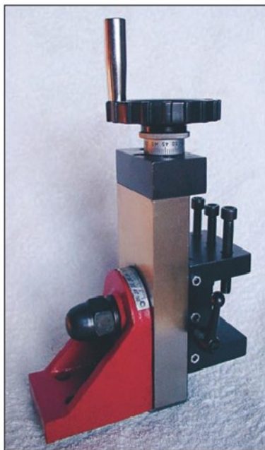
Photo 2 The vertical slide for the C3 lathe as supplied by Arc Euro Trade.
