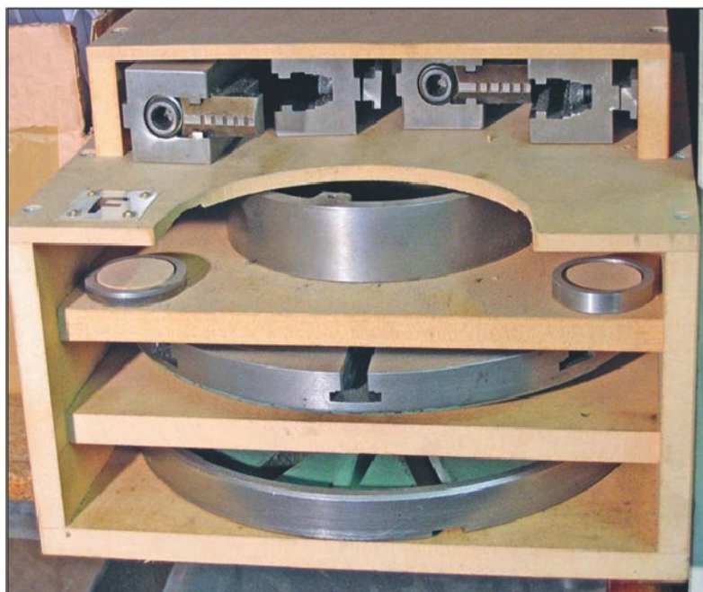
Photo 10 Faceplates stored flat with extended jaws.
