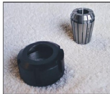
Photo 15 A detail view of an ER32 collet and closing ring.
