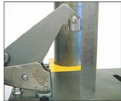
Photo 16 The maximum capacity of the Mole wrench.
