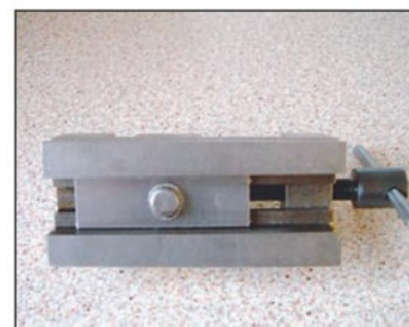
Photo 10 The underside of the vice showing longer jaw plate.
