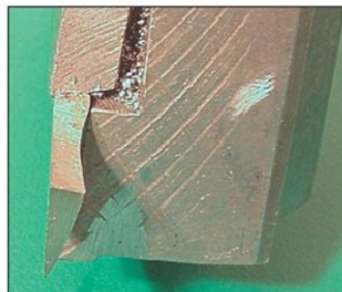
Photo 2: The trepanning tool, the cutting tip.
