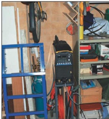
Photo 4 Zoning – Above the welder are the rods and other welding small tools, gas and filler rods are to the left, helmet and gas torch stored to the right. The blue frame is a folding welding table with a detachable top. This is the edge of 'my space' so there is also a bike hanging from the roof.
