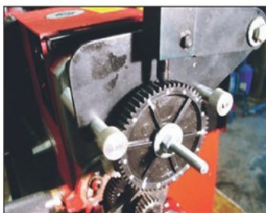
Photo 10 The changewheel has been marked to indicate the teeth to be used.
