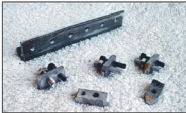
Photo 25 Clamps have been cut off, tidied up, and fitted with screws.
