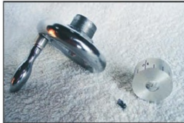
Photo 8 The handwheel with a graduated collar and friction rivet.
