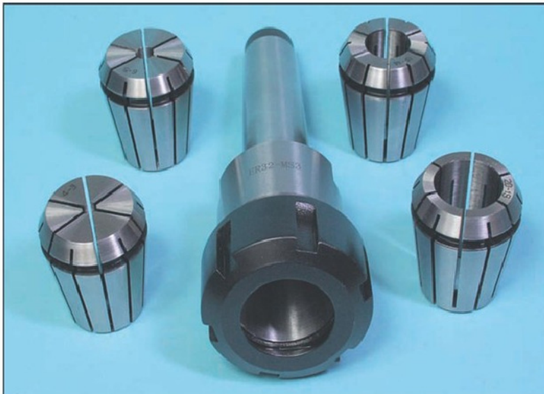
Photo 11 An ER collet chuck with a Morse taper mount.
