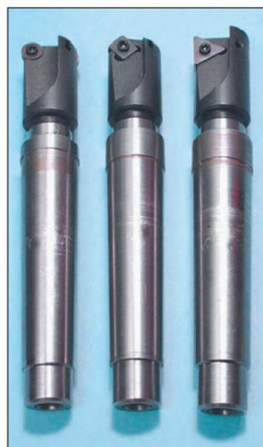
Photo 6 Indexable milling cutters with round, diamond and triangular tips.
