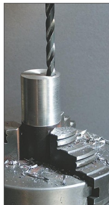
Photo 3 Drilling and tapping the offset hole.
