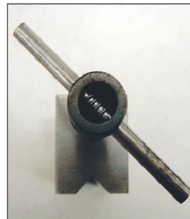
Photo 12 The tommy bar is retained by a spring.
