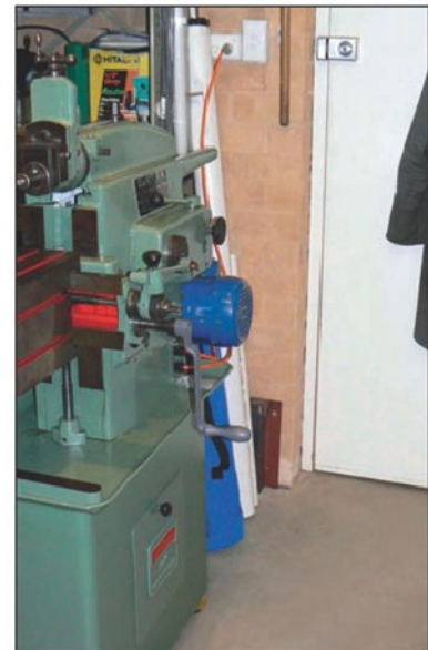
Photo 6 Shaper controls are accessed from the aisle way (machine operation from aisle ways) – a no-no in an industrial setting but all right at home. V belt changes are made from a space behind the drill press.
