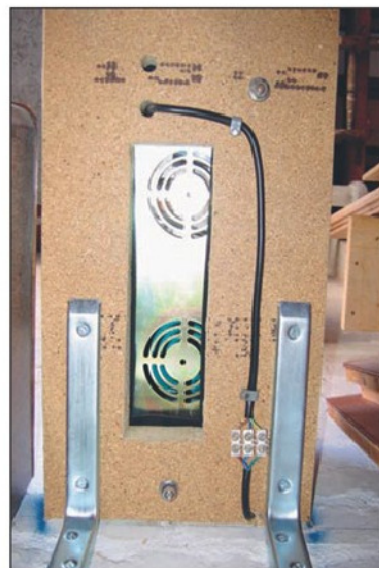
Photo 4 'Clarke' sander showing underneath air access hole.
