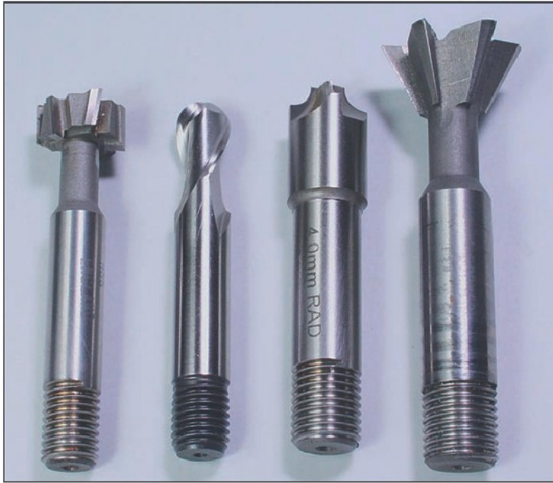
Photo 9 The four types of milling cutter that should only be purchased as a need arises. These are, left to right, T slot cutter, ball nosed end mill, rounding end mill and dovetail cutter.
