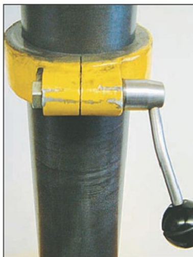
Photo 2 The head support clamp with added handle.
