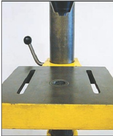
Photo 4 The drill table
