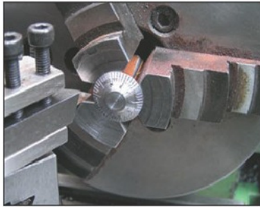
Photo 5 Engraving the divisions on the dial.
