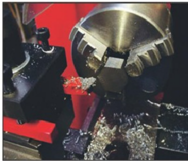
Photo 3 Facing the hexagon material.
