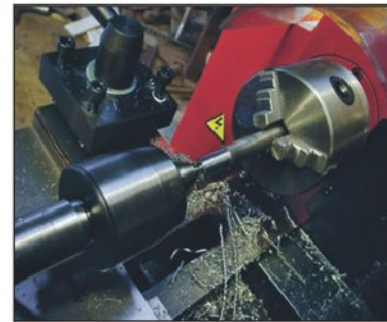
Photo 5 Turning the first section of the extension shaft.
