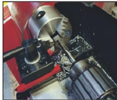
Photo 4 Tapping a nut under power.
