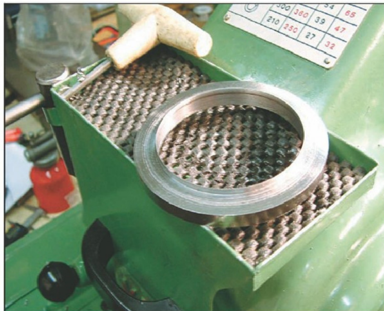
Photo 7: What's left: The ring produced by Trepanning and Parting off.
