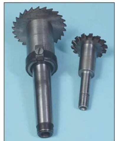
Photo 10 Disk type cutters mounted on adapters to enable them to be used on a vertical machine.
