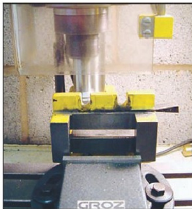
Photo 8 Cutting the mounting lugs off the vice.
