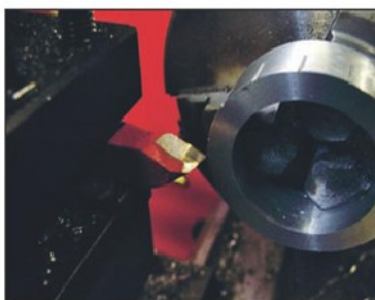
Photo 11 A vee tool has been mounted on its side to cut the divisions.
