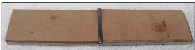
Photo 12 Three pieces of MDF serve as a punch guide.
