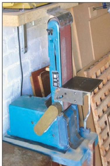
Photo 2 'Clarke' sander with replaced belt guard support.
