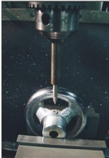
Photo 7 An extended centre drill reaches places others cannot.
