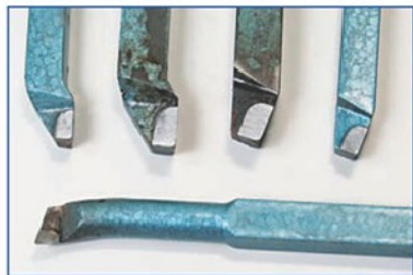
11 Lathe tools having brazed tips.
