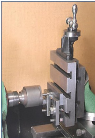
3 A vertical slide provides the third axis for milling.
