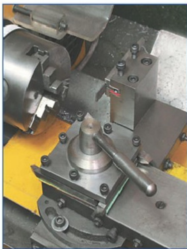
14 A four way post makes your four most used tools almost instantaneously available.
