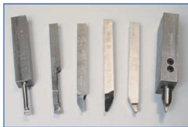
12 High speed steel lathe tools are essential for special shapes that cannot be obtained in the other two types.
