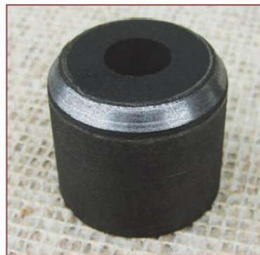
P4 A roller showing the heavy chamfer to clear the channel radius.
