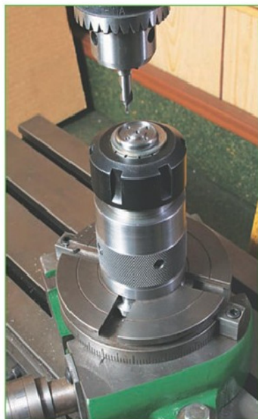
16 The lathe's collet chuck being used on the adapter in photo 14.
