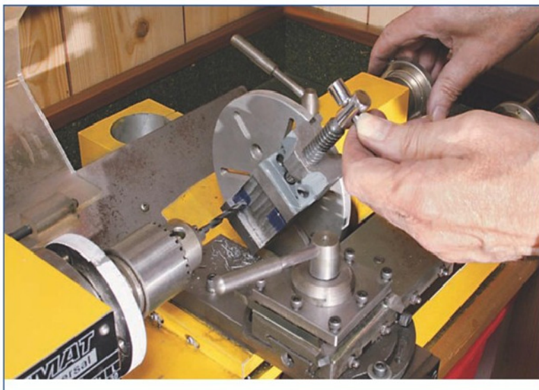
1 Using the lathe as an alternative to a drilling machine is possible but not ideal.
