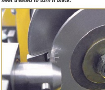
Photo 11 The engraving has been heat treated to turn it black.
