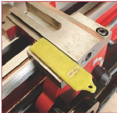
18 Milled surface of the cross slide dovetail is lightly rubbed with the lap.
