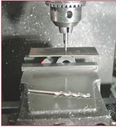
16 The RH leadscrew bearing being set up for drilling an oil way.
