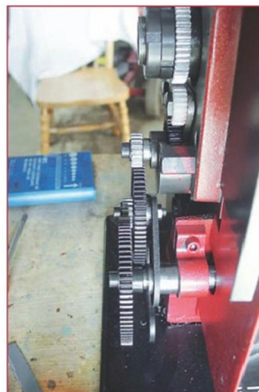
9 Showing the misalignment of the change wheels.
