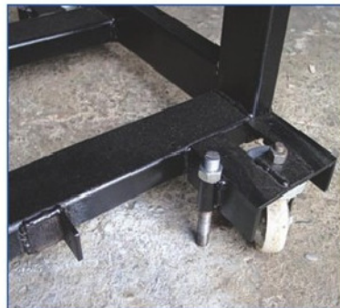
P04 Detail view of castor bracket and adjustable foot. Bracket for splashback is also visible.
