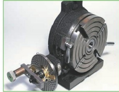
3 Commercial tables can often have a dividing facility added. It is though, usually supplied separately.
