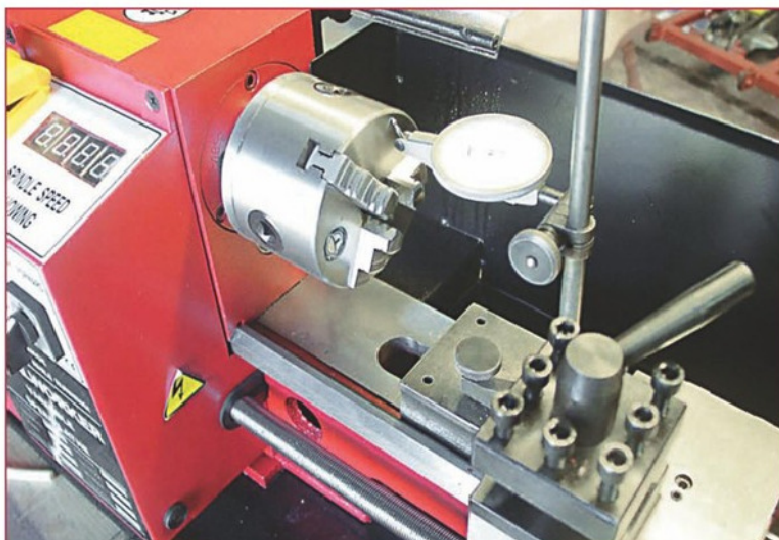
6 Set up to check spindle end float.
