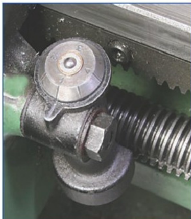
7 A thread dial indicator is required to ensure the half nut is closed at the correct position when screw cutting.
