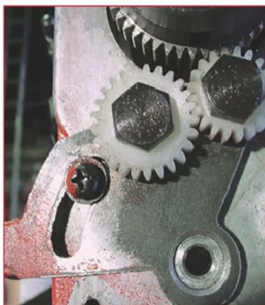
11 Showing clearance between larger white gear and washer.
