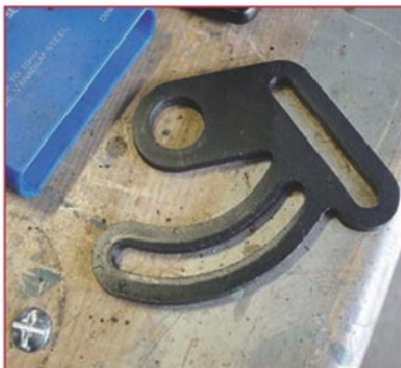
20 The tumbler bracket is a pressing with sharp edges on one face.
