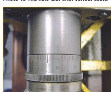
Photo 15 The new dial with vernier scale.
