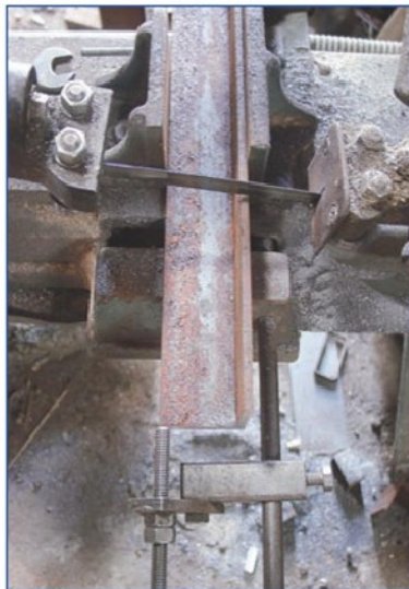
P08 Cutting material in the bandsaw, stop set to avoid jamming
