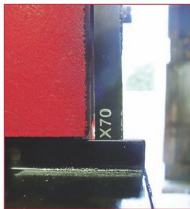
12 After adjusting the motor position, clearance has been gained between the belt and the headstock casting.
