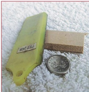
13 The diamond lap has been carved away at an angle to permit access to the root of the dovetails.
