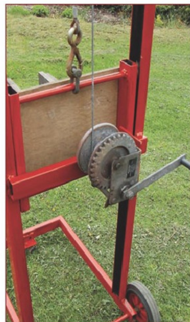
P6 A view from rear showing the winch. The plywood parts are also visible.
