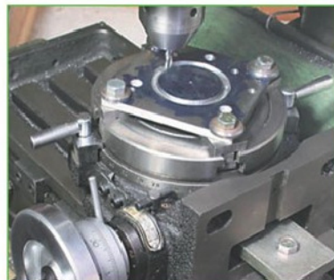
19 Rotary tables can be used to cut large holes and make large disks. This plate is for fitting to the rear of the chuck in photo 15 .
