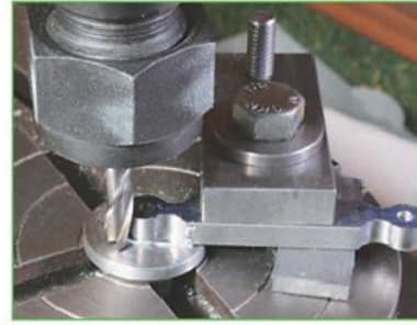
7 Machining a radius on both ends of a small crank arm.
