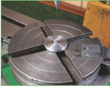
5 A locating plug with spigot that was used when machining the parts in photos 6 and 7.
