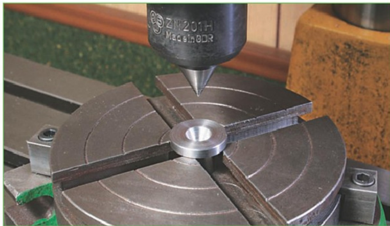
13 An alternative and potentially more accurate method of centralising the table than that shown in photo 12 .
