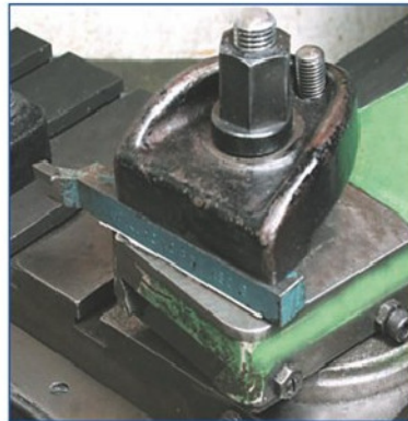
13 Not an ideal method, but mounting the lathe tool directly on the top slide will sometimes be necessary.
