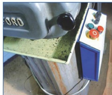
P07 Corner of tray roughly filled with weld then dressed off
