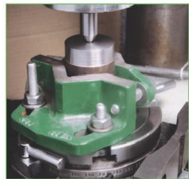
11 Positioning the workpiece for machining the hexagon seen in photo 4 .
