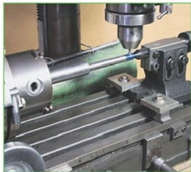
18 Using the rotary table in the vertical position, together with its tailstock.
