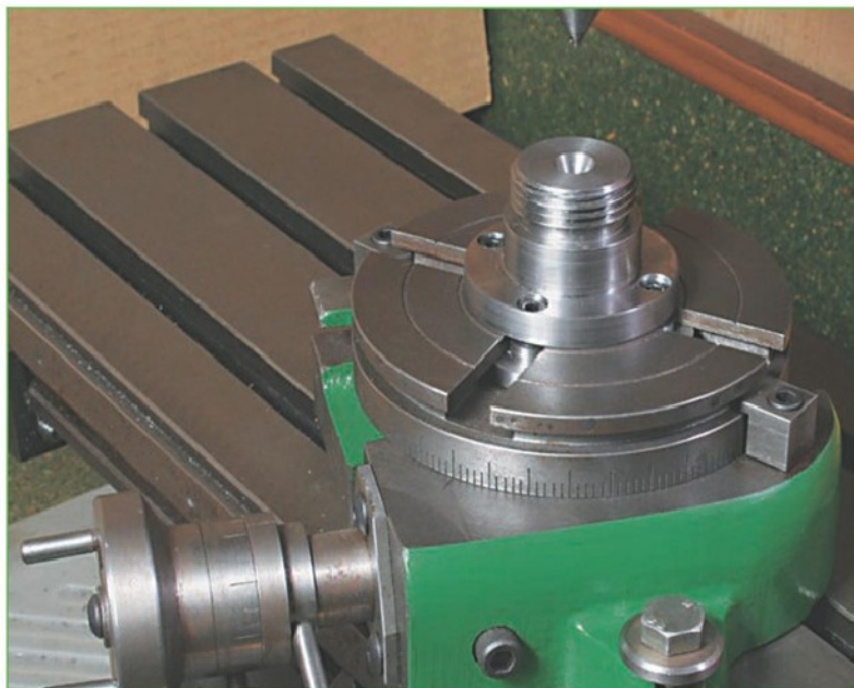
14 An adapter that replicates the lathe's spindle nose would enable a lathe chuck to be fitted.
