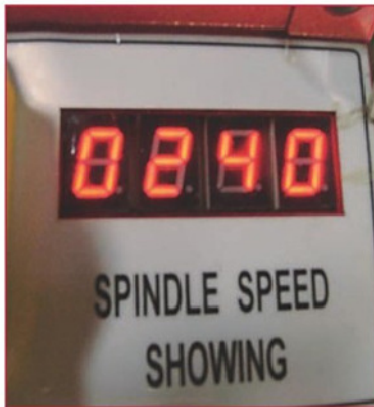
4 The tachometer shows the spindle speed.
