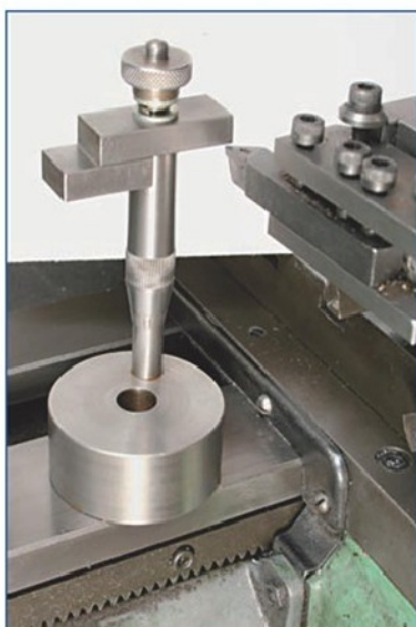
15 Setting the height of your lathe tool is quickly done with a calibrated tool height gauge.
