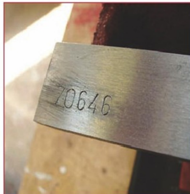
14 Raised metal around stamped numbers has been dressed off with lap.
