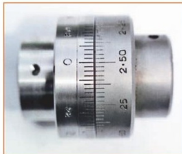
Photo 1 The original Y-axis collar (right) and the new easier to read version.
