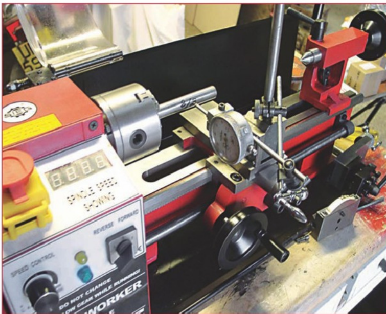
5 Checking headstock alignment and chuck run out.
