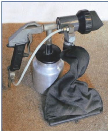
P09 Grit blast gun is fine for detail work but not for large areas
