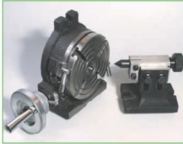
2 A 150mm diameter commercially available table.
