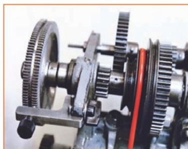
Photo 3 The Drummond lathe set up for direct indexing of 125 divisions.
