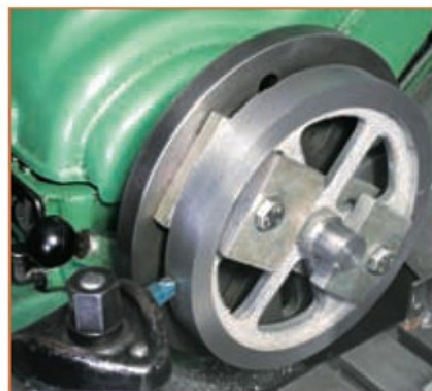
21 Carrying out the initial machining of the flywheel's outer diameter and the central boss.
