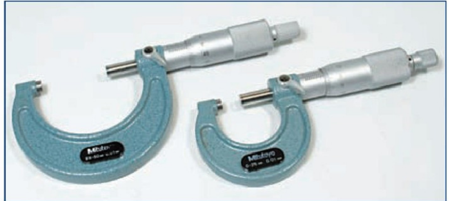
1. 0-25 and 25-50mm micrometer. Both are essential in most workshops.
