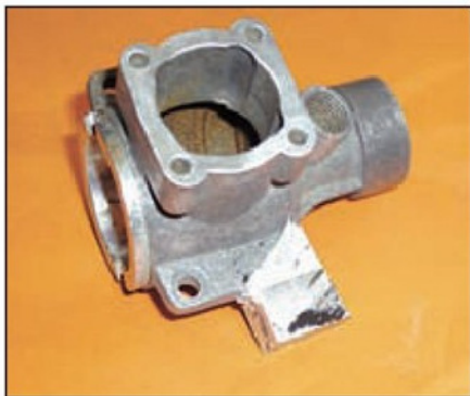
Photo 9 A solid bond has been produced. The replacement part is oversized to make handling easier.
