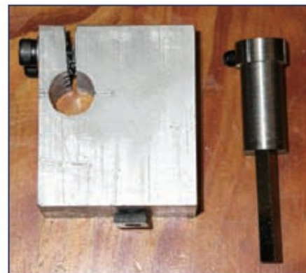
1 The crude boring bar holder and home made collet used to hold the HSS blank.
