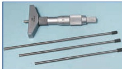
2. 0-100mm depth micrometer having interchangeable spindles.
