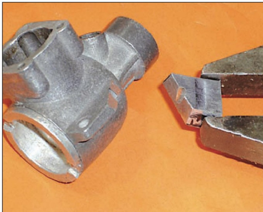
Photo 2 The mounting lug filed flat and a duralumin replacement prepared.
