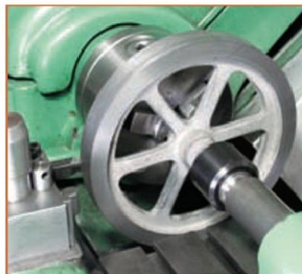
22 With the flywheel now held in the three-jaw chuck, the outer diameter and sides were finished to size.
