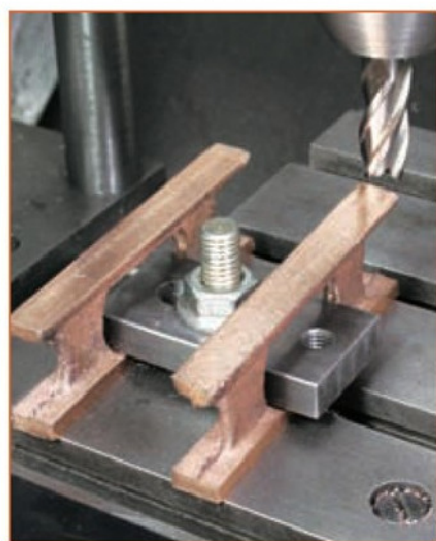
18 Two parts being machined at the same setting to ensure that they are exactly the same height.
