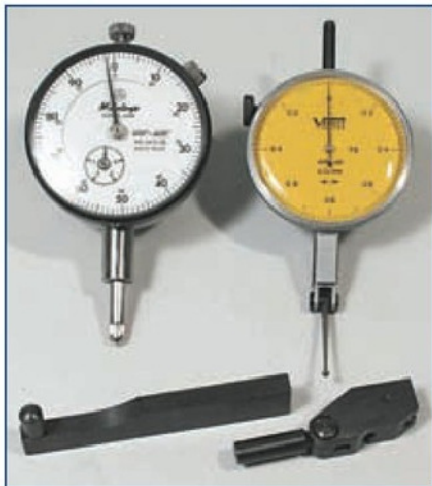
8. Dial indicator (left) and a dial test indicator (right) plus mounting accessories
