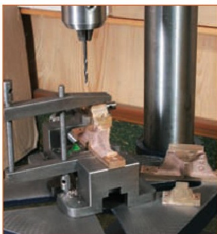
24 Drilling the bearing caps on the small drilling machine. Note that the vice should be clamped down.
