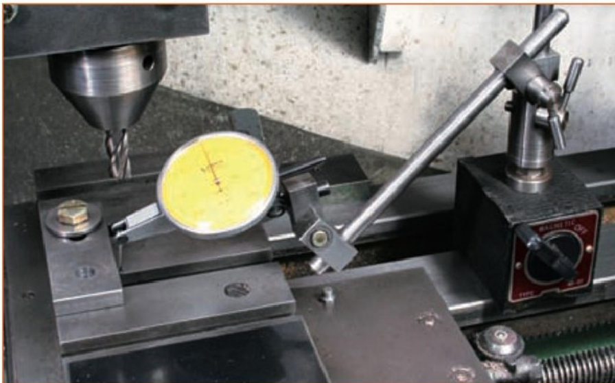
19 Setting a fence parallel to the cross slide traverse for machining the sides of the part as seen in photo 20.
