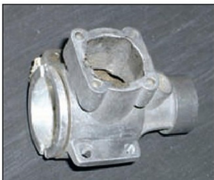
Photo 11 Sawn, filed to shape, and drilled, the repair is a success.
