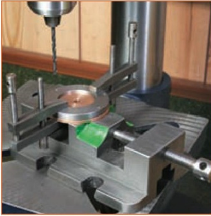
27 Using the drilling jig (Sk.1, last issue) to drill the cylinder end covers.
