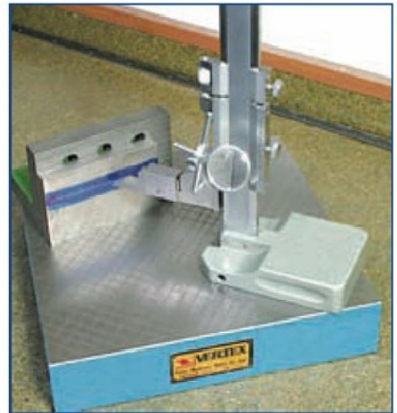
7. A Height gauge is able to very accurately mark out and measure items on the surface plate.
