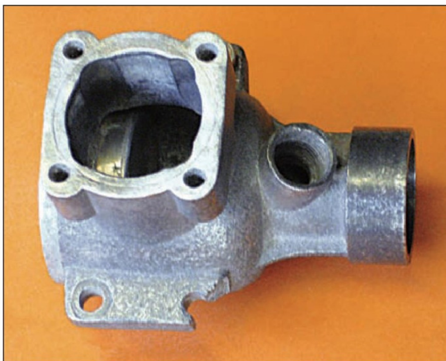
Photo 1 The patient, an Oliver Tiger crankcase with a damaged mounting lug.
