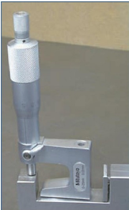
5. With the anvils removed the micrometer can be used for measuring steps.
