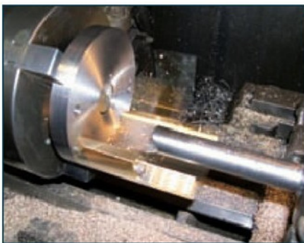
4 The fixture transferred to the lathe.
