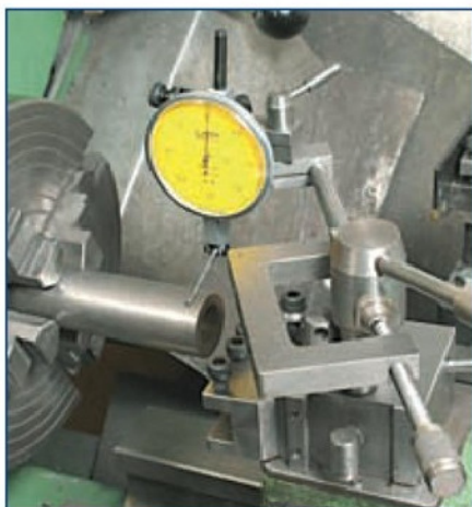
9. A DTI being used to ensure a component is running true in a four-jaw chuck.
