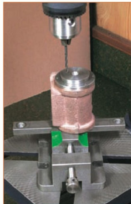
26 Using the drilling jig (Sk.1, last issue) with a location bung to drill the cylinder block ends.
