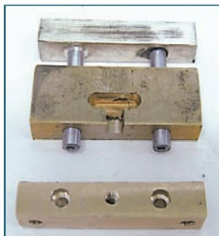
Photo 6 The polisher with the bars fitted.
