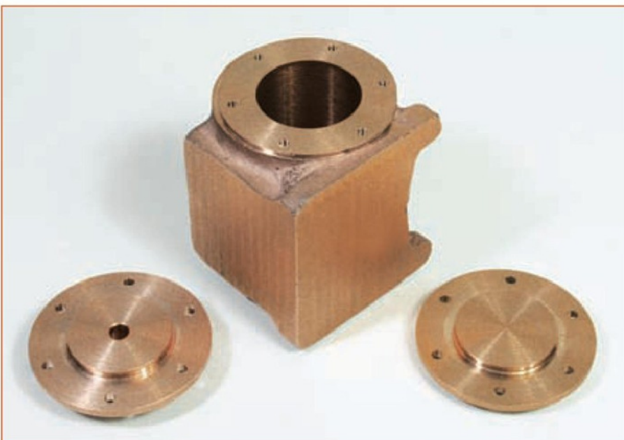
28 The cylinder block drilled and tapped for the end covers.
