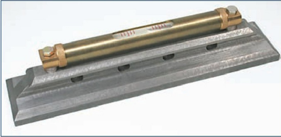
13. A shop made precision level, often quoted as necessary for the initial setting up of a lathe. However, alternative and simpler methods are equally acceptable.
