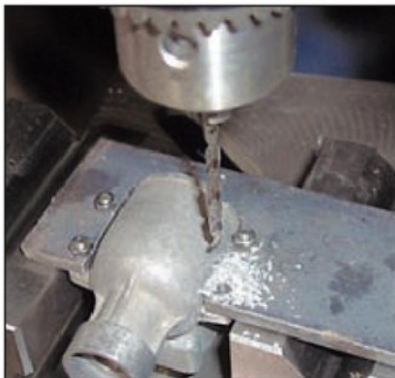
Photo 10 With the repair blended in, the bolt hole is drilled using a simple drilling jig.
