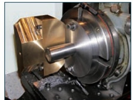
3 The fixture mounted on the rotary table.
