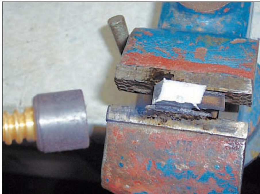
Photo 7 Likewise the replacement is "tinned". Note the plywood pads to insulate the work from the vice jaws, now somewhat charred.
