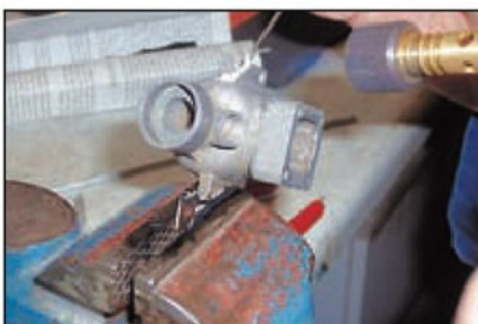
Photo 6 The surface is abraded through the molten weld using the stainless rod.
