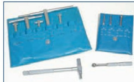
12. These gauges are used in conjunction with a micrometer and or a calliper to measure internal dimensions. Those on the left up to 150mm and on the right 13mm.
