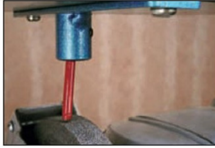
Photo 9. The dresser in position over the grinding wheel.
