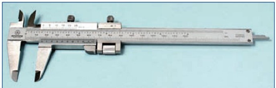
6. For many years, the Vernier calliper has been the normal method for measuring larger dimensions, say 50mm plus, but has largely been replaced by its digital counterpart.
