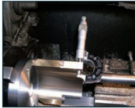
11 Measuring the inside diameter.
