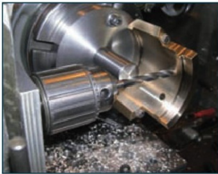
13 Drilling the holes.
