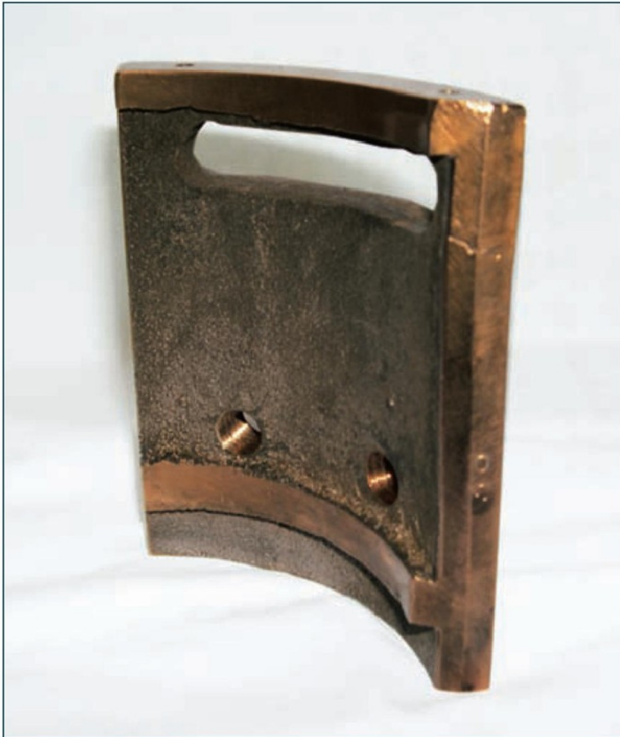
1 The original cracked casting.
