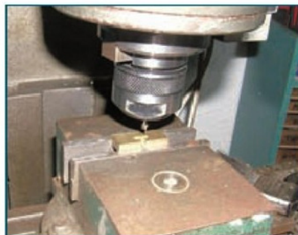
Photo 2 The slot for the steel insert being milled.
