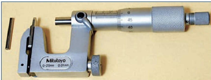
4. A multi anvil micrometer.
