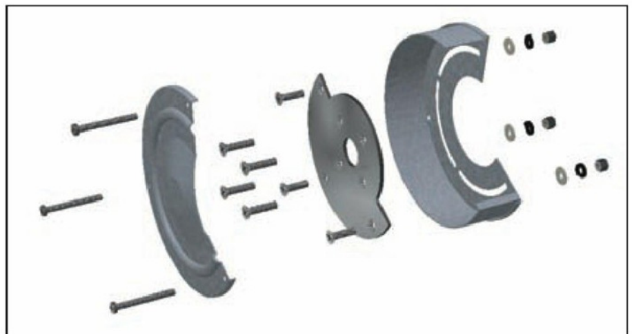
Figure 2. Exploded view of the modified left-hand wheel guard
