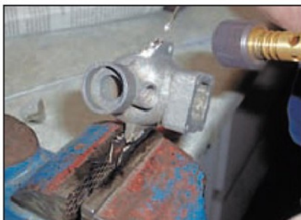
Photo 5 The mating surface "tinned".
