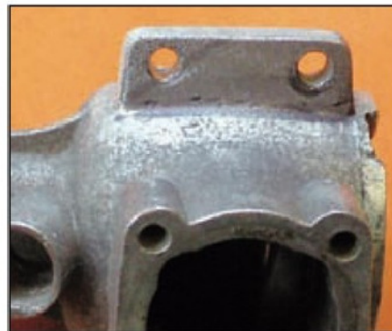
Photo 13 Disguised, the finished repair almost disappears.
