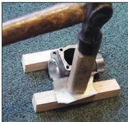
Photo 12 To match the repair with the crank case shot blast finish, I used sand paper tapped rough side down on the shiny surfaces.
