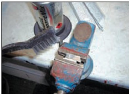
Photo 3 The mating surfaces are cleaned using the stainless steel brush provided in the kit.
