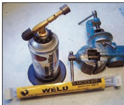
Photo 14 The basic requirements for weld-aluminium at low temperatures.
