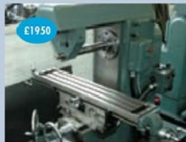
Tom Senior Major / horizontal + powered swivel table to cut bevel gears
