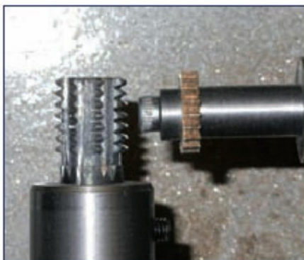
7 The cutter and the wheel blank set up in the wheel-cutting engine.
