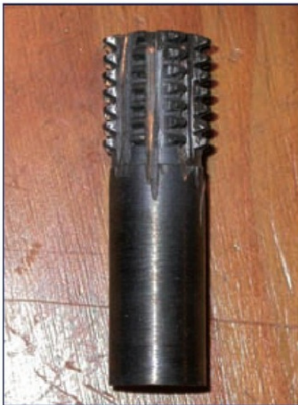
6 The cutter after "gashing" with eight longitudinal cuts.
