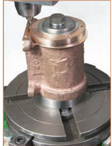
30 Two complex milling operations on the cylinder block using a rotary table that clearly shows the extent of tasks that can be carried out using the milling head.
