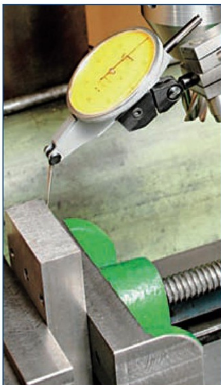
10. A DTI can ensure a workpiece is parallel with the milling machine's table traverse.
