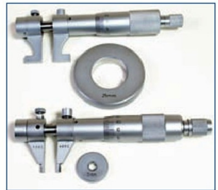
3. Inside micrometers are also very useful. These are 5-30mm and 25-50mm sizes.
