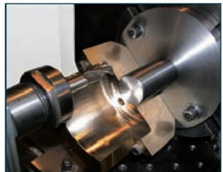
9 Rough milling the inside radius
