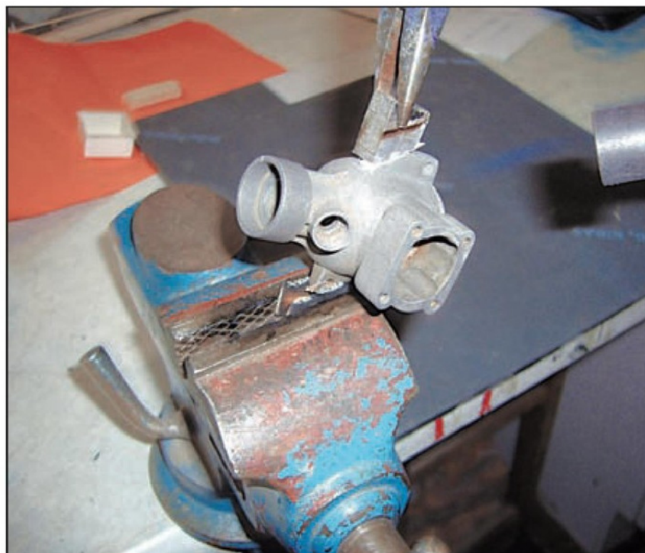
Photo 8 Both parts are brought up to temperature, and then held together while the temperature is allowed to drop.
