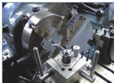
5. Card packing protects the aluminium in the chuck.
