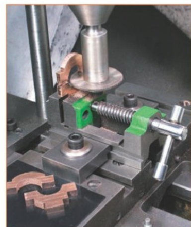
14. The slitting saw being used to split an eccentric.
