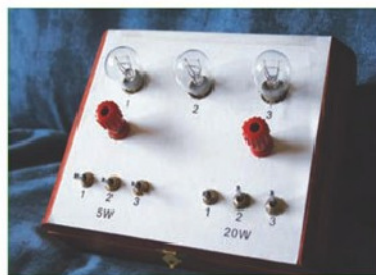
9. A suggestion of how a current control with light bulbs can be made
