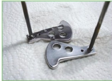
4. The part in the back is not cleaned well enough. The water stays on it in beads.
