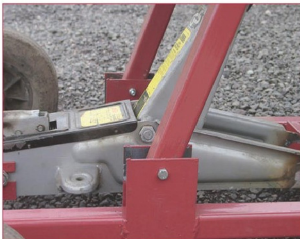
9. Alignment of lower pivots with jack arm pivot.
