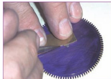
4. Marking the second side of the spoke.
