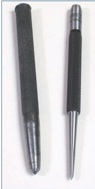
6. Standard centre punch, left with spotting punch on the right.
