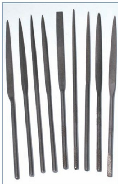
2. Needle files are essential for detailed intricate detailed work.
