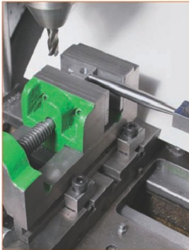
9. The vice mounted in line with the cross slide for machining the end of the connecting rod.
