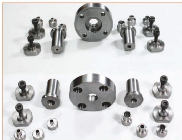
3. The parts that make up the workpiece locating jig, Sk. 3. A mirror has been included so as to see the bore and locking pin in the upper plate.
