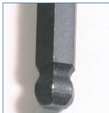
5. Ball ended hexagon wrenches are much easier to use than the more normal type.
