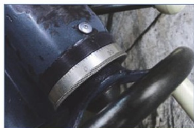
2. Indexing ring fitted to Chipmaster tailstock.
