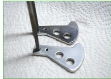
5. Etching in lye takes away the shine but cleans the part very well.
