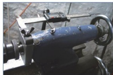
4. The depth rod interferes with the hand wheel.
