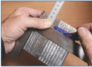
10. Marking out with a hand held square.
