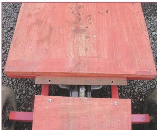
4. Attachment angle for access ramp – also shows the ramp detached.
