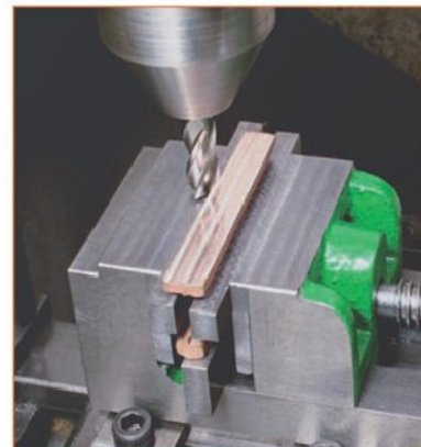
8. A toolmaker's style vice gives greater flexibility in positioning compared to vices with fixed clamping points.
