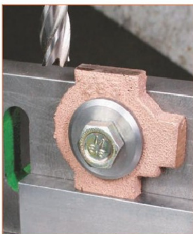
12. Machining the two sides of the eccentric outer bearing ensuring that they are parallel so that they can be held in the vice.
