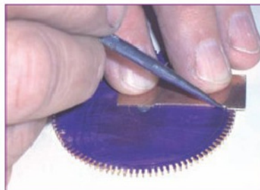
3. Marking the first side of the spoke.
