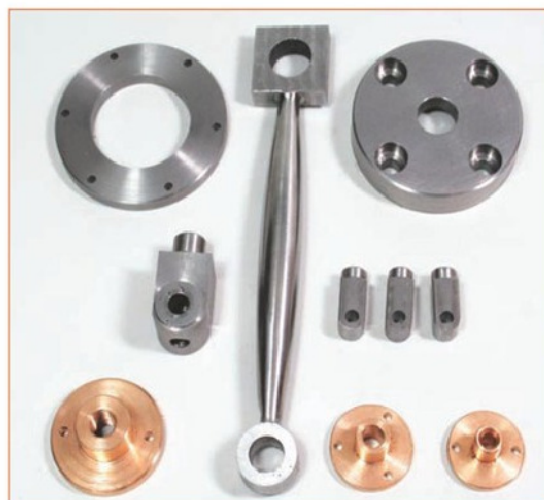
4. Items that were made using the rotary table.
