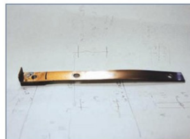
8. Copper strip folded with added 3mm part.
