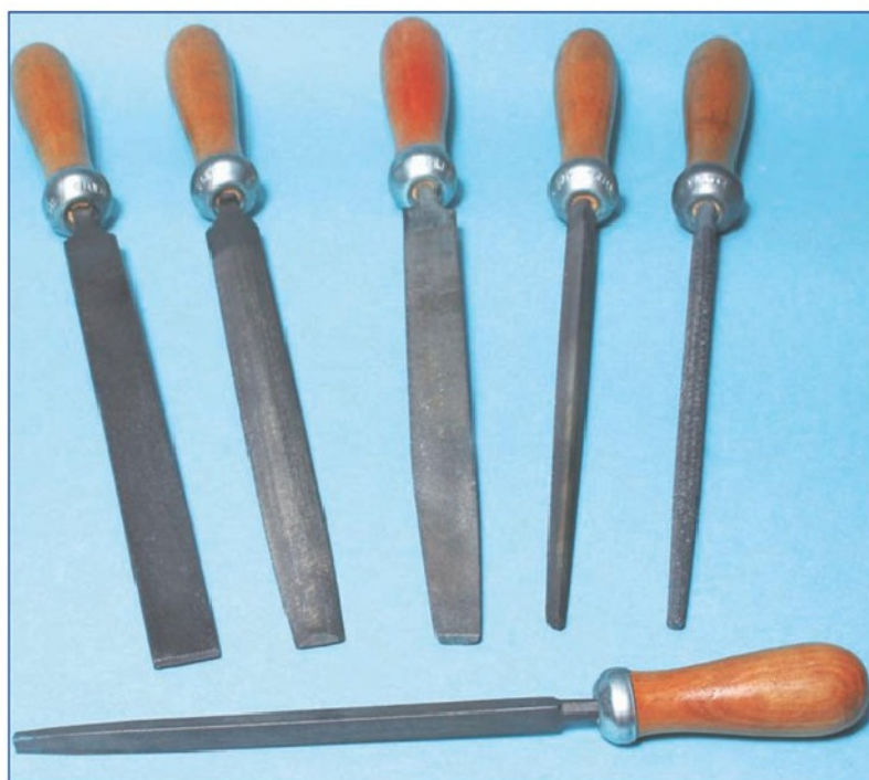
1. The six most common file types. Left to right they are Hand, Half round, Flat, Three square, Round. A Square file is at the front.
