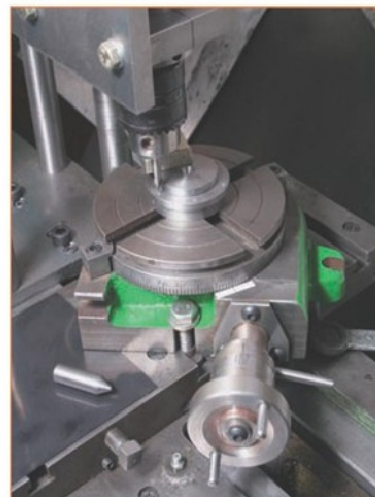
2. Six holes on a PCD being positioned using a rotary table. The item being made is the drilling jig (Sk. 1)
