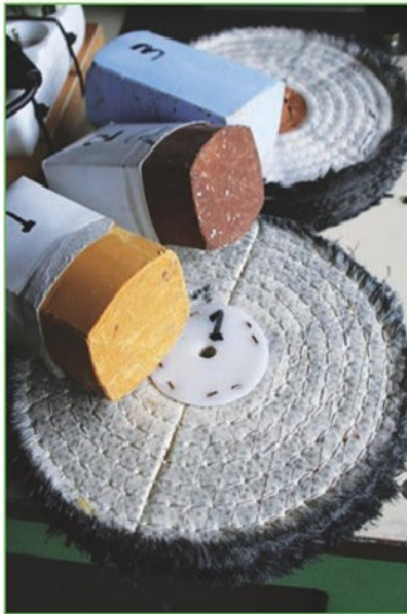
3. Some of the compounds used in buffing. From coarse (1) to fine (3).
