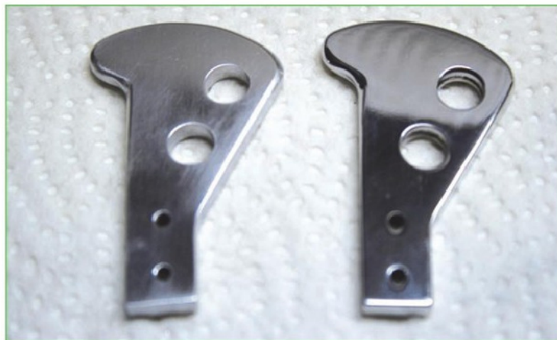
1. The part on the left is sanded, the one on the right buffed.
