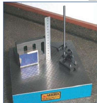
13. Using a surface plate and surface gauge for marking out. Where complex shapes are involved, this is the only practical method.
