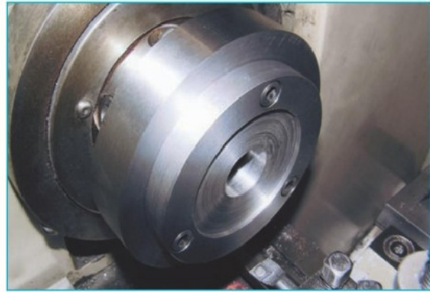
5. The register machined ready to take the chuck adaptor.
