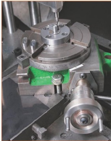
5. Creating a radius on the end of a small link using the rotary table to establish the radius and the workpiece locating jig to position the part.
