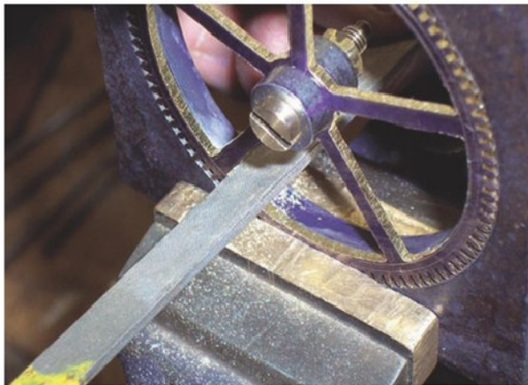
13. Filing the periphery from left to right.
