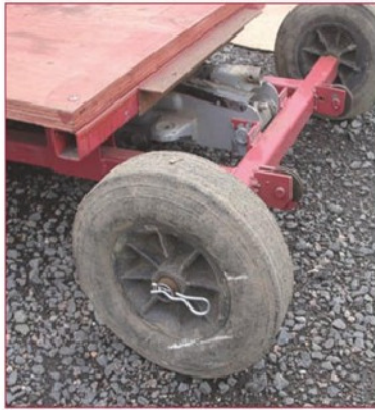
6. Large detachable wheels make for easy moving.
