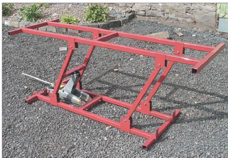
1. The completed framework for the bench.
