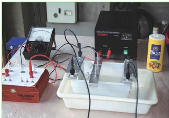
11. Setup with current control and analogue ammeter.
