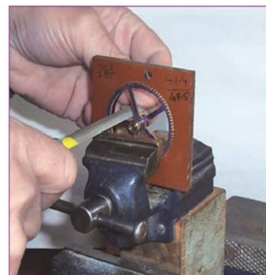
12. Filing the crossing.
