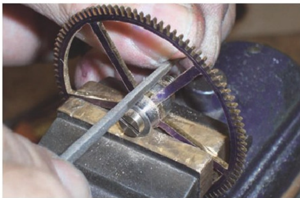
15. Filing the hub.
