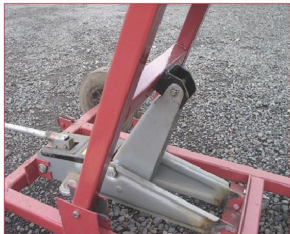
10. Contact between jack arm and rear lever arm.
