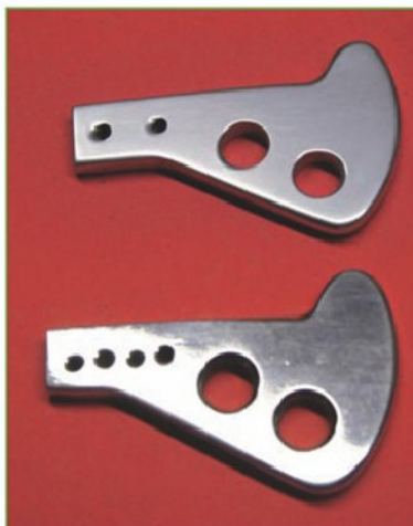
14. The difference in aspect between an anodised and sealed part and one that's just "bare".
