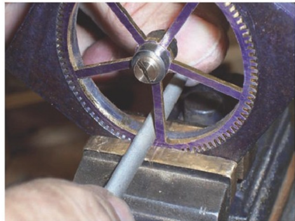
14 Filing the periphery from right to left.
