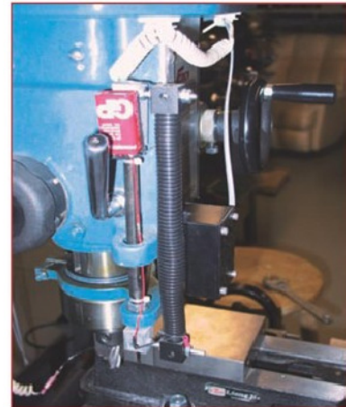
6. The battery showing the wires running down to the resistor and the LED.
