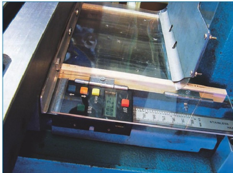
6. This shows the aluminium angle and the metal shields.
