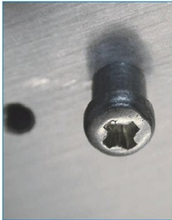
9. A crosshead screw and turned sleeve serve as the ball-ended post.
