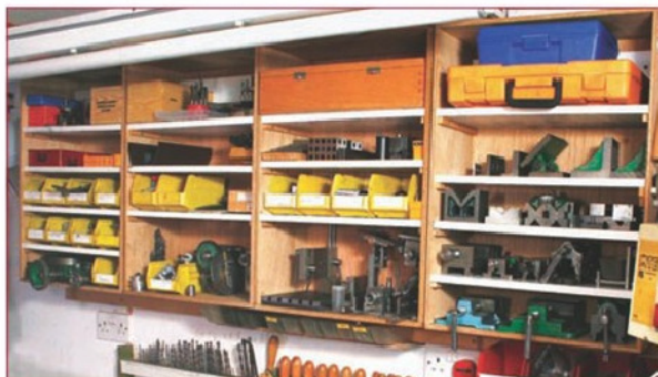
5. The main frame of one end of this shed has been made from 144 x 18mm timbers providing an ideal method of supporting shelves
