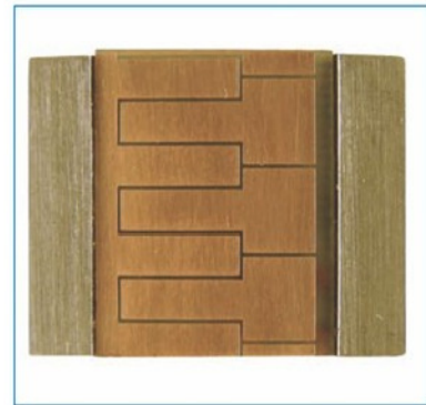
16. A short section of the printed circuit from inside a scale.
