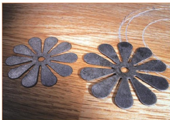
2. Petals for pulse jets produced by water jet cutting
