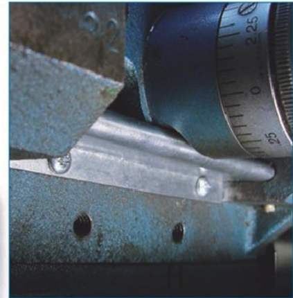
10. The bearing housing needs some clearance.
