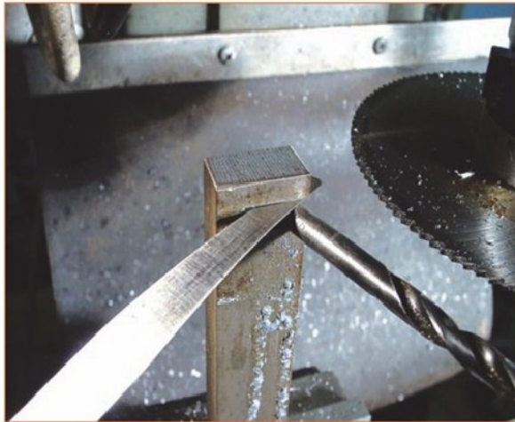
7. Checking slot width with a drill and a feeler gauge.
