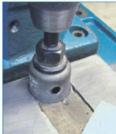
7. A hole saw is used to extend the slot for the cross axis leadscrew.
