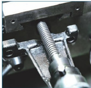
9. The cross slide feed screw needs disconnecting if you are using the taper turning attachment.
