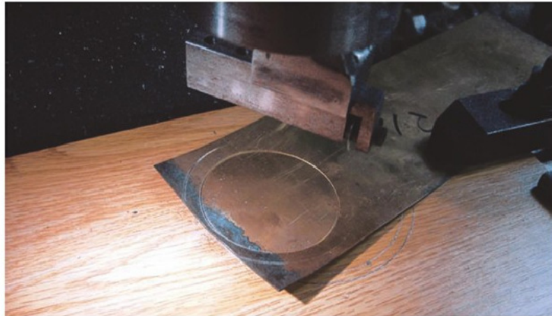
5. Partway through cutting a brass component, note the edges have risen.
