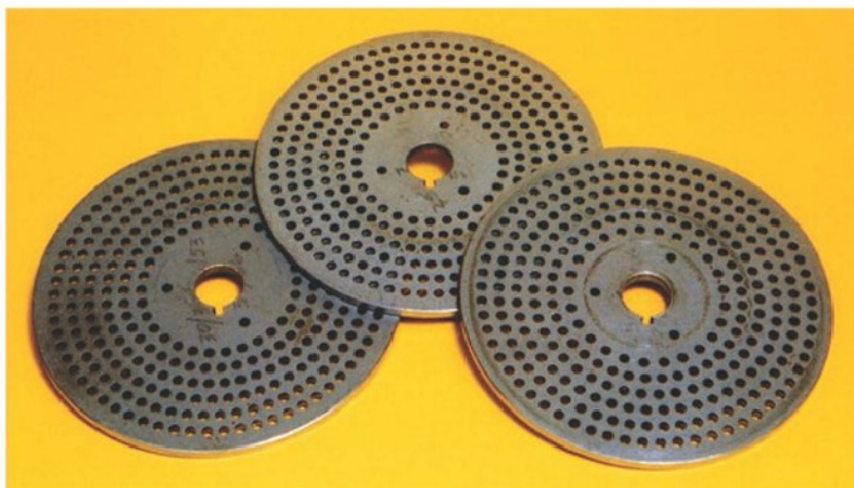
1. This set of three dividing plates, each with 6 rings of holes, give 18 different hole numbers.
