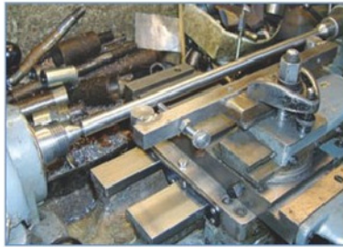
4. Setting the sine bar true with the centres bar.
