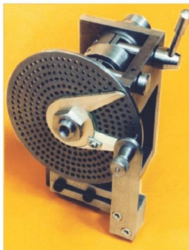
6. A dividing head set up for direct dividing, that is, division plate mounted onto the head spindle.
