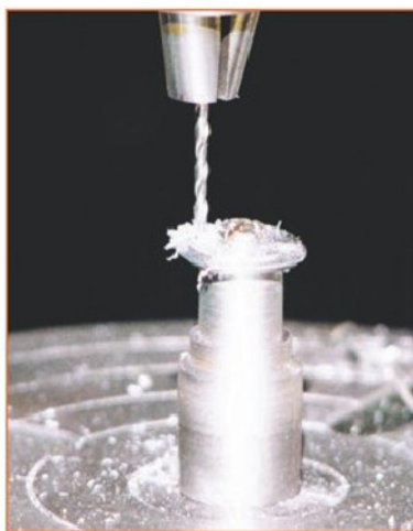
7. Drilling the stress-relief holes.
