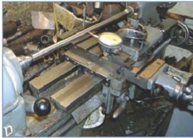
3. Clocking the bar to ensure tailstock and top slide are set true.
