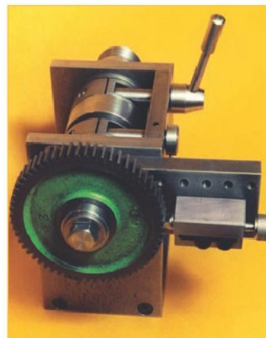
7. A dividing head set up for direct dividing but using a gear to set the divisions.
