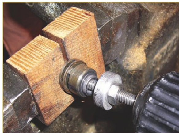
5. The bore lap is put to work. The cylinder is clamped between shaped wooden blocks.
