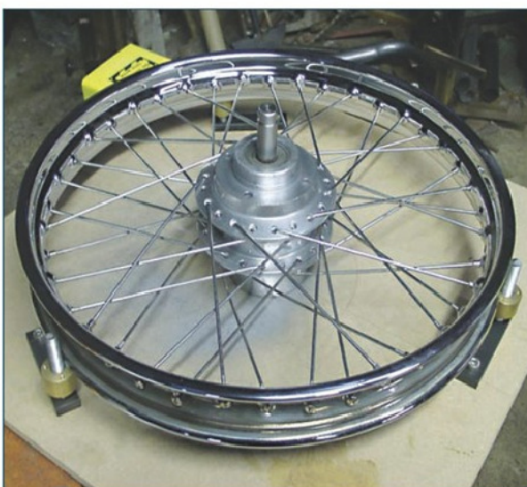
12. Hub, rim and spokes assembled in the jig.
