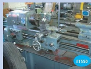
Harrison L6, 6" x 24" geared head lathe, gearbox, power cross feed in very nice order
