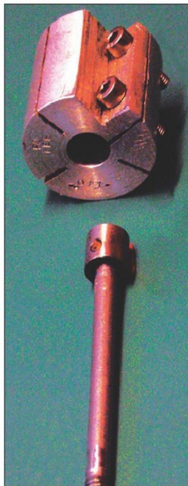
8. A piston mounted on its shaft ready for lapping in a piston lap.
