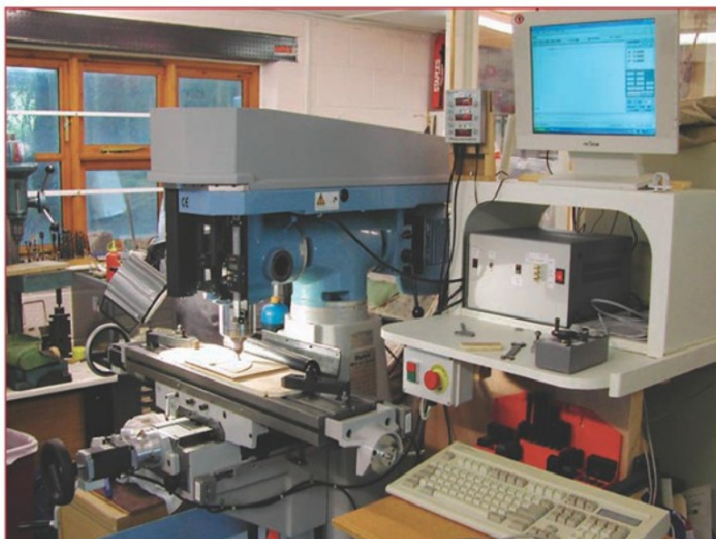
1. The milling machine complete with fabricated cover testing a CNC routine on some MDF.
