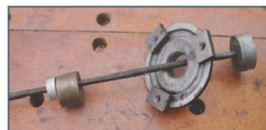
8. Tie bar assembly to retain disc in chuck.
