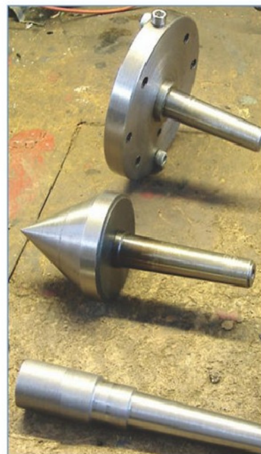
7. Some finished tapers.
