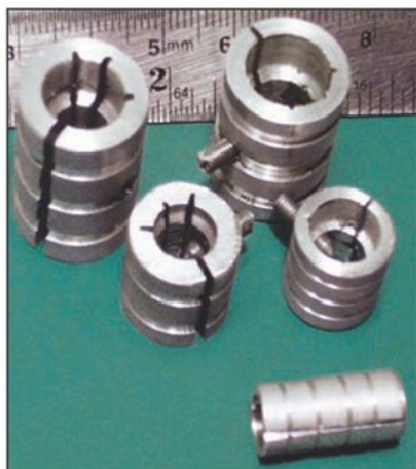
6. A selection of bore laps for engines of different sizes.
