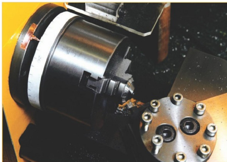
5. Another method of making the divisions on a dial using a marked strip of paper on the chuck's backplate.
