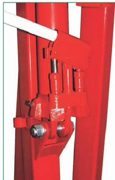
6. Detail of two rams on engine lifter.
