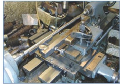
5. The sine bar and cross slide with packing in place.
