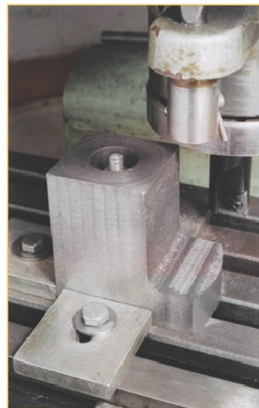
11. Surfacing the top of the foot for the fixing nuts.
