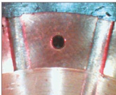
22. Alignment to a hole on a plain brass work piece.
