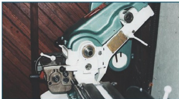
46. The tailstock end of the newly painted lathe, partly assembled. The stage when this photo was taken was the second milestone in the renovation work on it. However, the belt guard was not yet properly fitting - - -
