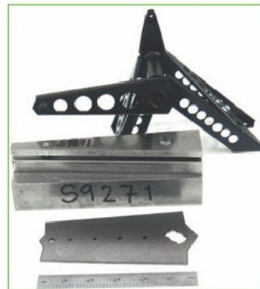
2. (right) Blank, form tool and fabricated assembly.
