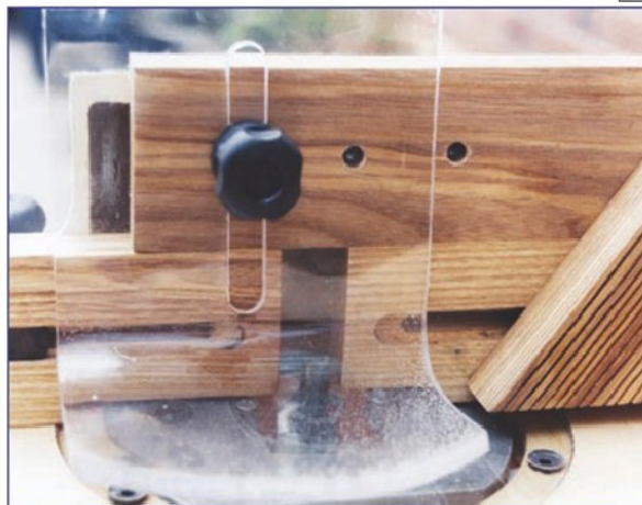
15. Infeed fence has vertical extension to carry feather board and safety screen.
