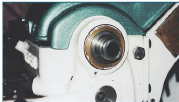
47. - - - as can be seen in this photo, where the cut-out at the front over the front mandrel bearing housing is fouling it, preventing the guard from properly closing down on to its PVC buffers. The cut out on the other side was clear.
