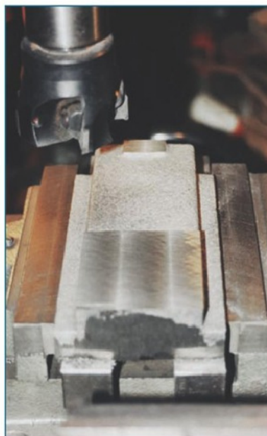
37. Machining the tool platform on the top slide casting.
