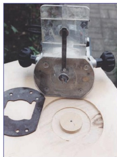
6. Circle cutting base fitted to router - resting on test piece.
