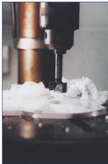
8. Boring polycarbonate sheet with Forstner bit.
