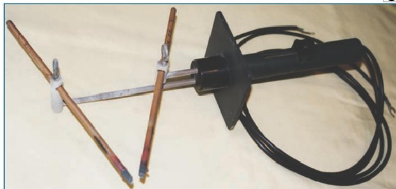
52. This is the commercially made carbon arc brazing unit. The rod to which the left carbon electrode is attached is gradually moved towards the other carbon electrode as the two are consumed by equal amounts.
