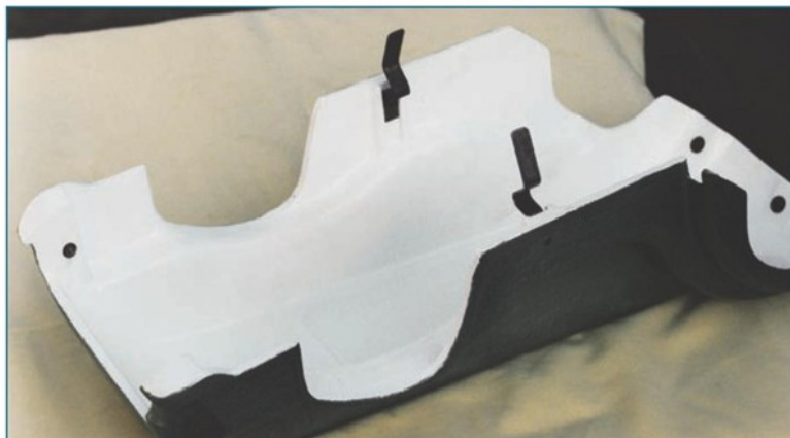
45. The belt guard required the cutouts nearest the camera to be built up and smoothed to remedy the rough way that they had been enlarged with a hacksaw, as was shown in Photos 17 & 18. This photo shows it after painting.
