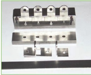
3. Form block allowing four components to be handled together.
