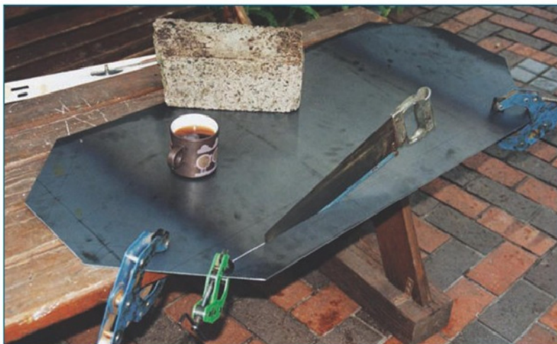
49. The 2 mm steel plate for the cabinet tray is shown partly cut. The reader's attention is drawn to the very hi-tech anti-vibration methodology applied to facilitate hacksawing – thus there's the broken concrete block and the crab clamps at each end of the steel plate to attach it firmly to the rustic garden table.
