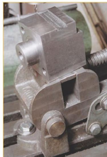
15. Creating the dovetail edges to take the parting off blade.
