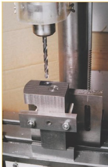
12. Drilling base and turret for the locating plunger.
