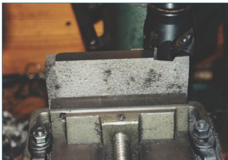
38. Machining one of the edges on the top slide casting.
