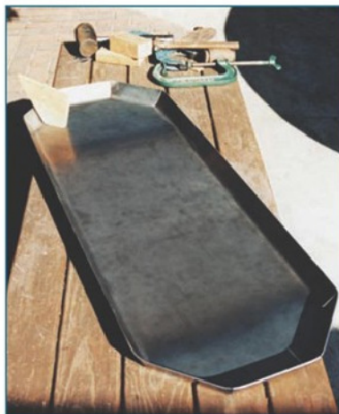
50. The cabinet tray with the edges bent to their required angle, and the corners at the eight butt joints slightly rounded for appearance and to close up the butt joints.
