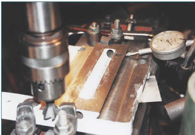
43. This photo shows the apron mounted upside down on the mill/drill table and how it was set truly square, using the dial gauge along a vee way as a datum. A straight edge was first placed along the vee groove to check that it was straight, and hadn't been worn to an uneven shape. It hadn't been. The vees were very lightly skimmed with the dovetail cutter, which was lowered sufficiently to provide clean surfaces to an identical depth on both sides, against which the top slide bears. The part-circular marks from the dovetail cutter can just be discerned on the right. The width of the slightly depressed re-machined surfaces were made slightly wider than the corresponding surfaces on the new cross slide.
