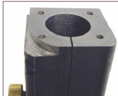
8. The guide is relieved by filing to give clearance for the fork.
