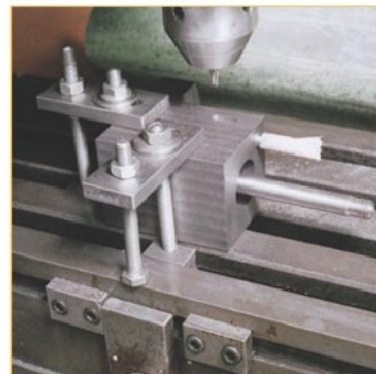
13. Milling the slot for the locating plunger handle.
