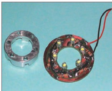
17. Assembled Circuit Board: note that the components are mounted on the copper track side of the board.
