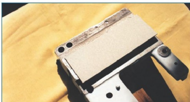
42. This photo shows the upper face of the apron. The original machined surfaces on both sides of the veeway along which the cross slide engages had both been quite badly worn below the original level. The surface on the headstock side – ie with the two slotted screws in the mounting holes for the travelling steady – had the worst wear, which can be discerned in the photo. The piece of cardboard is obscuring the apron on that side closest to the camera – there was some reason for putting it there for the photo, but I can't remember why!
