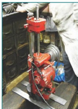
The BUMA boring machine in action.
