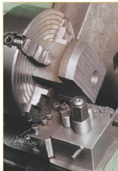
9. The front of the casting's foot can, if you wish, be machined at this stage.
