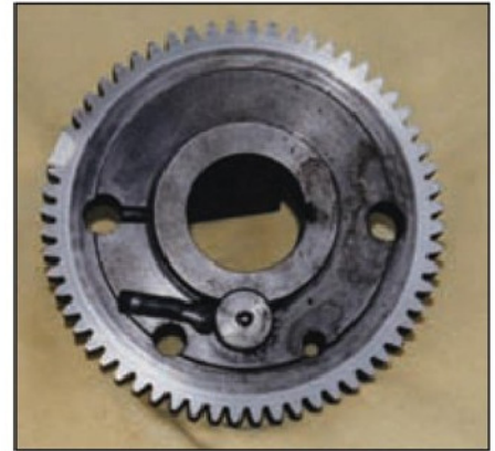
15. The 60T bullwheel showing the repair fillet machined to the wheel profile. But the two 5/16in. diameter holes should be noted - what are they for if not to fit a short bar with two pins...
