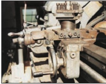
4. A close-up of the lathe carriage. The base of the 4-way tool post can be seen welded to the cross slide. The end plate (or extender bracket) supporting the cross slide handwheel is clearly non-standard. There is no thread dial indicator, and the knob on the carriage handwheel is definitely non-standard. The cross slide looks rusty - it sure was.
