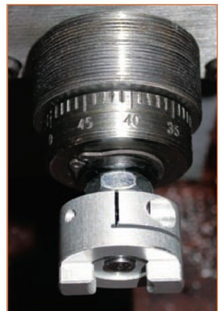
6. Part reassembled with half of coupling in place.
