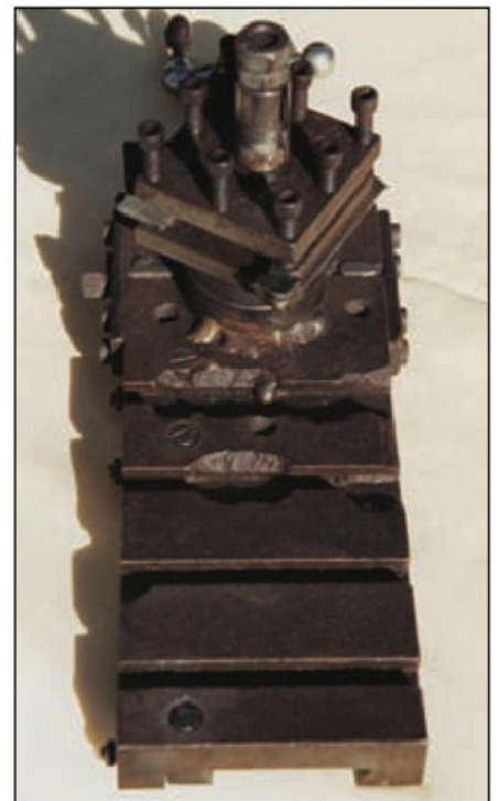
13. This photo shows very clearly the brazing of the base of the 4-way toolpost on to the top of the cross slide; the badly damaged tee-slots; and the brazing across the top on both sides of the toolpost. The two strengthening plates can just be seen on both sides of the cross slide.
