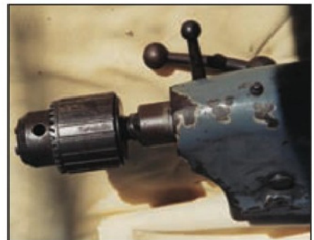
8. The front end of the tailstock showing the drill chuck No.2 MT arbor actually brazed both to the tailstock barrel and to the drill chuck. If the tightening lever looks slightly bent towards its boss end, in fact it is. One of the half dozen unceremoniously hacksawn graduating marks can be seen on the barrel.
