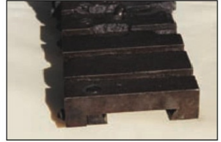
11. I have included this photo, and the next three, to show how a vital part of a lathe can be mutilated beyond recovery – viz the cross slide assembly. The cross slide is shown the from its rear end, with a vee undercut at the normal 60 degrees on the RHS, but that on the LHS is machined at a right angle: this the normal Myford procedure. The thick two-piece gib strip is attached to the body of the cross slide with four screws.
