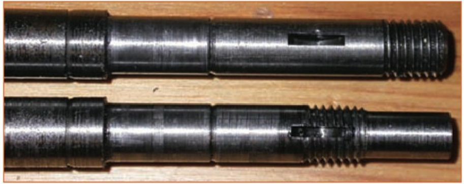
5. Before and after remachining the lead screw.
