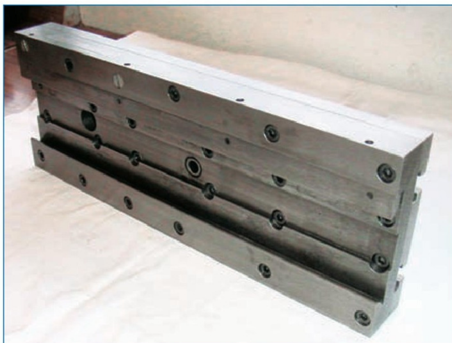
11. Underside of cross slide showing attachment bolts for steel strips.
