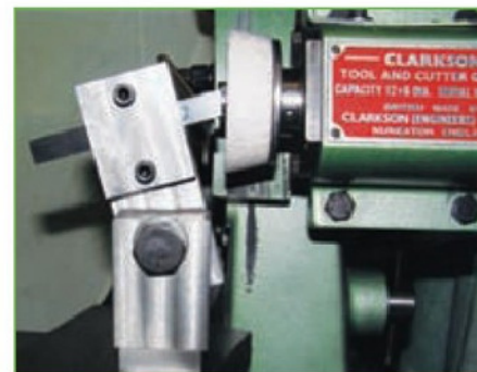
14. Fixture specifically for parting blades. That shown is a Churchill Emperite, which is ground only on the end.
