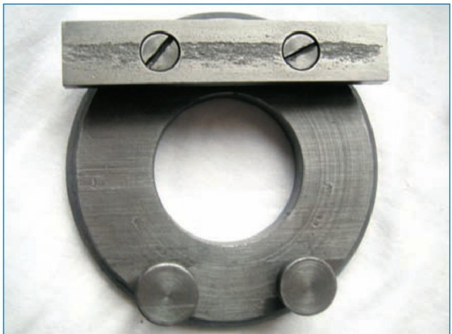
9. Underside view of annulus showing T bars.
