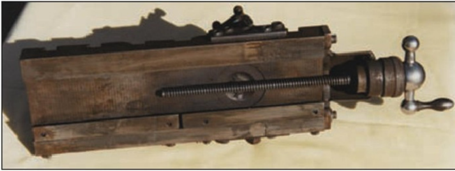
14. The underside of the standard Myford Super 7 cross slide is shown in this photo, fitted with the standard thick gib strips in two halves, which are bolted to the slide from the upper surface. The gib strip is in two halves because a single strip this thickness would not be satisfactorily flexible along its whole length to give the right "feel" for the movement of the cross slide over its whole travel - it would, in fact, be impossible to adjust it. Two brazed repair welds can be seen. A total break occurred across the casting at the point where the holes are drilled on either side and tapped for screws that tighten brass locking thrust pads against the topline spigot. Although the feedscrew assembly is complete, the end plate is an amateurishly made replacement. The Acme thread had been damaged at one point, not shown in this photo. Also the graduated end of the micrometer dial had been damaged by grinding.
