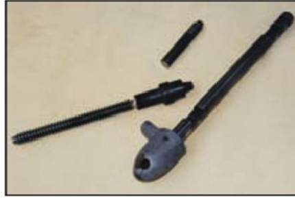
10. This photo shows the remodelled feedscrew for the topslide on the LHS, which had yet to be completed at the time this photo was taken. Also shown is the camshaft lever (for releasing the drive belts) with its lever arm missing. A crack can be seen at the tip of the CI end fitting, and also a piece of metal has been broken from the edge of the hole which takes the handle shaft.
