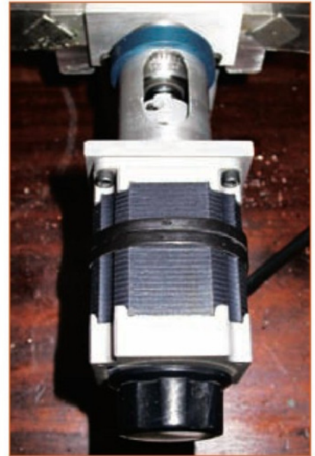
8. Motor refitted now driving through Oldham coupling.
