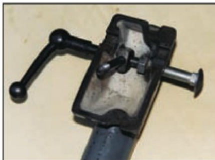
7. This view of the underside of the tailstock body shows how the eccentric arbor was pushed through the distorted slot in the eyebolt using a coach bolt. Although, initially, turning the nut to tighten the coach bolt against the arbor and the other side of the tailstock casting didn't move the latter through the slot in the eyebolt, a light tap on the head of the bolt soon shifted it, albeit by a small amount. This procedure was repeated until the arbor was clear of the eyebolt. Doing the job this way avoided having to apply any potentially damaging impact force on the casting. Another, minor, problem was the tight fit of the arbor in the hole through the rear of the tailstock casting - seen on the LHS in this view.
