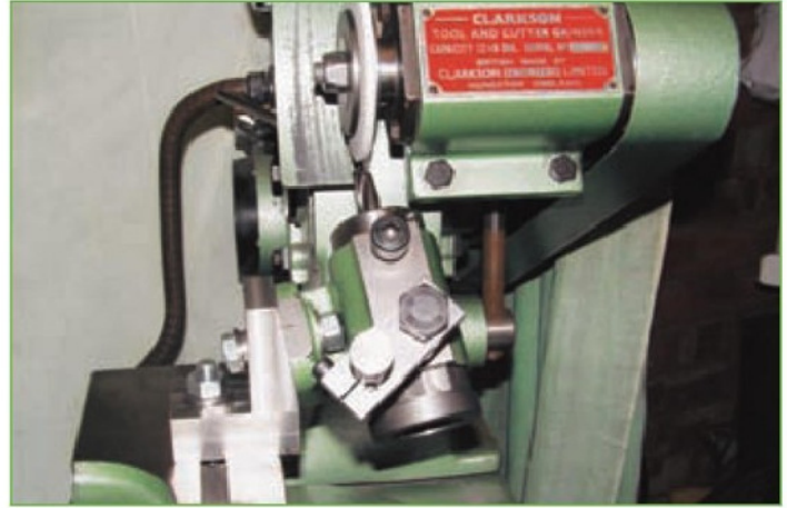
5. Set up for reforming end teeth on slot drill.
