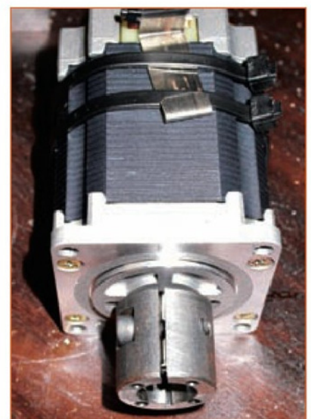
3. Four holes can be seen in the end of the coupling.
