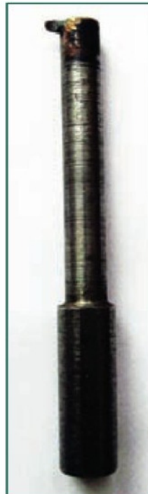
5. A small boring bar made by silver soldering a short length of carbide rod.
