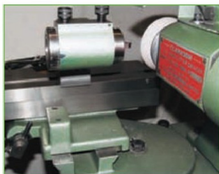
12. Protractor ring permits accurate control of angles on part off or grooving tool.
