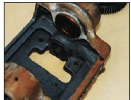
16. ...for engaging with the protrusion seen in this view inside the headstock casting just in front of the RHS mounting hole in the base when loosening a tight chuck? This would presumably save a high force being applied to the Woodruff key in the vee cone pulley when releasing a tight chuck, or would it smash the gearwheel against its key to the lathe mandrel? Maybe the wooden wedge idea is the best of all for avoiding tooth damage, but it still wouldn't help the Woodruff key for the gearwheel.
