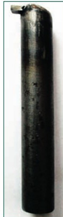
6. A boring/grooving tool which uses a recycled parting off insert.
