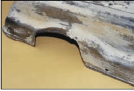
17. Headstock belt guard showing the clearance cut-out for the swing arm casting on the RHS from the front, which has been very roughly increased in size.
