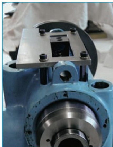
2. The Z axis mounting plate at an early stage, with quill in situ, and linking block in place.
