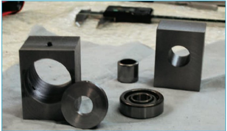
5. Top bearing housing (left) showing the spacing collar and grub screws used to locate it prior to fitting dowel pins. The bottom bearing housing (right) was bored to take the needle race as a light force fit.
