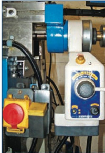
3. Power feed and starter colliding.
