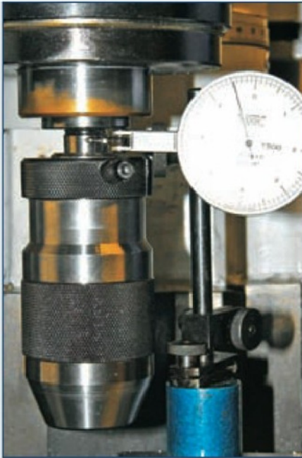
11. Checking keyless chuck taper adaptor run out.
