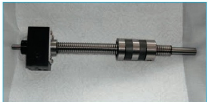
7. Ballscrew and nut with top bearing in place. Note the PTFE sheet swarf shield screwed to the RH end of the bearing block.
