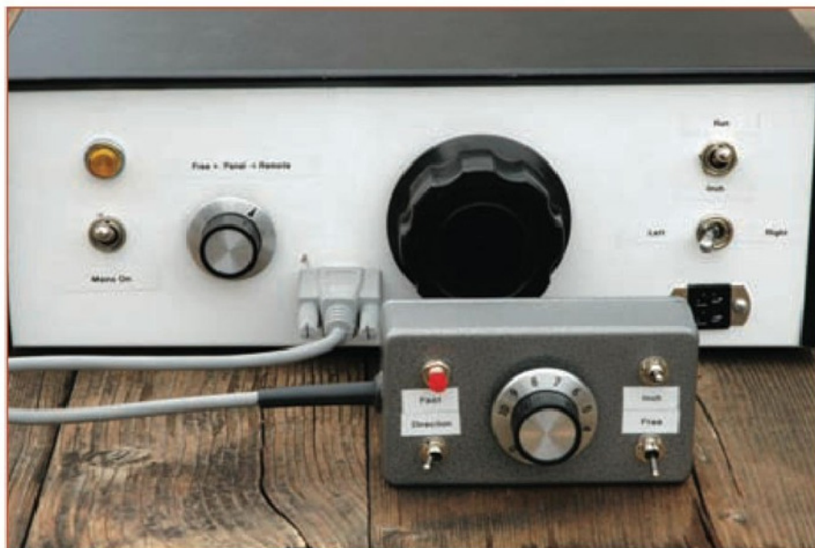
1. Completed unit with hand held box in foreground.
