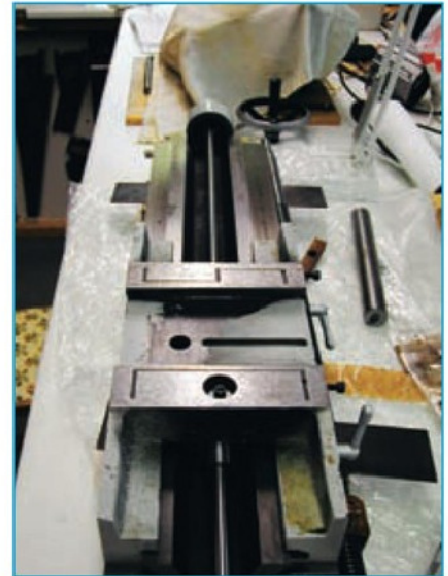
13. Showing the oil channels on the underside of the Y axis slide.
