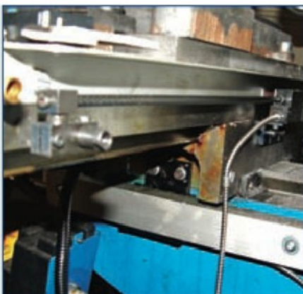
5. X-Axis linear encoder mounted on the back of the table.
