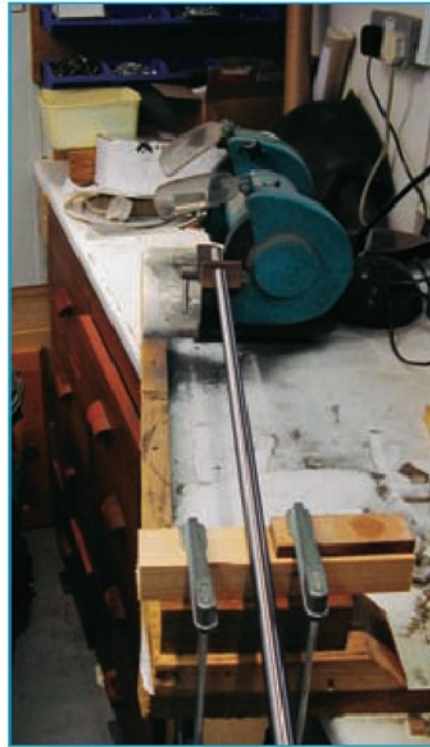
9. The setup used for grinding the hardened skin off the ends of the feedscrews. The wooden blocks in the foreground provide location. A wooden collar abuts the rest on the grinder and controls the length ground.
