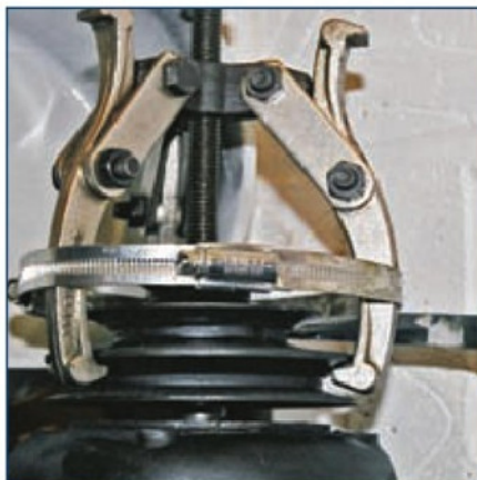
8. Lifting the motor pulley.
