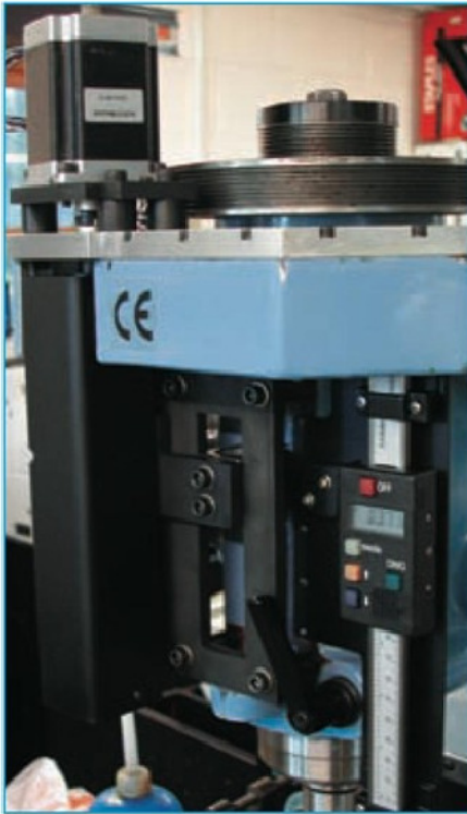
8. All the Z axis parts in place, complete with swarf shield and DRO.
