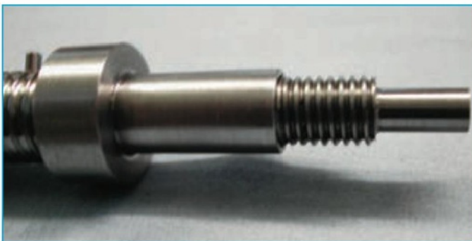
6. The top end of the ballscrew showing the extension for locating the bearing and the coupling to the stepper motor.
