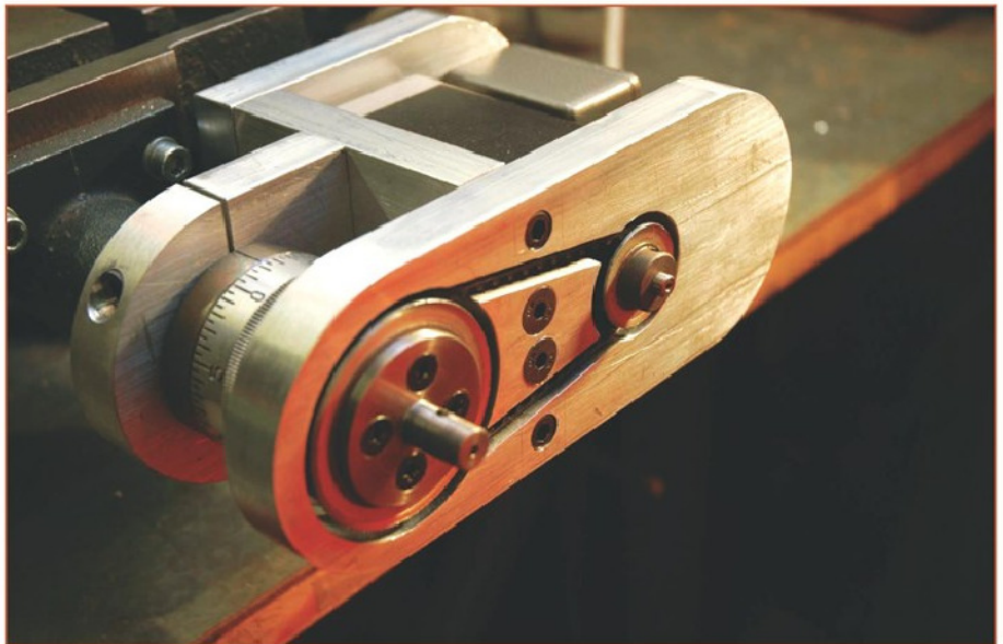
1. Finished drive before refitting the handwheel and chip guard over the motor.
