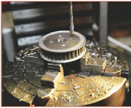
3. Drilling holes to attach the leadscrew extension to the pulley.
