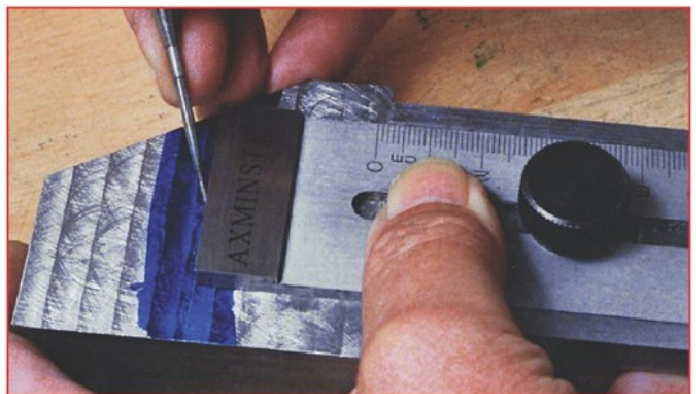
16. Marking out the cutting line to make two off clamp 5 from a piece of waste steel.
