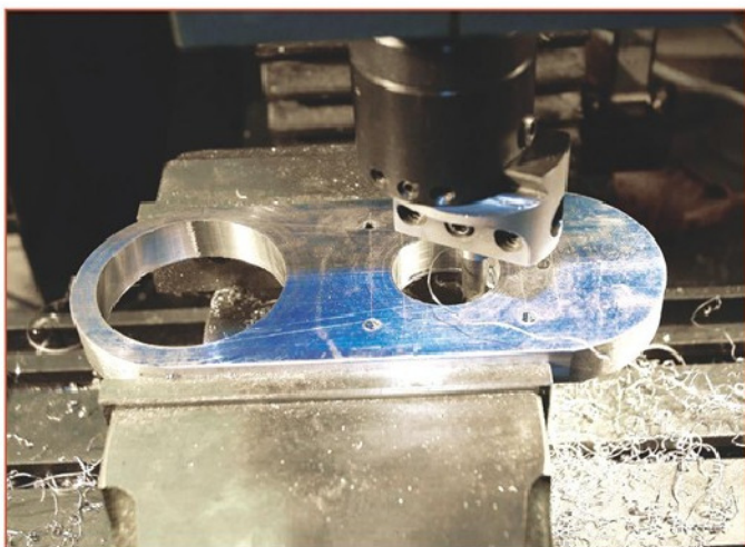
11. Boring the pulley cut outs.
