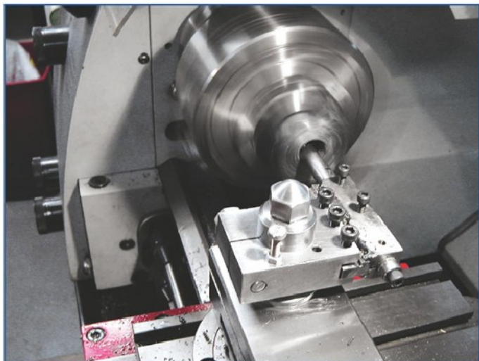
(Above left) 5. Boring the ballnut housing in the four-jaw.
