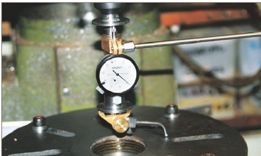
9. Device in use on mill to set head vertical.
