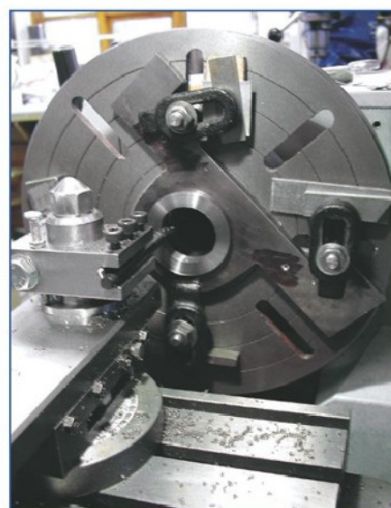
13. X axis register plate, boring the ring on which the bearing housing will locate.
