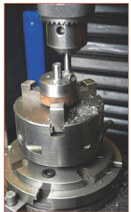
5. Countersinking the holes.
