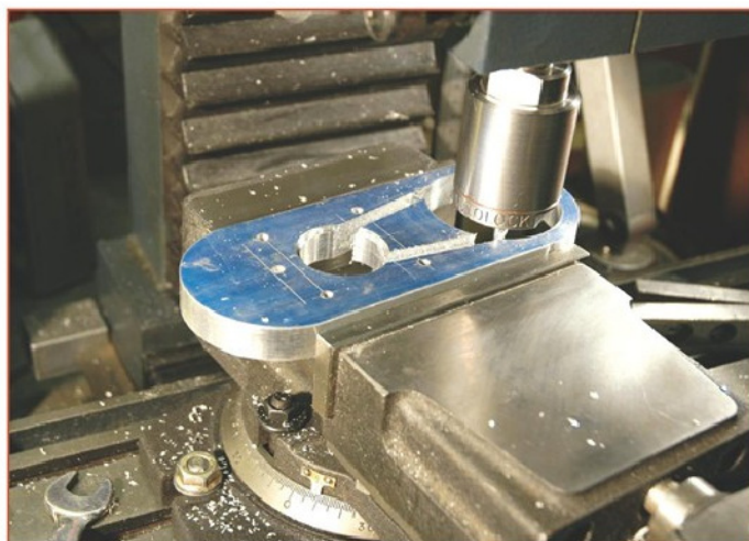
12. Cutting the 9degree belt slots.
