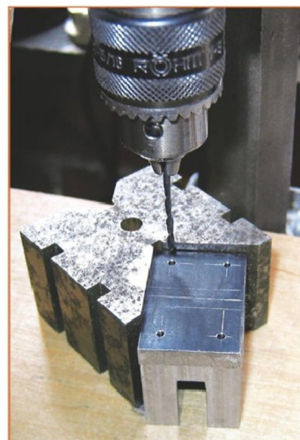
14. Spotting holes using a Vee block.
