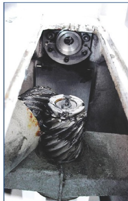
9. The knee casting showing the rear bearing housing for the Y axis mounted on the levelling plate. Two levelling grub screws and two fixing cap screws for the plate can just be seen above the bearing housing.
