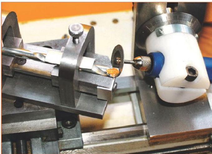
18. Masonry drills can be sharpened, but note the angles.
