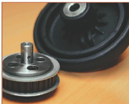
9. The finished lead screw extension.
