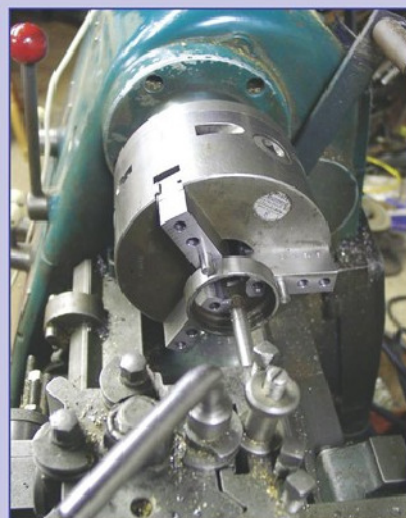
Gripping a ring via the pins allows the jaws to be trued up with a boring bar.
