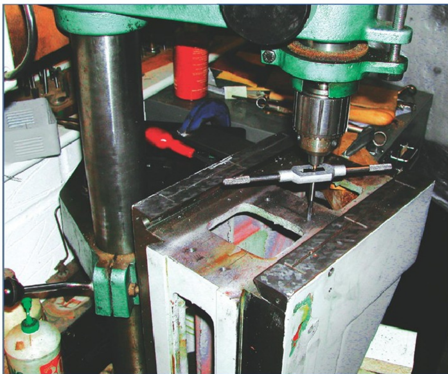
8. Knee tapping! My pillar drill is at its limit here to drill and tap the four fixing holes for the levelling plate which locates on the inside of the knee and takes the rear bearing housing for the y axis.
