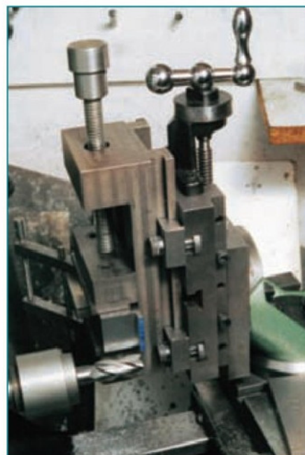
3. Machining the second end with its step for locating the jaw plate.
