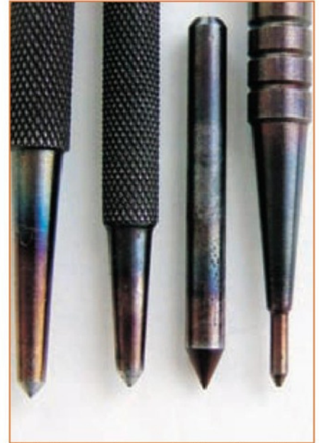
7. A closer look at a selection of punches correctly tempered to brown.
