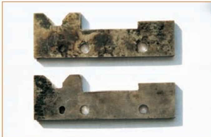
5. Two mild steel templates which have been case hardened.
