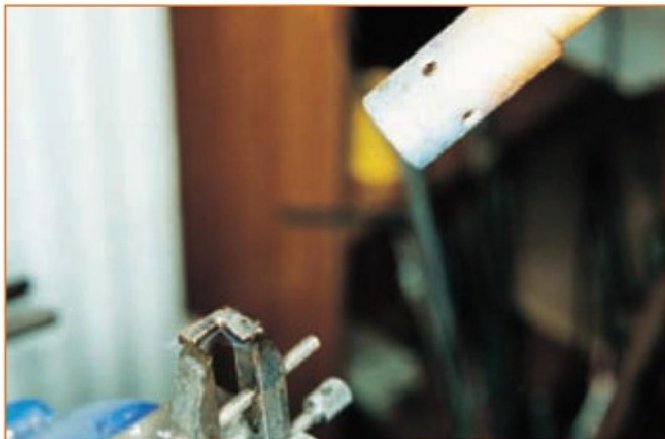
4. The flammenwurfer in action, tinning a piece ready for soft soldering.
