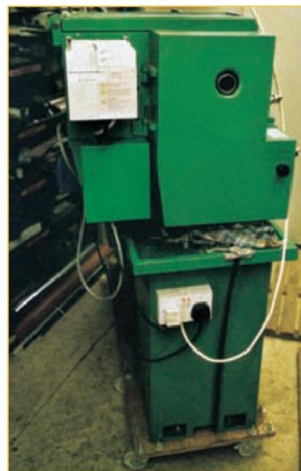
2. Electronic box located to rear of machine. Also shows lathe mounted on castors for easy movement within garage.
