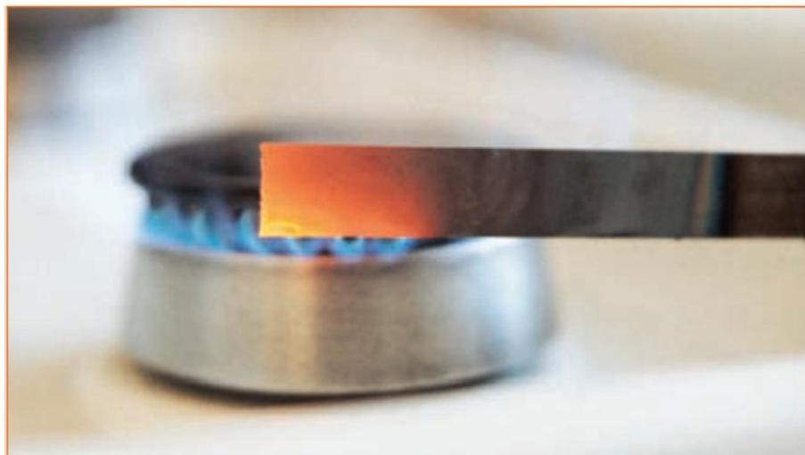
1. Heating a steel strip in a gas cooker flame, note the beginning of a piece of scale..
