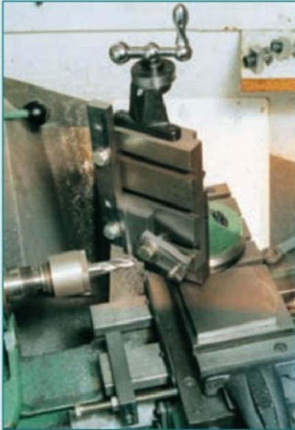
4. The vertical slide is set at 45 degrees to machine the vee in the jaw plate.
