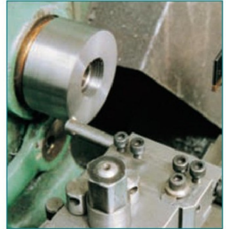
5 Skimming the outer diameter of the chuck adaptor using a modified boring bar.
