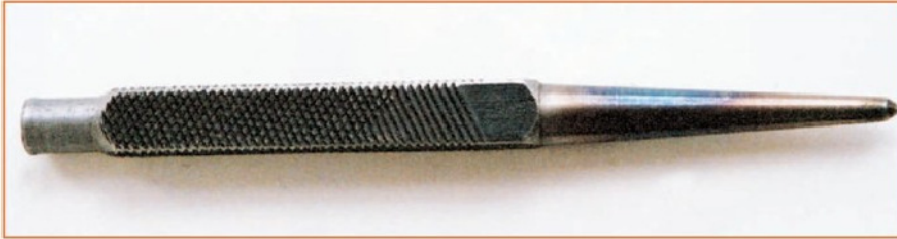
6. A square file which has been softened and made into a centre punch by re-hardening.
