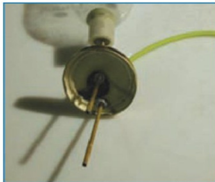
2. Underside view of lid showing delivery and return tubes and threaded parts.
