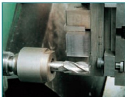
2. Surfacing the first end of a jaw.
