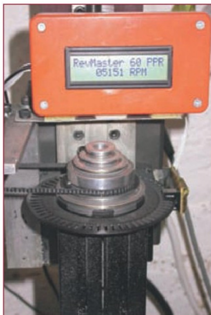
4. Sensor fitted to Taig mill using slotted disc.
