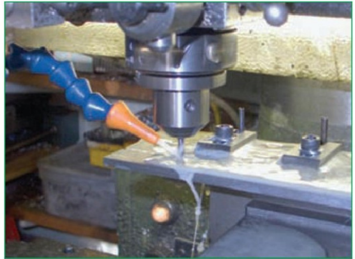
5. Machining groove in base.
