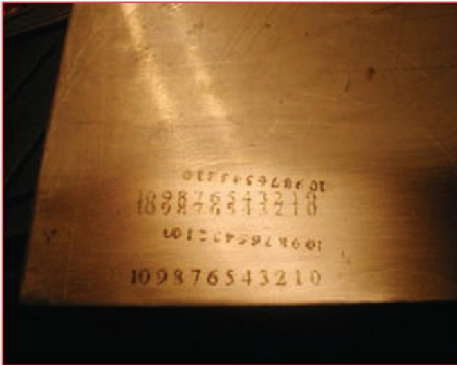
8. Results of electrolytic etching trial.
