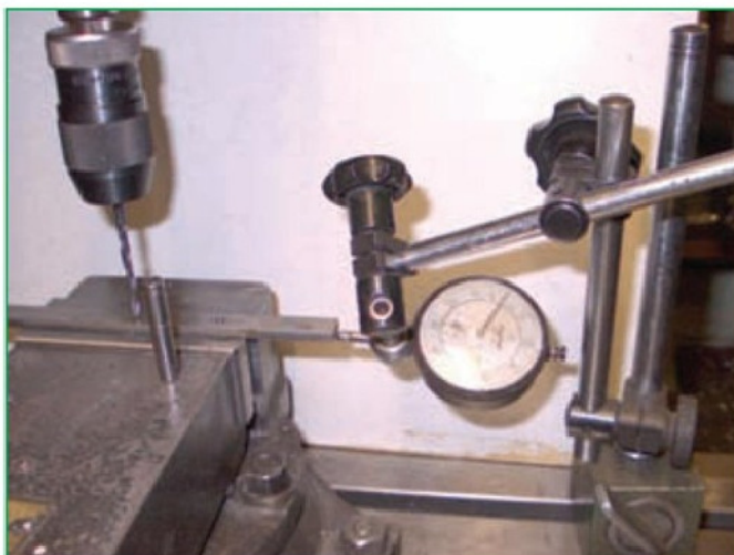
2. Setting piece removed, work moved to zero clock reading.
