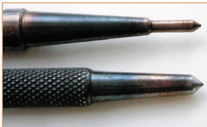
2. Two correctly tempered punches. Photo by Pauline Loader.
