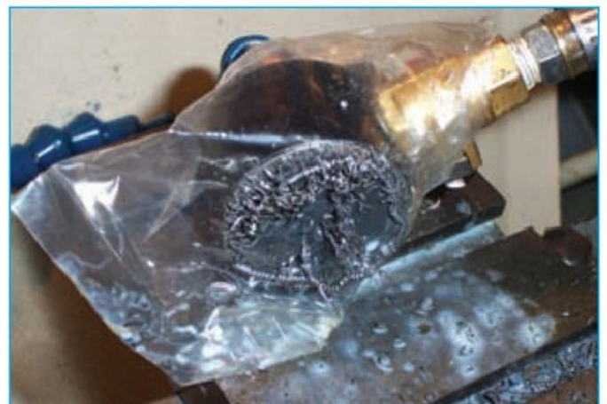
3. Use of polythene to assist in the removal of the swarf.
