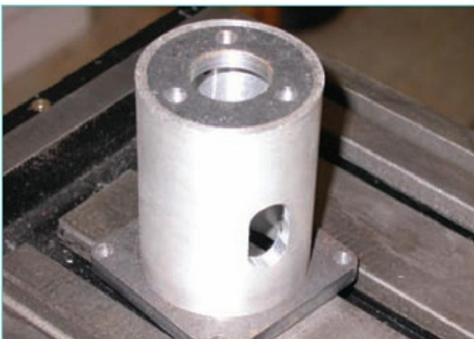
2. Stepper motor mount, as used for rotary tables etc.
