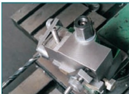
13. Collars and similar can also be drilled at an angle.
