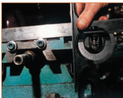
4. Checking alignment of bearing bracket fastenings for transfer to gear-train backplate.
