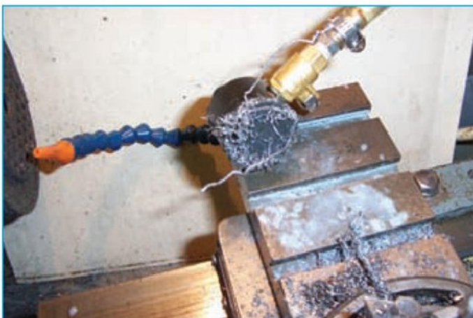
2. Swarf attracted to the original magnetic base.
