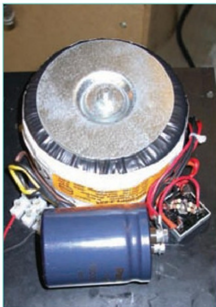
11. Transformer and associated components fitted to backplate.
