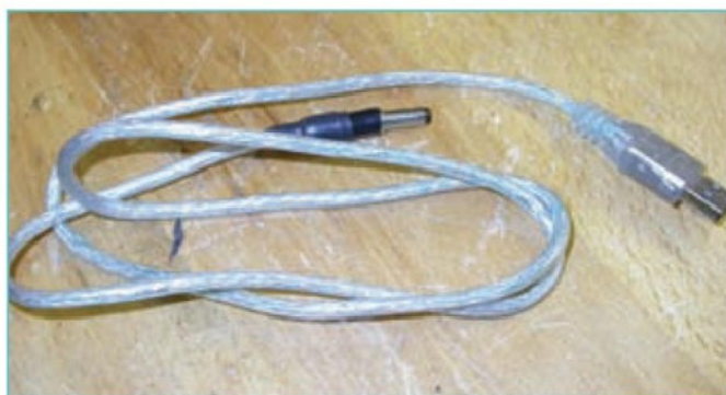
14. Modified USB cable provides 5V supply.
