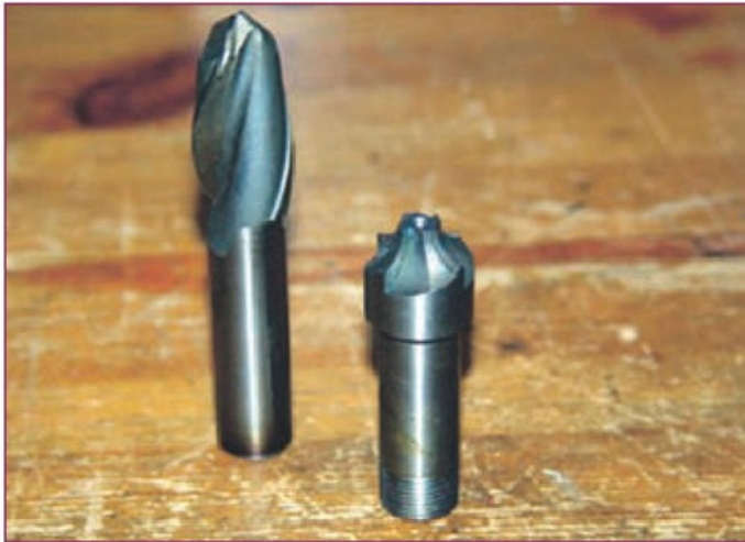
4. Form cutters for top tool (right) and bottom tool (left).
