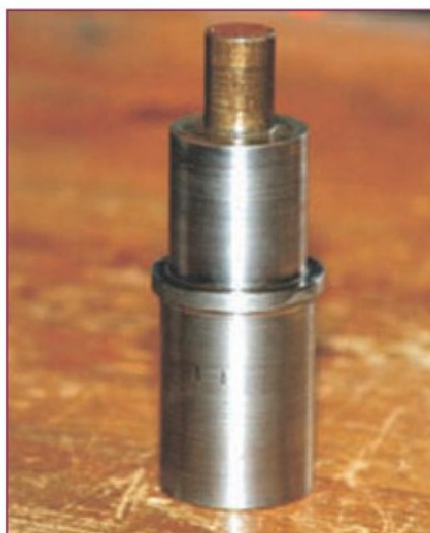
7. Top tool mounting mandrel.
