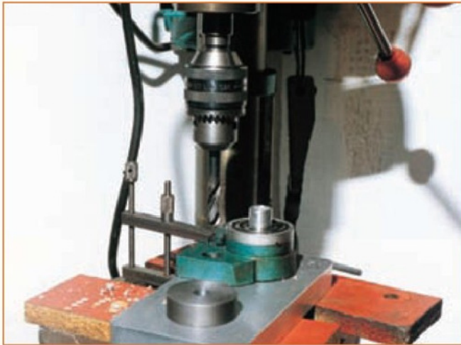
5. Drilling holes in gear-train backplate using lead-screw bracket as template which has been located with a mandrel axially and set radially to the angle of the holes as measured on the table end.
