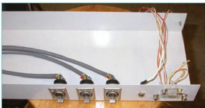
13. Showing wires and connectors fitted to lid.
