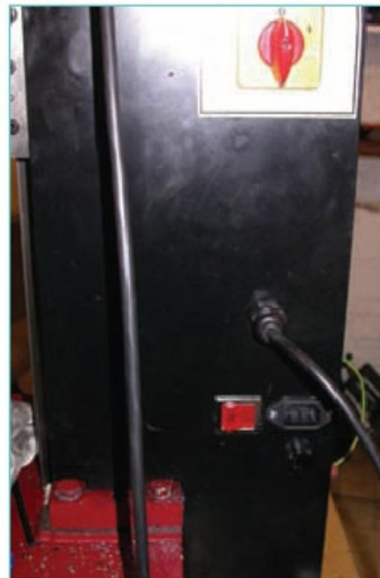
9. Showing mains rocker switch, fuseholder and IEC socket fitted to housing.
