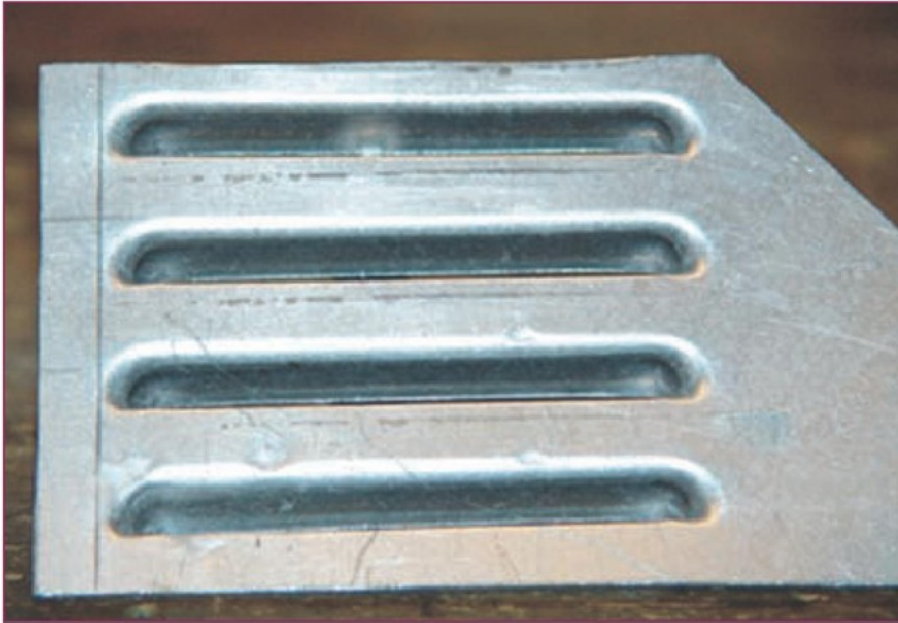
1. Rear view of louvres i.e. upper surface of workpiece.
