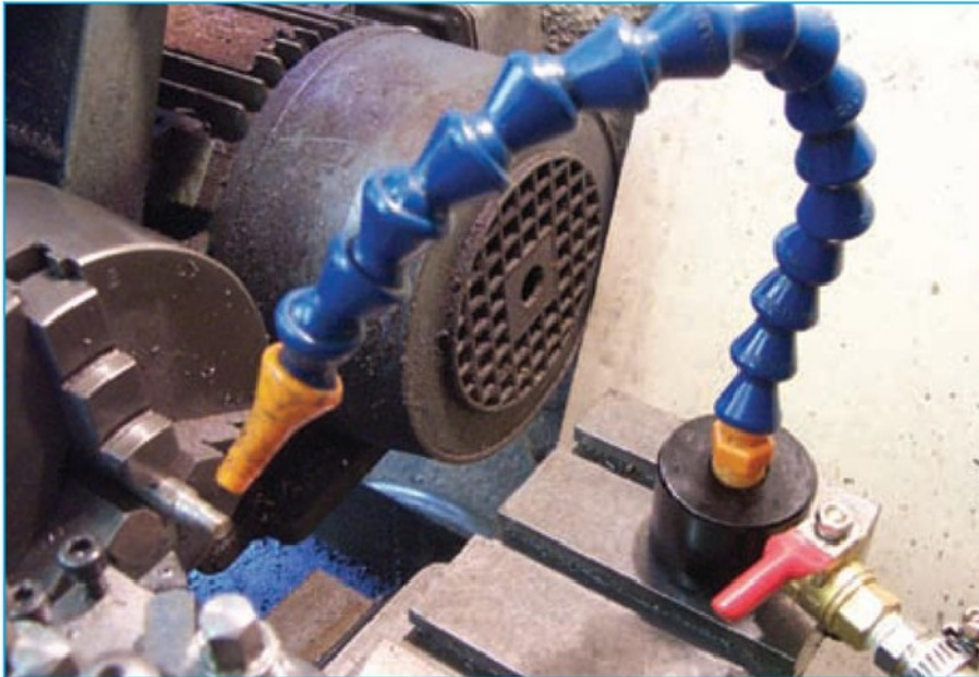
1. Original base with "Lockline" spout.
