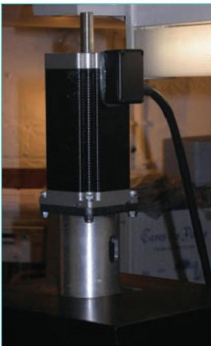
8. Z axis motor, located at top of head.
