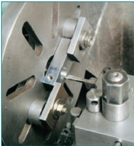
8. Boring the bush holder to size
