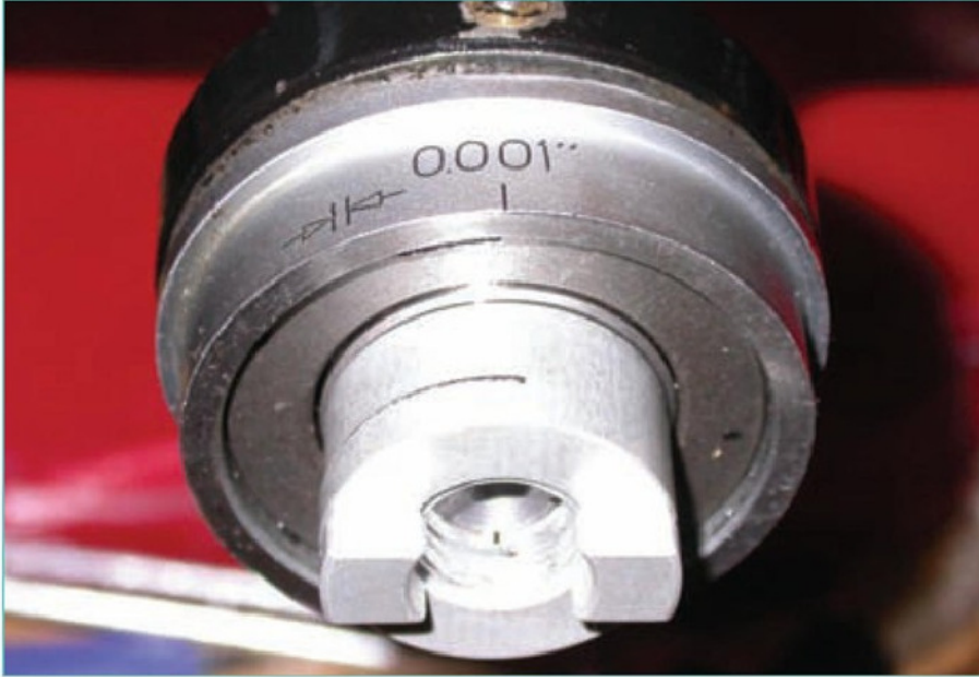
1. One half of the Oldham coupling has been threaded to allow endfloat adjustment.
