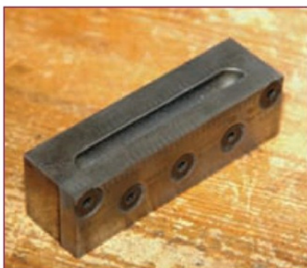
6. Upper surface of bottom tool.
