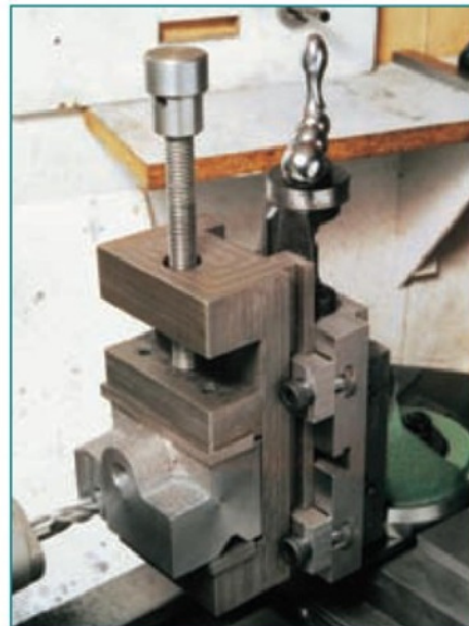
5. A toolmakers vice mounting arrangement gives flexibility over the position of the vice. Very helpful on a small vertical slide.
