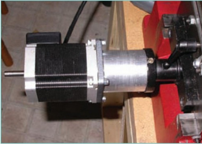
6. Y axis motor in place.
