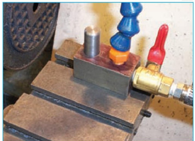
7. Close up showing new base mounted on the cross slide.
