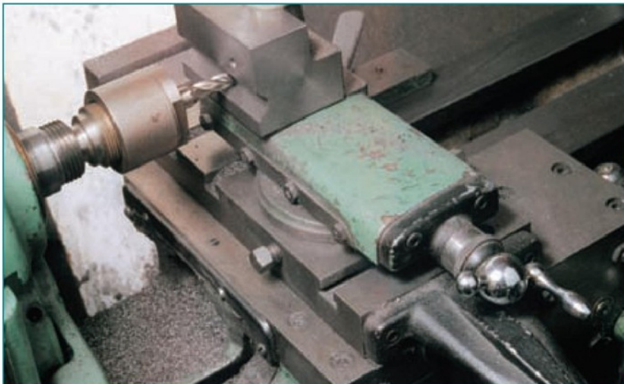
4. The Vee is machined using progressively smaller end mills, and doing this whilst on the top slide ensures that it is at centre height.
