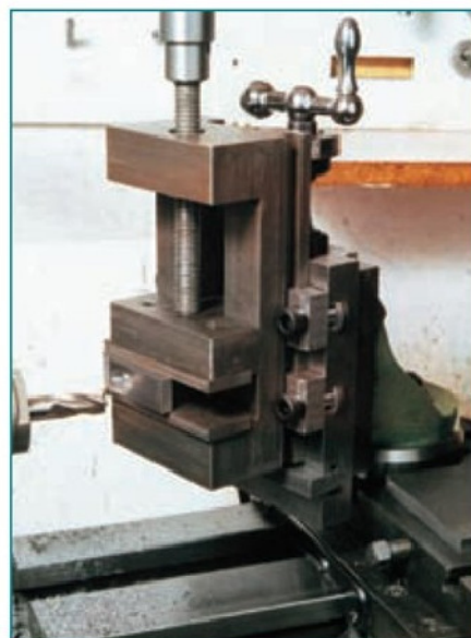
6. Being able to rotate the vertical slide is a definite plus over using a conventional vertical milling machine.
